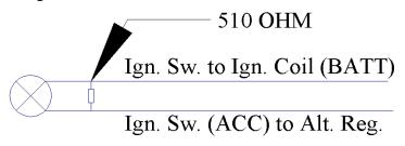
The  $510\Omega$  resistor can be found on the Mustang white gauge pod. Carefully clip the resistor leads leaving them as long as possible. You may want to protect this junction with tape, etc. solder the wires (with resistor soldered together ahead of wire ends).
