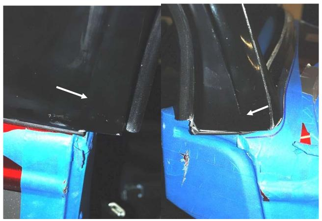
Align the front and rear edge of the door cut out with the molded trim line on the Hard top and make sure that the front windshield area sits on the body properly.
