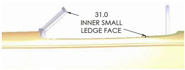
In order for the soft top to mount correctly on the car, the angle of the windshield needs to be correct. Make sure the top corner of the windshield to the top rear of the door opening. If necessary slot the holes slightly for the windshield.
