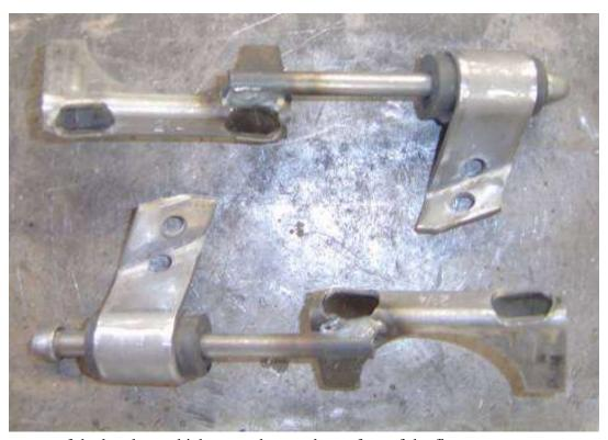
Grind the corners of the brackets which protrude past the surface of the floor.
