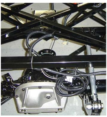
Drape the harness over the rear axle straight back to the rear of the frame so the harness can "T" at the back of the frame.
