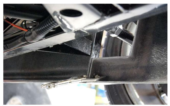
Clamp the nose cone to the front of the body section so that the bottoms are flush and the outside trim pieces align.
