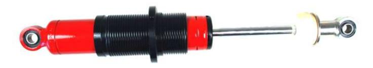
Slide the coil sleeve over the body of the damper beginning at the end which has the rubber bump stop. The unthreaded end of the sleeve goes first so that it will sit on the snap ring on the shock body.
