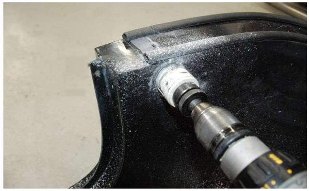
Use a 1.75" hole saw to drill a hole at each of the marks.
