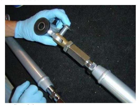
Install collar onto adjuster clevis.
