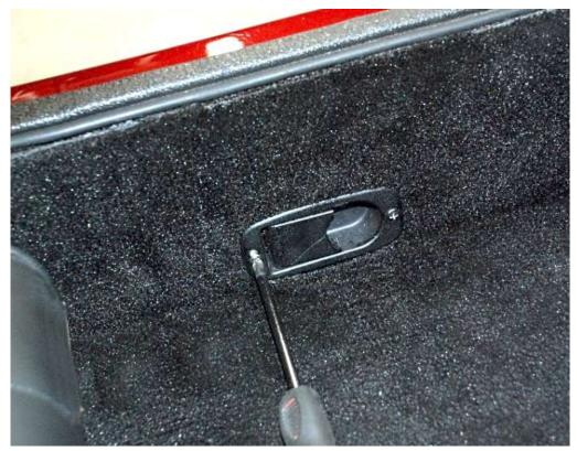
Attach the handle to the aluminum using a Philips head screwdriver and oval head screws.
