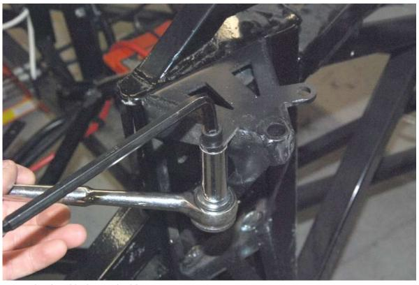
Install 3/8" socket head bolts on the hinge standoff as hinge stops.
