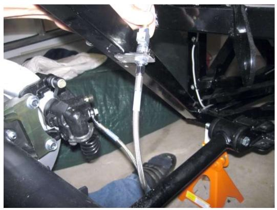
Attach the flexible brake line to the brake line frame mount by hand so that you can make sure that the brake line is not tight. If necessary move the brake line mount to a new location so that the flexible line will reach without being tight. Keep in mind that the axle is hanging down so this is the maximum it
