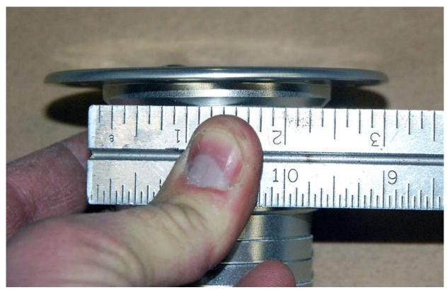
Use a ruler to measure the OD of the cut-out needed for the fuel filler cap.
