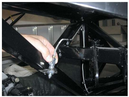
Hand tighten the rear brake line to the end of the brake line mount assembly and position the mount on the frame.
