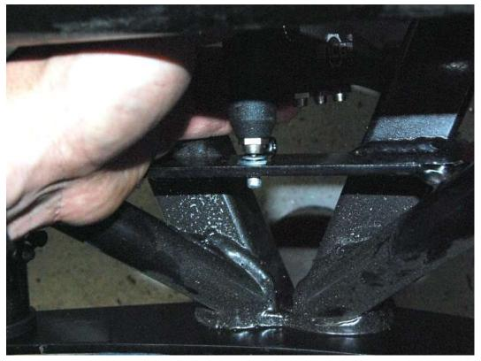
Rivet the line clip to the back of the lower control arm mount plate.
