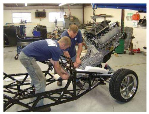
With the help of some friends install the engine and transmission into the chassis. Make sure to bolt the Energy Suspension engine mounts to the engine before installing the engine. If the chassis is powder coated you may want to protect the engine bay down tubes.
