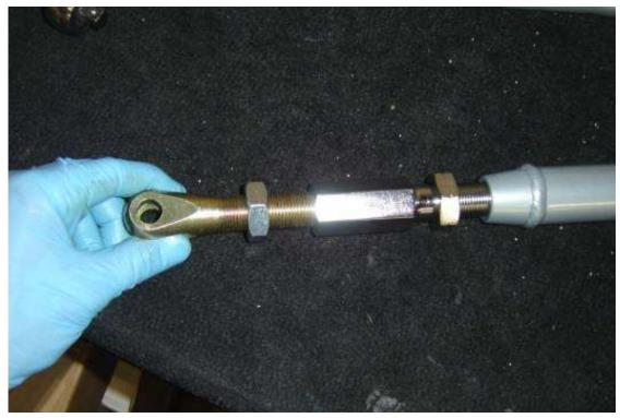
Screw the Clevis into the adjuster in the lower control arm.
