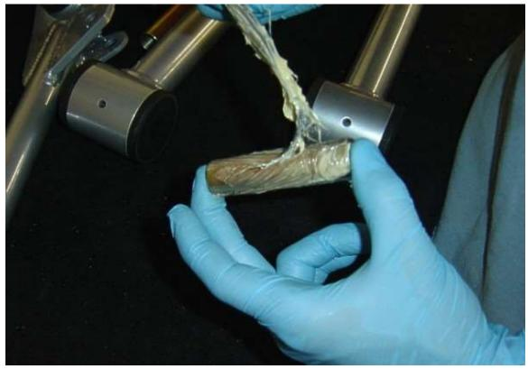
Apply grease to front lower collar sleeve.
