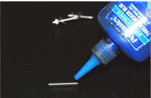
Put a drop of lock-tite on one end of the threads for the bezel studs.
