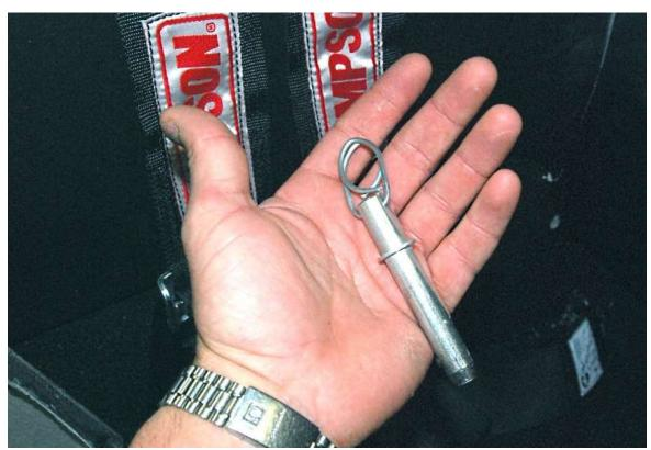
The quick release pins can be used as is but a large 1.50" hole must be drilled in the rear cockpit cover for the ring or, squeeze the pin ring in a vise and a smaller 1" hole can be made. The hole is behind the seat and can not be seen.
