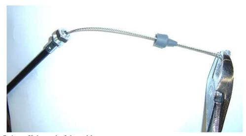
Cut the barrel fitting off the end of the cable.
