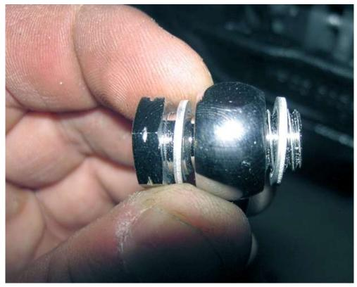
Place a crush washer on either side of the banjo fitting on the flexible brake line.
