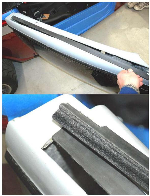
Carefully push the felted rubber seal onto the top of the door. If necessary use tin snips to trim the ends so that they can push all the way on. If you can not push it all the way on, check the thickness of the top of the fiberglass door. It can be no thicker than  $\frac{3}{16}$ " for the felted rubber seal to go on. Grind the inside of the door if necessary to remove material.
