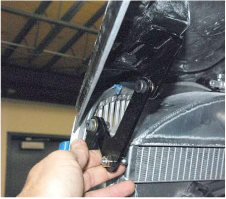
With the hinges mounted on each side and hood in place, rotate the hinge up so that the hood mount bracket touches the hood.
