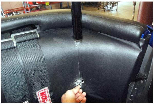
Install the rear cockpit cover and test fit the release pin. If necessary open the hole up slightly.
