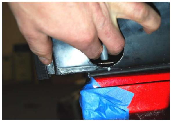
On the rear of the top, use a marker in the hole saw holes to mark the body through the ½" drilled holes.
