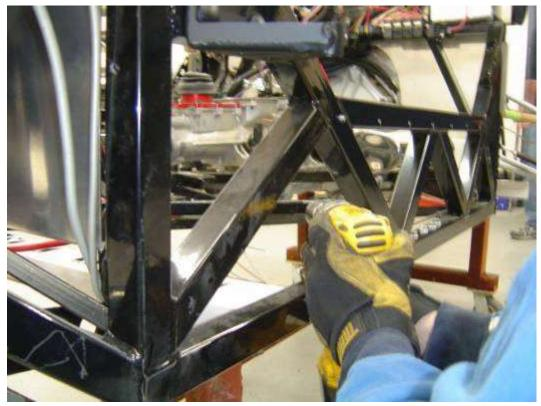
Remove the exhaust mounts and drill the frame where you just marked with a 3/8" drill bit.
