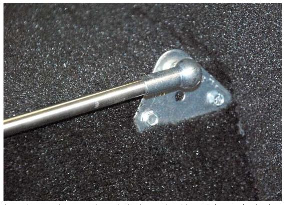
Reattach the trunk prop rod mount to the trunk aluminum using either 3/16" rivets or the aluminum screws.
