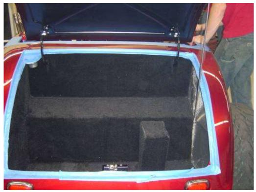
Carpet the trunk. Start with the center section of the trunk. You will also have to slice a little section out for the prop rod stud and the trunk latch bracket mount.
