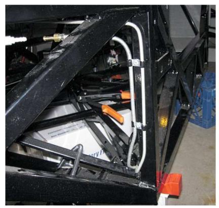
Run the fuel line down the back of the 1.50" tube and then bend and snake it over the  $\frac{3}{4}$ " tube and under the top 1.50" tube.
