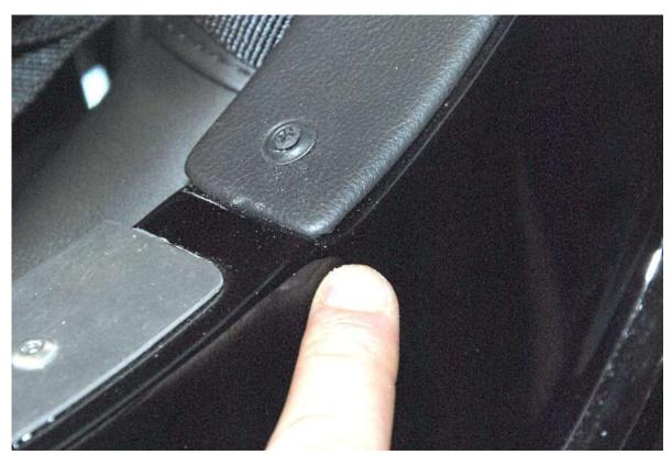
The rear cover can either be installed with riv-nuts,  $^{3}/_{16}$ " rivets or black trim screws.
