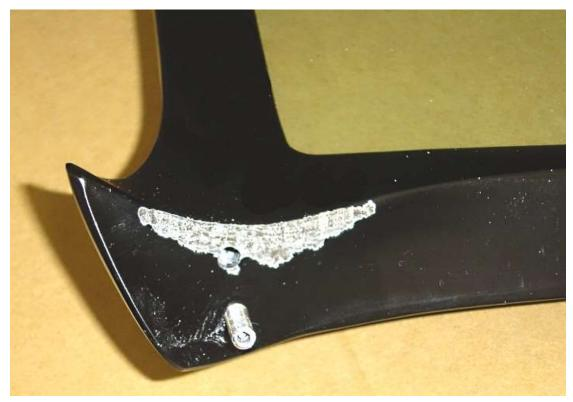
If necessary remove material on the windshield so that the correct angle is reached and the windshield sits flat on the gasket/body. This windshield had a small ridge in the area shown that had to be removed.
