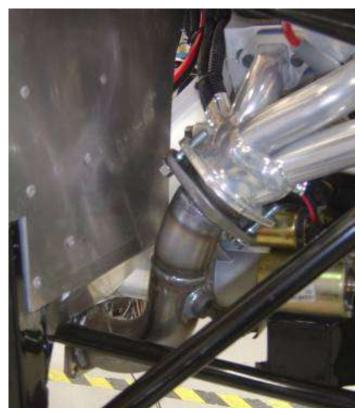
Attach the shorty pipe to the shorty header coming off of the engine. Do not fully tighten this ball and socket joint yet.
