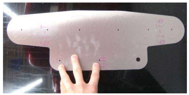
Lay the template on the dash and either mark the centers of the holes or clamp the aluminum to the dash and drill through the holes for the ignition, horn, headlight and gauges.
