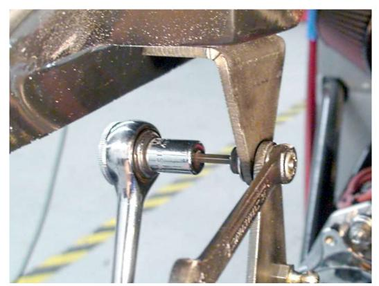
Remove both upper hinge pins and remove the hood.
