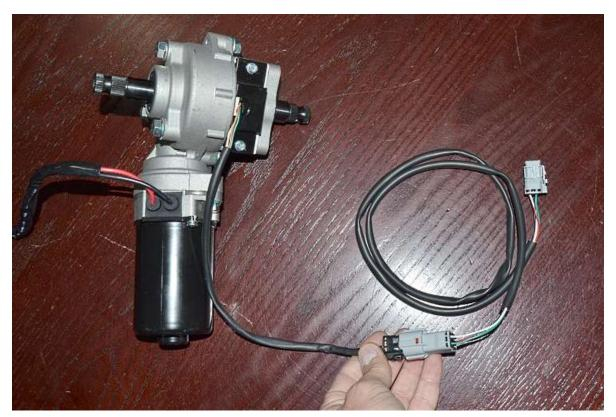
Attach the controller harness to the motor.
