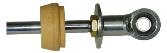
Slide the rubber bumper about two inches down on the shaft.
