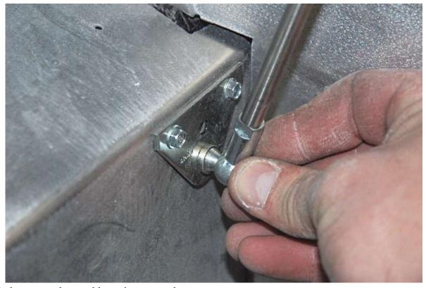
Attach the prop rod assembly to the prop rod mount.
