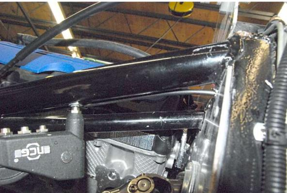
Mount the cable to the frame using small insulated line clips and self tapping screws or  $^{3}/_{16}$ " rivets near the firewall.
