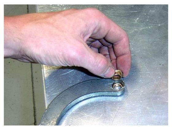
Temporarily attach the trunk hinge arms to the frame. Do this by installing the bronze bushings in the trunk hinge arms.
