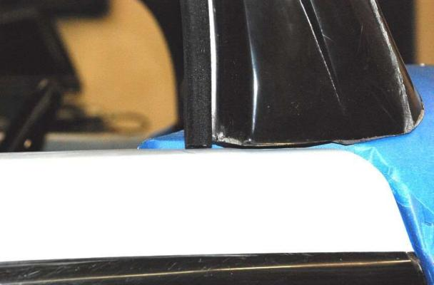
Starting at the back of the window opening as close to the door as possible, hanging below the Hard Top, push the weather-stripping onto the flange around the door opening to the front of the door, again hanging below the Hard Top as close as possible to the door.
