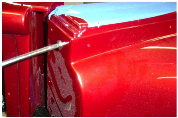
Install the rear cockpit cover temporarily with clamps, black trim screws or masking tape.
