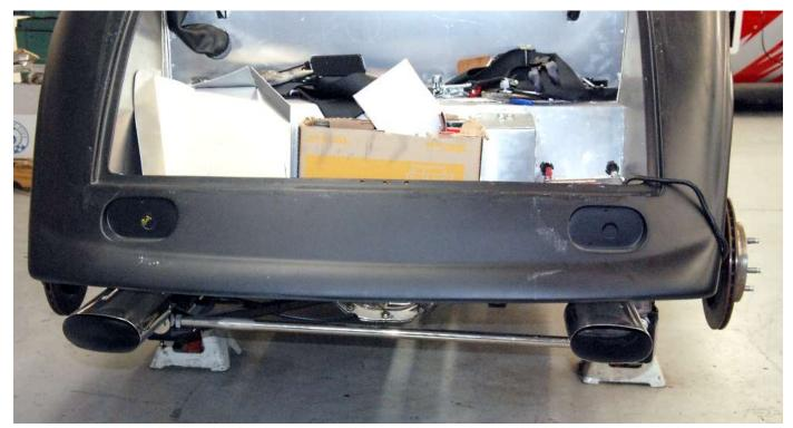
Attach the exhaust tips and locate them so that they are below the tail lights. Move the rubber hanger if necessary.
