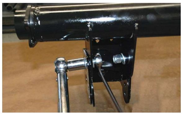
Tighten the two short bolts. Torque to Ford Specs 75-95 Nm (55-70 lb-ft).
