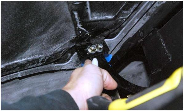
Hold the hinge mounts on the trunk so that the carriage bolts are centered in the slots and the mount is on the trunk mounting area.
