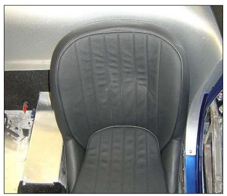
With the body still on, set the rear cockpit fiberglass piece in place to determine the seat location. Position the seats in the chassis and adjust them to where you would like.
