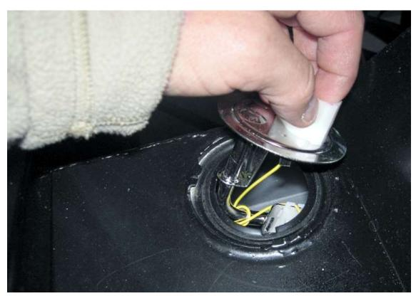
Insert the Fuel level sender into the tank, the float will point towards the middle of the tank once the small locating tabs are in the slots.
