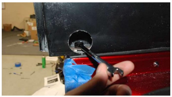
Place the Hard Top back on the body and attach it at the locations just behind the door using the  $\frac{1}{4}$ " bolts provided and a  $\frac{3}{8}$ " wrench. Double check that the molded trim line on the top lines up with the door edges and that the front windshield area sits on the body properly.
