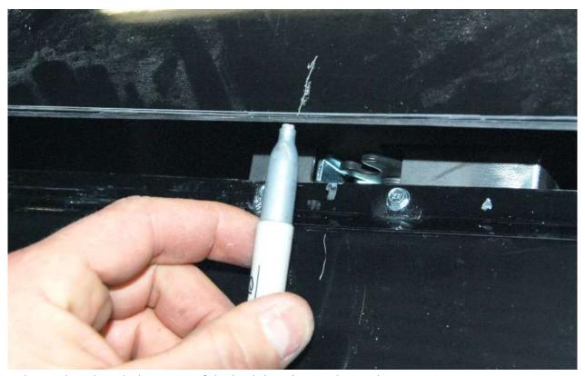
Close the trunk and mark the center of the latch location on the trunk.
