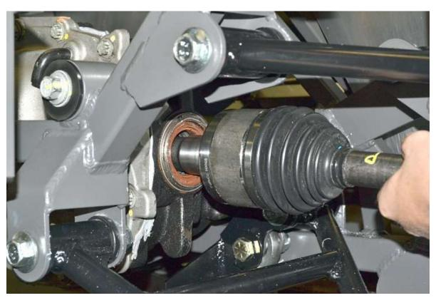
Starting with the left side using the correct axle, push the inner CV joint into the center section.
