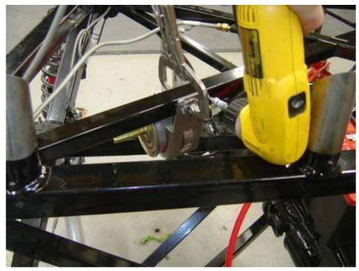
The fuel filter is installed near the battery behind the passenger seat. If necessary slide the tank back a bit then drill and attach the filter to the frame with  $^3/_{16}$ " rivets.
