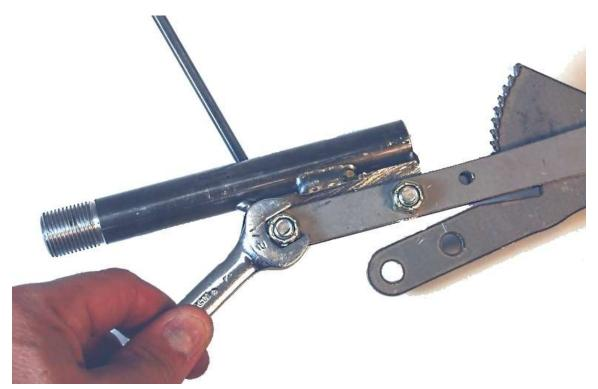
Slide the lower handle between the ratchet to handle mount plates and bolt the three pieces together using the two  $^{5}/_{16}$ "x 1" button head screws.
