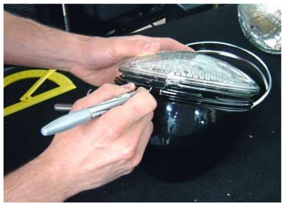
Use a marker to mark the side of the bucket if the locating bulges on the side of the bulb do not line up with the notches in the bucket.
