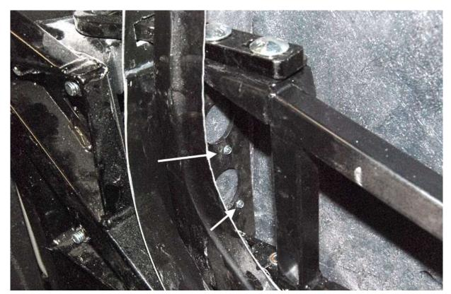
Recheck the alignment of the door then put a couple of the aluminum screws through the door frame rear plate. Spread them apart if possible so the door can not rotate.
