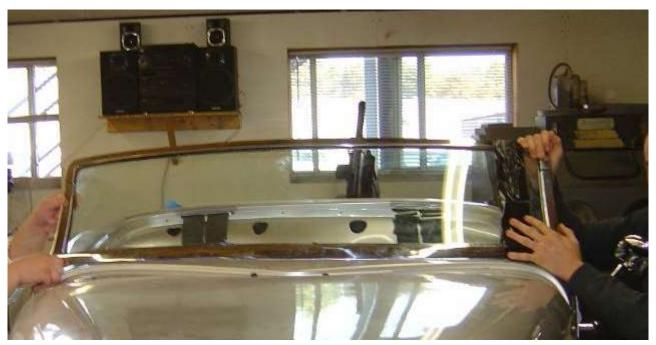
Have a friend assist you and mock up the windshield on the body. Make sure to check the measurements from the door opening to the corners of the windshield to make sure the windshield is square.
