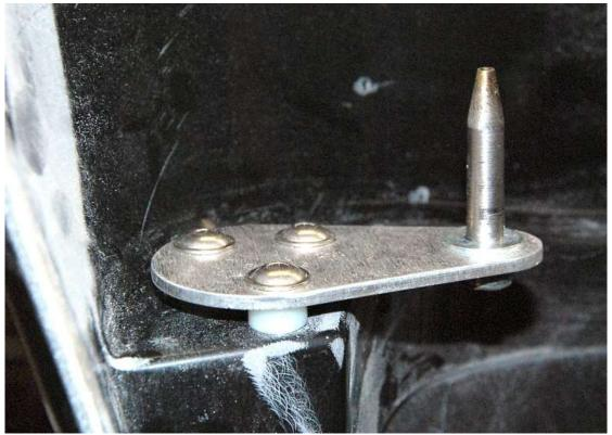
If needed, space the pin mount bracket so that it will go far enough into the receiver.
