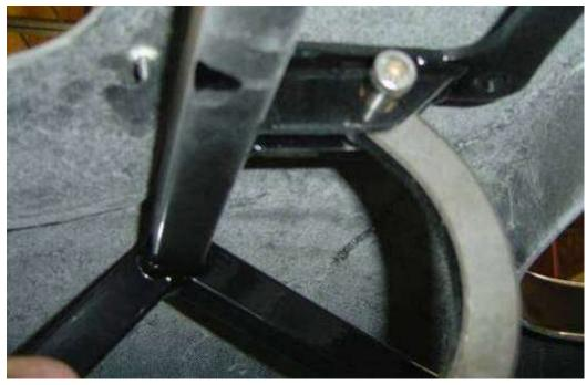
The trunk hinge is attached to the frame with the 1" shoulder bolt. The arm attaches to the frame on the bracket which is located above the fuel tank towards the outside of the vehicle.
