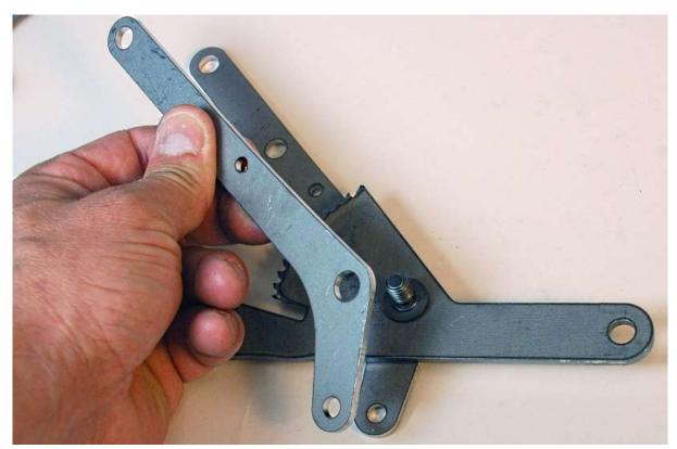
Put the other ratchet to handle mount on shoulder bolt from the other side of the fixed gear.
