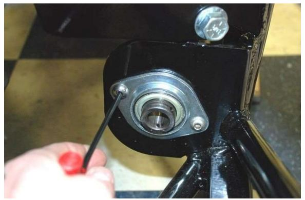
Attach the second flange bearing to the frame bracket using the 5/16" button head fasteners. Install the flange bearing is installed on the front face of the frame mount with the locking collar forward. Do not tighten the locknuts until the steering shaft has been installed so that the bearing is in the correct orientation.
