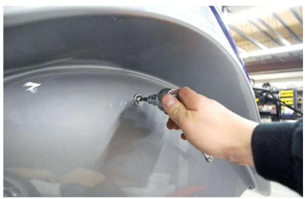
Install the rear wheel well  $^{5}$ / $^{16}$ "x 1.5" mounting screws using the spacer between the wheel well and the frame.
