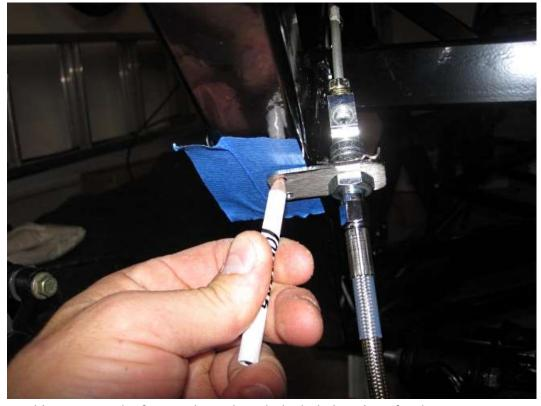
Place some masking tape on the frame tube and mark the hole locations for the mount.
