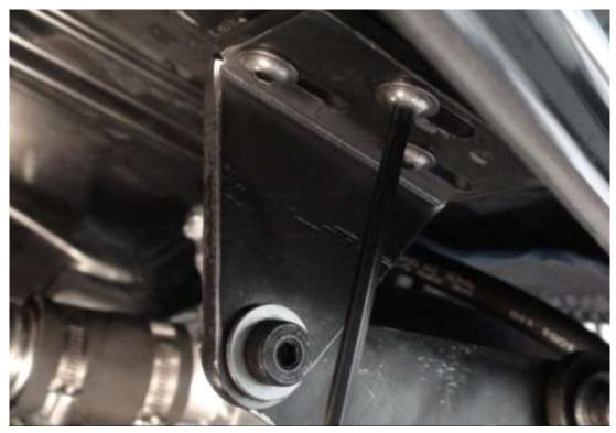
Place the hood on the car and attach the hood mount to the hood finger tight to allow for adjustment.
