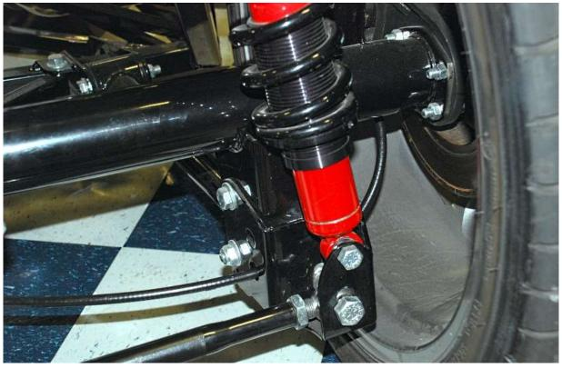
Make sure your routing is out of the way of any moving parts and the cable has slack to move with the axle. Two possible ways are shown below, either in front of the rear shock or through the lower hole in the traction lock bracket.
