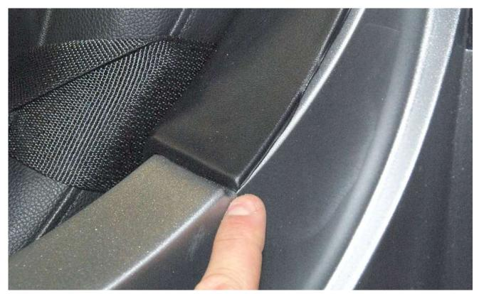
Mark the lower edge of the cover so that it sits down in the body recess at the rear of the door.
