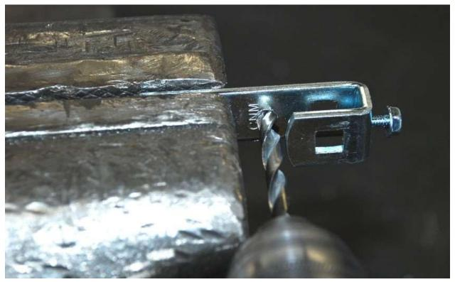
With the lever in a vise or drill press, drill a 1/4" hole in the center of the lever at the points marked.
