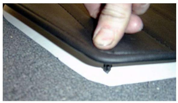
Cut out the panel to make a template then lay it over the door panel and press the trees into the template.
