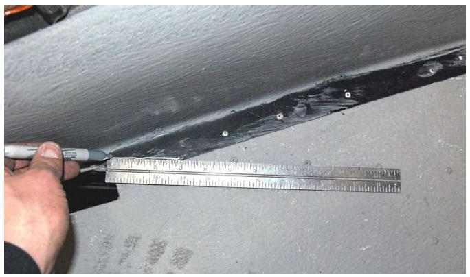
Inside the cockpit, use the rivets as a guide to draw a line on the transmission tunnel. This is the location of the tube underneath that the e-brake handle should hit for the front mount.
