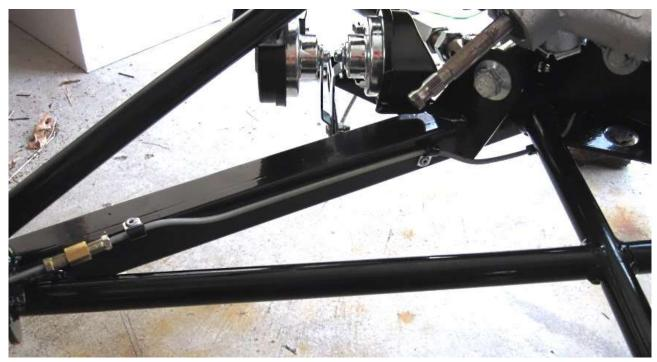
Coming off one side of the brake line union, attach a 20" section of brake line. Route this brake line to the front of the car running along the inside of the 1.5" frame rail.
