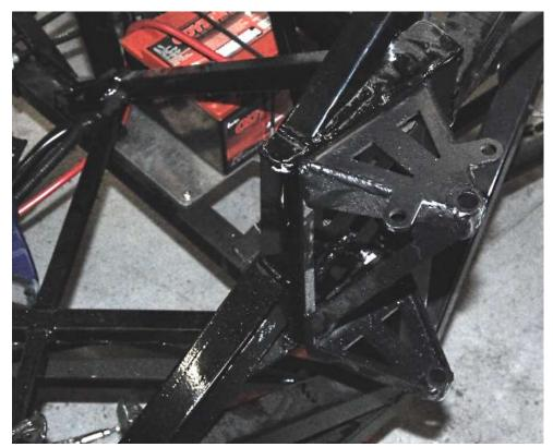
Mount the door hinge standoff to the frame with the small ears at the top using the short ½" carriage bolts and flanged locknuts leaving the bolts just loose enough so the standoff can move.
