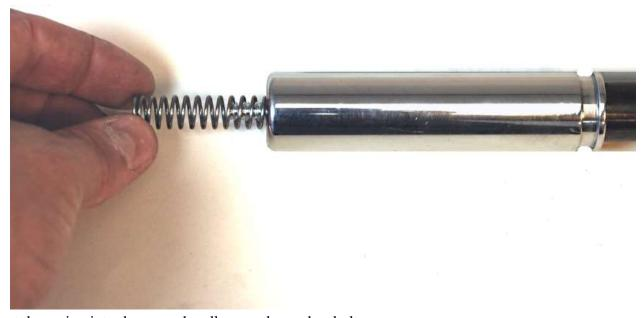
Insert the spring into the upper handle over the anchor bolt.
