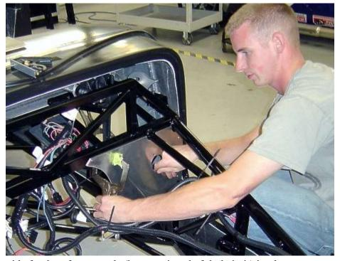
Clamp the driver side footbox front panels (has steering shaft hole in it) in place.
