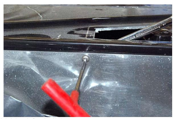
Attach the bolts to the firewall and body.
