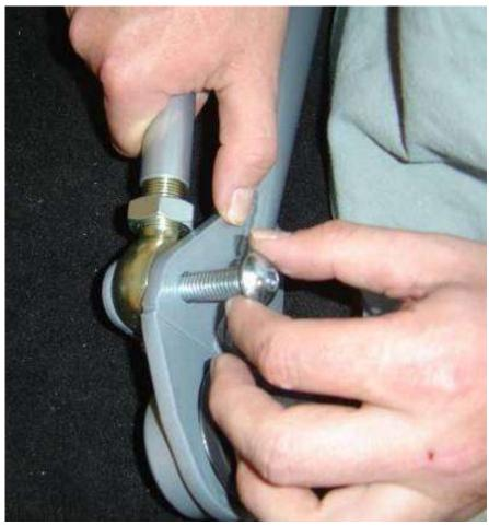
Rod end install on lower control arm
