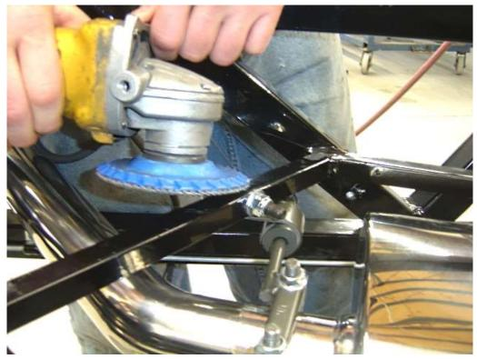
Check to make sure none of the bracket of hardware is above the top surface of the frame rails. If need be, grind anything that is sticking past this leading edge where the aluminum floor must sit.
