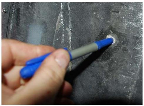
From the underside of the body in the windshield area, use a marker through the ¼" holes drilled to mark the underside of the Hard Top windshield area.
