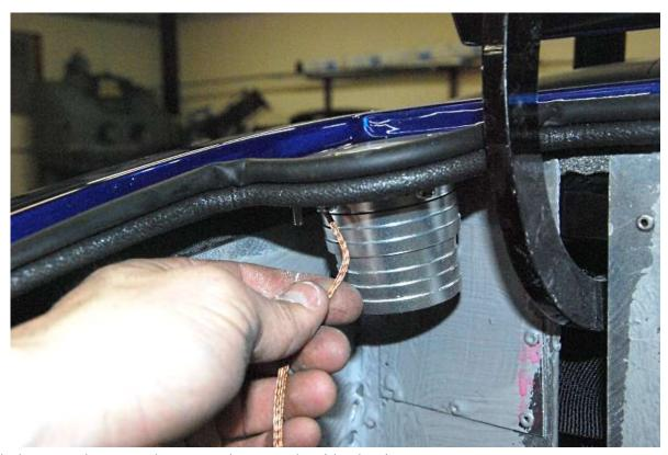
Attach the ground strap to the screw closest to the side aluminum.
