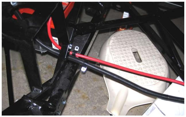
At the back of the cockpit area, go under the 1" tube and over the 1.50" tube.
