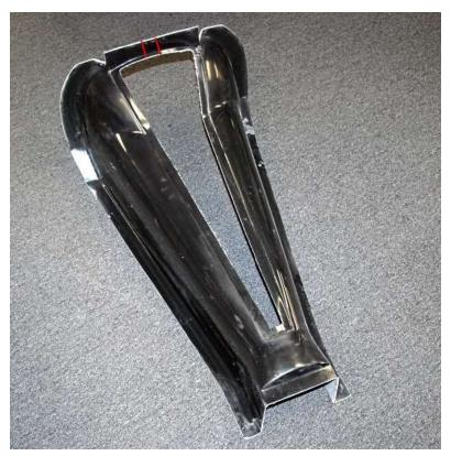
Cut the middle area fiberglass holding the two sides of the transmission tunnel together at the front the same amount measured before.
