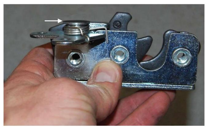
If using the clear zinc latches and it is needed, grind the end of the spring post to give additional clearance.
