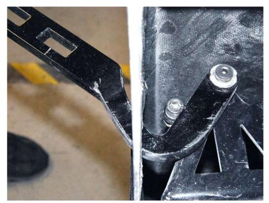
Test the hinge arms to make sure there is clearance between the arm and the body cut-out on the top and bottom. Move the arm through its range of motion making sure that the top arm can contact the bolt stop and also point straight towards or slightly in from where the striker would mount.
