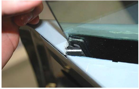
Move the U-channel and push it onto the edge of the glass.
