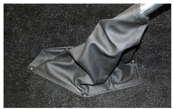
Repeat the drill and screw procedure around the boot so that the boot will seal against the floor.
