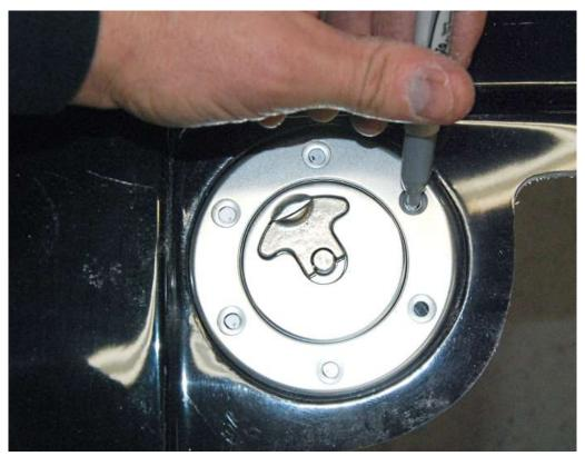
Test fit the filler cap and mark the mounting screw hole locations.
