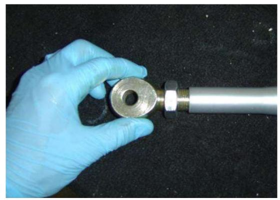
Insert a rod eye into the front of the lower front control arm with the jam nut in place.
