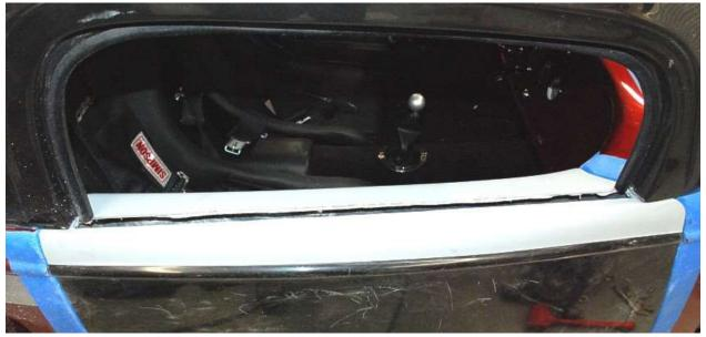
Cut the outer lines marked using a jigsaw or air saw. Check to make sure that the glass will fit in the length of the hole. If necessary cut a little more on the length.
