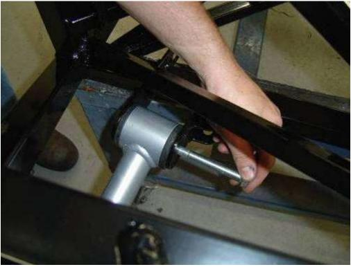
Install the lower control arms onto the frame with the provided hardware, making sure to install this bolt from the center of the car going outward to the side of the car (FFR# 13976 & 13706 & 13751)
