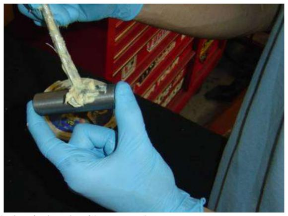
Grease the sleeve for pivot points of the upper control arms
