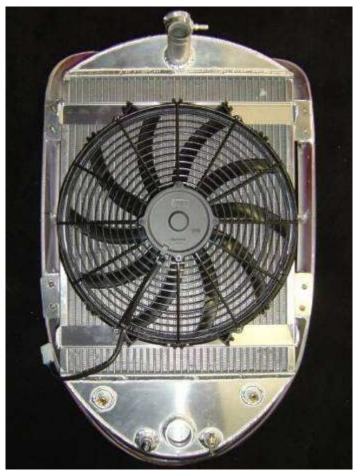
Push on the fan mount sides against the Radiator tabs or hold the fan mount side against the tab with a pair of pliers.
