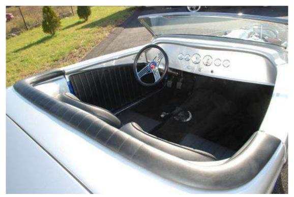
If building the car as a roadster, install the rear cockpit trim piece. The hardtop footprint is covered by this piece if you are going to run both. Attach this piece so you can remove it by using Velcro, silicon or anything of your choice.
