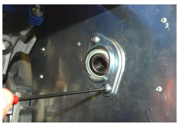
Attach the steering shaft flange bearing to the front surface of the firewall using the  $\frac{5}{16}$ " Button head and locking nut.
