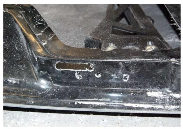
Remove the material between the two ½" holes using a hacksaw blade or jig saw.
