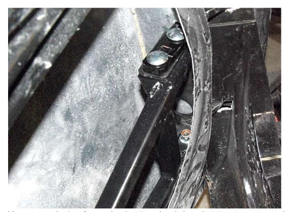
Attach the hinge arms to the door frame using the  $\frac{1}{2}$ " carriage bolts and a  $\frac{3}{4}$ " socket so that the frame can still move around on the arms.
