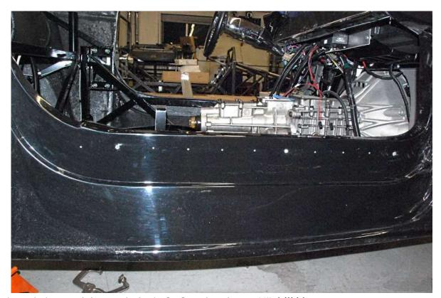
Drill through the remaining marks in the **body** only using an 1/4" drill bit.
