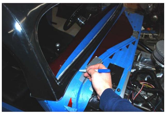
Mark around the inside and outside of the front of the Hardtop on the masking tape.
