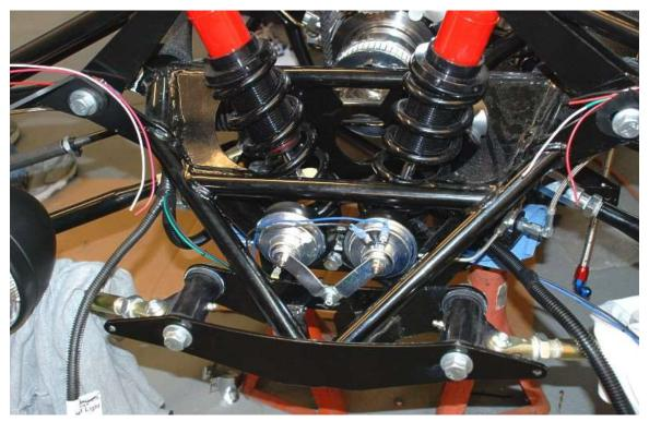
There are a couple of possible locations to mount the Horns. If you plan on running the car without the engine side covers, a hidden location is between the front shocks.
