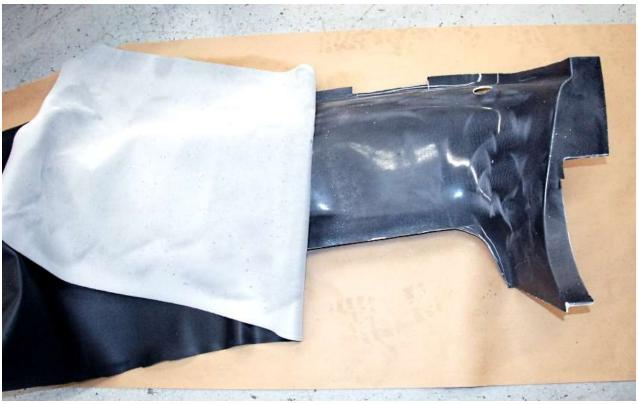
Flip the middle large vinyl piece over in the center and spray glue on the back of the vinyl and the fiberglass.
