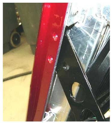
Hold the grill up to the grill frame mounts so that the mounts are on the inside of the grill.
