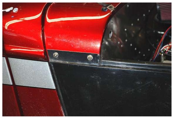
Temporarily attach the panel to the grill with 1/4"-20 flange head fasteners.
