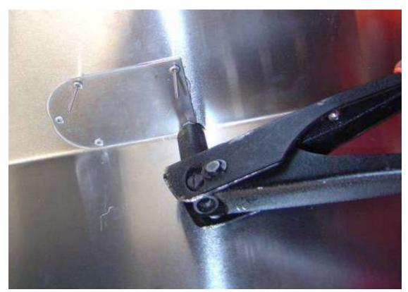
Install the patch panel on the passenger side floor. The drive side hole will be used for the trunk release.
