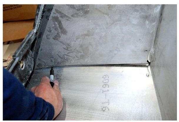
Install the trunk sides. If they are tight on the rear lower body flange, use a marker as a guide and trim off the area needed with tin snips.
