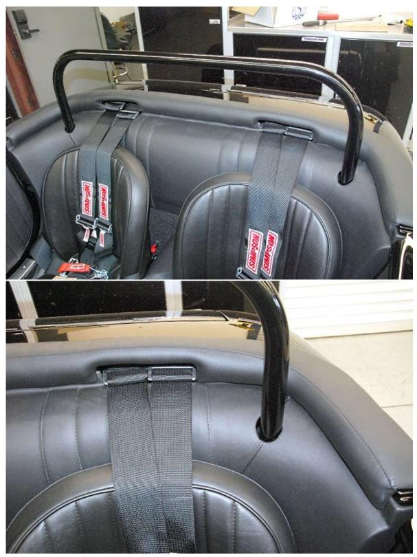
The above picture shows a rear cockpit cover that has been sent out for covering. The sewn lines that are in the seat and the top trim cover were added to the vinyl.
