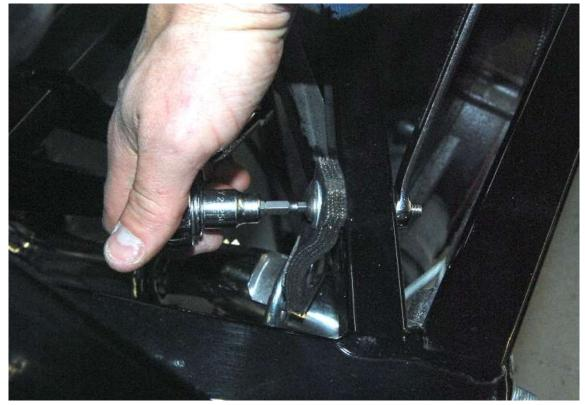
Rotate the rubber hanger and attach it to the tube using the included 5/16" bolt and washers.
