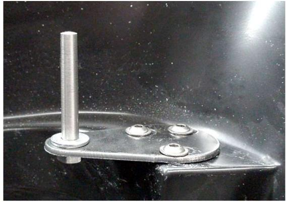
Mount the pin with a washer to the hood mounted bracket finger tight and just loosen the bracket screws to allow for adjustment.
