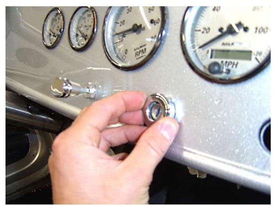
Install the ignition switch in the dash from the backside. Secure it in place with the threaded ring from the front. It maybe helpful to sand the backside of the body if the front threaded ring is not engaging far enough onto the ignition switch itself.
