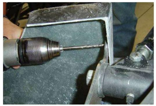
Drill through the frame mount for the nose cone. This is the same piece of steel on the frame which the lower control arm is attached to.
