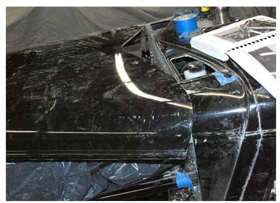
Check to make sure that the hood does not fall off the body at the back of the hood. If necessary, unbolt the lower gas strut mount, position the hood how you would like noting the lower gas strut mount position then drill and remount the gas strut mount in this location.
