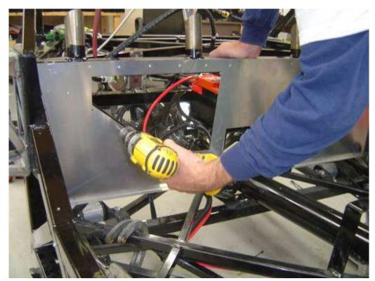
Install the rear cockpit wall piece of aluminum. When installing these aluminum panels, use the 1/8" rivets located in the rivet pack of the kit and the same process s used on the firewall.
