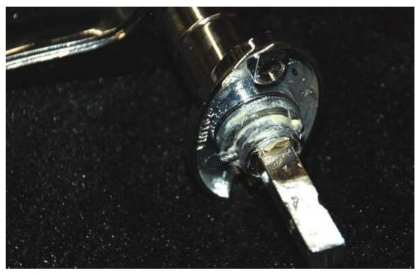
Use Lithium or chassis grease to lubricate the exterior door handle.
