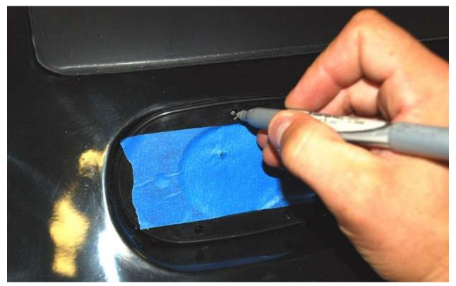
Hold the gasket on the tail light location on the body (the single bezel mount hole goes at the top) and mark the three mount hole locations and the wire hole location.
