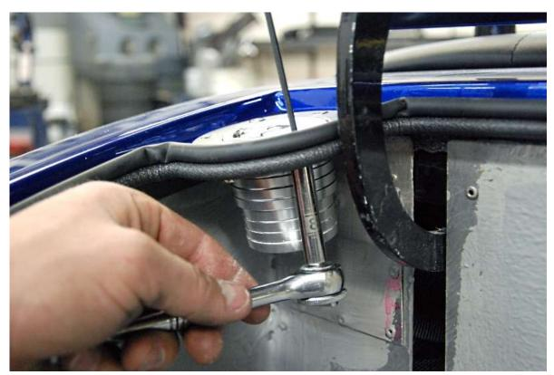
Attach the fuel filler neck to the body at all of the bolt locations.
