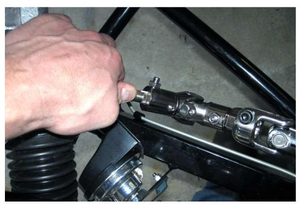
Attach the rack joint onto the steering rack so the screw is on the flat side and the end of the rack is flush to the inside of the joint.
