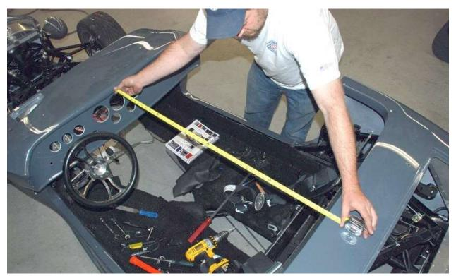
Use a tape measure between the front and rear of the cockpit and set the distance to 45.50" by raising or lowering the body.
