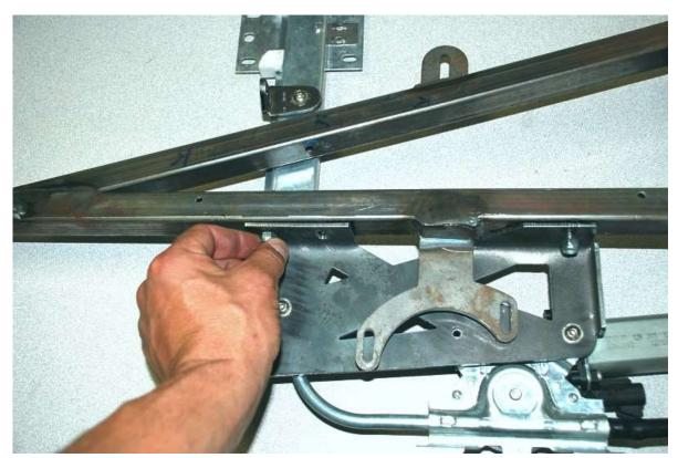
Attach the lower motor bracket to the door frame using a couple of the ½"-20 x 1.50" bolts provided.
