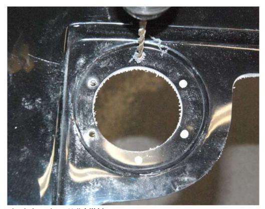
Drill the mounting holes using a 3/16" drill bit.
