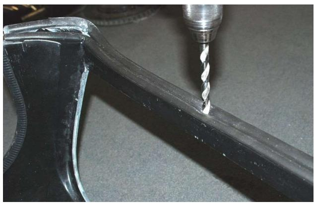
Remove the Hard Top again, put it upside down on the floor, and drill  $^{25}/_{64}$ " holes in the bottom of the Hard Top windshield area in the center between the two weatherstrip pieces at the areas marked. If
