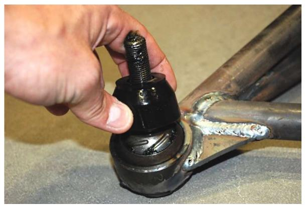
Install silicone dust boot packed in the kit, on the front upper control arm ball joint.
