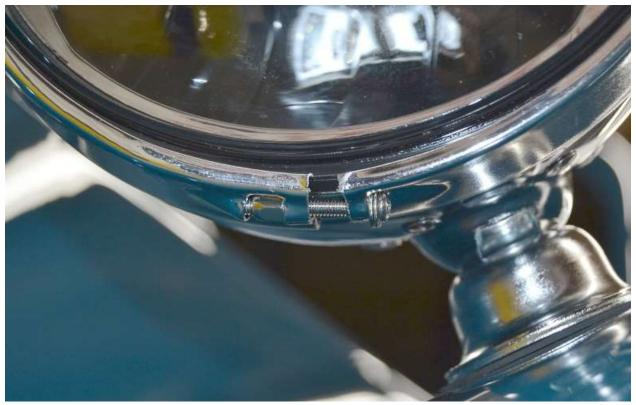
Test fit the bulb and then check the fit of the locking ring, it may be necessary to cut some off the ends so that the ring holds the bulb tight.
