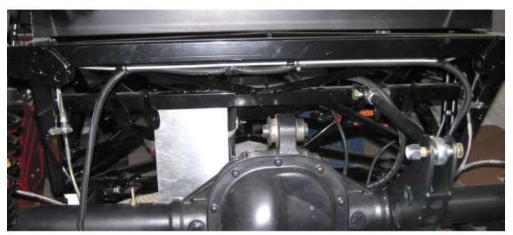
Zip tie the rear light wires to the rear brake line running across the car.
