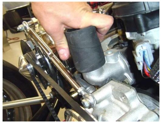
Open one of the radiator hose adapter kits and remove the adapters inside the larger hose and the hose clamps from the outside of the hose. Push the hose onto the engine outlet.
