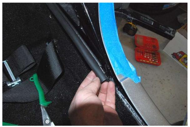
Cut the weatherstrip 1" long and remove 1" of the hard clip leaving the bulb.
