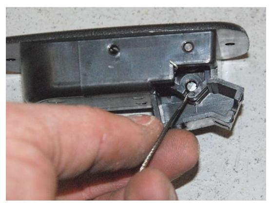
At the handle end of the cable push the barrel end of the cable into the handle so that the wire can go into the slot and swing forward.
