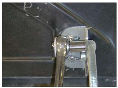
Push the hinge arm up to the trunk and tighten the hinge arm carriage bolts
