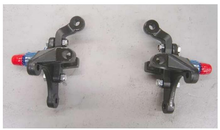
Assemble the spindles (passenger side is on the left; driver side is on the right).
