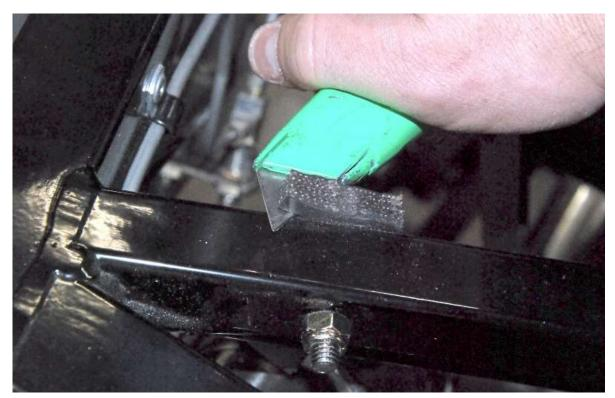
Cut any rubber that sticks up past the top of the frame tubes.
