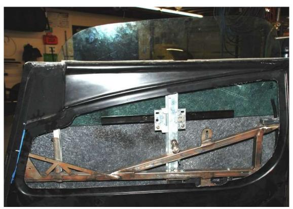
Slide the glass down into the door and into the glass holder. The taller end of the window goes towards the back of the car. Also note that the logo and information on the passenger side window is backwards when viewed from outside the car. This is normal practice even on OEM Vehicles that use the same glass for each side of the car.
