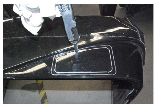
Cut the inner line for the access panels.
