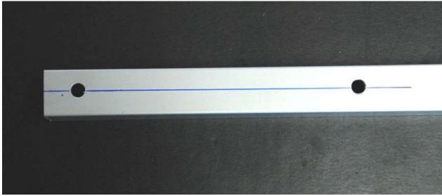
Drill <sup>13</sup>/<sub>64</sub>" holes at the ½" and 4.50" points marked.
