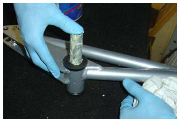
Insert the greased sleeve into the bushings in the upper control arm
