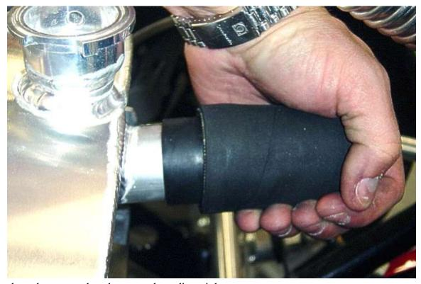
Push the large hose over the adapter on the radiator inlet.
