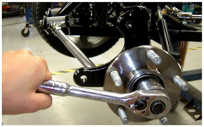
Install the hub nut onto the spindle. Torque this nut to 235ft-lbs.
