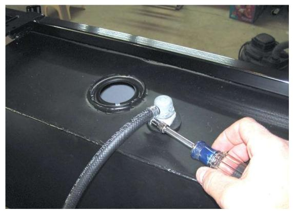
Attach a 25" section of 5/16" fuel line and fuel line clamp onto the vent and rotate the vent so that it points forward.
