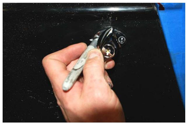
Place door handle in the outer door skin hole and mark the mounting holes.
