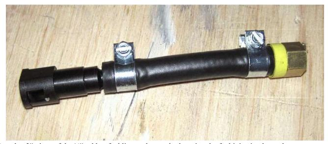
Attach a 3" piece of the 1/4" rubber fuel line to the two barbs using the fuel injection hose clamps.
