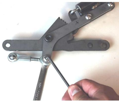
Slide the male rod end between the ratchet to handle mount plates and attach it using the ¼" flange head bolt and locknut.
