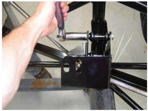
Install the engine mount mounts onto the frame with the  $\frac{1}{2}$ "-20 hardware (FFR# 33454 & 25619). It is helpful to only bolt the top of the mount in for now and pivot it down and away while installing the engine to provide more clearance.
