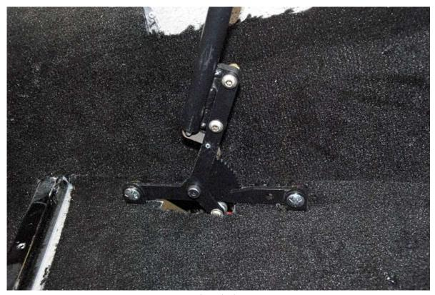
Attach the handle to the frame using the 5/16" carriage bolts.
