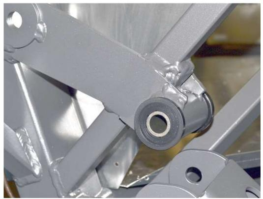
Use a plastic mallet to install the polyurethane bushings marked 2048 and the longer  $(3^{1}/_{16}")$  sleeves where the front of the center section will mount.
