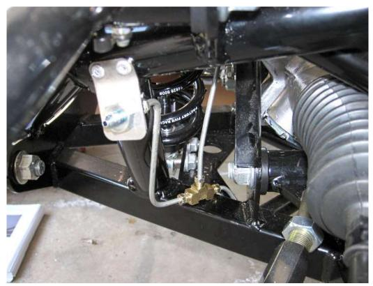
At the end of the 20" brake line section, install the 3-female T-junction.
