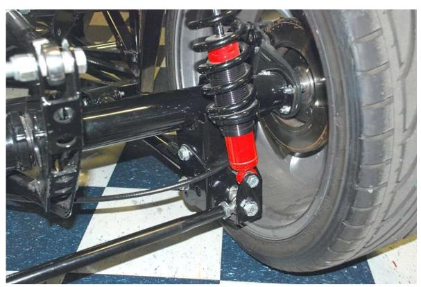
Route the brake cables over the Panhard mount if using a 3-link
