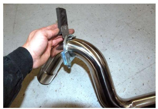
Slip one of the hangers under the clamp and hand tighten the clamp so that it can be easily adjusted later
