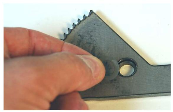
Push the other bushing into the other side of the fixed gear.
