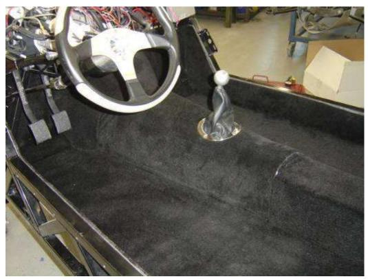
Once the carpet is installed install the shifter handle, boot and trim ring. We suggest you bend and form the trim ring to the contour of the tunnel.
