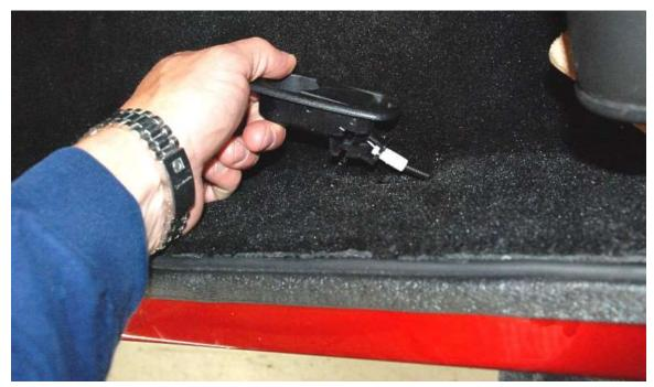
Pull the trunk release cable through the hole and attach it to the handle.
