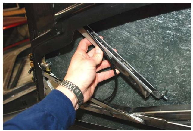
Insert the U-channel assembly into the front of the door and put the  $\frac{5}{16}$ " carriage bolt from the top through the window guide bracket and through the door frame mount.
