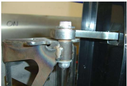
Attach the hinge arms to the hinge arm standoff but leave the nut hand tight.
