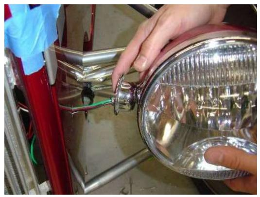
Pass the wires though the radiator mount into the engine bay.
