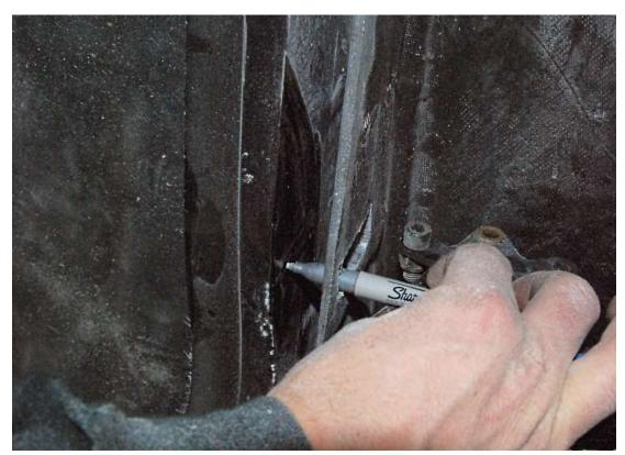
Use the marker to mark the door hinge body cut-out locations on the door.
