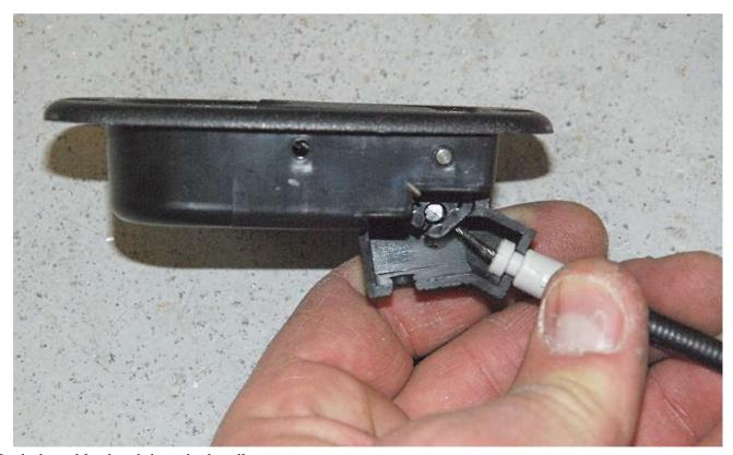
Push the cable sheath into the handle.
