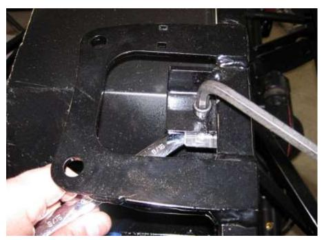
Install the tank using the  $\frac{3}{8}$ " fasteners. Place the washers on the tank side of each of these mounting locations.
