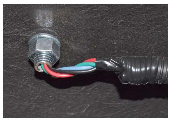
On the underside of the fender, mark the stud two or three threads past the end of the nut.
