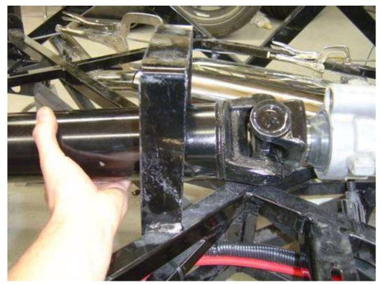
Install the drive shaft next. Begin by inserting the front of the driveshaft onto the output shaft of the transmission.
