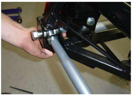
The Panhard bar is then installed on the Panhard frame mount (driver's side) and mounted with a 0.375" spacer (FFR# 33239) on either side.
