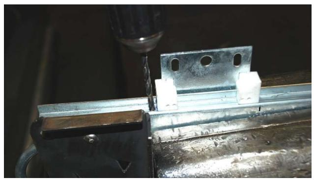
Remove the locknut and open the hole up to  $^{13}/_{64}$ ".
