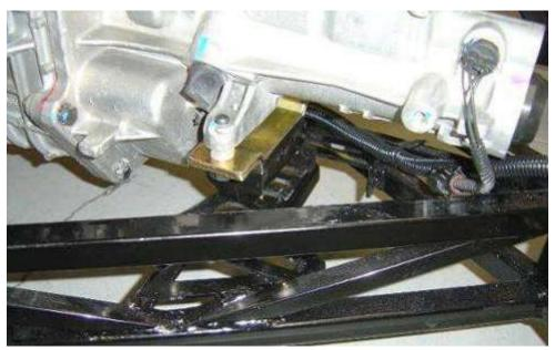
The transmission mount plate is fully adjustable and can be positioned on the chassis to provide more adjustment to the front or the rear depending on the transmission choice. Lift on the rear of the transmission and slide this bracket into place. It is fastened to the chassis with the ½" carriage bolt, washer and nut.
