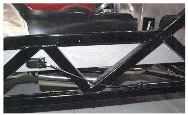
Run the cable forward along the 1.5" square tube to where the handle will attach
