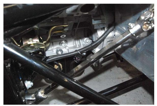
Loosely run the front harness to the front of the car. The best place to bring this harness into the engine bay is to the left of center directly under the firewall piece of aluminum passing through the front of the transmission tunnel.
