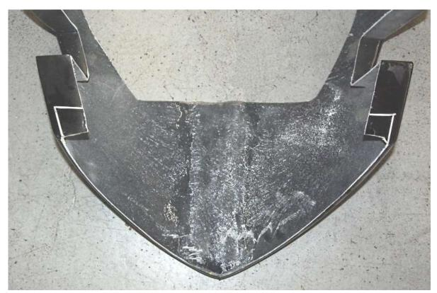
If not cut, mark the top of the nose cone 1.75" back so that the grill will fit in the nose cone.
