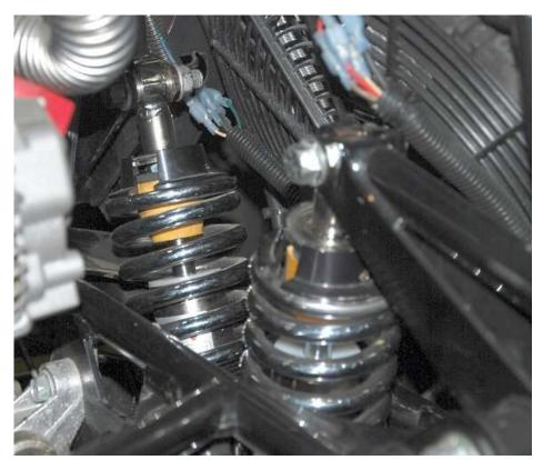
Install the shocks on the chassis with the body down. Use the 0.32" spacers on either side of lower the spherical joint.
