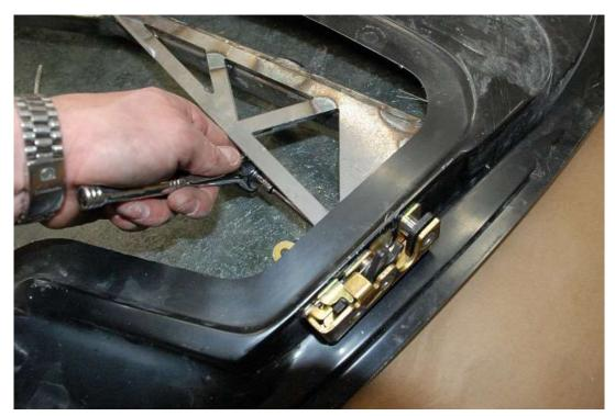
Attach the door latch to the door frame through the holes drilled earlier using the  $\frac{1}{4}$ " flange head bolts from the inside of the door out and a  $\frac{3}{8}$ " socket and Ratchet.
