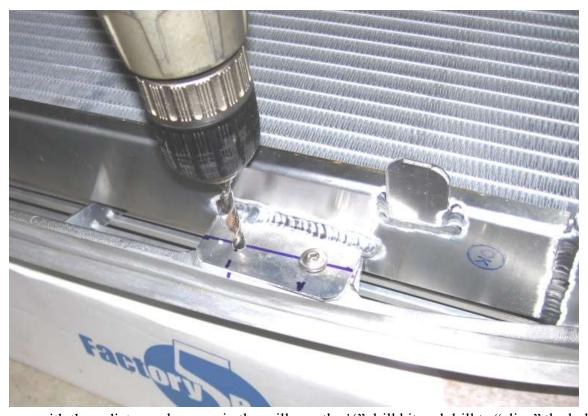
If necessary, with the radiator and screws in the grill, use the 1/4" drill bit and drill to "align" the holes.
