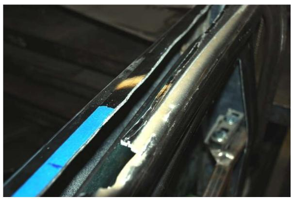
Lower the window so that the top of the glass is just below the top of the door.
