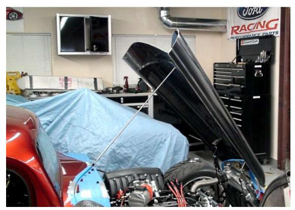
Mock up the Prop Rod to find the desired placement.
