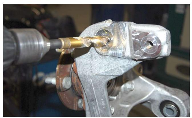
Use a 5/8" drill bit to drill out the tapered hole at the top of the spindle.
