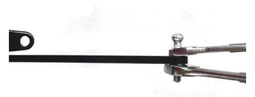
Attach the ball stud to the top hole of the accelerator pedal.
