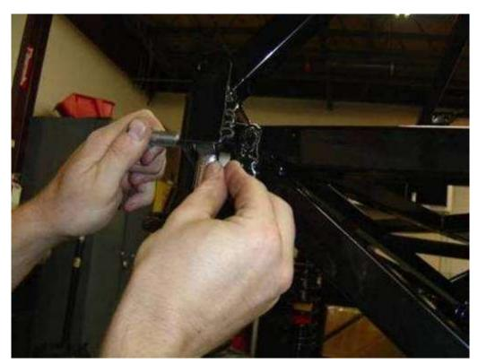
Install the shocks onto the frame with the body of the shock down (FFR 12217 & 12218 & 33241). Make sure to use one of the 0.32" spacers on either side of the spherical joint. Make sure to insert the bolt from the front placing the nut to the rear of the car (allows you to remove the shocks when the car is complete)
