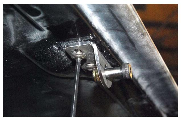
Install the trunk latch striker mount with 3/4" flange head screws onto the trunk centered on the bolts.
