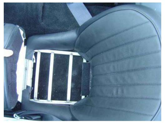
Reattach the seat in the holes drilled before using the fasteners provided.
