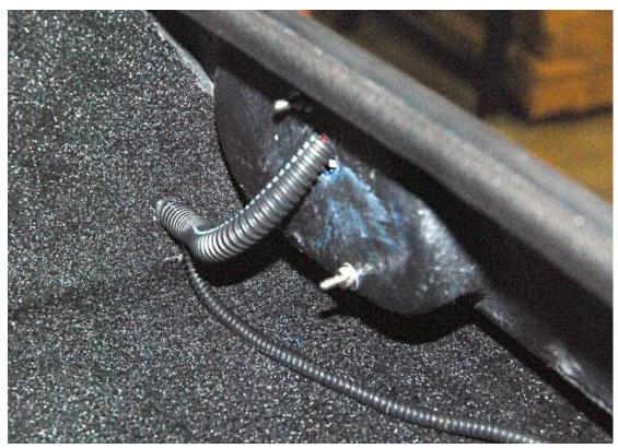
Put the wire loom on the wires in the trunk.
