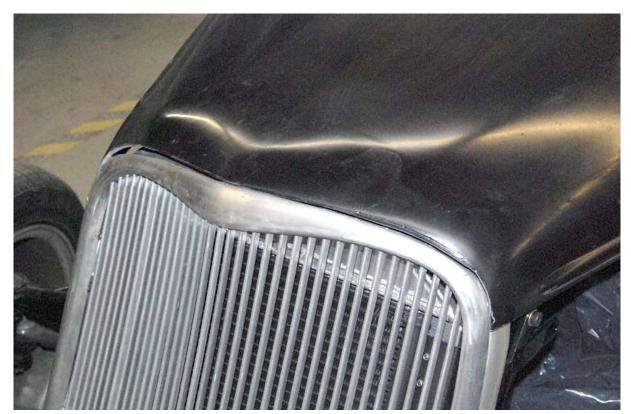
Set the hood in place for initial fitment so that the front is down in the grill recess. Trim the hood around the grill a little at a time if necessary so it just fits.
