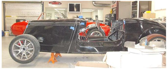
Mark and trim the bottom edge of the hood so that there is a  $\frac{1}{8}$ "- $\frac{3}{16}$ " gap between the hood and top of the side cover.
