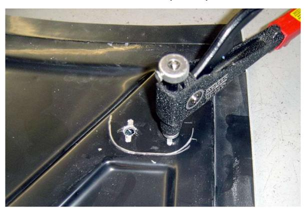
Install a 1/4"-20 rivnut in each of the holes drilled.
