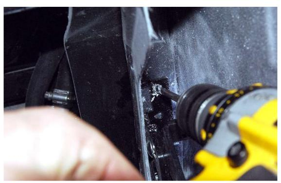
Use an 1/8" drill bit and drill through door through the top hole in the door latch mount.
