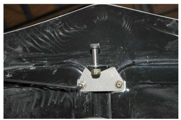
Mount the hood striker bracket to the hood loosely to allow for adjustment.
