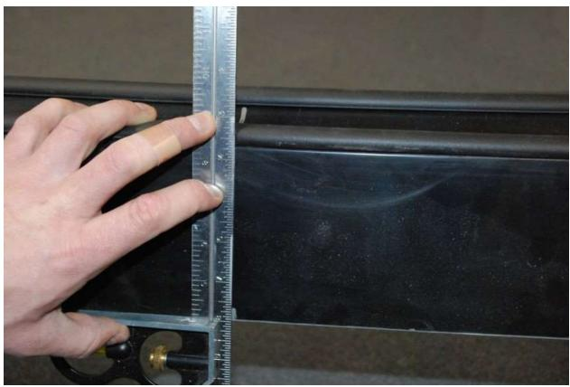
Use a square to mark the bottom of the Hard top from the window center mark made so that the middle rear of the top is found.
