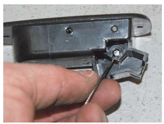
Attach the cable to the handle the same way as was done for the trunk handle. At the handle end of the cable push the barrel end of the cable into the handle so that the wire can go into the slot and swing forward.
