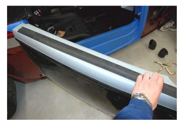
Carefully push the felted rubber seals onto the top of the door. Check the window up and down with the door open and closed. The idea is to have the felted seals to just touch the window and not put a lot of
