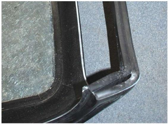
Attach the half moon weather-stripping to the underside of the front of the hardtop along both the inside and front edges.
