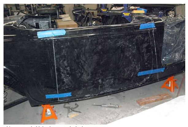
Use masking tape to hold the door onto the body.
