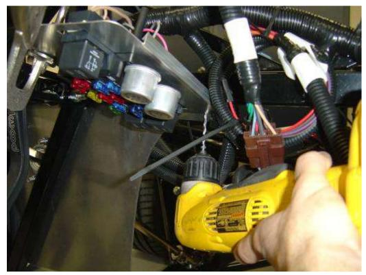
Clamp the fuse block mount plate into place to the right of the pedal box mounting location. Drill into the 1.5" square tube (firewall mounting surface tube) and the ¾" tube (lower one) which triangulates the pedal box mounting location. Install the panel with rivets.
