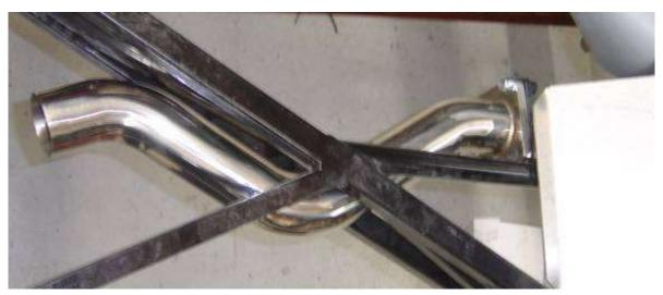
Pass the front exhaust assembly through the frame from the front so that the flange is at the front and will match up with the shorty pipe
