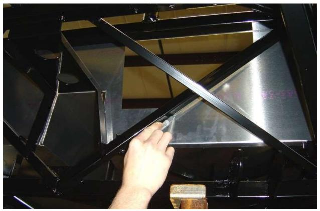
Before removing the aluminum from the chassis, mark each panel and take pictures of how the panels fit together (i.e. which is on top). To get straight and evenly spaced rivets, trace the underside of the aluminum panel around the frame members with a black permanent marker.
