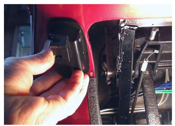
Mark the hole for the hood release pull under the dash on inner edge of door jam by drawing around the flange.
