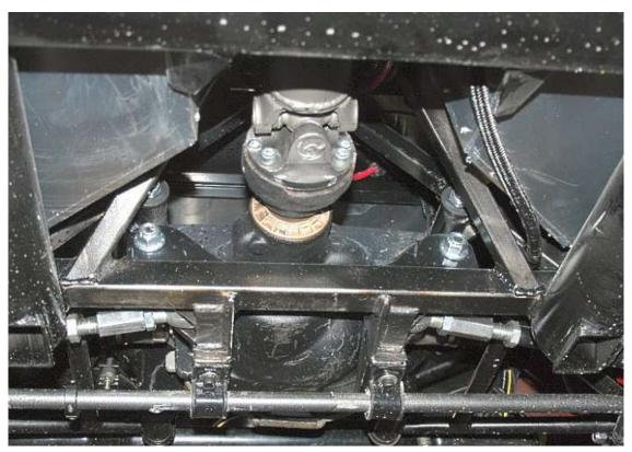
Insert the driveshaft into the transmission, bolt the rear flange to the driveshaft adapter and torque the bolts to 95Nm (70 ft-lb).
