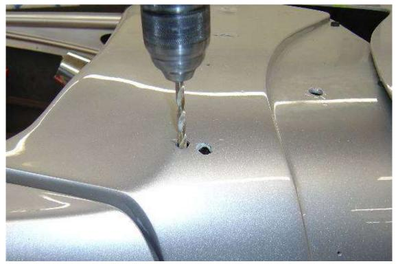
Drill the 1/4" holes in the body which you just marked which are the mounting points for the windshield.
