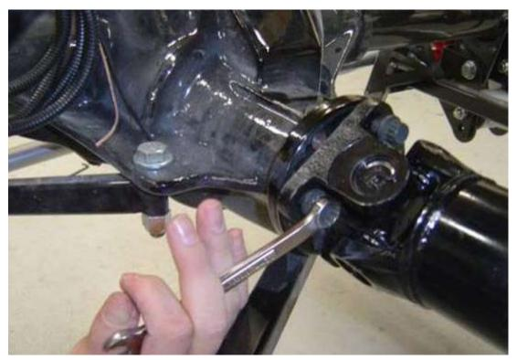
Fit the driveshaft snug against the yoke and install the bolts and tighten. You can put the transmission in gear to stop the driveshaft from turning while you tighten. Torque the bolts to 95Nm (70 ft-lb).
