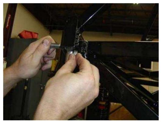
Hot Rod - Attach the rod end of the shock to the upper shock mount using the two equal length 0.32" kit spacers. Make sure to insert the bolt from the front placing the nut to the rear of the car (allows you to remove the shocks when the car is complete).
