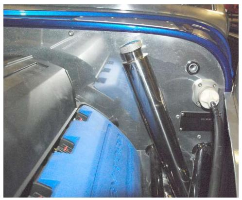
The overflow tank can either get mounted to the radiator as shown in the diagram before the radiator installation or directly to the firewall.
