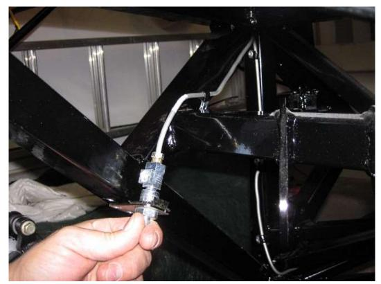
Route the brake line on the inside of the 1.5" tubes to behind the rear axle upper control arm mount tube.
