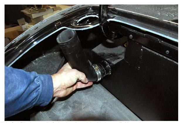
Install the fuel fill tube onto the fuel tank and attach it with the supplied hose clamp.
