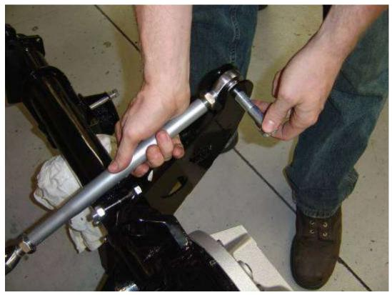
Install the upper link onto the axle clamp bracket using the 5/8" x 3.00" bolt and locknut
