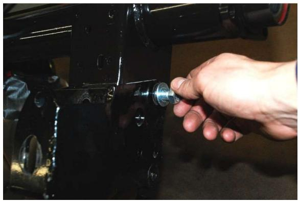
Position the Traction Lok brackets on the rear end with the bolts provided (the two short bolts go on the sides).
