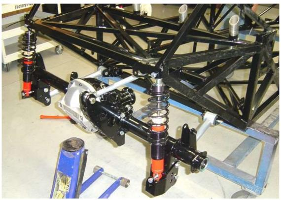
Install the shocks (body down) to the rear axle assembly (FFR# 12332 & 10834). The longer spacer (FFR# 33238) is placed at the front of the shock and the smaller 0.125" shim (FFR# 13210) is placed at the rear.
