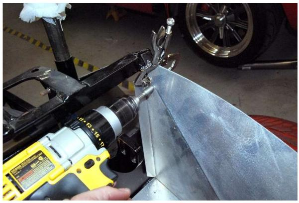
Clamp the trunk wall aluminum to the frame then screw it to the frame using one of the holes for rivets.
