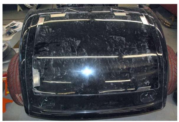
Tape the trunk in place with the shims so that it can not move.
