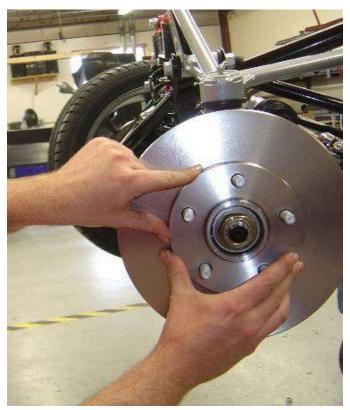
Clean the rotor with brake cleaner and push it onto the hub.
