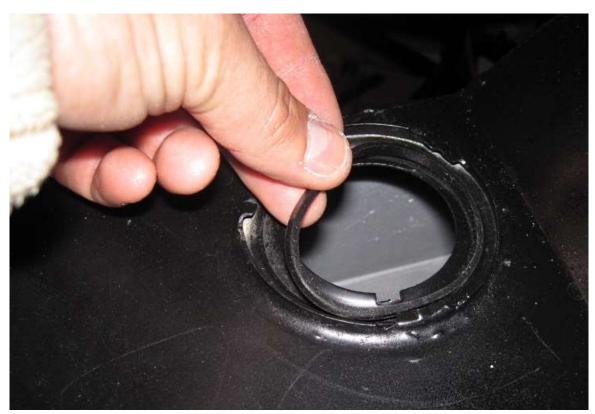
Place the rubber ring in the groove in where the sender will go, on the lower part near the trunk hinge arm.
