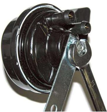
Attach one horn to the included bracket using one of the 14mm lock washers and nuts included. Note the orientation of the wire connectors when tightening the bracket so that it will be correct when installed. The flat horn outlet is pointed right.
