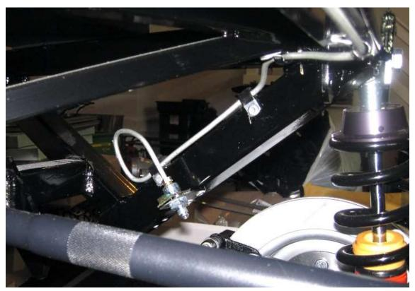
Run the brake line down the frame on the passenger side to a location similar to the driver side again leaving room around the 3-link mount bolts if running it.
