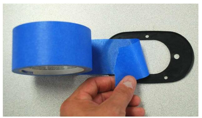
Put a piece of masking tape over the large hole in the center of the mounting gasket.
