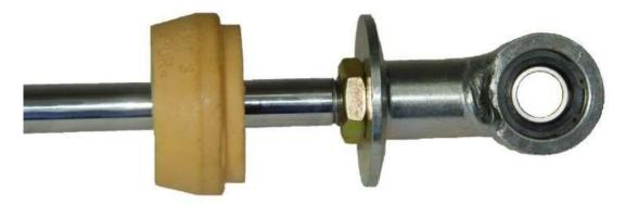
Slide the rubber bumper about two inches down on the shaft.
