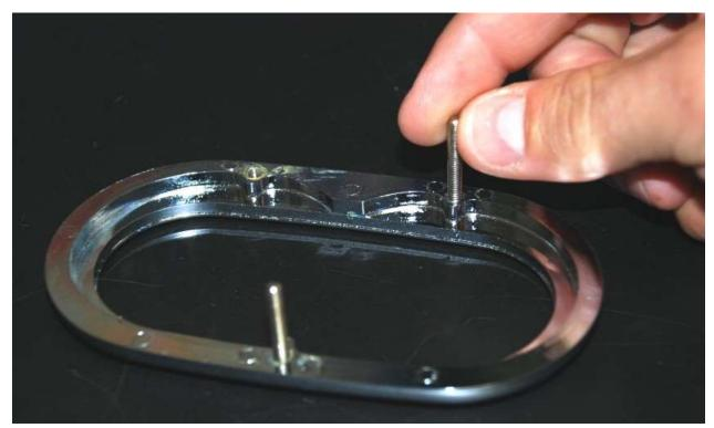
Thread the studs into the bezels.
