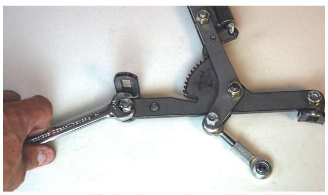
Attach the mount brackets to the fixed gear using a ½" wrench. Leave the locknut slightly loose so positioning can be done on the frame later.
