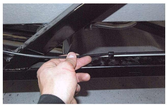
Attach the release cable to the frame using the small insulated line clips and 3/16" rivets.
