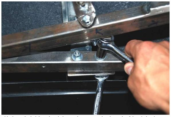
From inside the car look tighten the window track mounts so that the angle of the window is correct.
