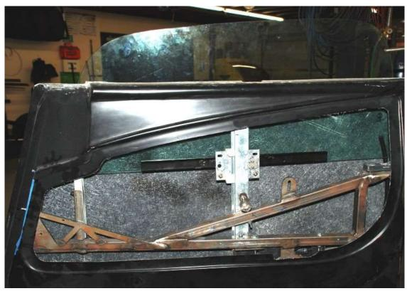
Reinstall the window track in the door with the bolts slightly loose
