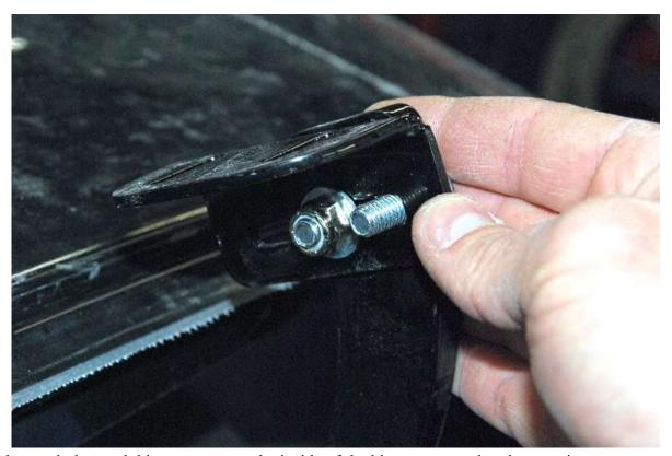
Loosely attach the trunk hinge mounts to the inside of the hinge arms so that they can just move.
