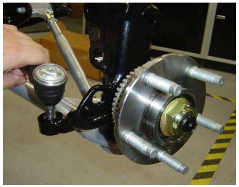
Insert the Tie Rod into the spindle with the stud pointing down. For now, align the front end by eye. Fasten the outer tie rods onto the spindle with lock nut.
