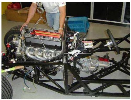
Once the engine is in place, pivot the engine mount brackets into place and bolt the engine brackets onto the chassis. Install the nut on the Energy Suspension mounts attaching the engine mounts to the modular mounts.
