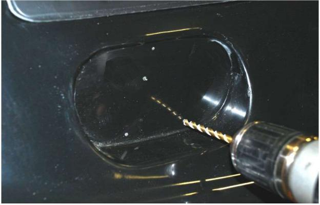
Drill the three mounting holes for the bezel stude using a  $^{3}/_{16}$ " drill bit.
