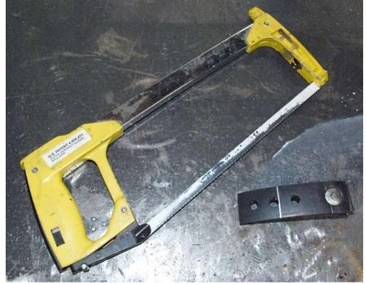
Cut the rubber hanger just below the second hole otherwise it will hit the trunk floor using either a razor or hack saw.
