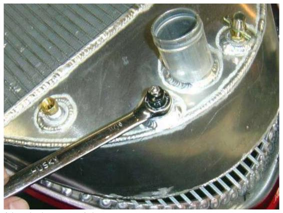
Carefully tighten the thermostat switch.
