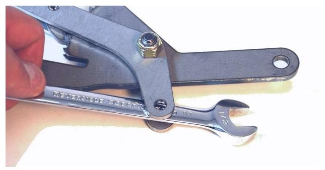
Use a wrench to spread the ears of the ratchet to handle mounts so that the rod end can just slide between them.
