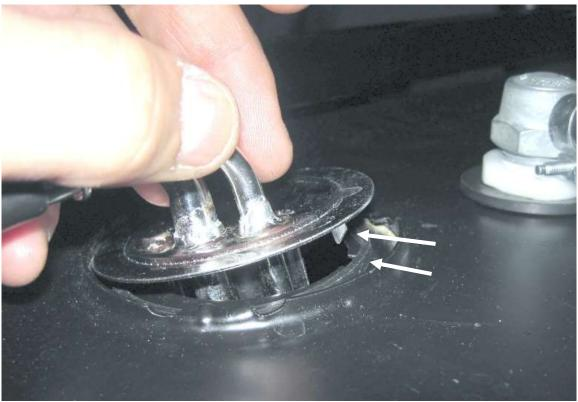
Insert the pick-up into the tank as shown, rotating it as it bends so that it will end up in the basket in the tank and the small tabs on the underside of the top plate go in the slots in the mounting area
