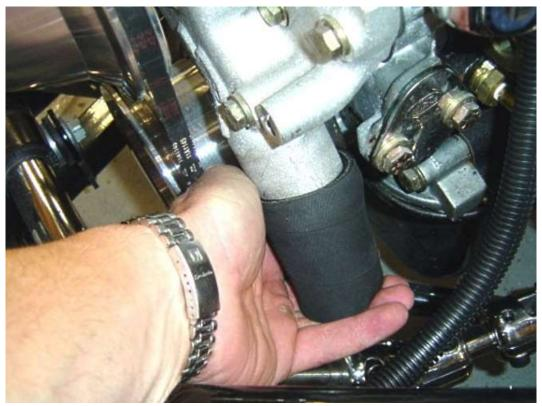
Open one of the radiator hose adapter kits and remove the adapters inside the larger hose and the hose clamps from the outside of the hose. Cut 1/4" off the end of the larger hose. Push the large hose onto the water pump inlet.
