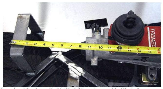
Measure forward from the rear side of the driveshaft loop to the center of the shifter handle.
