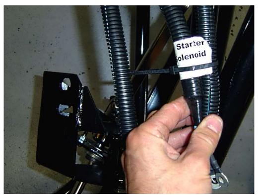
Locate the starter solenoid wires.
