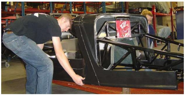
Two people can remove the body from the chassis. One person on either side located where the door openings are (if you have a third person, position them at the rear of the car. Removing the body should be done very carefully. Once the body is removed, it is fine to store it directly on the ground.
