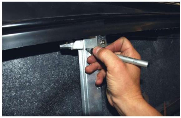
Close the door, and raise the window up to where you would like it to stop. Be careful doing this. Once this position is found, open the door and mark the window track where the bottom of the plastic guide is.
