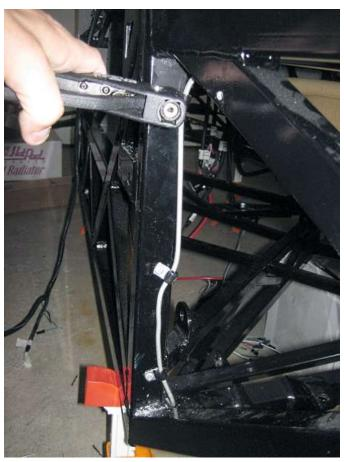
At the end of the passenger compartment, route the brake line up the back side of the vertical 1.5" tube. Stay to the inside of the tube as the body will be very close to the outside of this tube.
