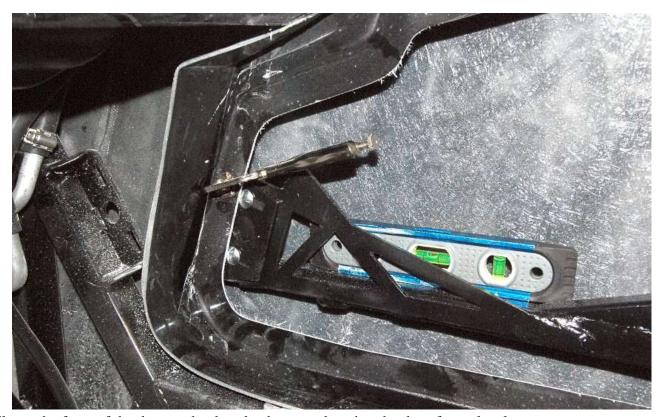
Clamp the front of the door to the door latch mount keeping the door frame level.
