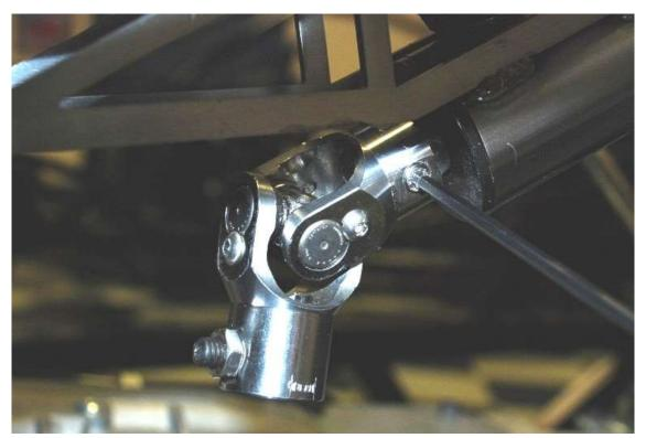
Attach the  $\frac{3}{4}$ " DD to  $\frac{3}{4}$ " DD joint on to the steering column output shaft using a  $\frac{5}{32}$ " Hex key and  $\frac{1}{2}$ " wrench. The smaller end goes on the steering column.
