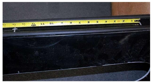
Measure the width of the rear window on the Hard top and mark the center of the window (around 15.50").
