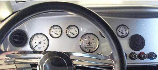
Other gauge layouts have been used by customers. Keep in mind though that the master cylinders and pedal box tubes are very close to the dash.
