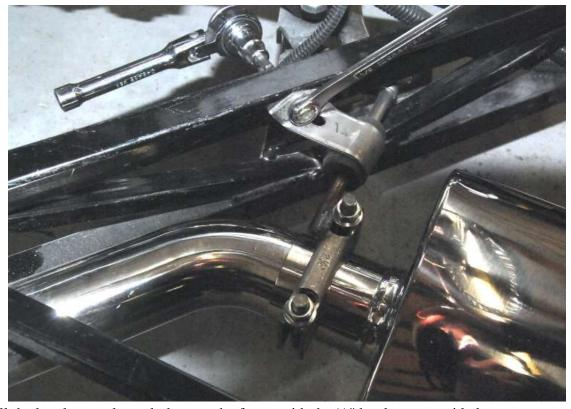
Re-install the brackets and attach them to the frame with the 3/8" hardware provided.
