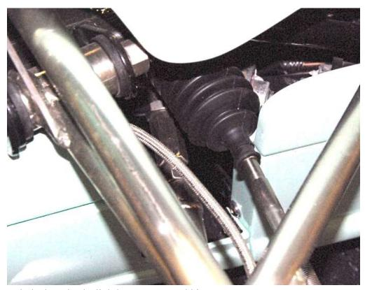
If necessary, push the boot back slightly to prevent rubbing.
