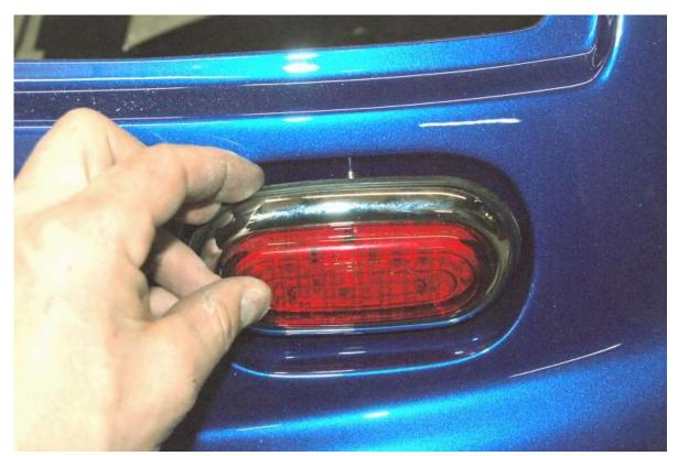
Insert the light wires through the body hole and insert the studs through the mounting holes.
