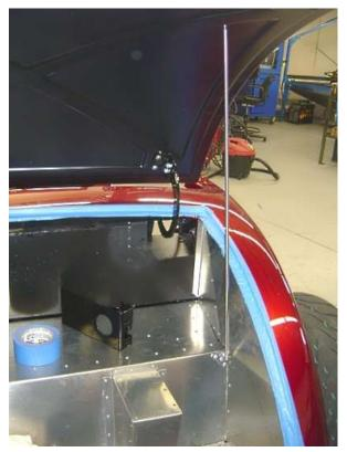
The trunk prop rod is mounted on the right side of the car on the vertical wall of the trunk.
