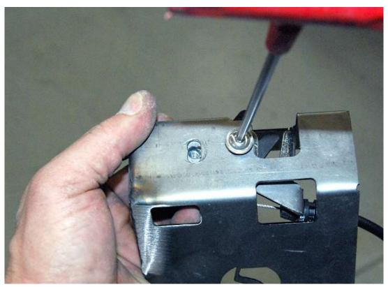
Attach the trunk latch and latch spacer to the trunk latch bracket as shown in the drawing at the beginning of this assembly. Leave it loose for now so it can be adjusted.
