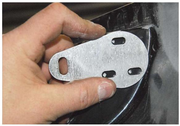
With hood upside down and level, mark the holes for the firewall pin brackets. Place the bracket so that pin slot (arrow) is vertical and there is enough clearance to slide the bracket outboard when maxing out the horizontal slots.
