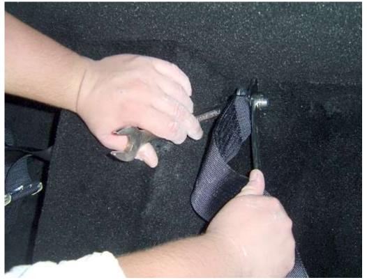
Install lap portion of the harnesses to the mounts on the chassis with the supplied hardware. It is a good idea to mount the belt on the outside of the tabs to provide the most amount of space for the seat.
