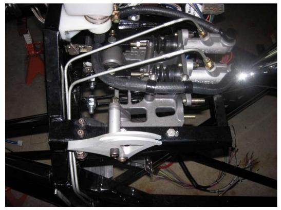
Run the brake lines starting at the master cylinders. The <sup>3</sup>/<sub>4</sub>" master cylinder is used for front and the <sup>5</sup>/<sub>8</sub>" master cylinder is used for the rear brakes. Connect a 60" section of brake line to each of the master cylinders directed towards the firewall.
