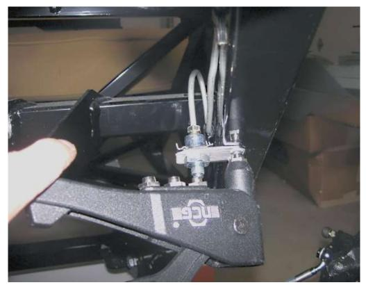
Reposition and rivet the brake line mount to the frame.
