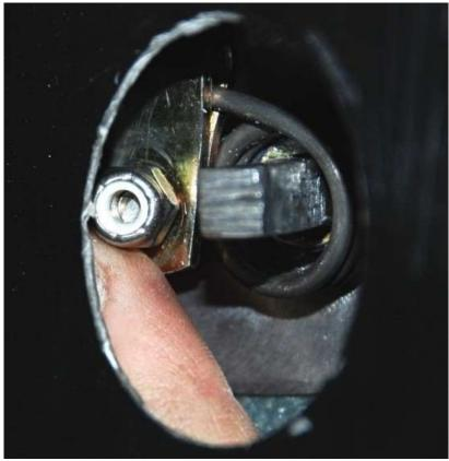
Attach the pressed clevis to the front handle screw using another 10-32 locknut and <sup>3</sup>/<sub>8</sub>" deep socket.
