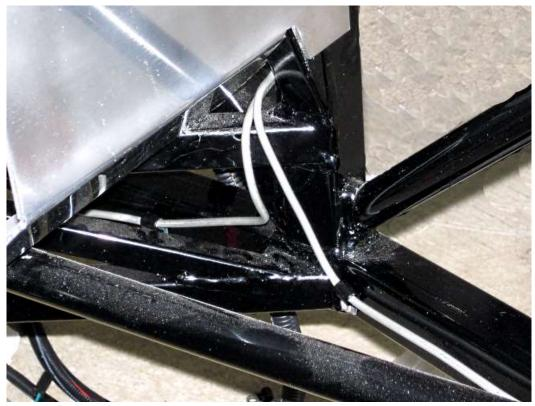
At the bottom of the footbox, split the lines and angle one towards the front of the car and one towards the rear.
