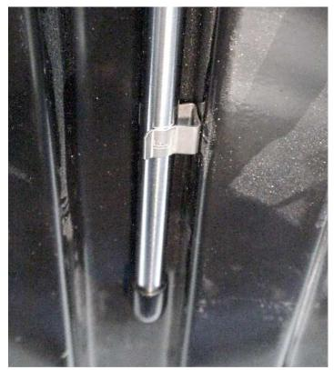
Snap the Prop Rod clip to the rod and mark the hood for desired placement.
