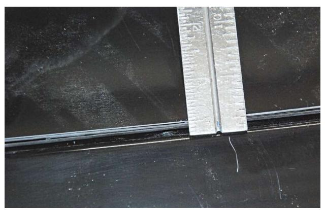
Close the trunk and measure the distance from the body lip to the trunk edge.
