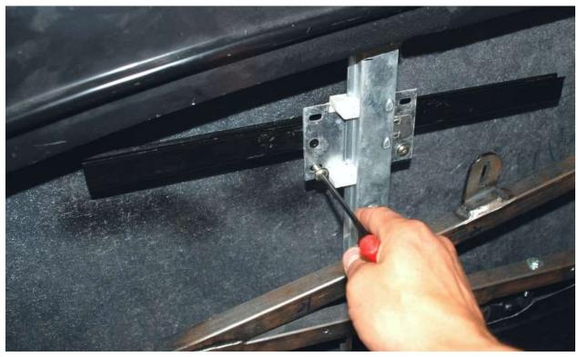
Attach the window glass holder to the lower holes on the track bracket. Center the bolts in the holes.
