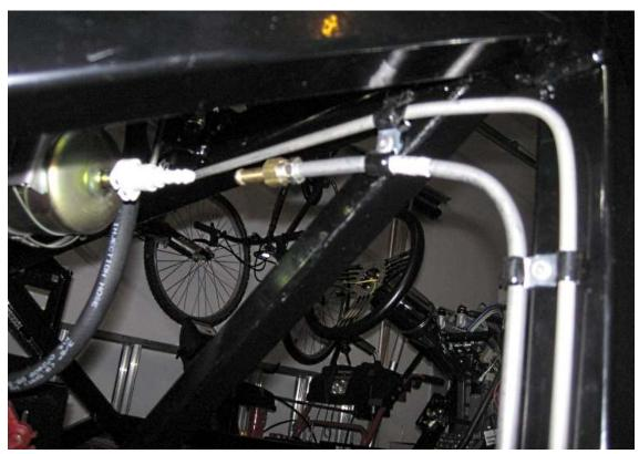
Position the end of the  $\frac{5}{16}$ " fuel line 2" from the fuel filter, far enough away that you can disconnect the fitting from the filter. Note the location of the vertical 1.50" square tube and bend the line so it will go down the back of the tube.
