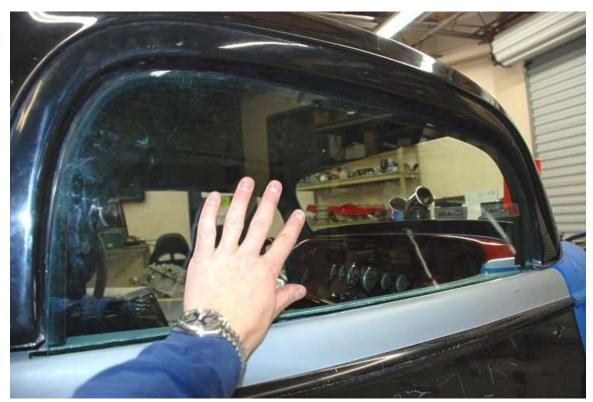
Slowly close the door checking the clearance of the glass at the front and back near the top then raise the window up and have a friend push the glass against the weatherstrip.
