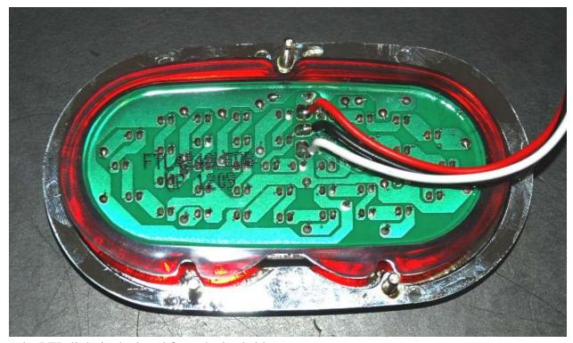
Place the LED light in the bezel from the backside.
