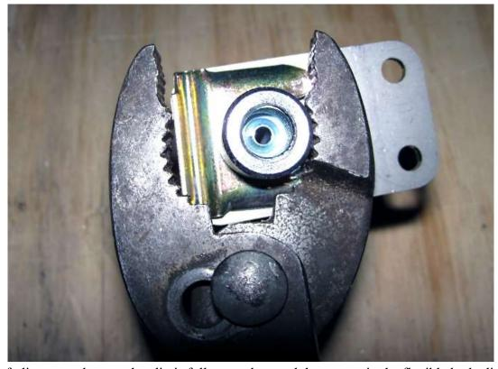
Use a set of pliers to make sure the clip is fully seated around the groove in the flexible brake line adapter.
