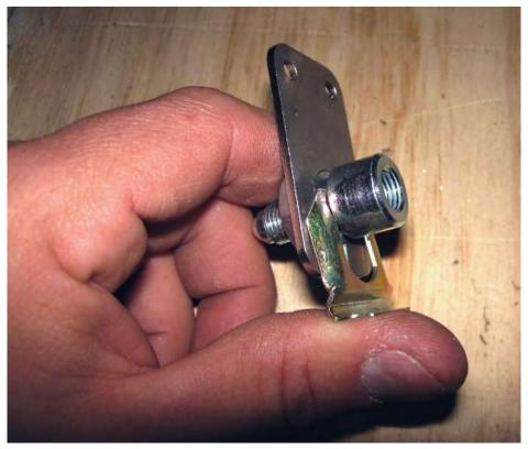
Attach the flexible brake line adapter to the frame mount using a brake line clip.
