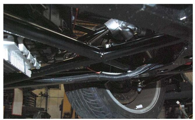
Run the harness forward to the engine mount then run it along the inside of the 1.50" square tube next to the brake line.
