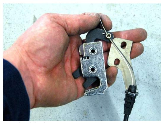
Insert the wire end through the wire stop.
