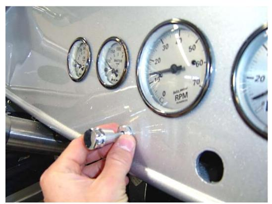
Install the headlight switch in the dash from the backside of the dash, thread the mounting nut into the housing itself to secure it in place. Place the knob over the switch shaft and then tighten the setscrew locking it in place.
