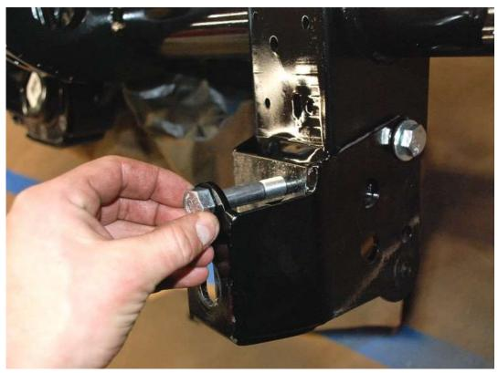
Insert the long bolt through the rear of the bracket and axle
