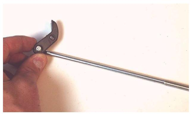
Put the ratchet tooth on the long anchor bolt as shown in the picture.
