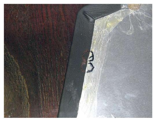
Pull the lever so that it is at the other extreme of its travel and mark the back of the panel again.
