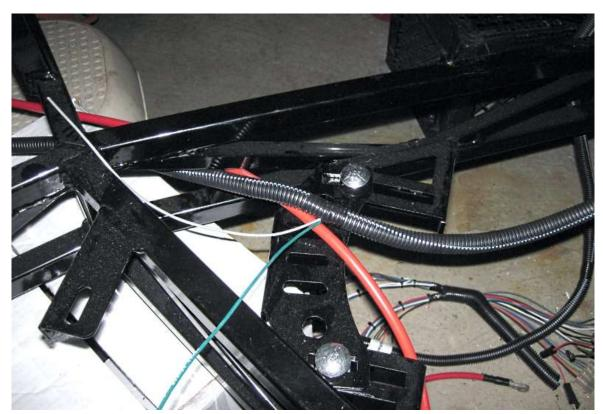
Starting at the firewall, route the cable and harness to the rear of the car by running it over the transmission mount and under the top 1" square tube holding it in place loosely with zip ties temporarily.
