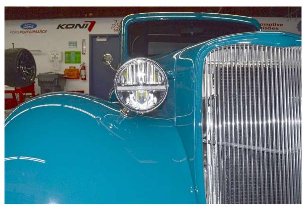
Position the headlight bucket left to right on the front fender so that the bucket is about 2.75" away from the cowl.
