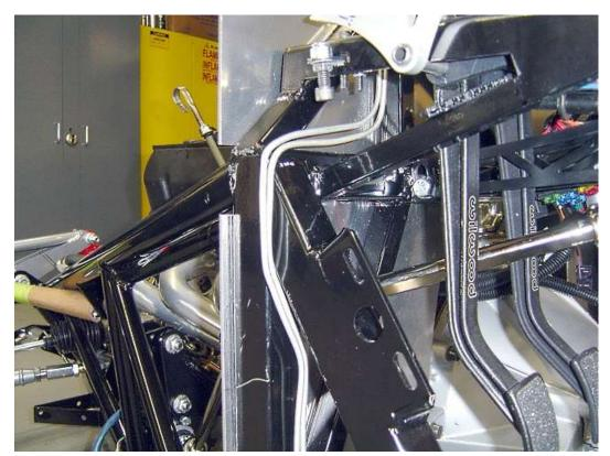
Route the brake line towards the outside of the car along the outside of the 1.5" frame rail.
