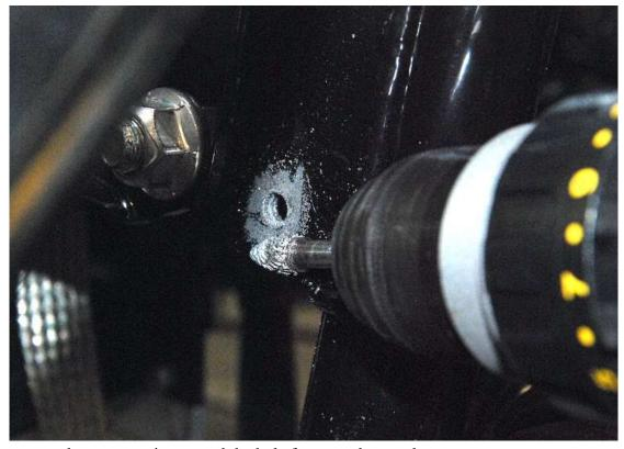
Remove any powdercoat or paint around the hole for a good ground.
