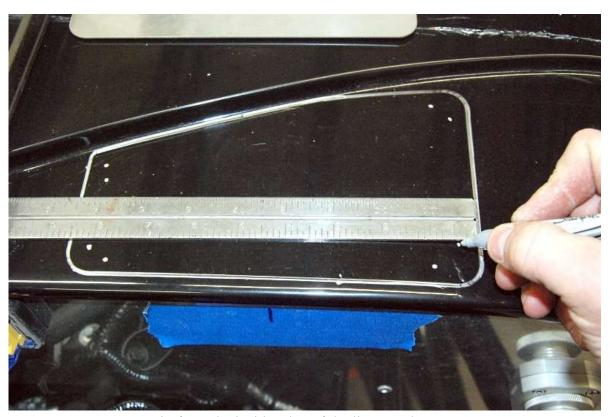
Use a ruler to make marks 3/8" in from the inside edge of the lines made.
