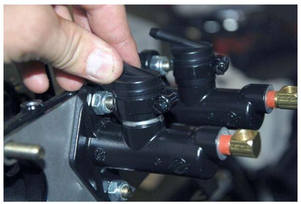
Put the plastic angled inlet adapter with hose clamp on the master cylinders. Use a 6mm socket and ratchet to tighten the hose clamp.
