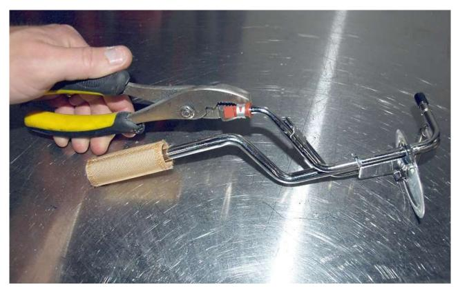
Remove and discard the rubber piece on the end of the return line, this can affect the fuel pressure at the engine.
