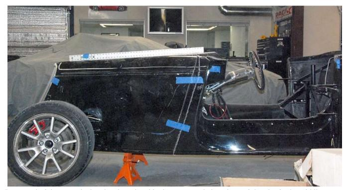
Put a yard stick across the hood and cowl and look at any gap below the straight edge in the middle. Adjust the angle of the grill and height of the grill so that there is no gap between the straight edge and the hood. The half moon trim accent on the hood should be aligned with the trim on the body and is either level or is slightly lower at the front of the hood.
