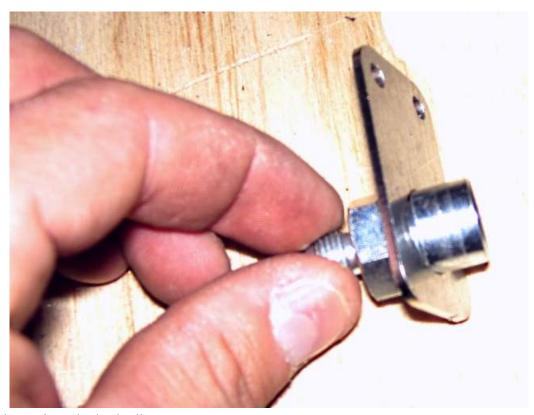
Insert the adapter into the brake line mount.
