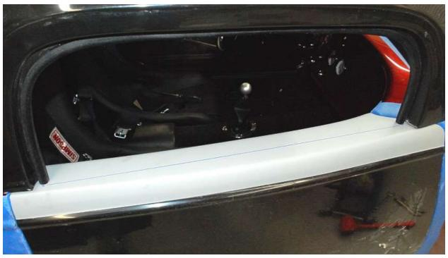
Using a ruler, straight edge, or the bottom of the side window, draw a line connecting the two marks made.
