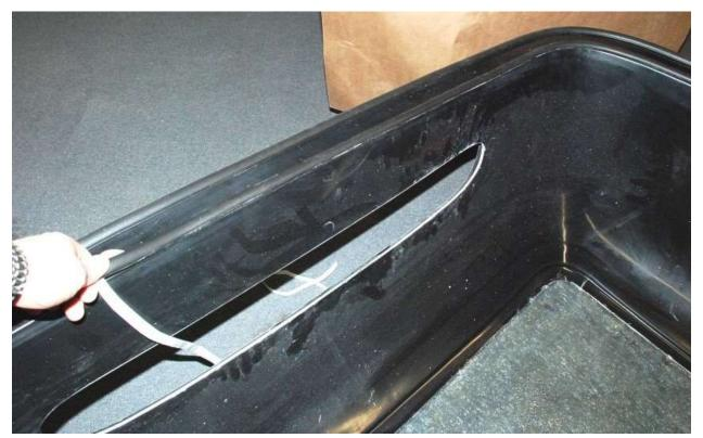
With the Hardtop sitting upside down on the roof, attach the half moon weather-stripping to the underside of the back of the hardtop along both the inside and rear edges.
