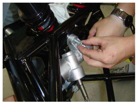
On the left side of the rack, use the M10 fasteners. Push the bolts through but do not fasten with the locknuts yet
