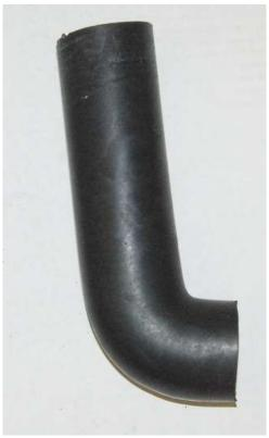
The fuel fill tube has to be modified to fit into the car perfectly. Trim material off both sides of the fill tube. The exact amount can vary, so trim a little at first and them test fit the piece.
