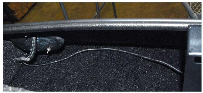
In the trunk, run the license plate wires over to the center of the trunk and push the wires through the grommet.
