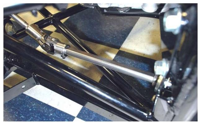
Insert the  $10^9/_{16}$ " lower steering shaft into the flange bearing and attach it to the steering rack joint. Again, make sure the end of the shaft is flush with the inner part of the joint.
