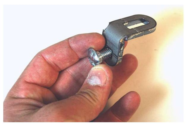
Insert a <sup>5</sup>/<sub>16</sub>" carriage bolt into one of the bent mount brackets so the square shoulder is in the square hole.
