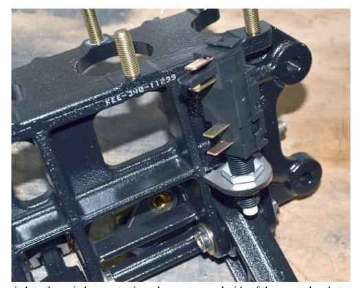
Connect the switch to the switch mount using a hex nut on each side of the mount bracket.
