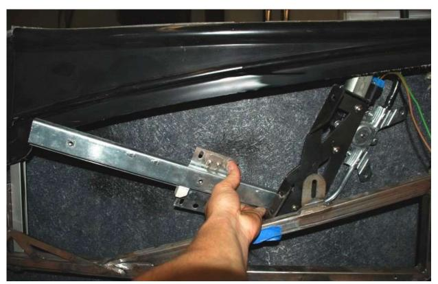
Insert the window track through the door opening with the motor towards the hinge end of the door.
