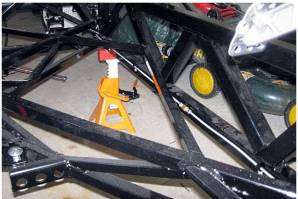
Route the initial 60" section of brake line along the outer 1.5" frame rail attaching it as you go with the 1/4" insulated line clips.
