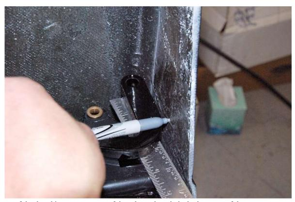
Place one of the door hinge arms on top of the ruler and mark the body on top of the arm.
