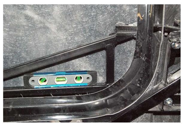
Place a bubble level on the door frame and make the door frame level.
