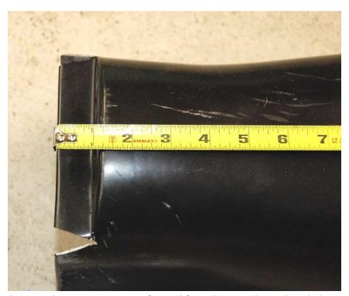
On the transmission tunnel cover top, measure forward from the rear edge and mark the cover where the center of the shifter is located.
