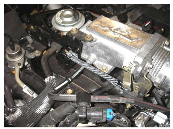
Accelerator cable mounted on '96 2 valve intake.
