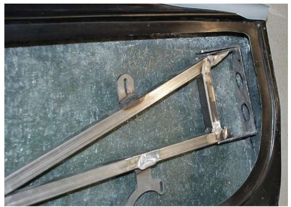
Place the door frame rear plate in the door so that the straight part sticks down and is towards the outside of the door.
