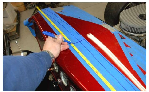
Use a tape measure at the front top corners of the door to locate and mark the middle of the front windshield area.
