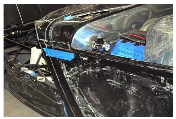
Tape the engine side covers to the body and the outside of the grill.
