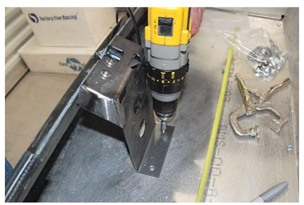
The bottom of the bracket is mounted to the trunk floor and attached with rivets from the bottom of the body.
