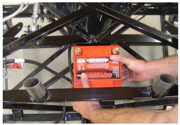
Install the battery on the platform centered behind the rear bulkhead of the cockpit. We recommend the Odyssey PC925 dry cell or similar
