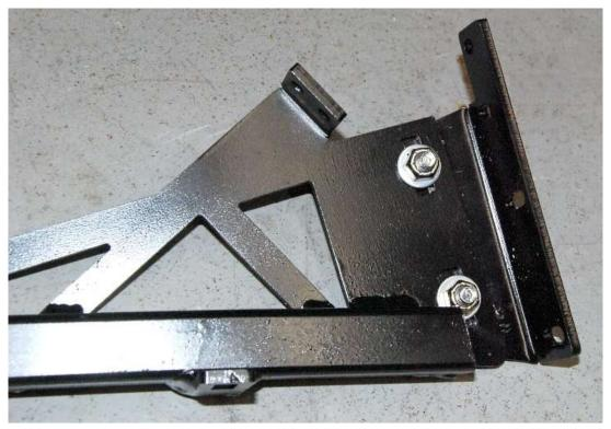
Center and attach the door latch mount to the door frame using the  $\frac{5}{16}$ " carriage bolts and locknuts. Leave the locknuts just loose enough so that the mount can slide if pushed.
