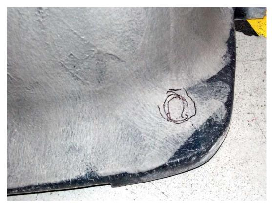
From inside the trunk, hold a marker inside the rollbar mount tube and bring it up to the rear cockpit panel and mark the underside of the panel for the rollbar hole.
