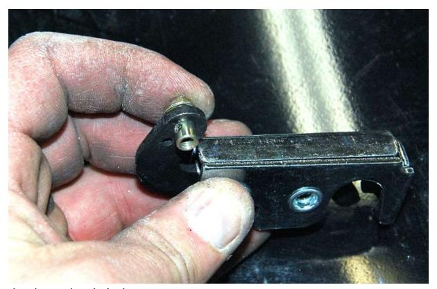
Insert the wire stop into the latch.
