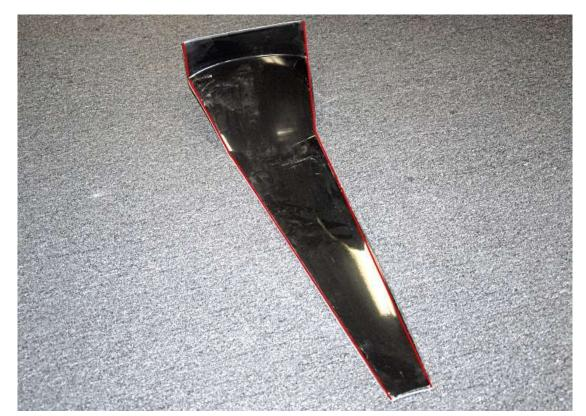
Cut the center of the transmission tunnel so that it sits down on the transmission tunnel flange.
