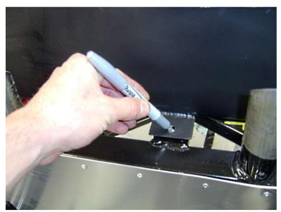
Using a marker mark the location on the frame where the (4) mounting locations.
