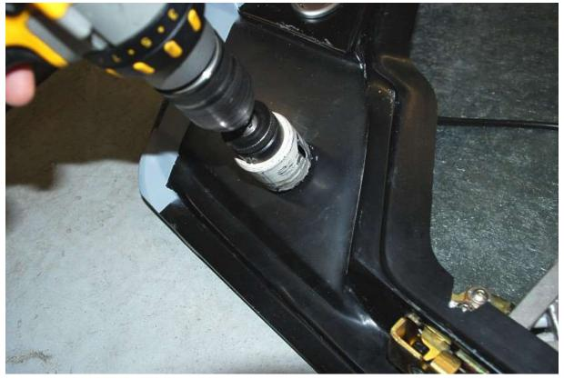
On the inner skin where the locating hole is, use a 1.75" hole saw through the inner skin only.
