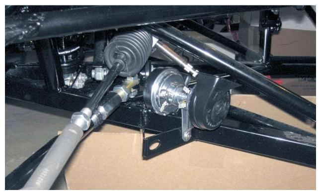
Attach the two horns to the backside of the side body mount behind the driver side front wheel using the supplied 1/4" bolt.
