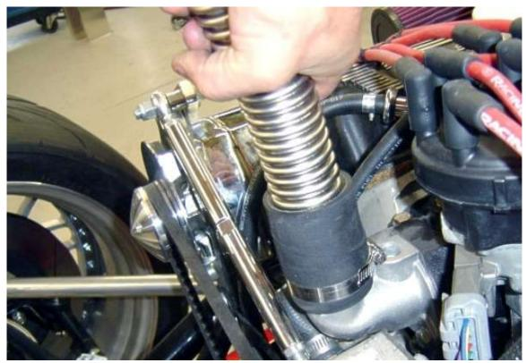
Attach the large hose to the engine outlet using one of the hose clamps and a 7mm socket and ratchet. It gives a clean look if you position the hose clamp so that the screw is accessible but is not seen.
