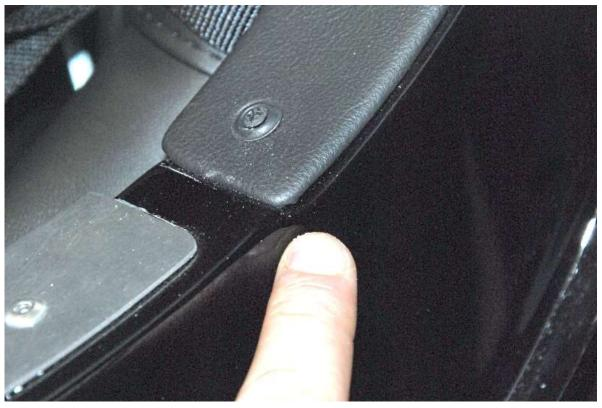
Install the rear cockpit panel in the frame and attach with black trim screws, rivets or preferred fastener.
