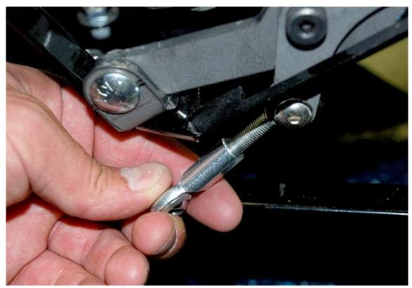
Release the brake and if necessary remove the  $\frac{1}{4}$ " clevis bolt and readjust the rod end so that the cable is tight.
