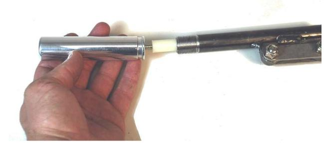
Spray a little WD-40 on the lower handle threads and screw the upper handle onto the lower handle.
