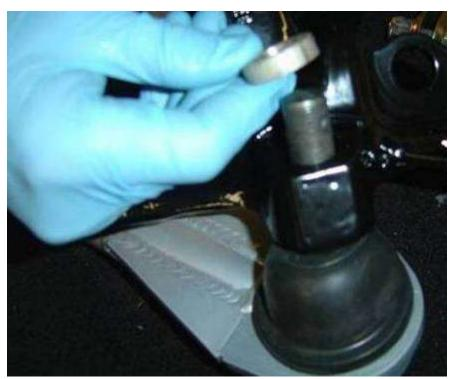
Install the spindle on the lower control arm ball joint stud. Then install the 0.25" spacer on top of the ball joint stud (FFR# 14406)
