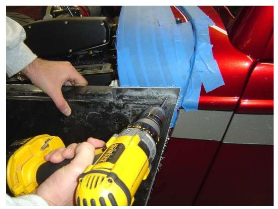
Drill a <sup>3</sup>/<sub>16</sub>" hole through the engine side panel mount flange and the body.
