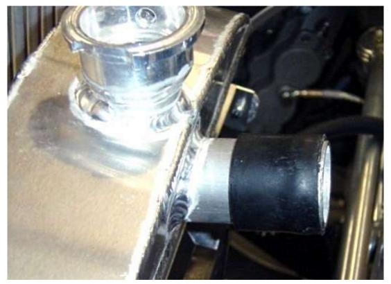
Push the thinner hose adapter onto the radiator inlet.
