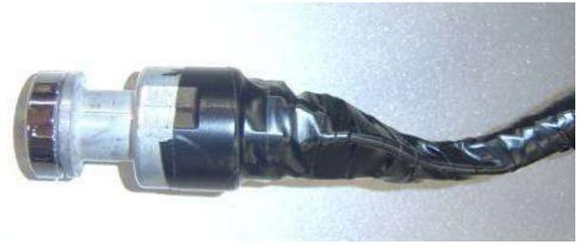
After you connect the wires to the correct terminals tape over the backside of the casing with electrical tape to prevent electrical shorts.
