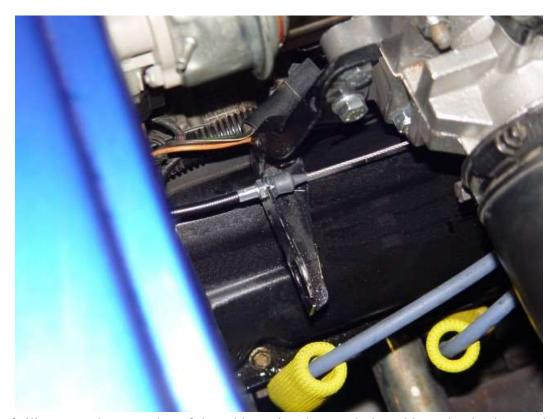
Put a dab of silicone on the rear edge of the rubber wipe then push the rubber wipe back onto the threads.
