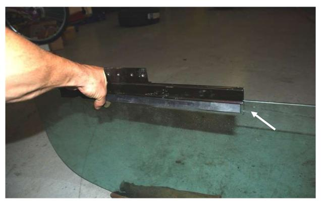
With the top of the glass resting on something soft such as a towel or a glove as shown, locate the rubber strip and window glass holder on the window using the glass marks made as a guide. Make sure that you have the glass holder the correct way around on the glass so it will mount correctly.
