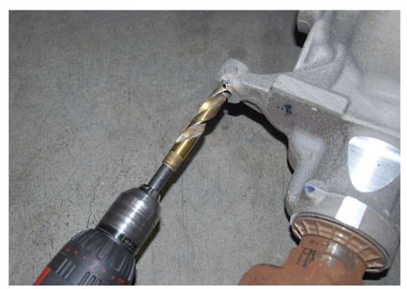
Use a  $\frac{5}{8}$ " drill bit to chase the front mount holes on the center section.
