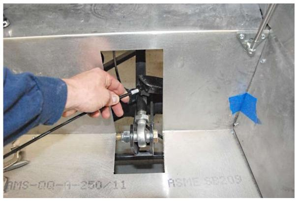
Pass the release handle and cable through the hole in the trunk floor.
