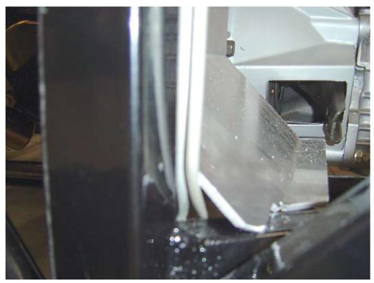
Route both of the brake lines through to the engine side of the firewall by passing it between the frame and the  $45^{\circ}$  angle section of the foot box front wall.
