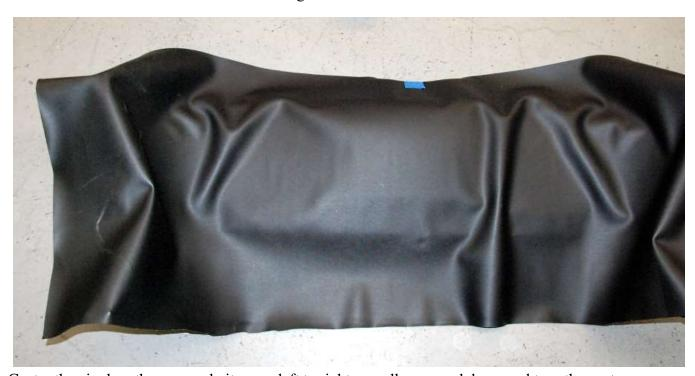
Center the vinyl on the rear cockpit cover left to right as well as up and down and tape the center.
