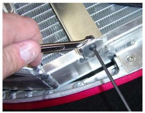
Attach the fan assembly to the radiator tabs using the screws and lock nuts provided. Pass the screw from the outside in for a clean look.
