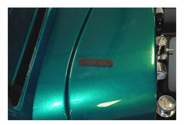
Mount a few rubber bumpers on cowl. Use the small and large bumpers included with the kit to set the height of the panel so that they are flush with the body. If necessary, cut the large bumpers to the correct height if the small ones are too small.
