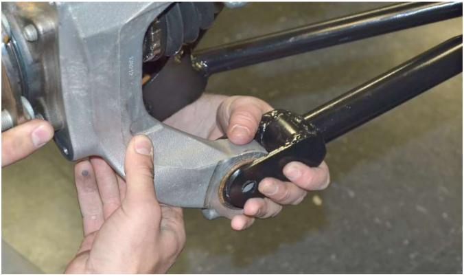
Attach the Toe link arm to the spindle using the M14 x 80mm bolt and locknut.
