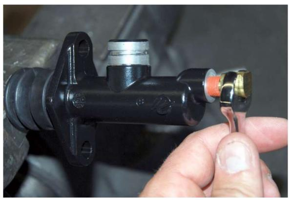
Screw the  $90^{\circ}$  brake line adapter into the end of the master cylinder making sure that the opening points up when tight.
