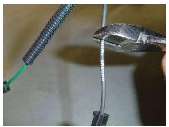
Cut 2" off the end of the chassis harness horn ground wire and strip the end of the chassis harness ground wire.
