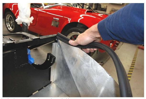
Push the aluminum weatherstrip onto the trunk sides.
