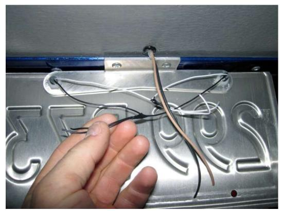
After the license plate is installed connect the white wires together and the black wires together.
