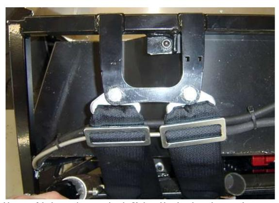
The shoulder part of the harness is mounted to the U-shaped bracket above the gas tank.
