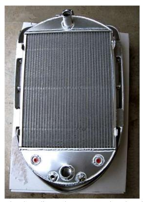
Place the radiator on the grill so that the radiator tabs are centered on the grill mounts.
