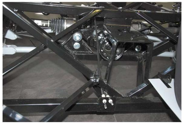
Push the cables into the bracket forward and to the right of the center section on the frame.
