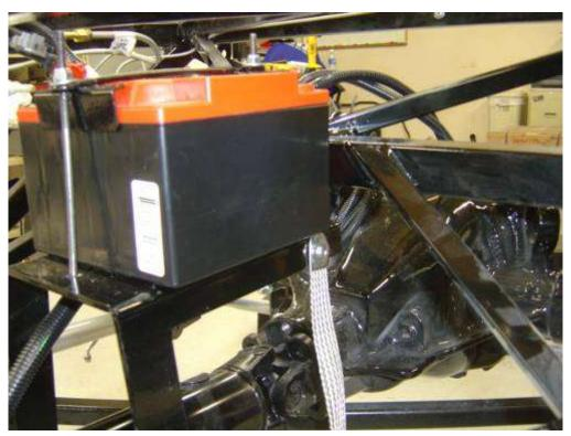
Drill a hole in the side of the battery mount plate for the ground cable to attach. Grind the paint or powder coat so that the ground cable has a good connection to the chassis.
