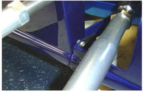
Turn the steering rack lock to lock and check the clearance of the boots with the nose cone.
