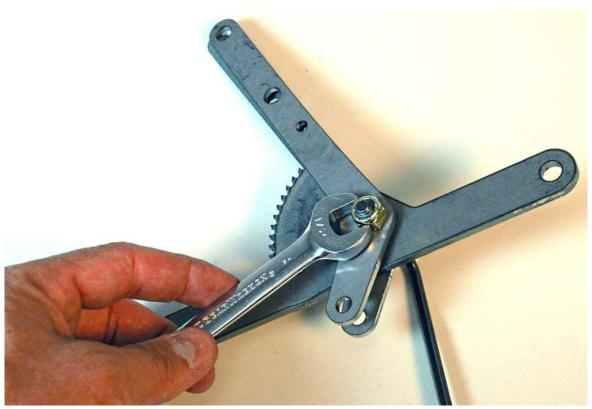
Using a <sup>3</sup>/<sub>16</sub>" hex key and <sup>1</sup>/<sub>2</sub>" wrench, tighten the shoulder bolt lock nut so that the ratchet to handle mount plates are against the bushings but they can still move up and down. Make sure the ratchet to handle mount plate next to the locknut does not get caught on the edge of the shoulder bolt.
