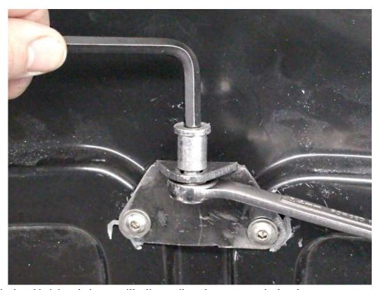
To adjust the hood height relative to grill adjust striker placement on the bracket.
