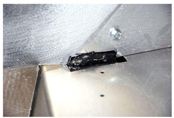
If necessary, trim the aluminum around frame welds so that the aluminum sits flat against frame tubes.
