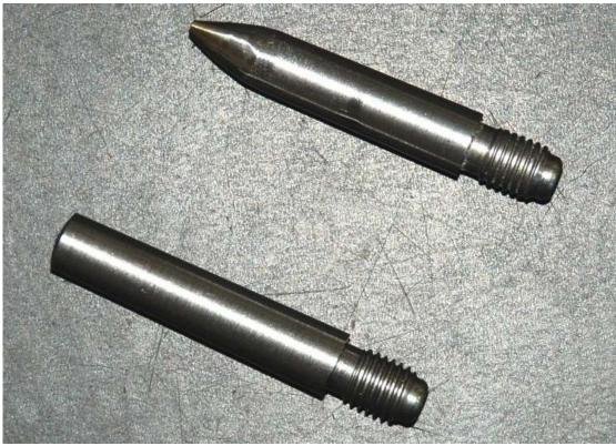
If the hood feels like it catches slightly when you close it, check the pins, they might be catching in the receiver slightly. If this happens, sharpen the end of the pins slightly as shown above and they
