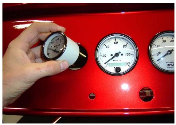
Install the gauges and toggle switches in the dash.
