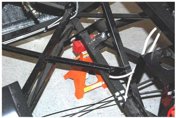
Check the location of the jack stands on the frame. The body will come down so that it is flush with the bottom of the frame. If necessary move the jack stands so they will not hit.
