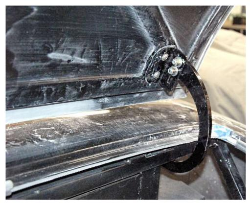
From outside the trunk, try opening the trunk. If it catches on the front edge of the trunk, more material will have to be removed.
