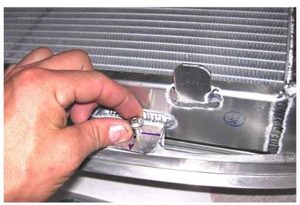
Lay the radiator back on the grill and check the hole alignment by putting the ½" button head screws in as many holes as possible.
