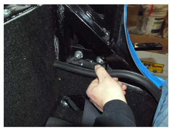
Push bulb on the side weatherstrip onto the rear edge of the side aluminum.
