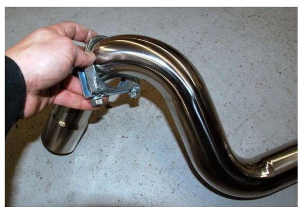
Slide one of the clamps onto the rear tube up near the top of the bend.
