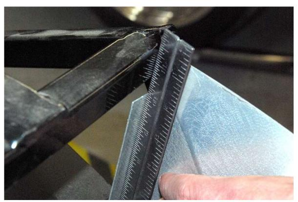
Use a ruler or straight edge to align the front bent flange on the side wall aluminum with the tube frame tube that goes across the trunk.
