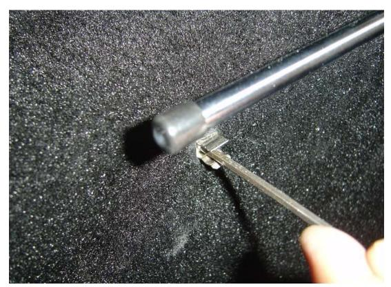
Remount the prop rod clip to the trunk aluminum. You can space the clip out from the carpet using a small rubber bumper behind the clip to give more clearance if desired.
