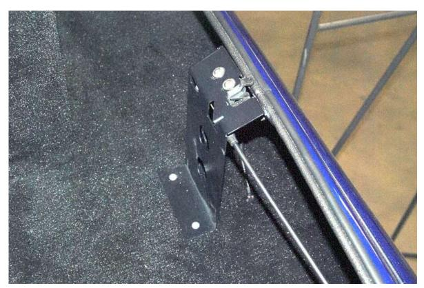
Remount the trunk latch assembly in the trunk using  $^{3}/_{16}$ " rivets.
