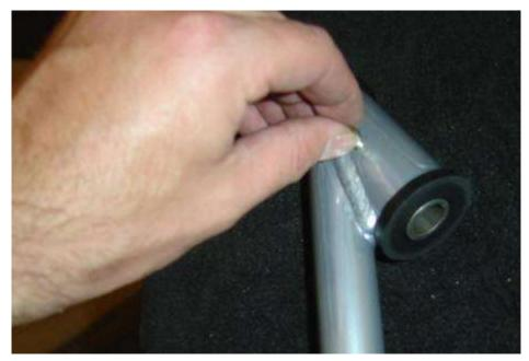
Install the grease fittings into the pivot points on the upper control arm. Attach a grease gun onto the grease fitting and fill with grease until the grease starts to seep out.
