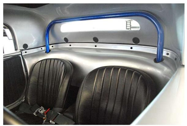
Raise the rollbar to the desired location but no closer than ½" or a finger width to the Hardtop so that there is no rubbing or contact with the top.
