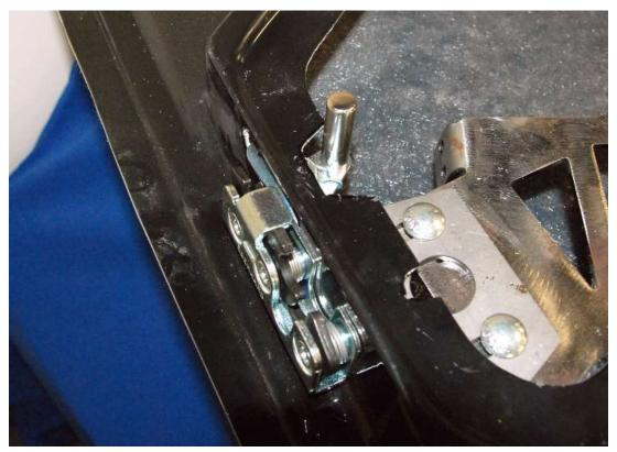
Insert the release lever into the latch and use pliers to hold it at the base. Screw the locknut onto the lever.
