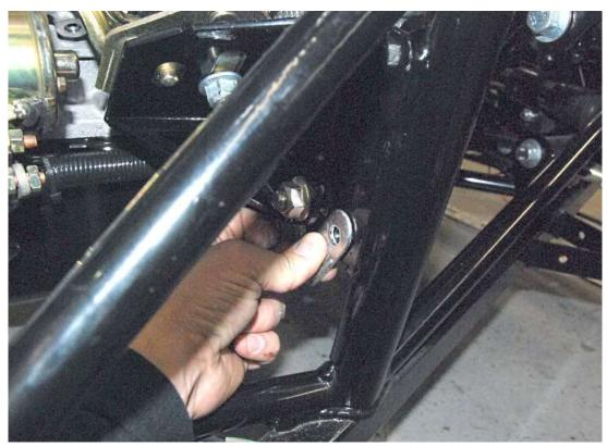
Find a location on the frame to mount the ground strap. The back side of the right engine mount is a good place.
