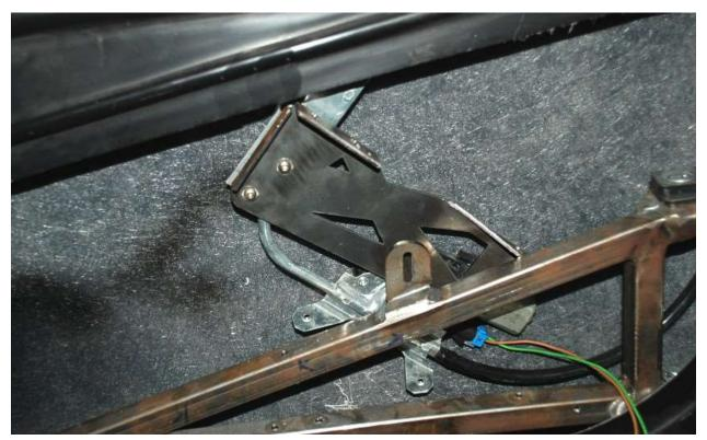
Unbolt and remove the window track. The easiest way to do this is by removing the track with the lower bracket on it. Remove the top window track bracket and bolts then slide the assembly as far to the back of the door as possible then bring the track up at the angle shown above.
