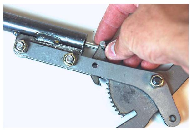
Rotate the ratchet tooth between the handle to ratchet mount plates and align the mount holes.
