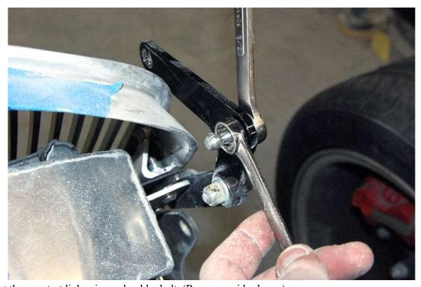
Mount the gas strut link using a shoulder bolt. (Passenger side shown)
