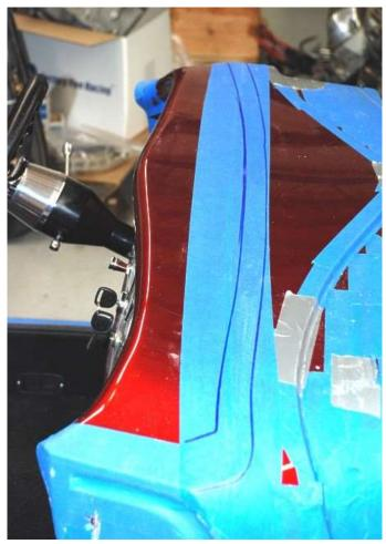
If the body is painted, use painters tape around the rear 2" of the body around the cockpit and two 2" strips across the front of the cockpit starting at the front edge of the door as shown in the above picture.
