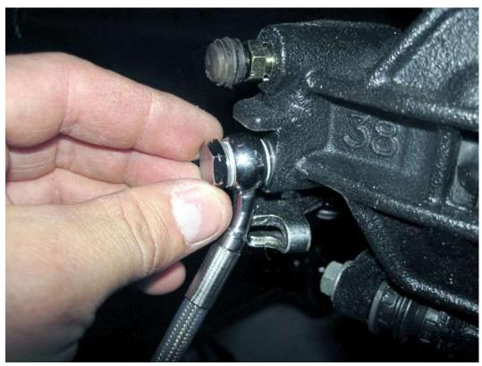
Loosely attach the flexible brake line to the brake caliper.
