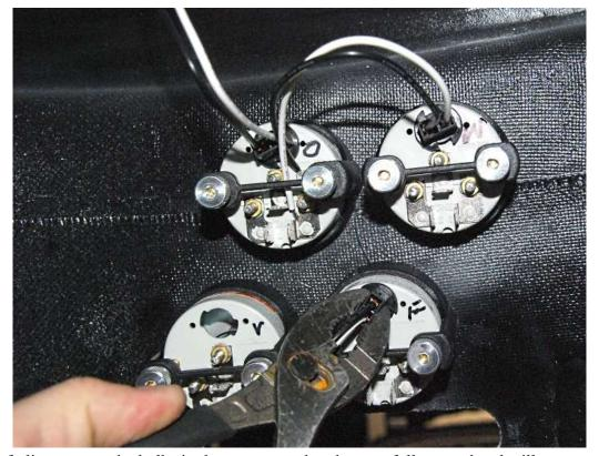
Use a pair of pliers to turn the bulbs in the gauges so that they are fully seated and will not pop out.
