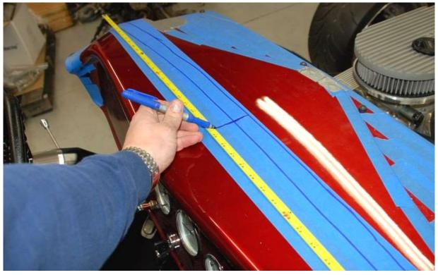
Remove the Hardtop and use a tape measure at the front top corners of the door to locate and mark the middle of the front windshield area.
