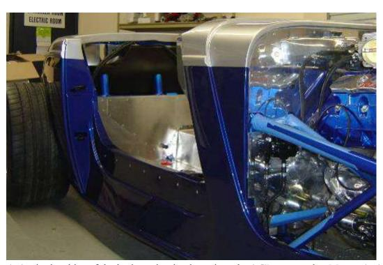
Drill mount holes in the sides of the body under the doors into the 1.5" square tube. Mount the body to the chassis with  $^{3}/_{16}$ " rivets.
