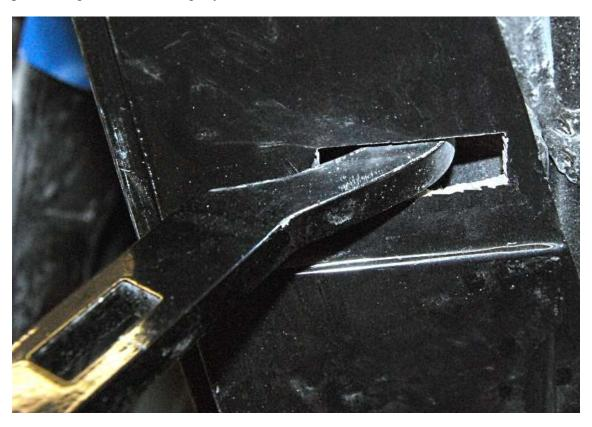
If necessary, remove the arm and cut more of the slot out. Remove the arms from the standoffs.
