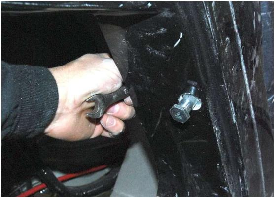
Mount the striker mount to the frame on the outside of the bracket using the  $\frac{5}{16}$ " carriage bolts provided and a  $\frac{1}{2}$ " socket and ratchet so that the striker goes through the mounting hole centered and the striker is  $90^{\circ}$  to the body.
