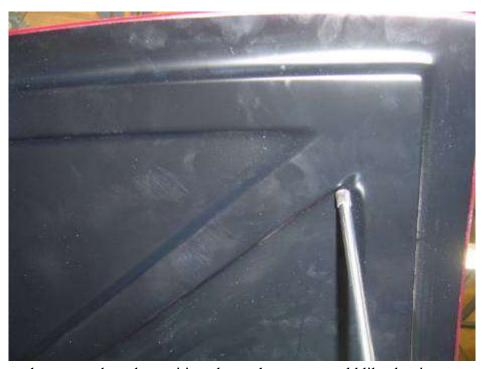
The rubber stop on the prop rod can be positioned anywhere you would like, but it seems to work the best in the triangular section on the trunk liner.
