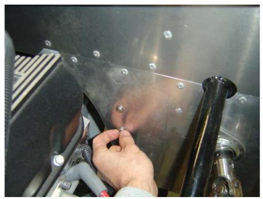
Mount the accelerator pedal to the aluminum footbox using two  $\frac{1}{4}$ "-20 x  $\frac{3}{4}$ " flange head screws in the secondary body fasteners. We like to install these fasteners from the engine side of the firewall for a cleaner look.
