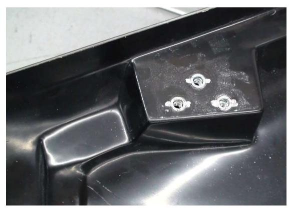
Install <sup>1</sup>/<sub>4</sub>"-20 rivnuts in the hood.
