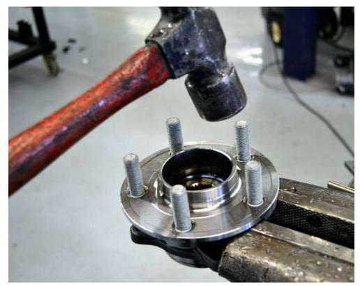
Use a vise to lightly hold the side of the wheel stud head then use a hammer to bang out the Mustang studs. Repeat for all of the studs.
