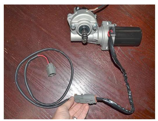
Attach the power wire harness to the motor.
