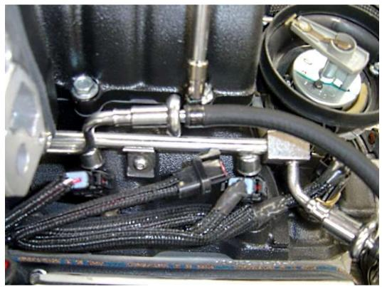
Install the rubber fuel hose from the hard line to the engine. Make sure to clamp the line onto the barbs with the correct size hose clamps.
