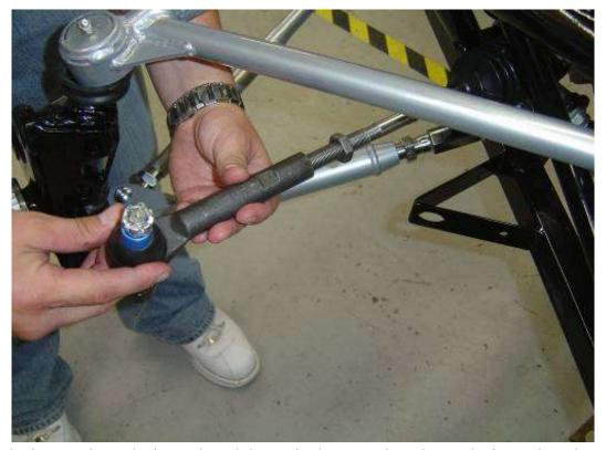
Make sure the jam nut is on the inner tie rod then spin the outer tie rod onto the inner tie rod.
