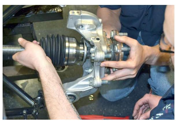
Slide the left spindle onto the outer CV joint and start the nut on the end.
