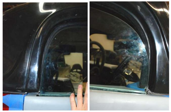
Slide the glass back and forth in the glass holder so that the gaps on each end are the same.
