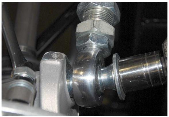
Use a  $^{15}\!/_{16}$ " wrench,  $^{15}\!/_{16}$ " socket and ratchet to tighten the locknut.
