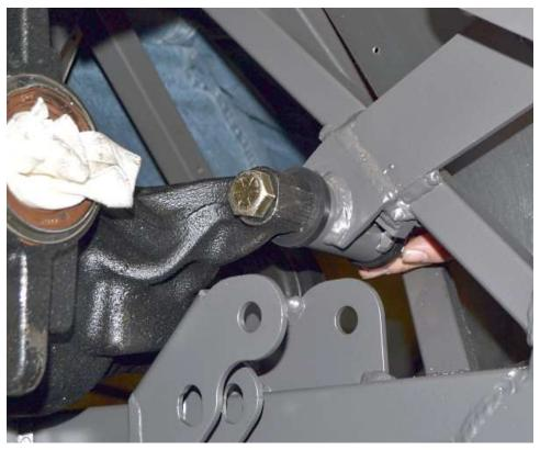
The larger/longer bolts and nuts are used for the front mounts.
