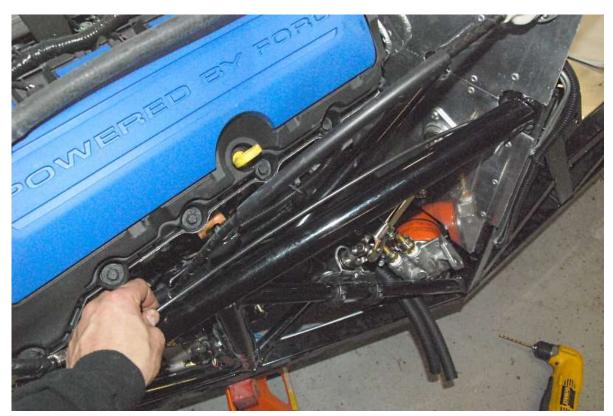
Route the cable down the inside of the 1.50" round tube towards the front of the frame.
