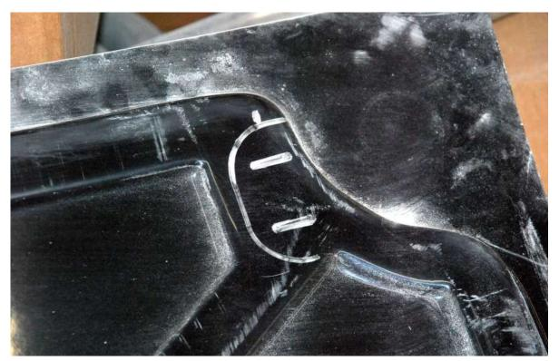
Mark around the hinge mount and in the mounting slots.
