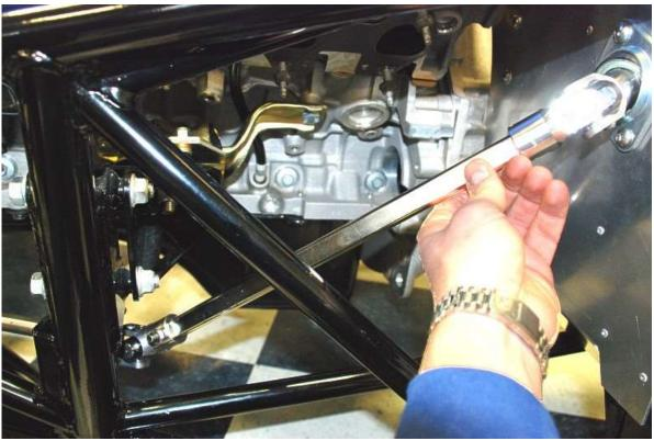
Insert the middle steering shaft into the lower joint first then insert it into the firewall joint.
