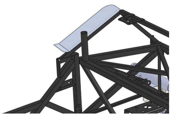
Push weatherstrip onto the top, outside and front edges of the cover panel. Insert and locate the panel so that the weatherstrip seals against the outside body and behind the door.
