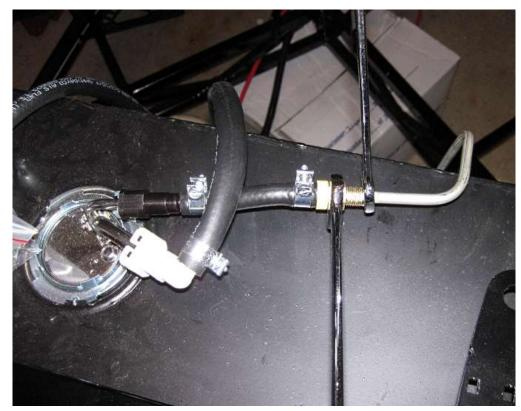
Attach the fuel line to the tank and the 1/4" hard fuel line.
