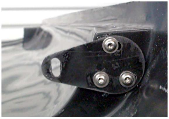
Mount the brackets to the hood centering the slots on the screws.
