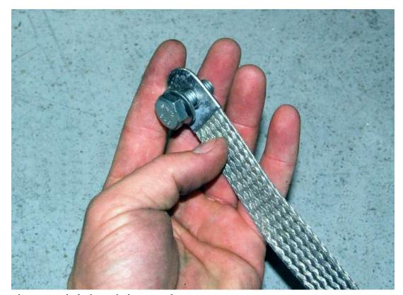
Pass the engine mount bolt through the ground strap.
