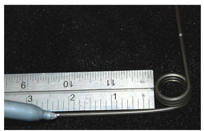
Mark the bottom leg of the spring 2.25" from the spring coil.
