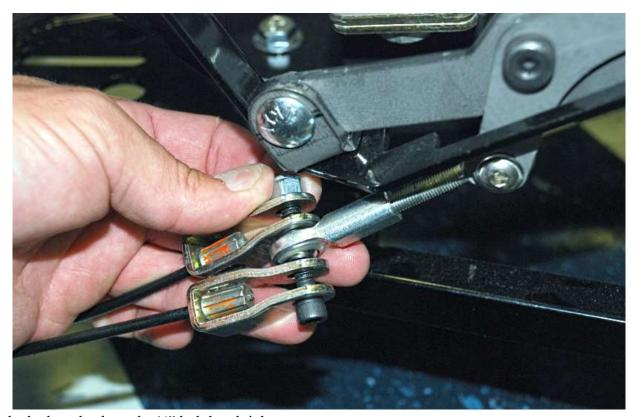
Put the locknut back on the 1/4" bolt hand tight.
