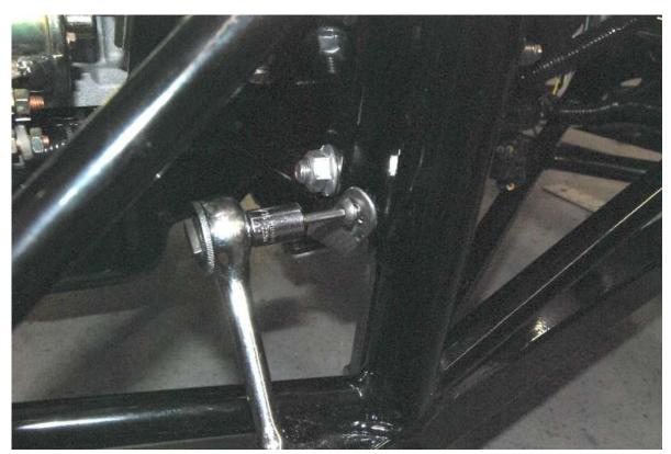
Attach the ground strap using the 5/16" button head screw and locknut provided.
