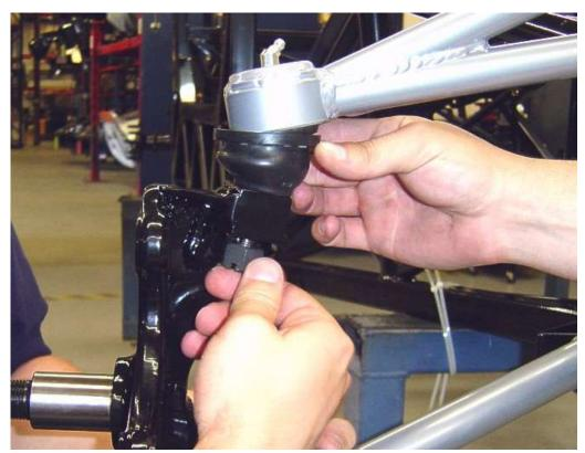
Install the front spindle on the front upper control arm with the supplied castle nut and cotter pin. Torque to 90 ft-lbs.
