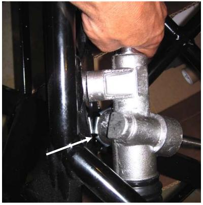
Check the fitment of the rack on the rack mount, make sure that the large nut on the rack is not hitting the plate. If it does, use a hole saw on the plate at this location for clearance.
