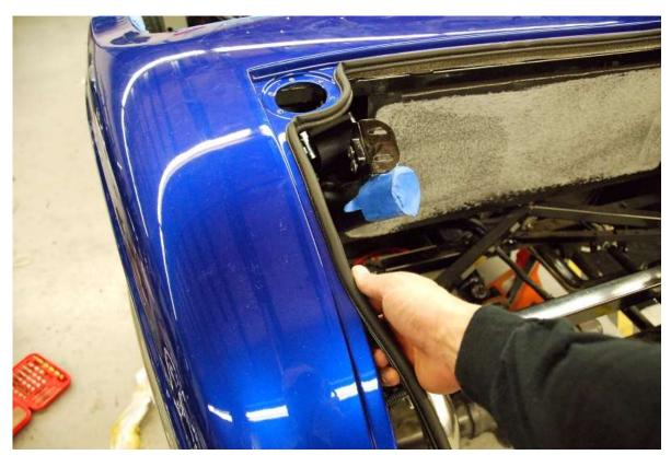
Push the bulb weatherstrip with the bulb on the side around the trunk opening starting at the bottom center.
