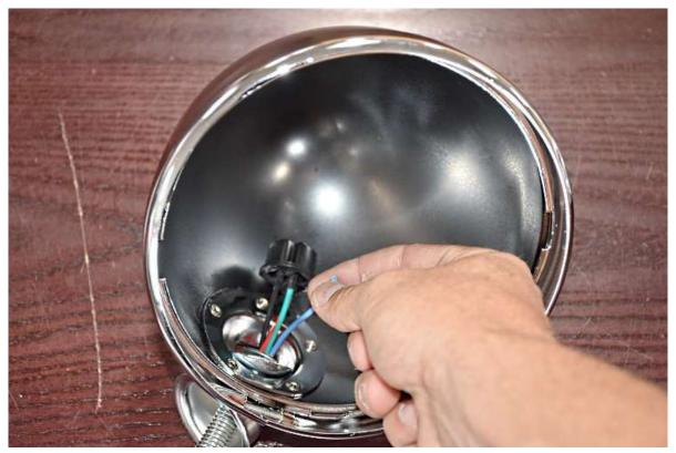
Push one of the blue wires through the mounting bolt.
