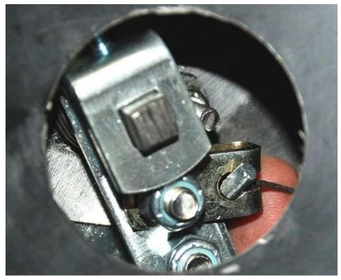
Rotate the handle the other direction so that the clevis is closer to the cable and insert the barrel fitting into the clevis.
