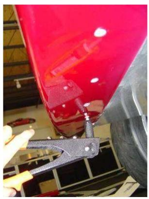
On the rear edge of the lower trunk where it meets the body, attach the trunk floor to the body with  $^{3}/_{16}$ " rivets. Apply a liberal amount of silicon between this panel and the body.
