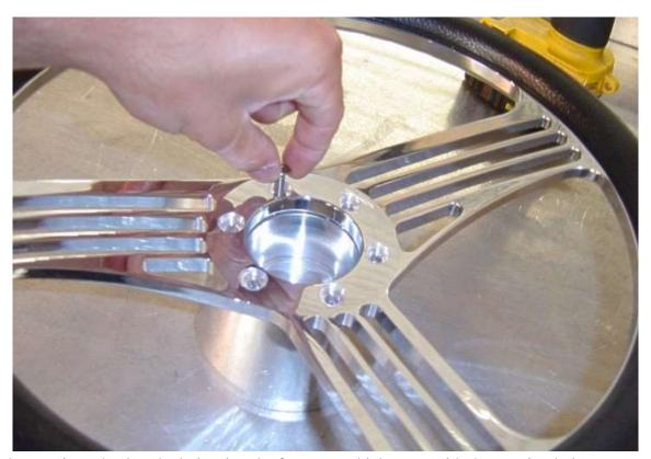
Mount the steering wheel to the hub using the fasteners which came with the steering hub.
