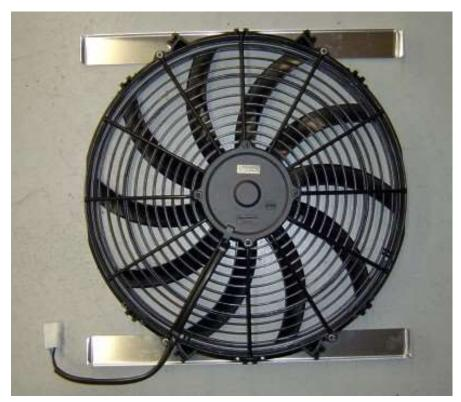
Rotate the fan assembly so that the fan wires are on the bottom and the mount bars go across the radiator then, push the fan assembly onto the back of the Radiator by putting one side in then the other. It should be a tight fit.
