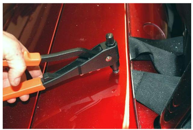
Insert and attach  $\frac{1}{4}$ " rivnuts in the  $\frac{25}{64}$ " holes drilled in the rear area of the body.
