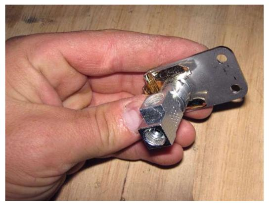
Rotate to clock the brake line adapter as shown in the picture and push on the brake line clip.
