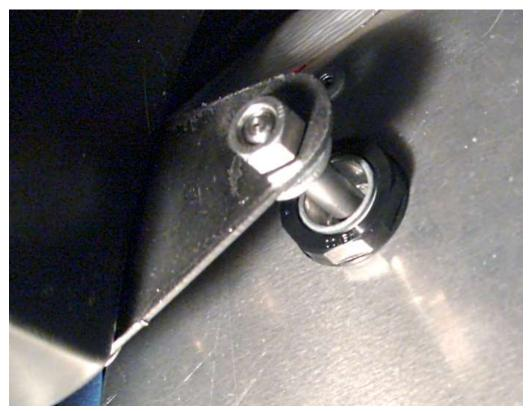
Partially close the hood, align pins with receivers, and close hood completely. Tighten the pin and bracket mounts. Open and close the hood to ensure proper alignment.
