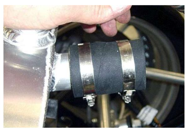
Attach the hose to the radiator using a hose clamp, 7mm socket and ratchet. It gives a clean look if you position the hose clamp so that the screw is accessible but is not seen.
