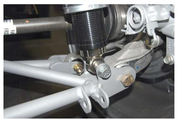
Jack the spindle up so the body end of the shocks can be mounted on the shock mount on the control arm using the longer 1.09" spacer on the back and  $\frac{7}{16}$ " spacer in front of the shock.
