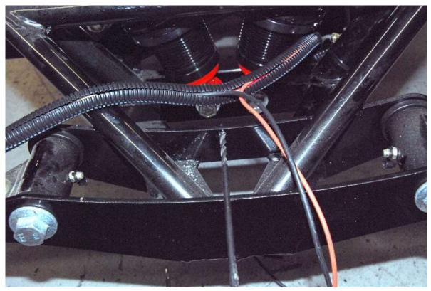
Drill a  $\frac{3}{16}$ " hole in the center of the rear lower control arm mount.
