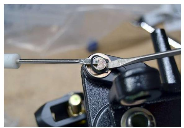
Use snap ring pliers or two small screwdrivers to remove the clevis at the top of the clutch pedal.
