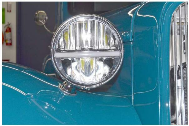
Hold the headlight up to the mounted bucket so that the center bar is horizontal and the bulb is the correct way up so the writing on the bulb is at the top.
