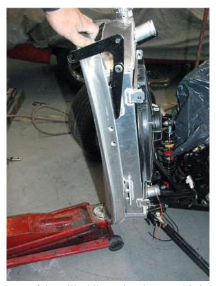
Use a floor jack to hold the bottom of the grill while getting the assembly into position.
