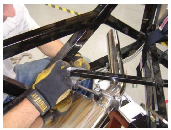
Also mark the location of the brackets that protrude past the surface of the frame where the aluminum floor sits.
