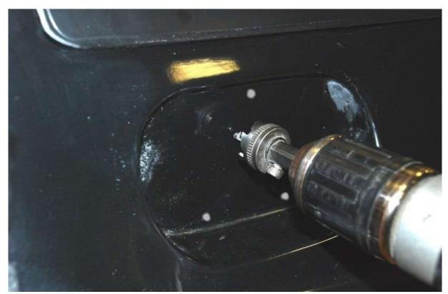
Drill the light wire hole using a ¾" hole saw.
