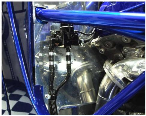
Attach the lines to the correct ports of the fuel pressure regulator or to the lines on the engine depending on your fuel system.
