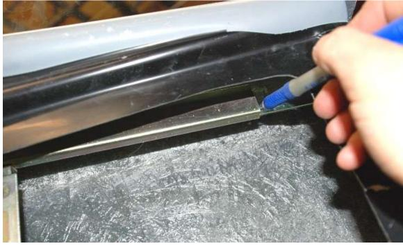
Carefully open the door without moving the glass and mark the glass at the back of the holder. Remove the window carefully. This will make it easier to locate the glass in the future.
