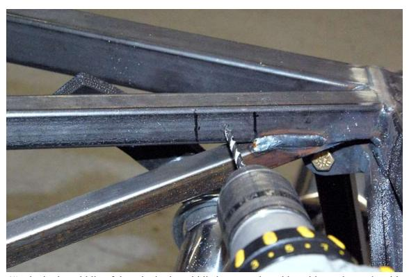
Drill the 1" tube in the middle of the tube in the middle between the rubber side marks made with a  $^{3}/_{16}$ " drill bit.
