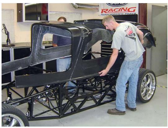
Pull the sides of the body outward ever so slightly to get the front of the body around the frame and front control arms. Make sure to tuck the front sections of the body around the upper control arms.
