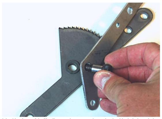
From the right side of one of the Handle to ratchet mounts, insert the shoulder bolt through the ratchet mount and then the fixed gear.
