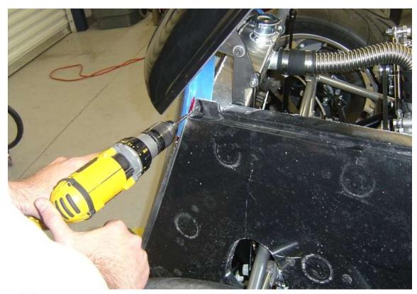
Drill a <sup>3</sup>/<sub>16</sub>" hole through the engine side panel mount flange and the grill.
