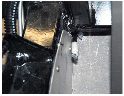
Push the gray end of the release cable into the cockpit.
