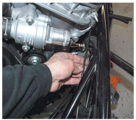
Run the cable under the 1" round tube.
