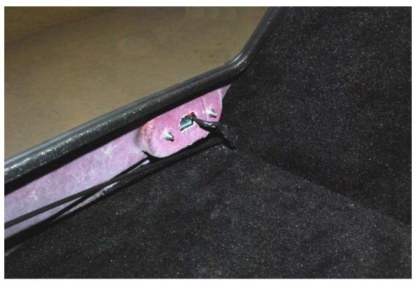
Drill an  $^{11}/_{32}$ " hole in the driver side of the trunk to run the trunk release cable through.
