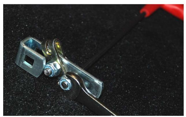
Attach another 1/4" flange head screw in the other hole as shown above. Only tighten the screw so that the screw goes through the nylon on the locknut about one thread. Remove the set screw from the end.
