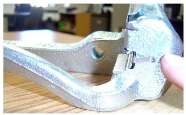
In the supplied hardware bag there are six steel clips that are designed to separate the pads from the caliper. These clips allow the pads to slide on a smooth surface and not wear on the caliper. The four clips that go on the ends of the hanger are different end to end, and must be installed with the long tab facing out.
