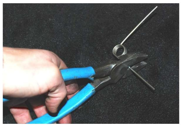
Use a heavy duty set of electrician pliers or a hack saw to cut the spring at the points marked.
