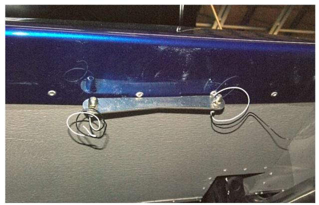
Attach the bracket with one  $\frac{3}{16}$ " rivet first then drill and attach the second rivet.
