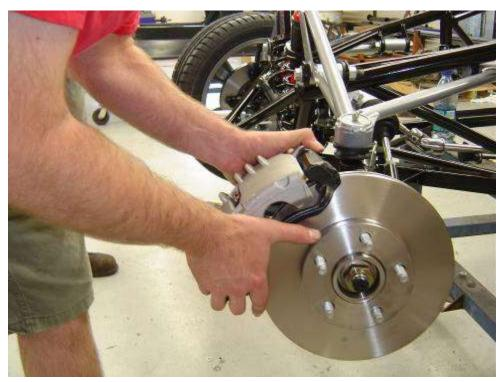
Install the calipers on the front spindles. Mount the calipers with the supplied bolts (FFR #14513). Make sure the pads are loaded into the caliper before installing it.
