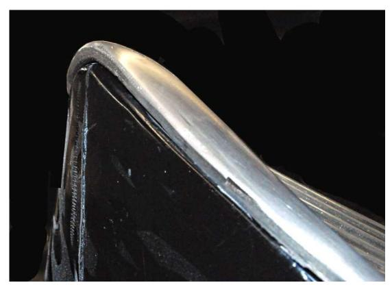
If necessary, sand some material off the bottom of the grill so the nose cone can lie flush on the bottom edge.
