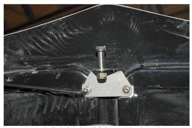
With proper engagement of striker in the latch and Grill clearance, tighten the mounting screws.
