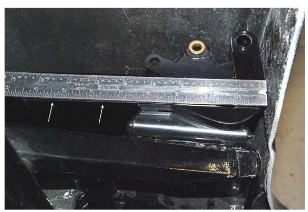
Remove the ruler and lay it on top of the hinge arm so that the arm is parallel to the frame and the ruler is along the edge of the arm and the hinge pin hole is straight forward from the standoff hole.
