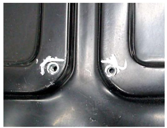
Drill the hood striker bracket holes and install 1/4"-20 riv-nuts in the hood.
