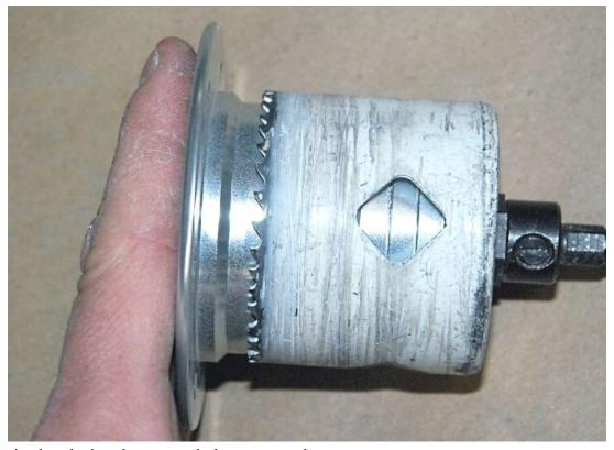
Check the size by placing the correct hole saw over the cap.
