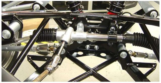
The steering rack is installed onto the chassis with the input shaft facing down and to the driver side.
