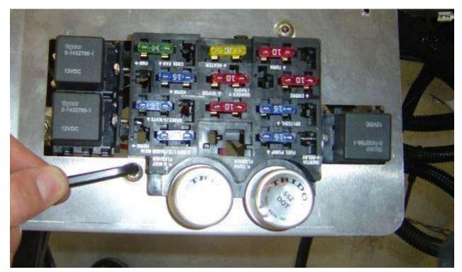
Attach the fuse block to the aluminum mount plate using the ¼" screws and locknuts. You will have to remove the flashers from the panel to do this.
