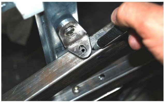
Rotate the track mount so that it sits flat on the angled door frame tube and with the end of the bracket flush with the edge of the tube, mark the middle of the slot for the bolt location.
