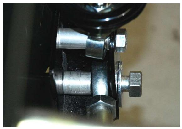
Install the shocks (body down) to the rear axle assembly. Passenger side - The longer spacer (FFR# 33238) is placed at the front of the shock and the smaller 0.125" shim (FFR# 13210) is placed at the rear.
