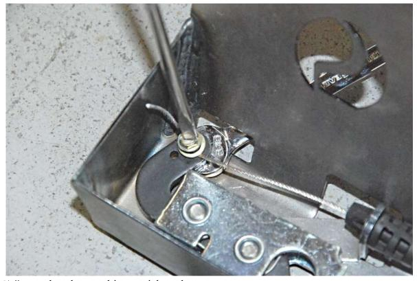
Use a  $\frac{5}{16}$ " wrench and screw driver to tighten the screw more.
