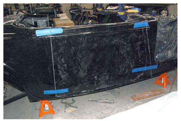
Without the door frame, hold the door up to the body, align and tape it in place.
