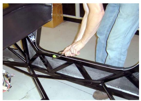
Push down slightly and clamp the door sills to the frame.
