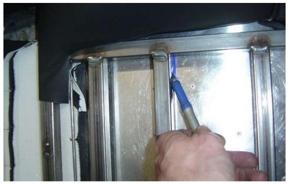
Mark the location of the seat frame on the aluminum floor.
