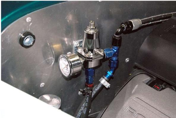
Decide where you would like the fuel lines to end up in the engine bay along with where you are going to install your fuel pressure regulator if using a separate regulator. Usually this is on the right side of the firewall.
