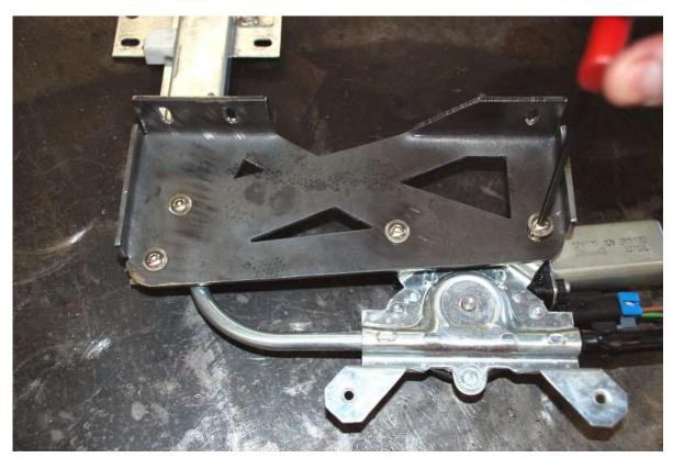
Attach the motor mount bracket to the motor/track assembly.
