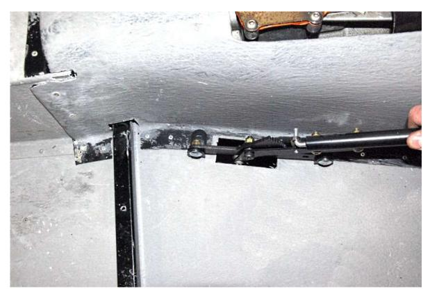
Insert a carriage bolt through the rear handle mount and into the hole drilled through the aluminum.
