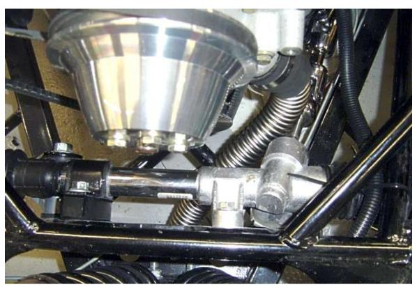
Route the corrugated tube over towards the steering shaft and into the rubber hose adapter on the water pump inlet. You will have to put a sharp bend in the end of the tube. Do not hose clamp it.
