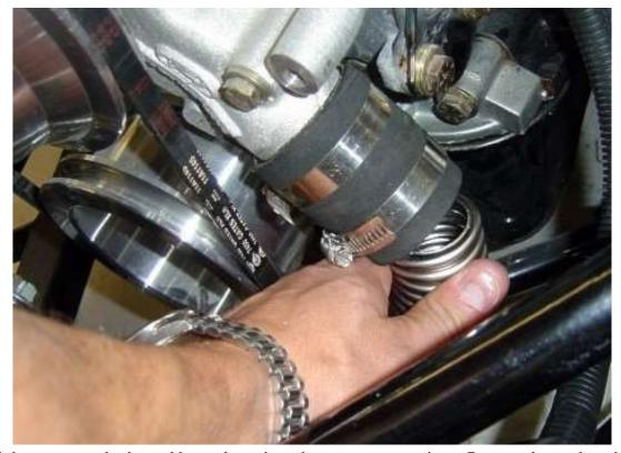
Re-install the corrugated tube and hose clamp it to the water pump using a 7mm socket and ratchet.
