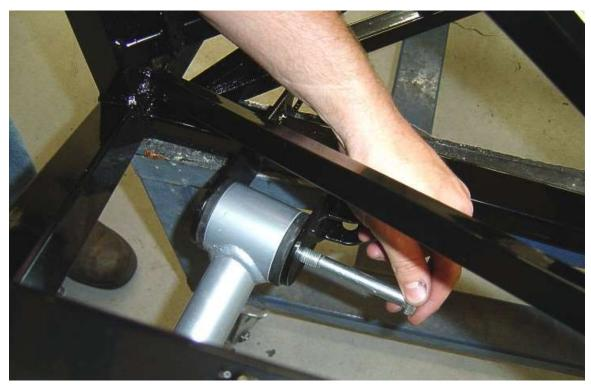
Attach the lower control arm onto the frame with the provided hardware; make sure to install this bolt from the center of the car going outward to the side of the car (FFR# 13976 & 13706 & 13751)
