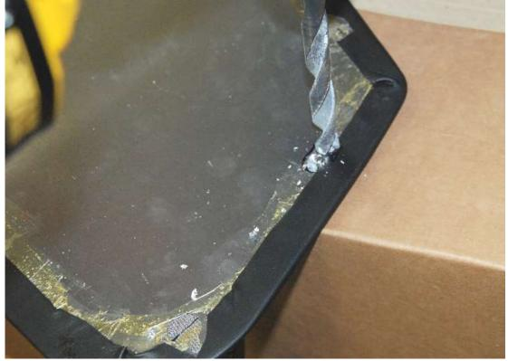
Use a  $\frac{1}{4}$ " drill bit followed by a  $\frac{5}{8}$ " drill bit to drill the two circle locations.
