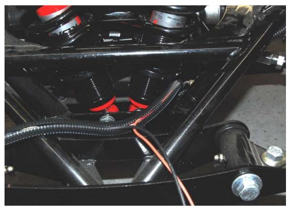
Locate/center the fan wires. If necessary, use scrap wire of the correct gauge to extend the ground wire. Re-tape where the fan wires come out of the harness.
