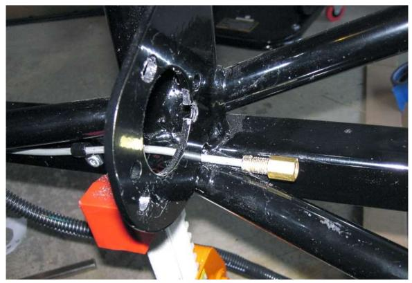
Around the location of the electric steer motor or the flange bearing for the steering linkage, install a female-female brake line union.
