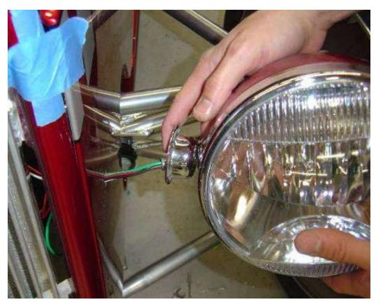
Pass the wires though the side cover, spacer and grill mount into the engine bay.
