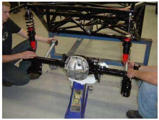
Place the rear axle assembly on a jack and move it into position.
