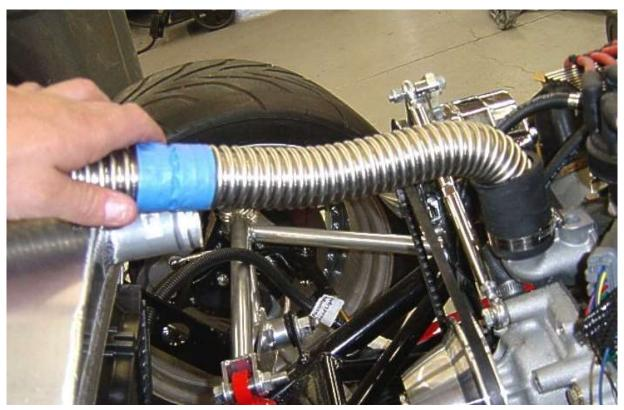
Bend and route the hose over to the radiator inlet and use a marker or masking tape to mark the cut location of the corrugated hose.
