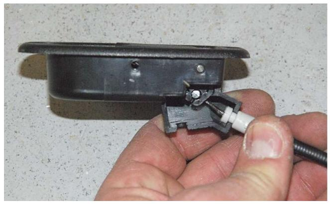
Push the cable sheath into the handle.
