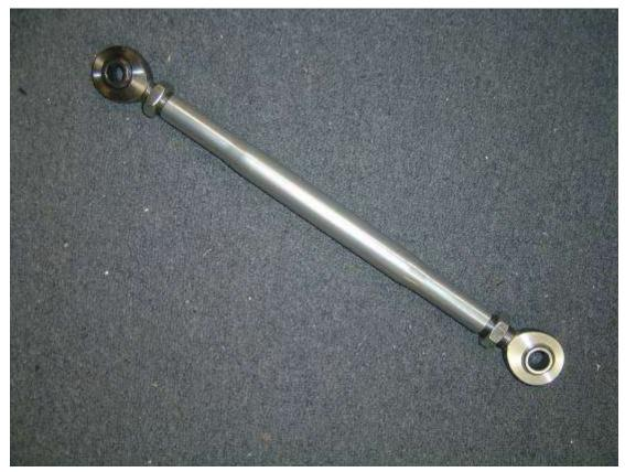
Insert the rod ends into the swaged tubes (one is right hand thread and one is left hand thread). The longer tube is the Panhard bar and the shorter one is the upper link.
