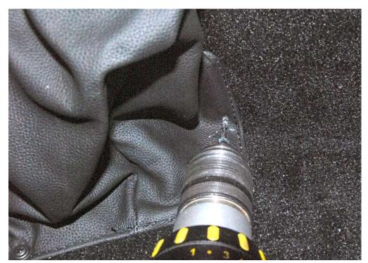
Hold the cover in place and drill a  $\frac{3}{32}$ " hole through the cover near the ring that is captured in the boot and the cockpit aluminum.
