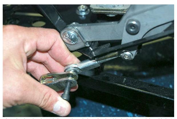
Adjust the rod end so that the 1/4" bolt goes through the rod end and both clevises and the cable is tight.
