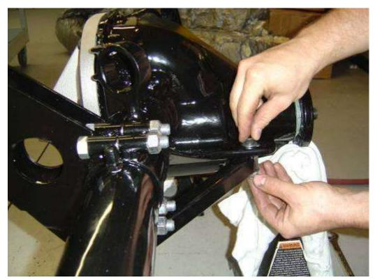
Attach the leg of the axle clamp bracket to the rear end housing (FFR# 11020 & 13964 & 13977)
