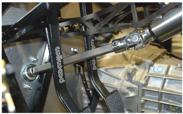
Install the  $11^{7}/_{16}$ " upper steering shaft in the other side of this joint and it passes through the firewall flange bearing.
