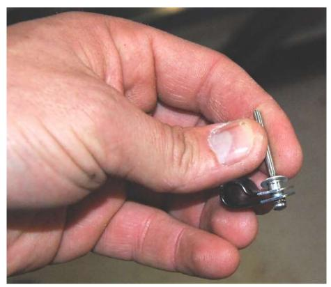
Insert a long <sup>3</sup>/<sub>16</sub>" rivet into a small insulated line clip.
