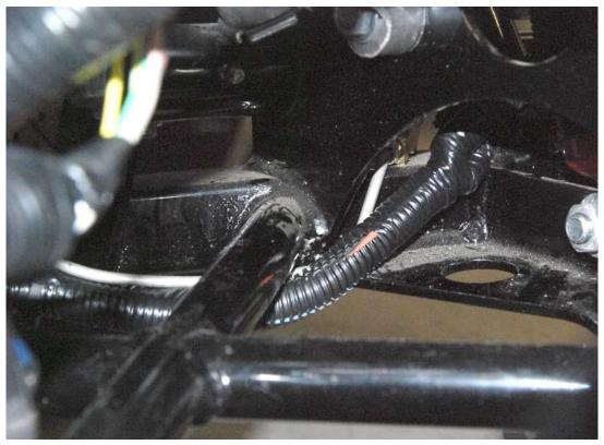
Forward of the "X" bring the harness up above the <sup>3</sup>/<sub>16</sub>" plate.
