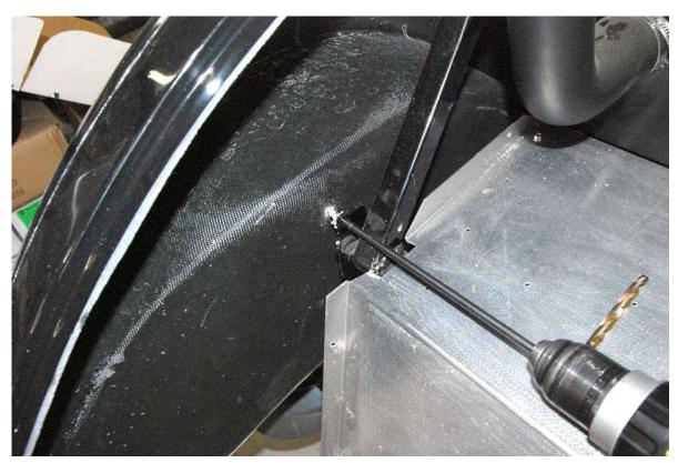
Drill through the rear wheel well body frame mounts and through the body with a  $\frac{5}{16}$ " drill bit.
