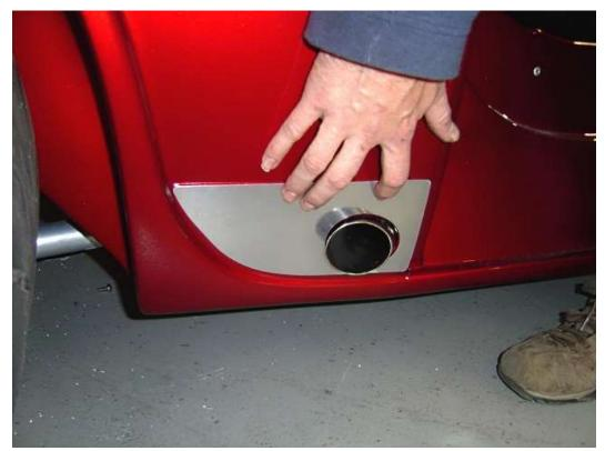
The stock exhaust is designed to exit through the body in front of the rear wheels using the aluminum with the cutout. The end of the pipe can be cut to the angle desired.
