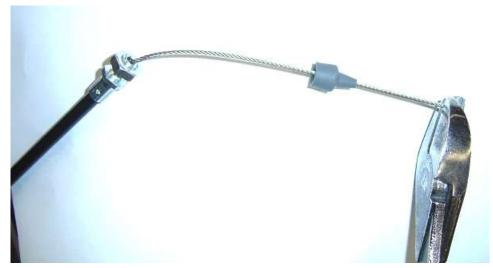
Using a pair of wire cutters, cut the barrel fitting off the cable.
