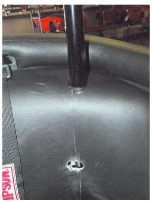
Drill the rear cockpit cover with the hole saw size appropriate for the way the quick release pins will be run.
