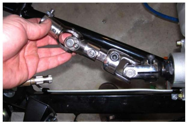
Insert the ¾" DD shaft into the steering rack and motor joints.
