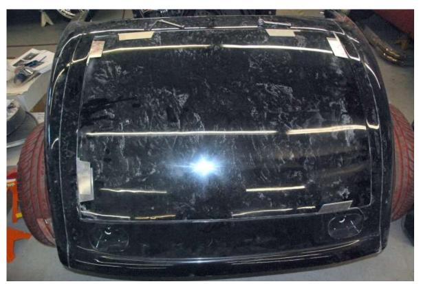
Use shims or washers to set the gap so that it is even around the sides and top of the trunk.
