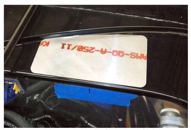
Place the aluminum access hole cover on the driver side of the hood recess of the body.
