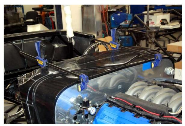
Attach the clamps between the dash and firewall.
