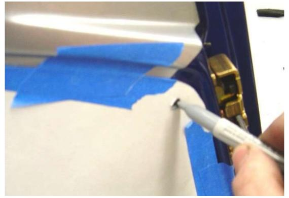
Position the template on the door and attach it with masking tape.
