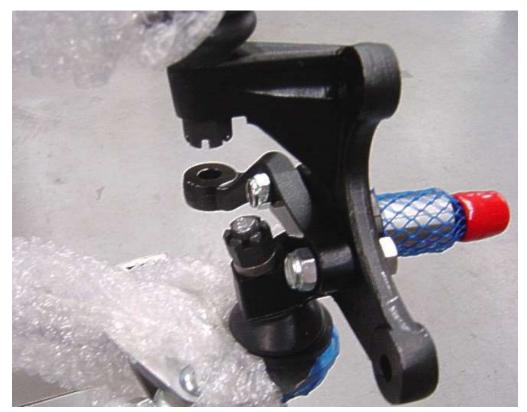
Install the spindles on the control arms next. Torque this castle nut also to 110 ft-lbs. Make sure to install the cotter pin after you torque it.
