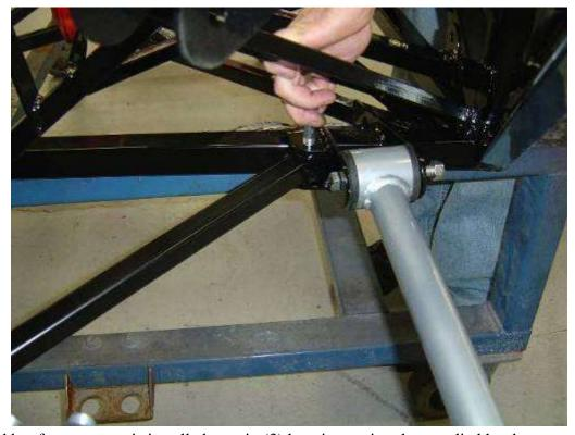
The Panhard bar frame mount is installed next in (3) locations using the supplied hardware.
