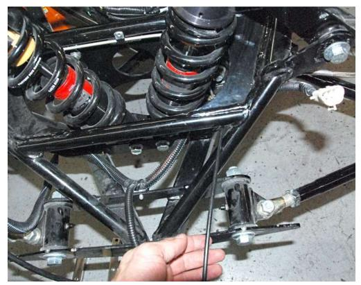
Run the cable under the coil over 1" cross tubes.
