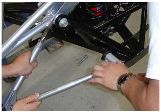
Install the lower control arm onto the frame. The fixed part with the ball joint is towards the rear of the arm.
