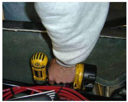
Drill through the flange on the bottom of the panel and through the body in two or three locations with a ½" drill bit.
