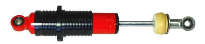
Slide the coil sleeve over the body of the damper beginning at the end which has the rubber bump stop. The unthreaded end of the sleeve goes first so that it will sit on the snap ring on the shock body.
