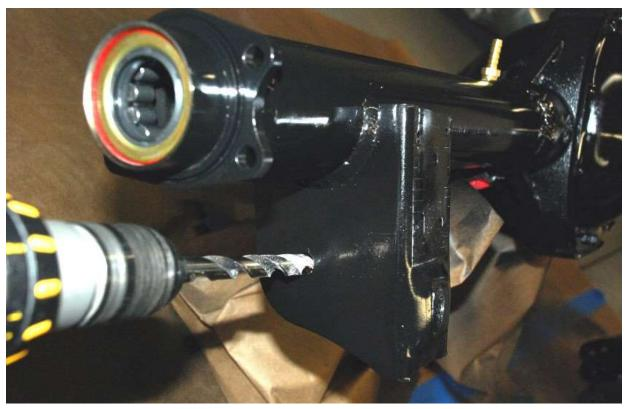
Drill the lower control arm mount holes with a ½" drill bit.
