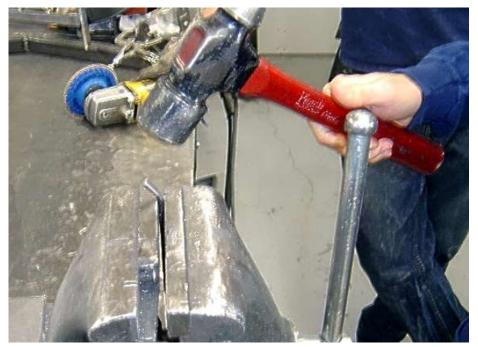
Place the J-bolt in a vise with approximately 1" of the shaft sticking above the jaws of the vice. Using a hammer, form a new "J" in the J-bolt.
