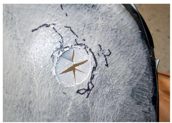
Cut the rollbar hole vinyl into pie pieces and roll them through the hole and stick them to the back side. Fold the vinyl over the edges of the fiberglass and stick it to the back side of the fiberglass.
