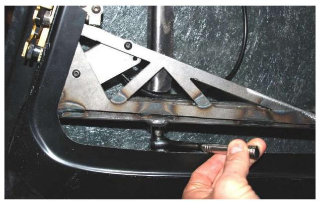
Make sure that the interior door latch cable goes under the U-channel and stays between you and the U-channel, not between the U-channel and the door skin. Tighten the carriage bolt lock nut with using a ½" socket and ratchet.
