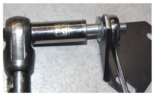
Attach the striker to the striker mount using a ¾" socket and ½" wrench leaving the locknut loose so the striker can move in the slot.
