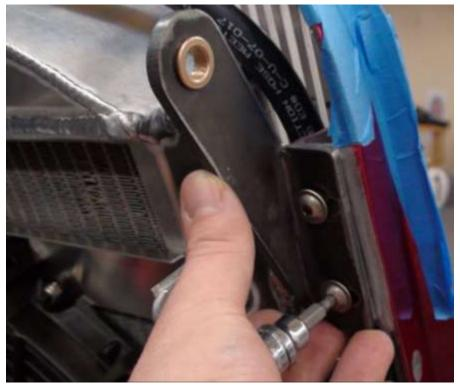
Mount the Grill mount to upper radiator mount. Leave the screws snug for later adjustment. (Passenger side shown)
