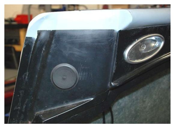
For easier access to the outer door handle parts it is recommended to have a hole in the angled part of the inner door liner which goes against the dash with the door closed.
