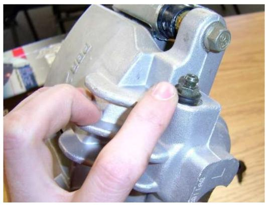
Install the caliper on the spindle; make sure that the fluid bleeder is at the top of the caliper. Note that the caliper marked LH will actually mount on the pass/right side so that the bleeder screw will be at the top of the caliper. Torque the caliper mounting bolts to 130Nm (95 ft-lb).
