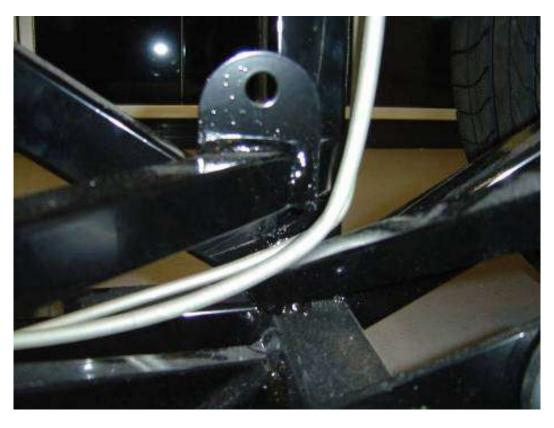
Run the fuel line down sharply to the lower inside of the side 1.50" tube. The lower the better (but above the bottom of the tube) to keep it away from the exhaust if you are going to run the side exit pipes. Position insulated line clamps to hold the fuel line every 12" or on each side of a bend.
