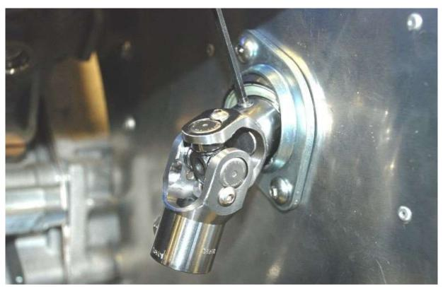
Attach another <sup>3</sup>/<sub>4</sub>" to <sup>3</sup>/<sub>4</sub>" DD joint to the end of the shaft after it exits the firewall with the shorter end touching the bearing. On this joint use the short set screw provided and no jam nut next to the firewall. Use Loctite on this set screw when tightening for the final time.
