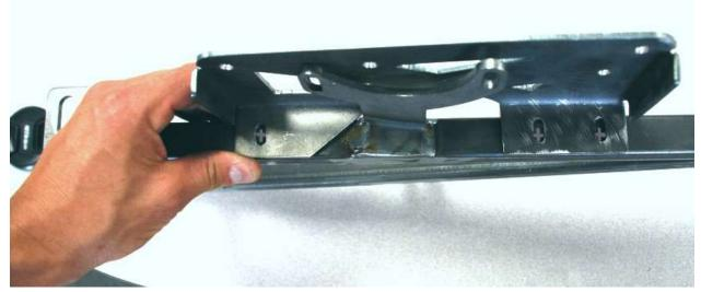
Use the bracket to double check the holes. Note that the bracket will not mount parallel to the frame but at an angle which is the reason behind the different measurements to the side of the tube. Make sure to offset the left side door frame hole to the correct side of the frame.
