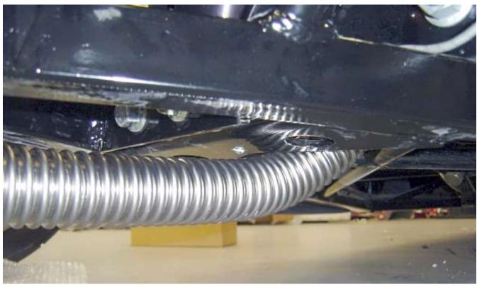
From the underside of the frame, pass the corrugated radiator hose up behind the shock mount plate but in front of the 1" tubes.
