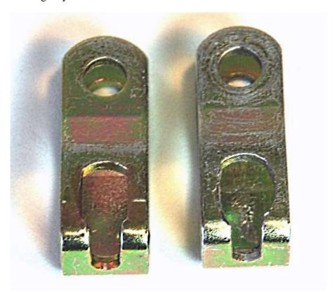
If necessary, use a drill bit and drill or a Dremel tool to open up the slot slightly.
