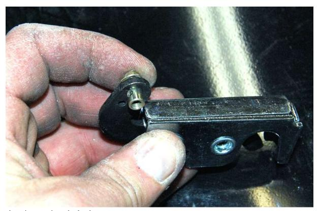
Insert the wire stop into the latch.
