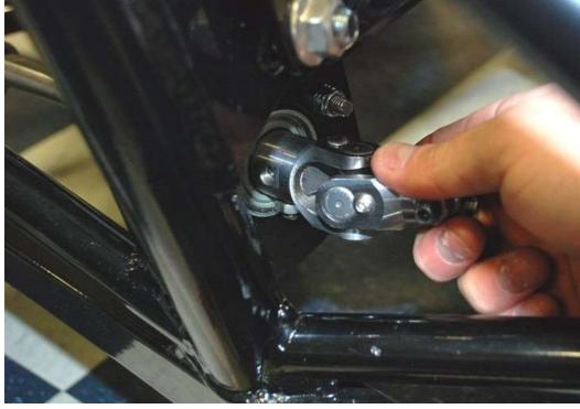
Attach the  $15^{1}/_{16}$ " middle DD steering joint to the end of the front steering shaft. The short end of the joint should mount to the front shaft and sit against the bearing.
