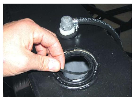
Place the rubber ring in the groove in where the sender will go in the top part of the tank near the vent.
