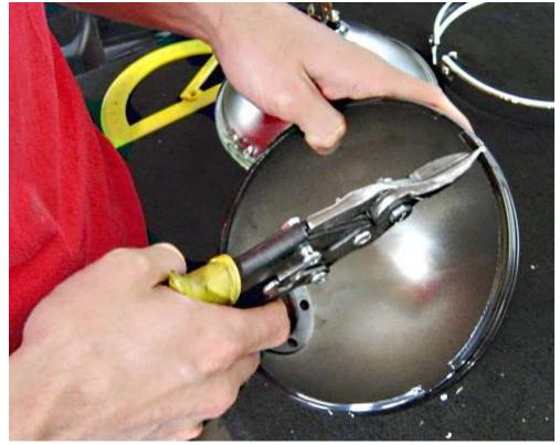
Use tin snips to cut the marked areas on the front face of the bucket for the bulb.
