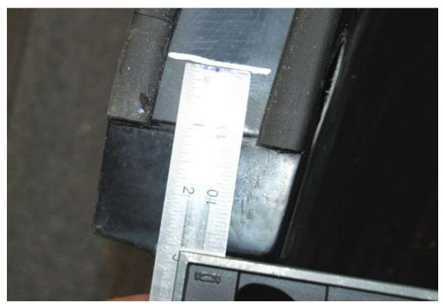
On the sides behind the window, mark 2.75" in from the inside window edge.
