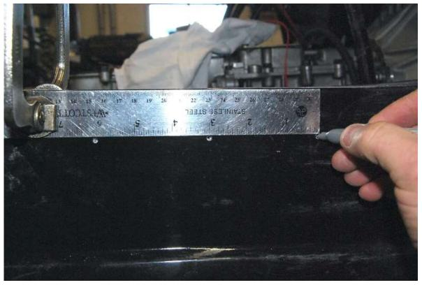
Use a marker and ruler to mark the under door body mounts 1" down from the door sill spaced every 3".
