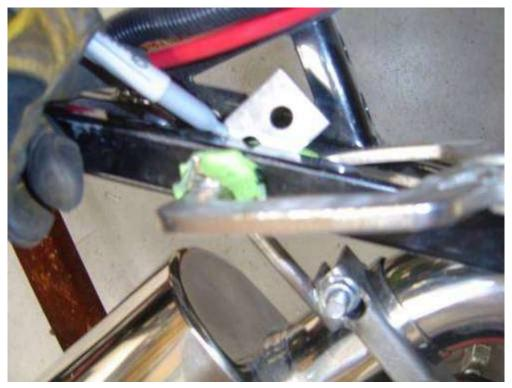
The mount tabs for the exhaust mounts have the ability to slide on the rubber bushing. Position the mount tabs so that they overhang the frame rails. Mark the location of the frame on the mount tab so that you can bend it up at a 90° angle to mount to the frame so that the bolt holding it to the frame is in sheer if possible.
