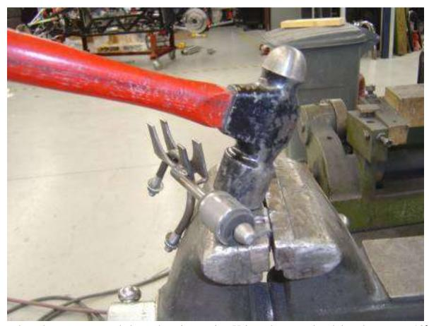
Remove the exhaust mounts and clamp them into a vise. Using a hammer, bend the tab over to a 90° angle.
