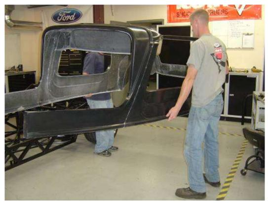
It is helpful to have a friend or two when mounting the painted body. One person on each side pulling out slightly and one in the rear is the easiest way to do this. Also make sure that the exhaust tip is not installed as it protrudes though the body. You can leave the door hinge standoffs on the frame just be very careful with the body when pulling it out to go over them one at a time.
