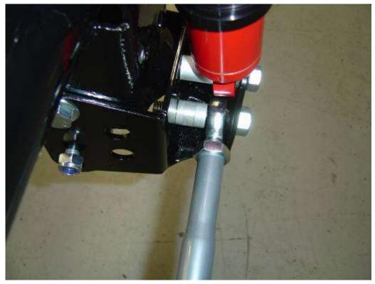
Install the Panhard bar into the passenger side traction lock bracket. Three spacers are used in the front (2) 0.375" (FFR# 33239) and (1) 0.25" (FFR# 33240). The rear uses the thin 0.0625" shim (FFR# 13337)
