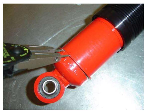
On the rear shocks only, use snap ring pliers to move the snap ring to the second groove on the shock body.
