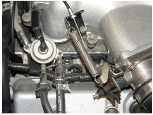
Accelerator cable mounted on '98 4 valve intake.
