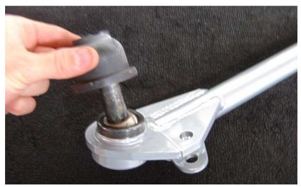
Dust boot placed over lower control arm ball joint.
