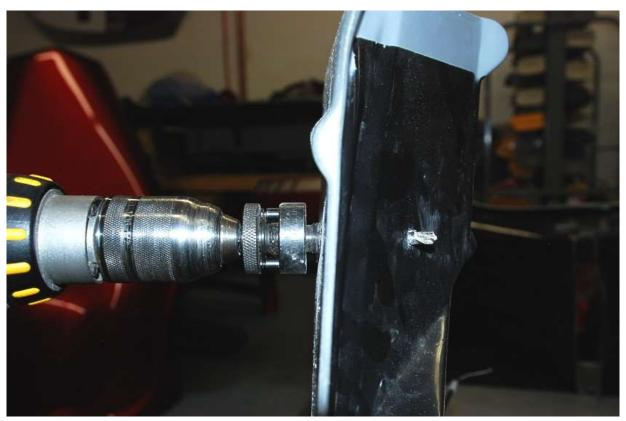
To locate this hole, once the outer skin is cut, go through the inner door skin with the pilot bit of the hole saw only.
