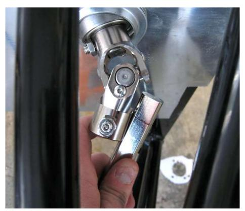
Hold the middle shaft up to the joint that is mounted on the firewall and mark where the shaft needs to be cut so that the end is flush with the inside of the joint.
