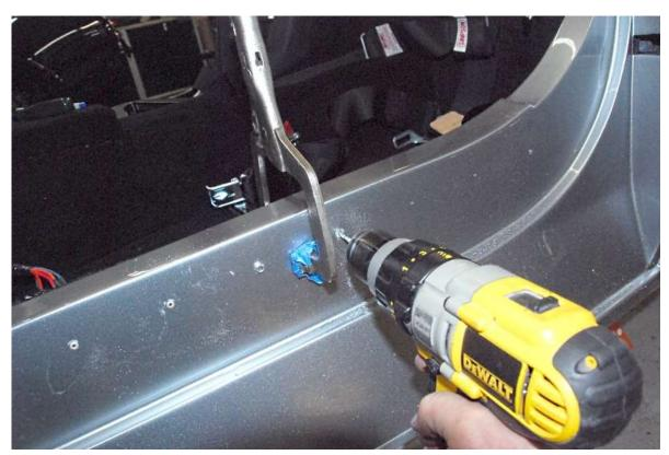
Drill and rivet the sides of the body to the frame using the screws used before paint as a guide for locating.
