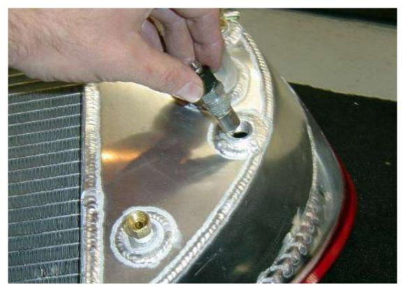
Insert the electric fan thermostat switch in the bottom center threaded bung on the radiator.
