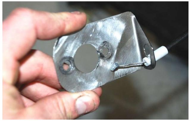
Insert the cable end into exterior door handle backing plate.
