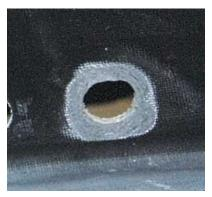
Test fit the ignition switch. If necessary remove material on the back side of the dash area to allow more than two threads to engage.
