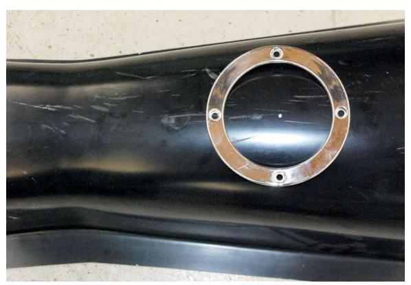
Center the shifter boot ring over the point marked so that the mounting holes are front/back and on the sides.
