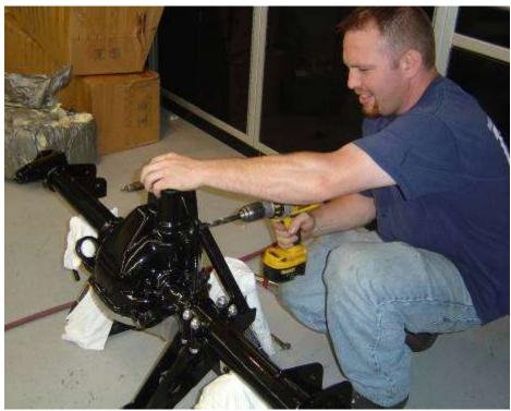
The bottom attachment of the axle clamp bracket attaches to the hole on the flange section of the pumpkin. This hole has some variance and may need to be drilled out from the bottom side.
