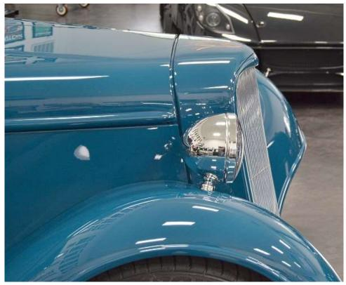
Front to back the front of the trim ring is even with the edge of the grill and the back is even with the back of the cowl.
