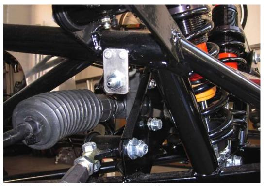
Torque the front flexible brake line to caliper banjo bolts to 29 ft-lbs.
