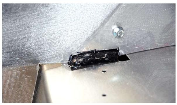
If necessary, trim the aluminum around frame welds so that the aluminum sits flat against frame tubes.
