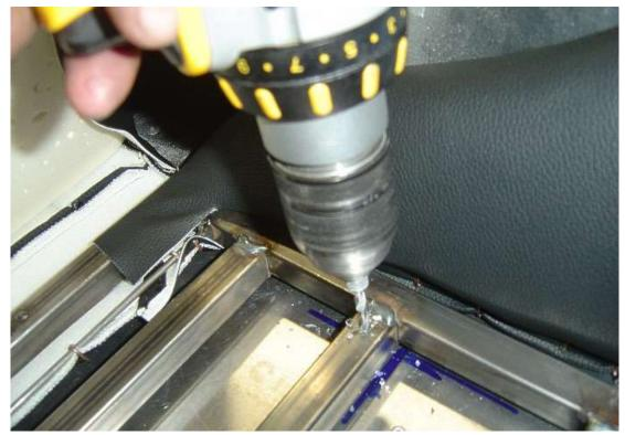
Drill (4) holes through the metal framework of the seat and through the frame.
