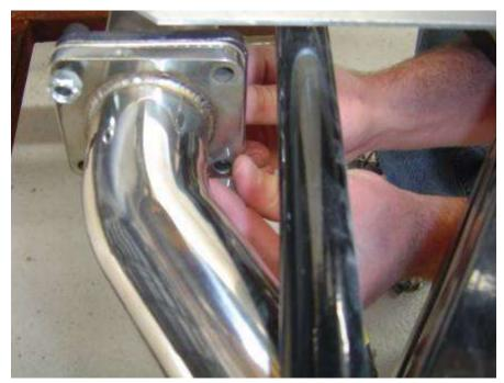
Attach the front exhaust pipe assembly to the shorty pipe with the supplied <sup>3</sup>/<sub>8</sub>" hardware. Make sure to install the supplied gasket (FFR# 33369) between the two square flanges.
