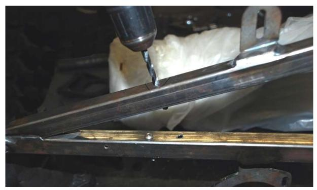
Remove the mount/window track assembly and drill the window track mount hole.
