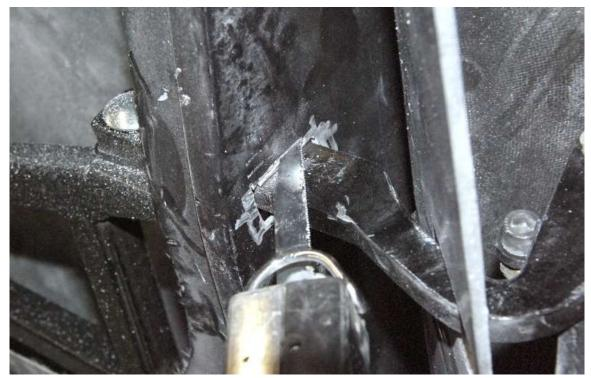
If the door is high, it may be sitting on the hinge arms. Trim the door hinge arm opening with a saw if necessary.
