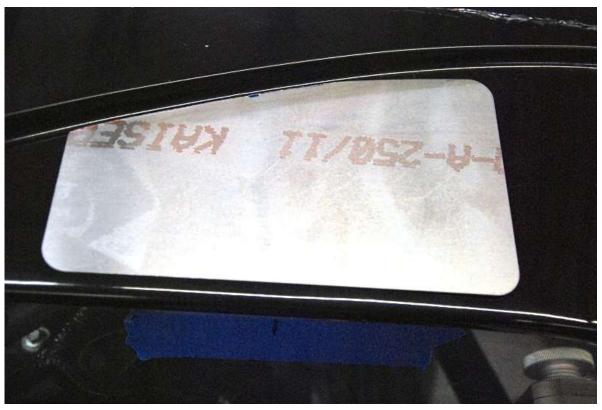
Trim the aluminum panel as needed and test fit.
