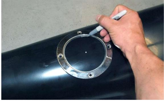
Reposition the ring so it is centered on the shifter point and mark the inside of the ring on the tunnel cover.
