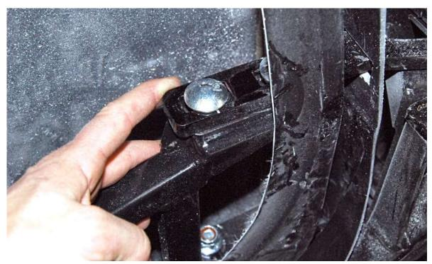
Move the hinge arms so that they are straight or as far towards the center of the car as possible. The top arm is especially important since this is the arm that hits the stop. The further in the arm is the more the door can open before it hits the stop. Cut the door hinge arm openings more if necessary. Try to make the latch mount vertical.
