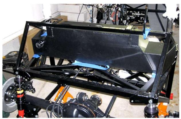
Position the tank in the frame so that is about even on both sides with the side 1.5" square frame rails. The tank should be slid all the way forward just before the front face of the tank comes into contact with the 1" down-tubes. Make sure the rear face of the tank is behind the horizontal tube located above the tank (the trunk aluminum has to attach to this tube during a later step.
