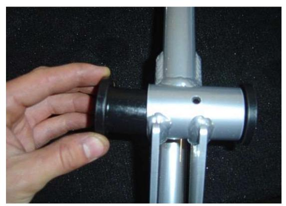
Insert the poly bushings into the front upper control arm.
