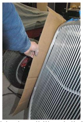
Cut one of the flaps off one of the larger boxes and hold it up to the side of the grill. And put a small mark on both the grill and cardboard where it starts.
