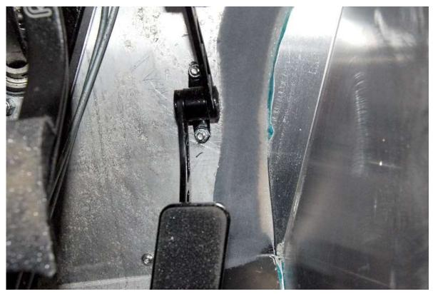
Mark the flange on the side of the tunnel if it hits the accelerator pedal mount.
