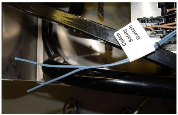
If a switch is not going to be used, connect the two wires together by either soldering the wires or using a butt connector from the "misc. electrical components" assembly in the Factory Five Racing main kit pack.
