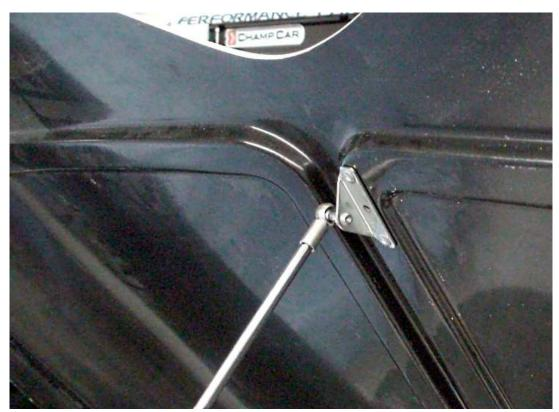
Drill and install <sup>3</sup>/<sub>16</sub>" rivets. Snap the Prop Rod onto the ball stud.
