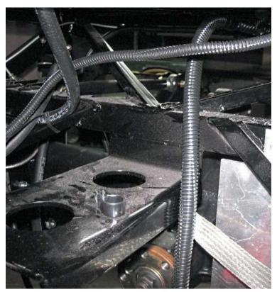
Here, the battery cable stops and will get attached to the battery after installation and the rear harness continues up next to the battery mount location and over the 1.50" tube.
