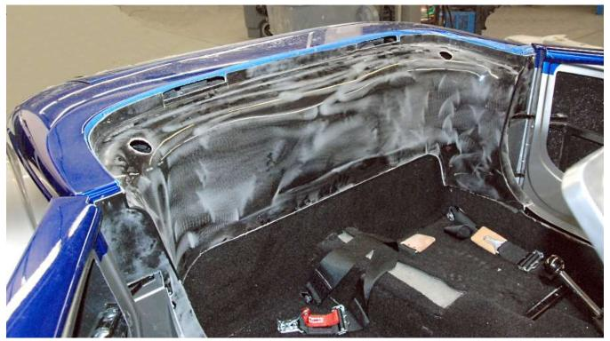
Sand the surface of the rear cover so that the glue will "bite".
