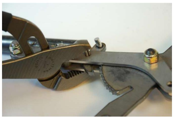
Push the included spring pin through the ratchet mount plates and the ratchet tooth using a pair of channel lock pliers.
