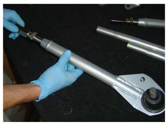
Thread adjuster into lower control arm
