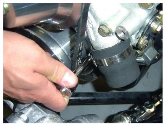
Attach the large hose to the water pump using one of the hose clamps and a 7mm socket and ratchet. It gives a clean look if you position the hose clamp so that the screw is accessible but is not seen.
