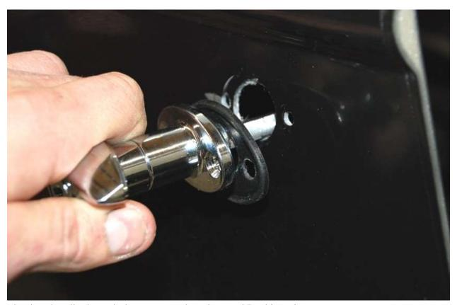
Pass the door handle through the mount gasket, door and Backing plate.
