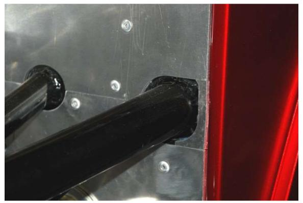
After the body is mounted for the final time, attach the Firewall fill pieces to the body flange using silicone and hold it in place with masking tape until it has dried.
