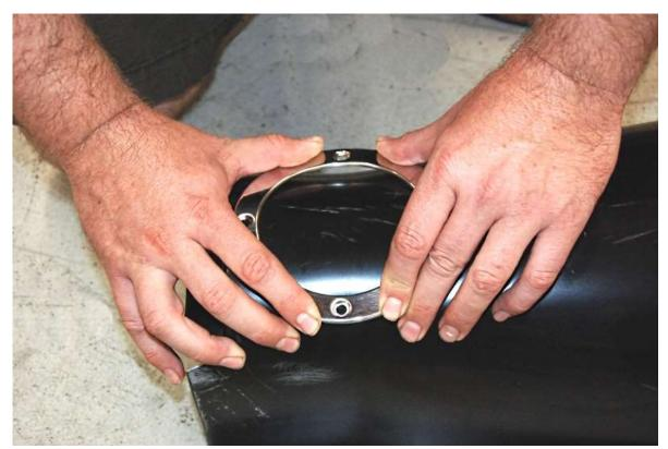
Push down on the sides of the ring so that the ring forms to the shape of the cover then move the ring back to the narrow part of the tunnel, make sure it is oriented correctly and push it down to the tunnel to shape the ring more. It will spring back a bit to the correct shape.
