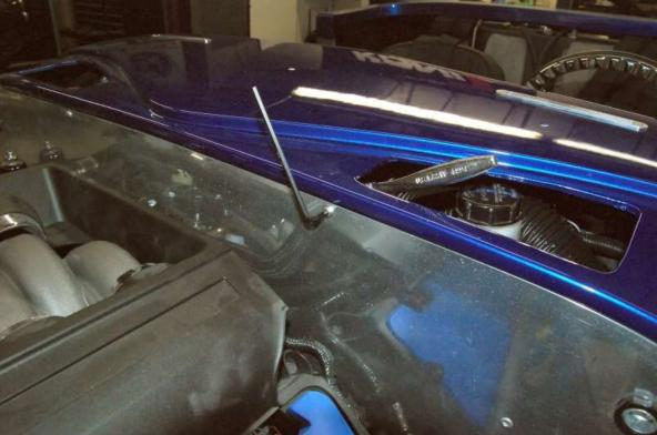
Attach the aluminum firewall and footboxes to the body using either  $^{3}/_{16}$ " rivets or screws.
