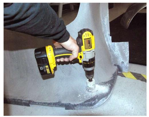
Turn the panel upside down and drill the hole positions marked using a  $1\frac{3}{4}$ " hole saw. Make sure that the hole saw is angled like the rollbar would be and **not** perpendicular to the panel surface.
