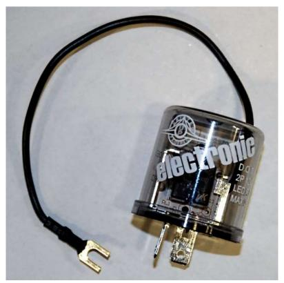
Locate the electronic flashers in the kit pack. These must be used instead of the standard flashers because of the LED rear lights. The flashers are located on the fuse block for the flasher and turn signal.
