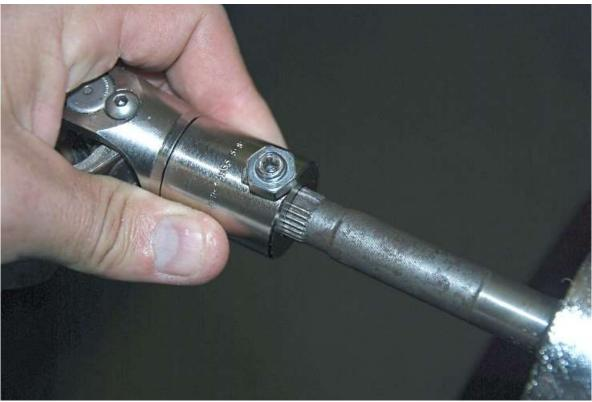
Push the steering joint (<sup>9</sup>/<sub>16</sub>"-26 spline to <sup>3</sup>/<sub>4</sub>" DD) all the way onto the input shaft of the rack making sure to align the set screw with the flat on the input shaft then tighten the set screw.
