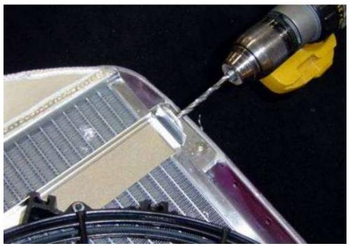
Drill though the radiator tab and fan mount with a  $^{13}/_{64}$ " drill bit.
