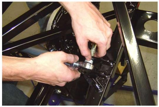
Install the upper link onto the frame, this bolt must be inserted form the inside of the frame going outward. Make sure to use one of the 0.25" spacers (FFR# 33240) on either side of the rod end.
