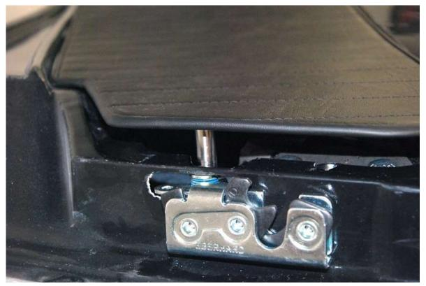
Place the inner door panel on top of the door so that it sits on the door release lever.
