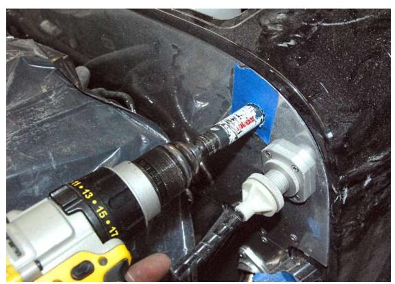
Use a ¾" hole saw for the pin receiver.
