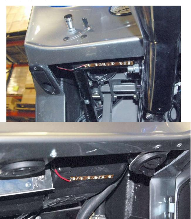
Install the under dash lights on the frame as desired according to the wiring harness instructions.
