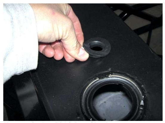
Insert the rubber grommet into the small hole in the top of the tank.
