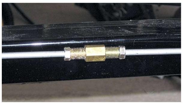
At the end of the 60" brake line piece, install a female-female union and attach a second 60" section of brake line.
