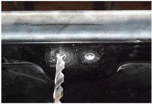
Drill  $\frac{1}{8}$ " holes through the trunk liner and the  $\frac{1}{8}$ " aluminum inside of the trunk then open the holes up with a  $\frac{25}{64}$ " bit and install rivnuts at the points marked.
