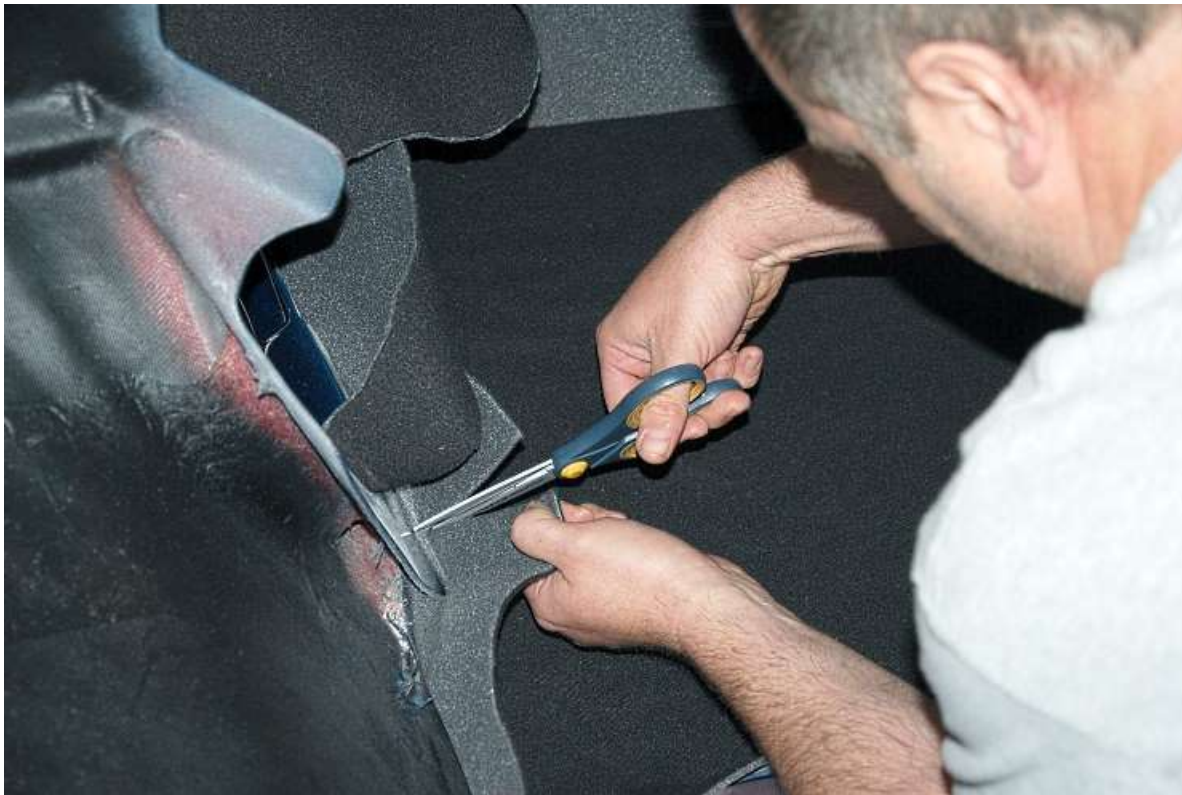
Making pie cuts around the tighter curves helps get the material to lay flat.
