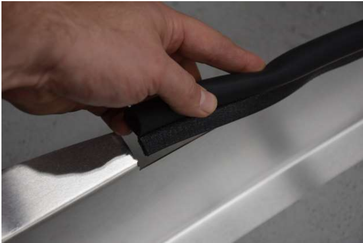
Push weather strip goes across the top of the firewall on either side of the windshield support flange.
