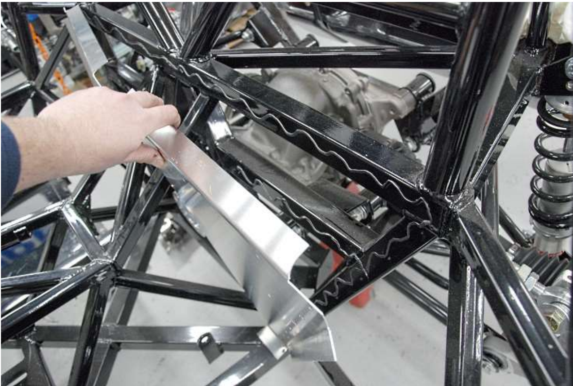
Silicone the rear cockpit wall frame tubes.
