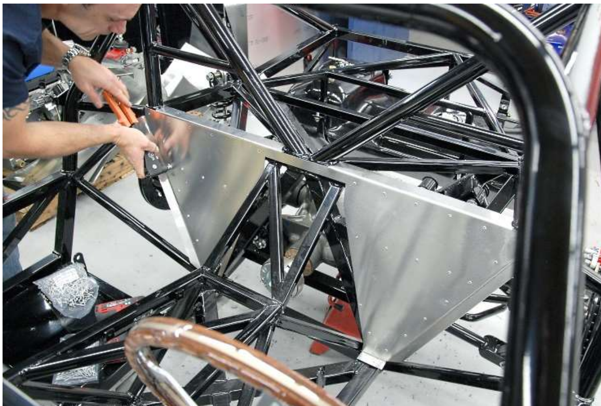
Use the #8 screws to hold the panel in place then drill and rivet the cockpit rear wall to the frame.
