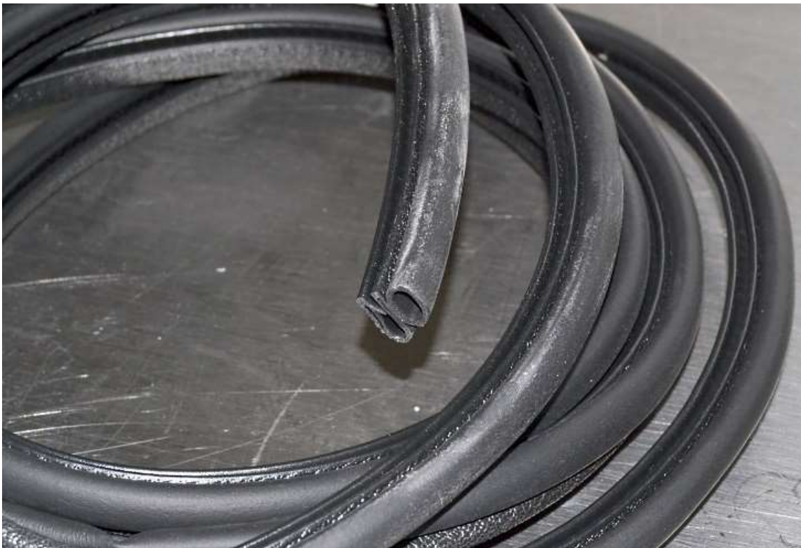
The weather stripping with the bulb is for the side windows, the bulb faces toward the outside of the car.
