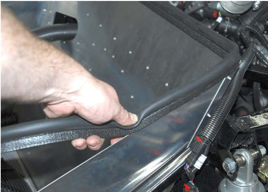
Push weatherstrip around the radiator aluminum.
