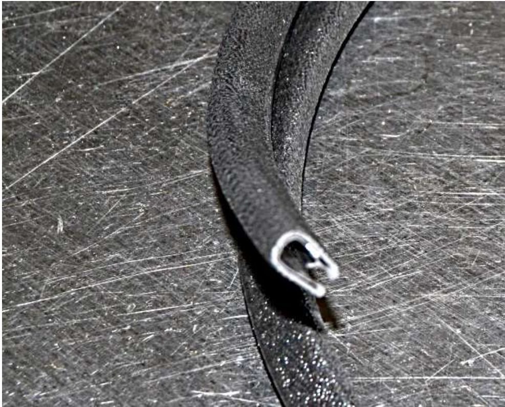
The windshield weather strip without the bulb is for the windshield surround.
