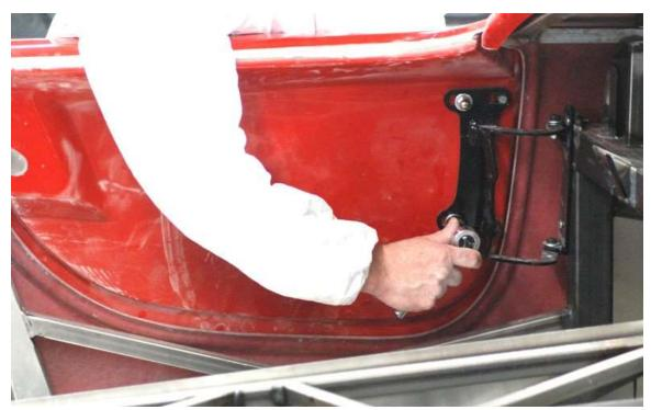
Hold or tape the door in position and attach the hinge to the studs.
