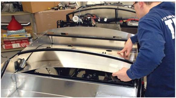
Work the corners of the panel down over the roll bar mounts and seat harness tabs a little at a time on each side.
