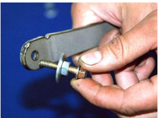
Insert the bolt with the nut and washer through the small hole in the rivnut tool from the side where the handle angles up.
