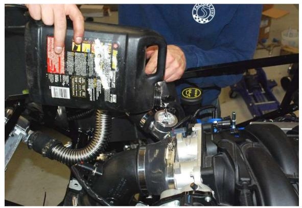
Fill the engine with Oil and coolant. Both these fluids should be rechecked after you have started the engine for the first time. Make sure there is some coolant in the overflow to start out, about 1/3 full is good.
