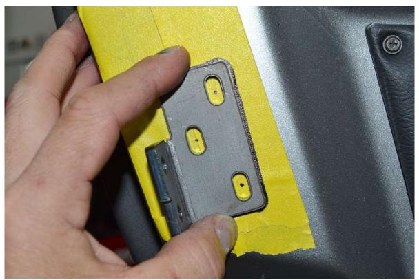
Align latch mount with the marks on the masking tape on the door and mark the center locations of the mounting slots.
