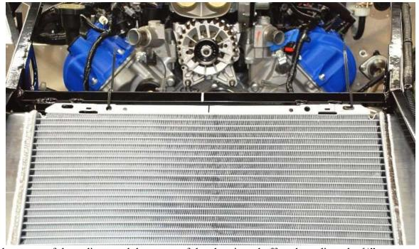
Mark the center of the radiator and the center of the chassis and offset the radiator by 5/8".
