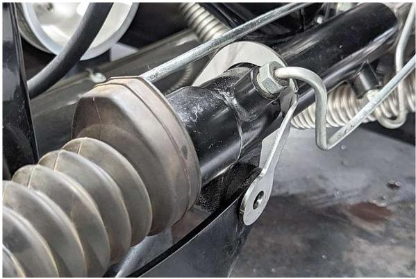
Line up the bracket mounting hole with the frame bolt hole.
