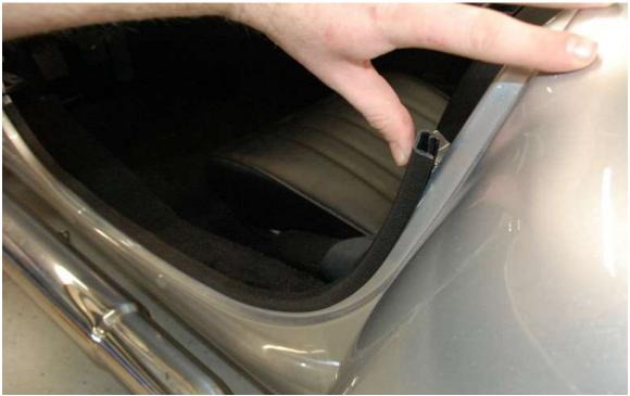
Cut a section of the large C channel weatherstrip to fit from the bottom of the door hinge to the door latch and push it in place over the body, aluminum and carpet to finish the edges off. The barb side goes towards the inside of the car.
