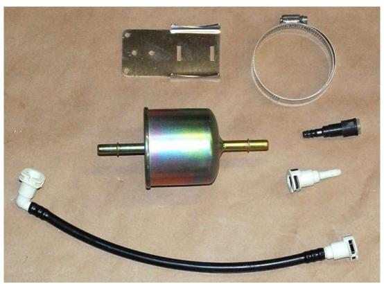
Unpack the fuel filter and mounting hardware.
