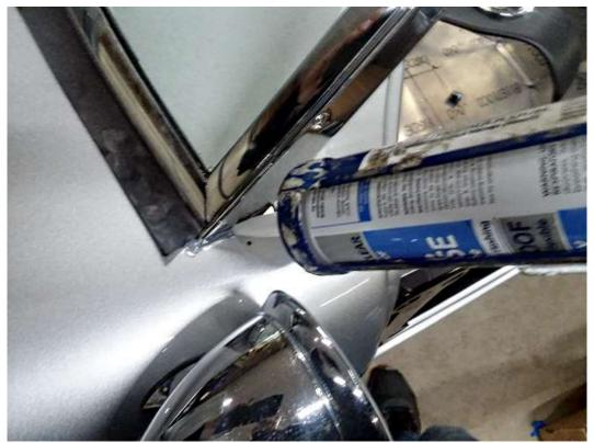
Remove the base plate and silicone in the slot around the windshield.
