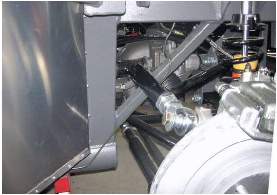
Run the brake line up the 2"x 3" tube and 1" square tube.
