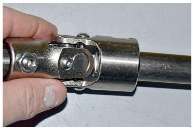
Slide the 1"DD tube into the upper u-joint so that it is flush on the inside of the joint.
