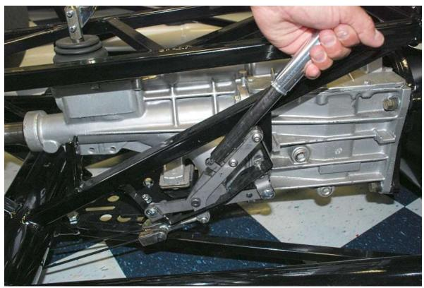
Slowly pull up on the handle to set the brake pads and remove any slack from the brake cables.
