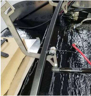
Screw the ball stud into the hinge arms from the outside of the car in then push the body of the gas strut onto the ball stud.
