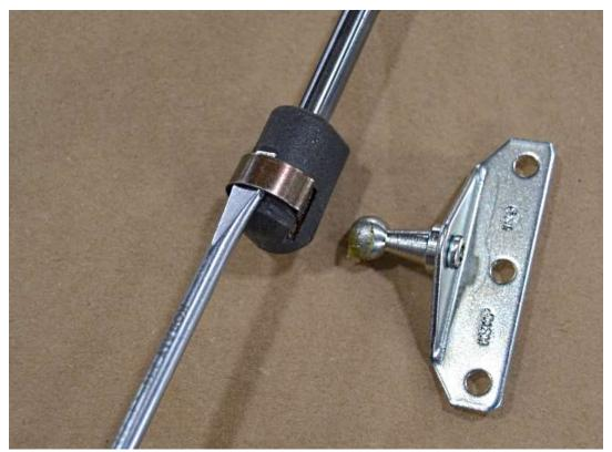
Remove the rod end ball stud bracket use a small flat head screwdriver to pry up on the metal clip holding the stud in.
