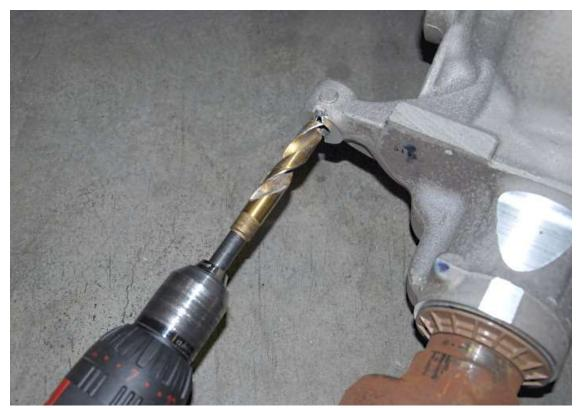
Use a 5/8" drill bit to chase the front mount holes on the center section.
