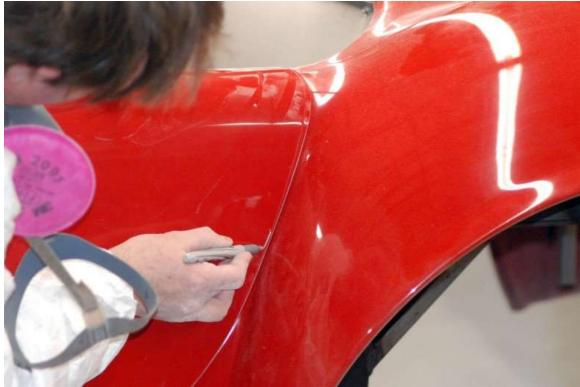
Position the door in the body to see where it may need to be trimmed to fit the opening. Mark the door and only remove enough material to get it to fit.
