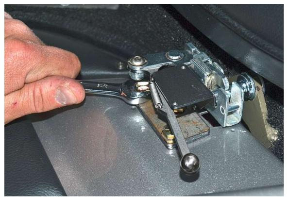
Close the door so the latch engages correctly then tighten the latch base using a 7/16" wrench.
