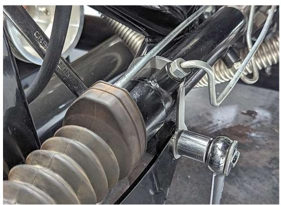
Use a ¾" wrench and ratchet to fully tighten the steering rack.
