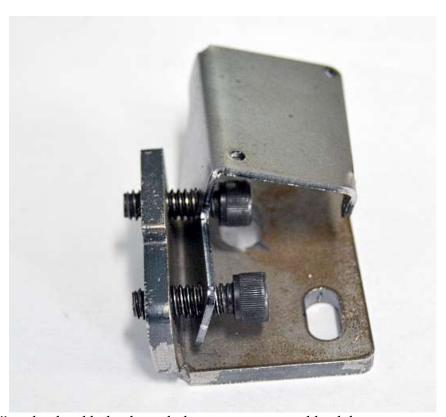
Run the  $\frac{1}{4}$ "x 0.75" socket head bolts through the cover mount and latch base.
