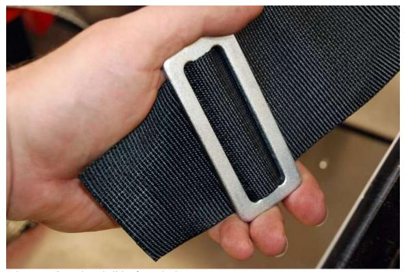
Remove the mounting tab and slider from the harness.
