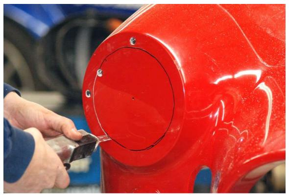
Using a jig saw, cut the inner hole out of the body, use a larger drill bit to make a hole to start your cut.
