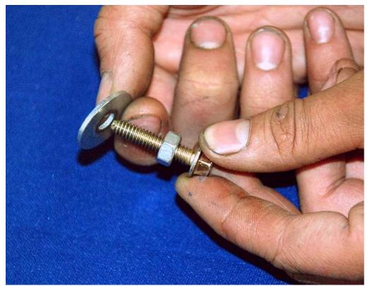
Next slide the 1/4" fender washer onto the bolt down to the nut.
