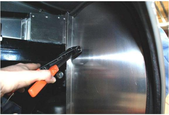
Silicone and rivet the panels in place.
