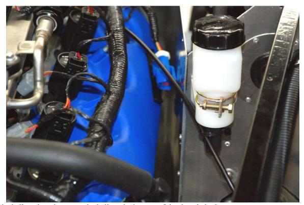
Push the ball stud retainer onto the ball on the bottom of the throttle body.
