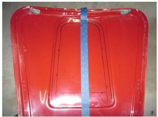
Mark the inner line to make sure the wrong line is not cut.
