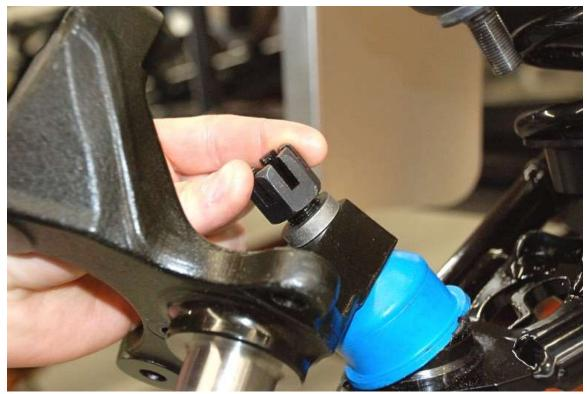
Place the 15803 countersunk spacer under the castle nut to ensure that the cotter pin is at the correct height. There is a small taper on the inside edge of the spacer that should face down toward the spindle.
