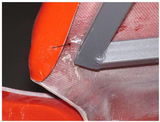
Check the outside corners of the dash tube. Make sure there is a ½" or so gap between the body and frame. Try pushing down on the body here, it should move.
