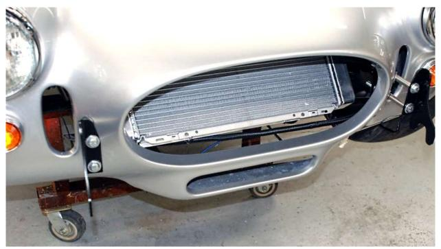
The radiator and its plumbing were installed before the body was mounted. The radiator is being held up at the bottom by a couple of zip ties through a quick jack bumper hole.
