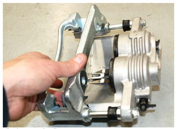
Slide the caliper hanger onto the caliper.
