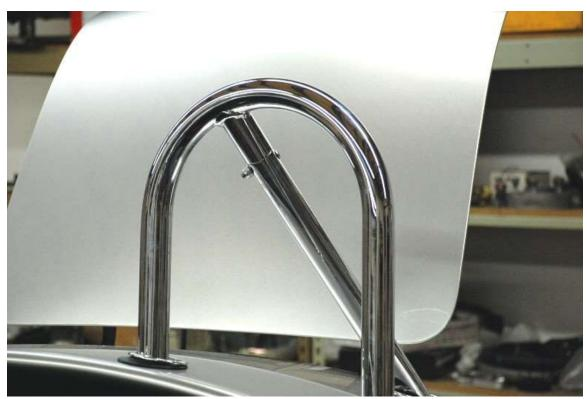
Re-mount the roll bar through the body. Make sure that the rear leg is in the correct orientation so that your holes will line up.
