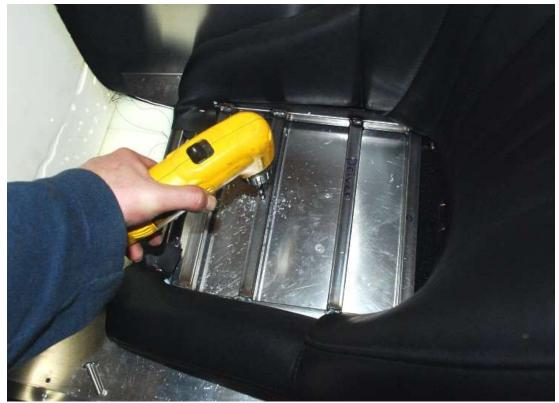
Drill the first hole for the seat mounting and install the bolt.
