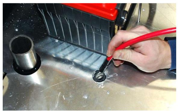
Push the small end of the battery cable through the floor from the top.
