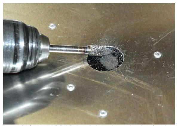
Remove any coating from the small circle in the trunk closer to the ground terminal of your battery.
