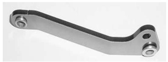
Press the bronze bushings into the holes in the hinge arms as shown. The short hinge arms are both the same. Left side long arm shown.
