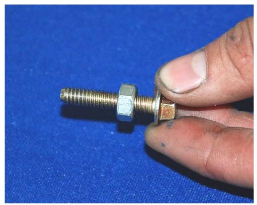
Thread the 1/4" nut about 3/4 of the way onto the 1/4" x 1.25" flanged bolt.
