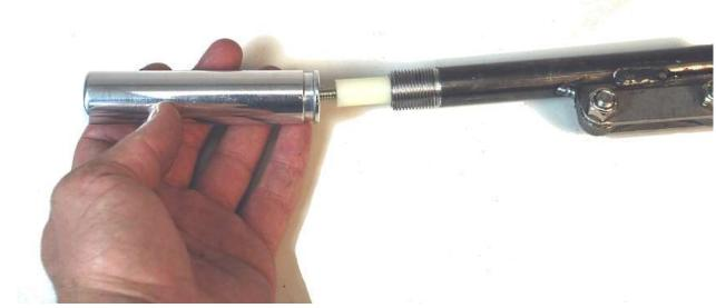
Spray a little WD-40 on the lower handle threads and screw the upper handle onto the lower handle.
