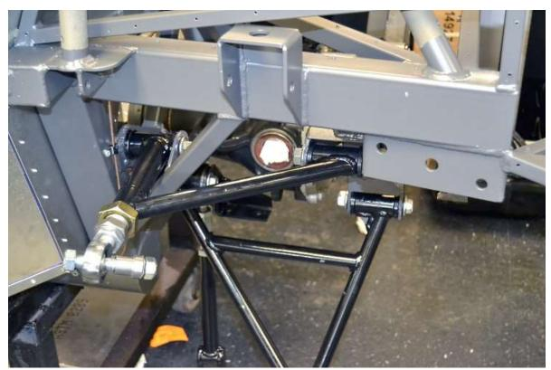
With the grease nipple pointed down, pass the upper control arm thick tube through the triangular area as shown in between the frame mounts. Use the longer M16 x 110mm ( $\sim$ 4<sup>5</sup>/<sub>16</sub>") bolts.
