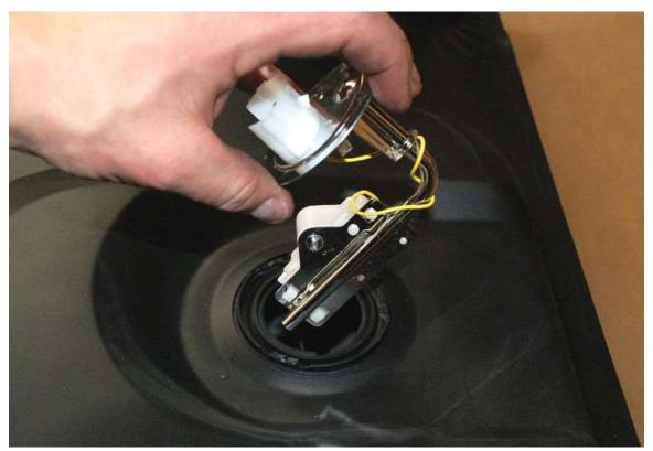
Insert the fuel level sender into the tank.
