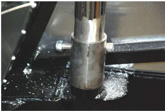
Insert one of the  $\frac{5}{16}$ "x 2" button head socket screws after drilling each hole to ensure that the rollbar does not move.
