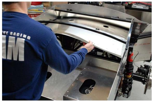
Drill and silicone the upper trunk floor. Bend it in the middle to get it into position.
