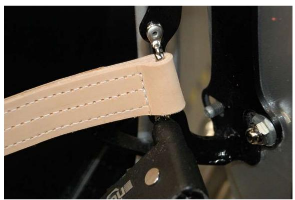
Rivet the check-strap to the door hinge using a <sup>3</sup>/<sub>16</sub>" rivet.
