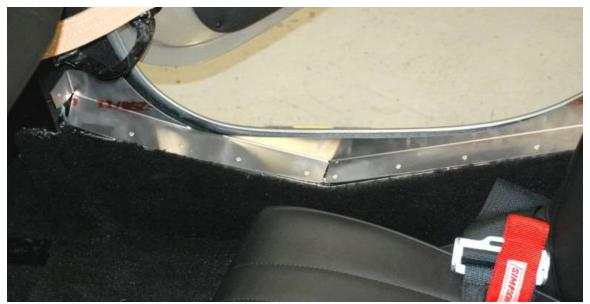
Silicone and rivet the panels in place, it is ok if the flanges do not cover the full width of the chassis tubes. It is more important that the panel is lined up with the body under the door.
