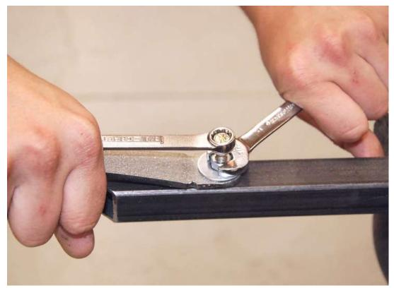
Tighten the clamping nut until the resistance changes as if it were a nut getting tight.
