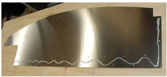
Mark the firewall and drill for riveting.
