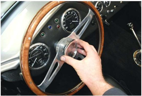
Unwrap the steering wheel center section and push it into the steering wheel and boss, a little WD40 on the O-ring helps if it is tight.
