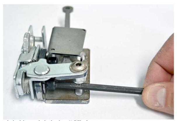
Tighten the latch base to the latch using a  $^{3}/_{16}$ " Hex key.
