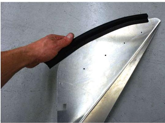
Remove the side panel then measure, mark, drill rivet locations where the ¾" tube is located and press on the bulb weatherstrip.
