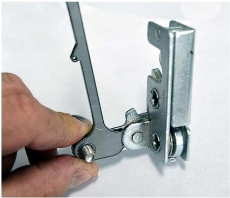
Run the  $\frac{1}{4}$ "x 0.50" Button washer head bolt through the latch lever then the handle followed by a locknut.
