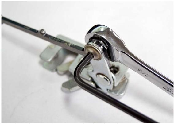
Use a  $\frac{5}{32}$ " Hex key and  $\frac{7}{16}$ " wrench to tighten the handle to the latch.
