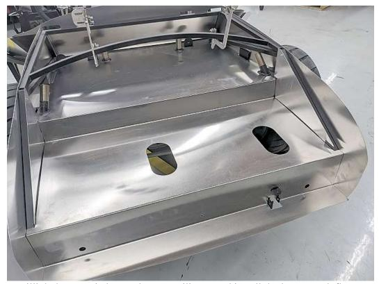
With the rear taillight harness tied up and secure, silicone and install the lower trunk floor.
