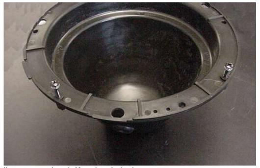
Screw the adjuster screws about halfway into the buckets.
