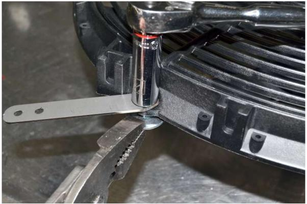
Thread on the lock nut and tighten with a  $\frac{7}{16}$ " deep socket.
