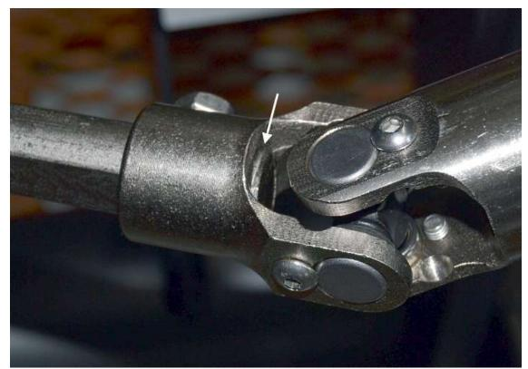
Push the shaft into the steering joint so that it is flush with the inside of the joint as shown above then tighten the set screw and jam nut using a  $\frac{5}{32}$ " Hex key and  $\frac{1}{2}$ " wrench.
