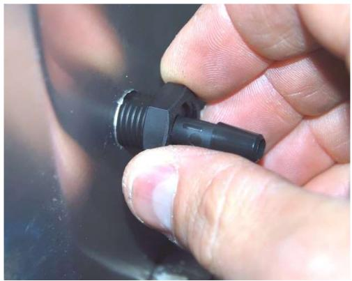
Insert the bulkhead fitting and spin the nut on the backside of the panel. Tighten the fitting using  $^{7}/_{16}$ " and  $^{11}/_{16}$ " wrenches.
