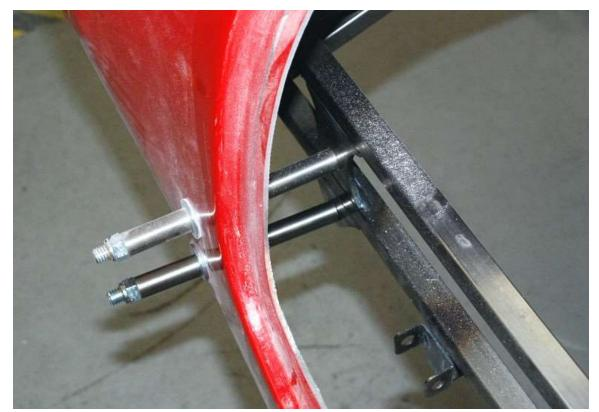
The nut and bolt use a 5/8" wrench and socket to attach the rear quick jack bolts to the frame and body.
