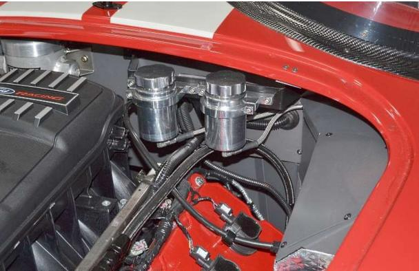
Find a location for the brake reservoir, it can mount to the front of the footbox just inside the hood opening or behind the engine on the firewall but this would require making a bracket. Use the reservoir with cap and locate it so the reservoir cap can be removed and filled with the body on.
