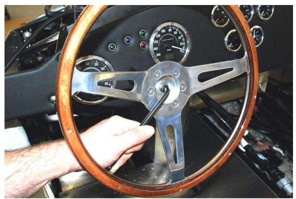
Bolt the steering wheel assembly to the steering shaft using a 3/8"x 1" socket head bolt and washer. Use thread-locker on this bolt.
