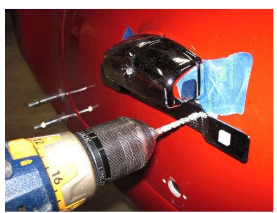
Push the light into the trunk and drill through the license plate mounting holes with a <sup>3</sup>/<sub>16</sub>" drill bit.
