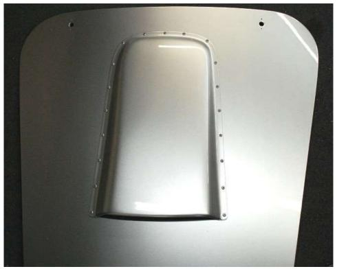
Rivet the scoop back in position on the hood.
