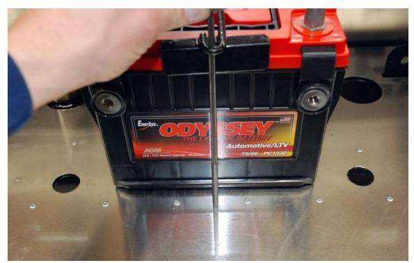
Drop the J-bolts in the mounting holes and mark where they hit the trunk floor.
