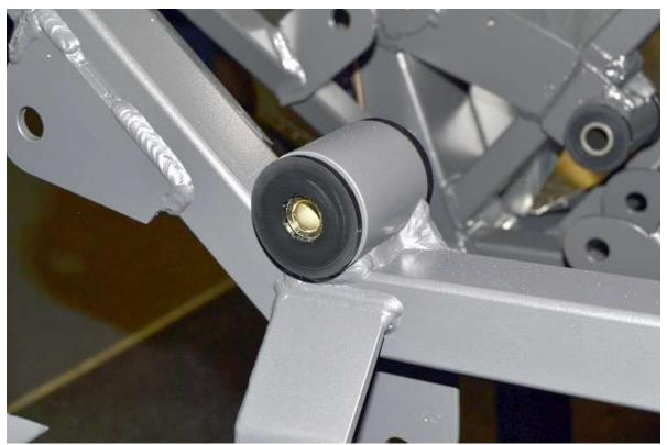
Use a plastic mallet to install the polyurethane bushings marked 2123 and the shorter (2.40") sleeves where the rear of the center section will mount.
