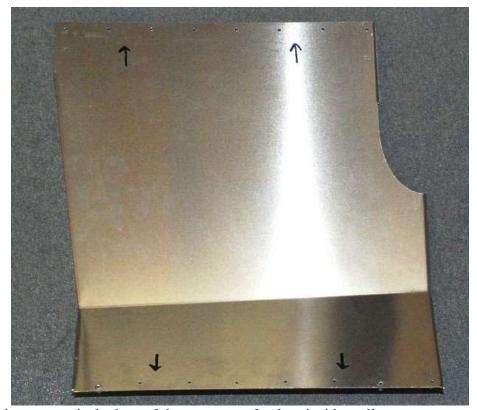
Mark and drill the two vertical edges of the passenger footbox inside wall.
