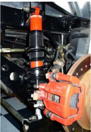
Run zip ties through the holes in the spring hat and around the spring to prevent the spring from becoming unseated.
