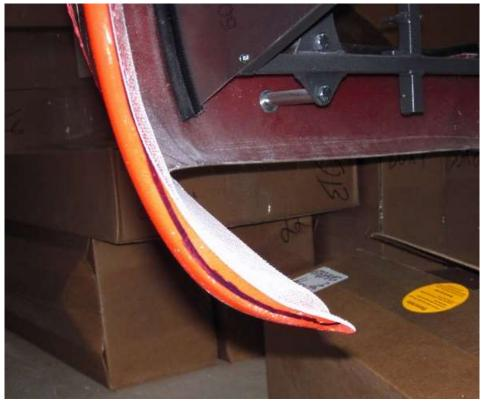
The curled under side body edges are not as visible but just taking a little time here to get the lines straight and a small radius makes for a much nicer finish as well.
