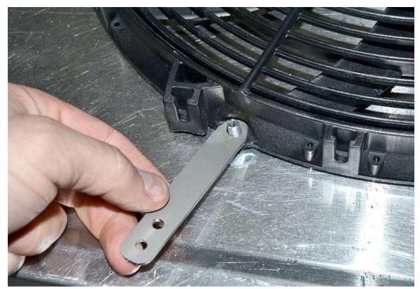
Put the fan mounting strap on top of the fan using the larger single hole at the end.
