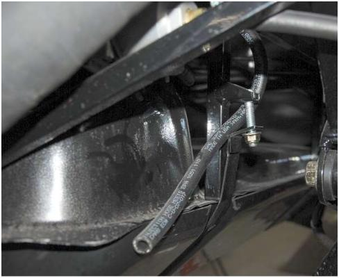
Run the vent hose down to the 3/4" tube near the battery and attach it to the tube using a zip tie.
