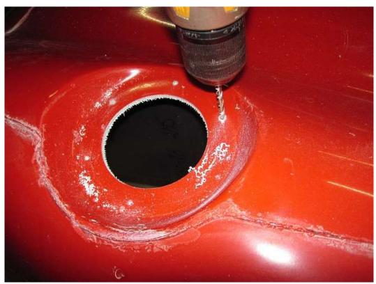
For one of the holes on the inside of the body Use a  $\frac{7}{32}$ " bit drill for the grounding strap bolt.
