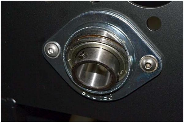
Attach the flange bearing to the front of the footbox with the set screw flange in the engine bay as shown using  $\frac{5}{16}$ " x 1" button head screws,  $\frac{3}{16}$ " hex key and  $\frac{1}{2}$ " wrench.
