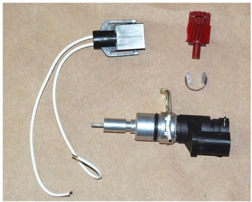
Unpack the speedometer sending unit components.
