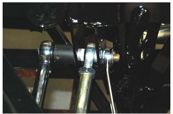
Jack the rear axle up and attach the upper link to the frame using a 12382 5/8"x 3" hex head bolt and 15216 mechanical locknut.
