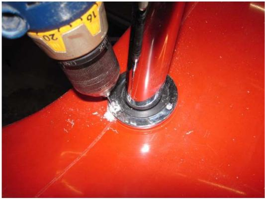
Locate and drill the front grommet holes.
