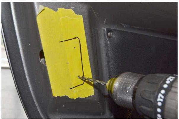
Starting with a <sup>3</sup>/<sub>16</sub>" drill bit then opening it up to <sup>25</sup>/<sub>64</sub>", drill a hole where you want to install the rivnut.
