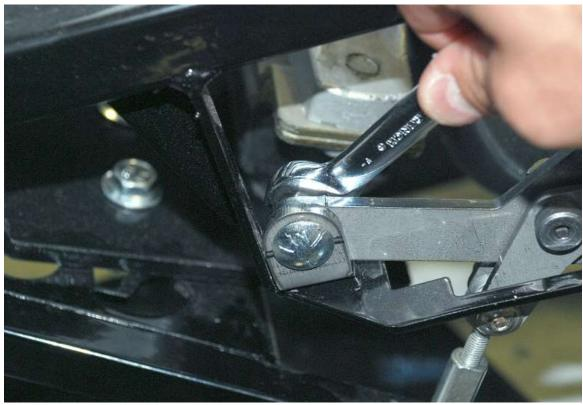
Tighten the mount bracket to fixed gear carriage bolts.
