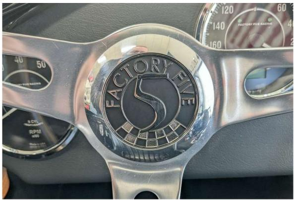
Peel the backing off the badge and stick it in the center section making sure you are aligned with the top of the steering wheel. If necessary, file any flashing off the bottom edge of the emblem so that it will fit.
