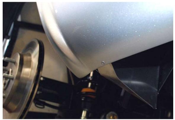
Use a long 1/8" rivet as low as possible to attach the tab to the lower fender.
