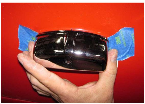
Remove the license plate light cover and use it to double check the template location.
