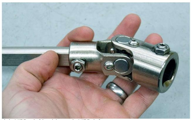
Push the 3/4"DD end of the u-joint onto the 3/4"DD shaft.
