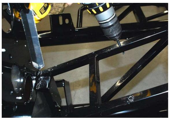
Loosen the bolts and remove the pedal box assembly from the footbox then use a ½" drill bit and drill to drill through the ¾" tubes at the locations marked for the rear mount.
