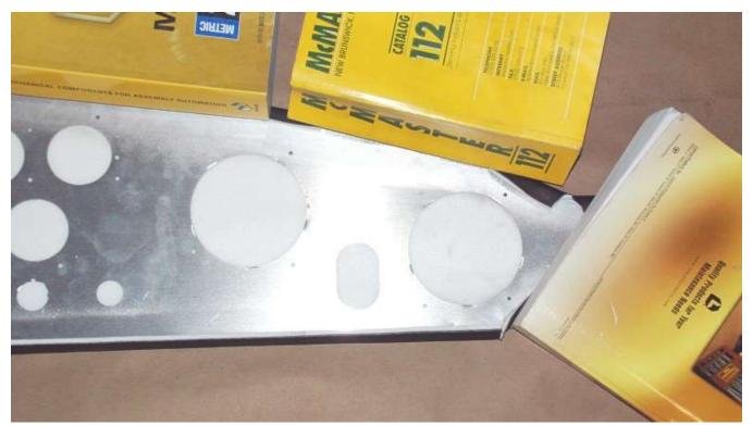
Wrap the dash pad around to the back and glue it. Use some heavy books to hold the pad in place until the adhesive has a chance to dry.
