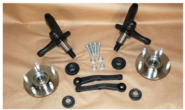
Unpack and lay out the hardware for the spindle's assembly.
