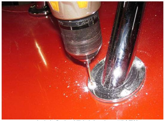
Locate the rear grommet so that it sits flat then drill the holes using an 1/8" drill bit.
