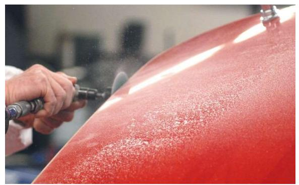
Sand, grind or cut the panel back so the marker line cannot be seen. Remount the panel and the resulting gap should be the same around the whole panel, about  $\frac{3}{16}$ ".
