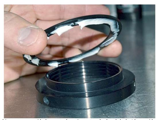
Put the Delrin spacer grease side down onto the spring seat on the threaded tube (shown without tube)
