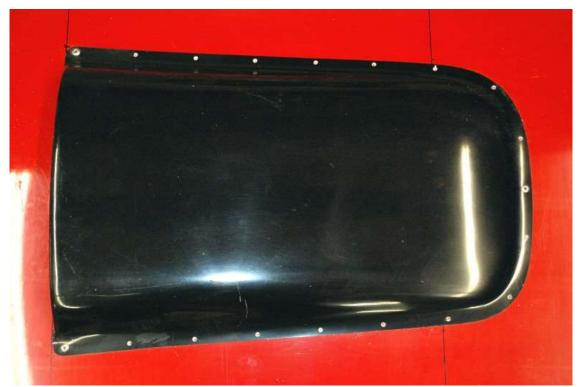
Drill two of the rivet holes on opposite sides of the scoop and the back-center rivet hole using an 1/8" drill bit. After drilling each hole place a rivet in the hole so that the scoop does not move.
