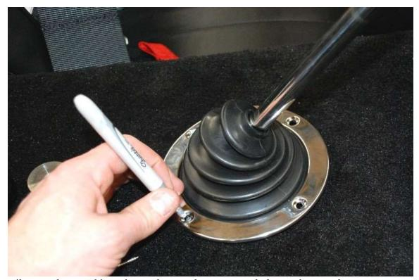
Using a silver marker or white paint marker, mark your screw holes on the tunnel.
