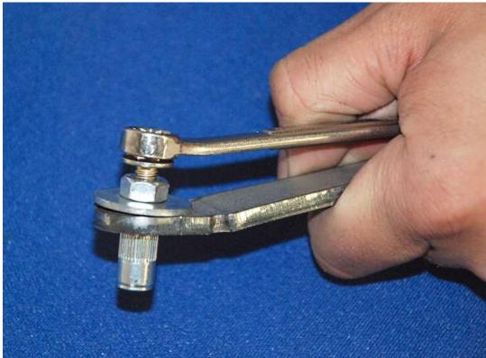
Using a <sup>3</sup>/<sub>8</sub>" closed end wrench hold the bolt from turning by clamping the wrench and the install tool in one hand.
