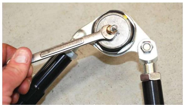
Screw the grease fittings in to the ball joints and tighten with a 3/8" wrench.
