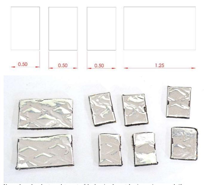
Use a ruler and marker to mark two sets of the damping then cut the pieces using a razor knife.
