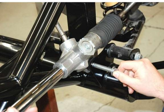
Bolt the rack into the frame using the ½"x 4" bolts. It is easier to do the driver side first then swing the passenger side down into the mount.
