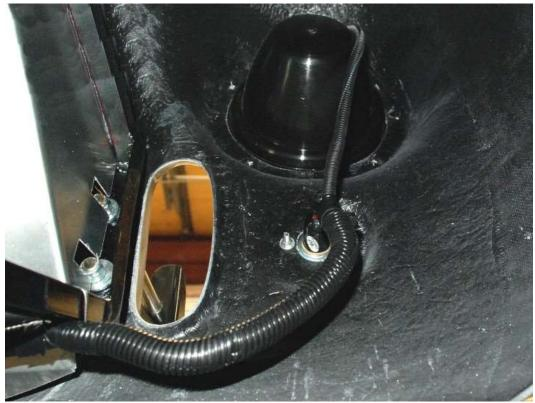
Wire in the headlights to the chassis harness. On the headlight, there are three wires, black is ground, white is high beam and the red is low beam.
