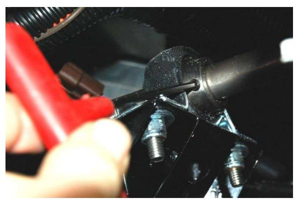
Tighten the set screws on the bearings using an 1/8" Hex key.
