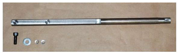
Unpack the upper steering shaft from the primary chassis components box.
