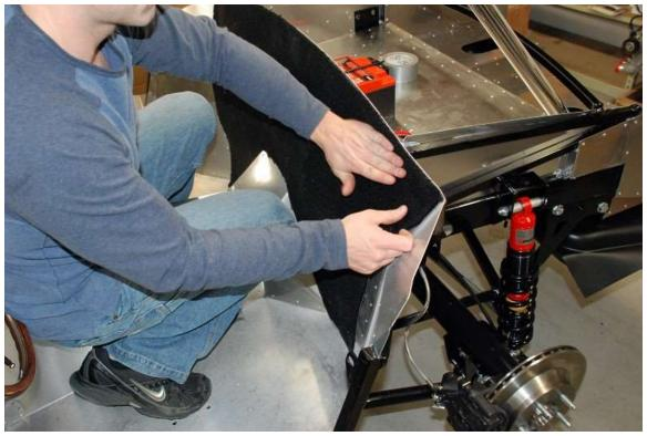
Start with the large rear cockpit wall of carpet. Position it before gluing so you understand where it will go then, apply the adhesive and glue it into position.
