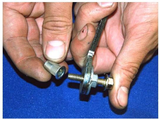
Thread the rivnut onto the bolt until it is snug against the tool. The bolt threads should just stick out of the bottom end of the rivnut. Adjust the bolt depth if needed.
