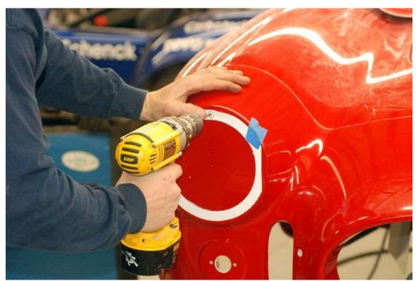
Drill the two smaller corner holes with a 1/4" drill bit to mark their location. Follow this with a 3/8" drill bit.
