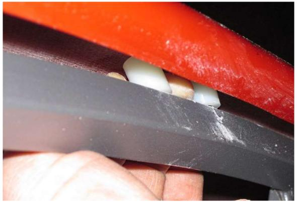
Put the plastic spacers between the dash tube and the body so the screws can go through them.
