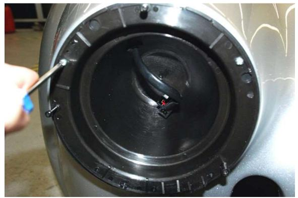
Screw the bucket to the body using the screw that came in the mounting assembly.
