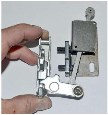
Pass the handle under the cover mount and line up the threaded holes in the latch.
