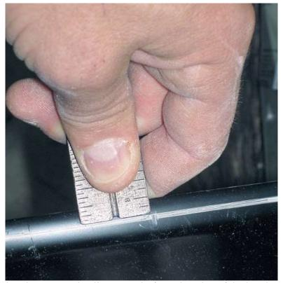
On the top side of the hood scoop mark a line 0.25" in from the edge of the hood scoop flange all the way around the scoop.
