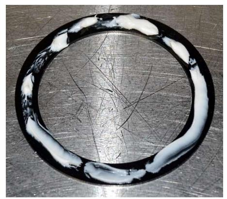
Place a small amount of white lithium or chassis grease on one side of the Delrin washer.
