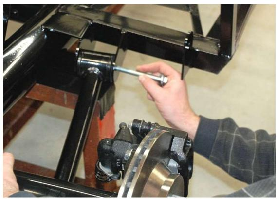
Attach the lower control arms to the frame mounts using the 13706 M12 x 110mm bolts.
