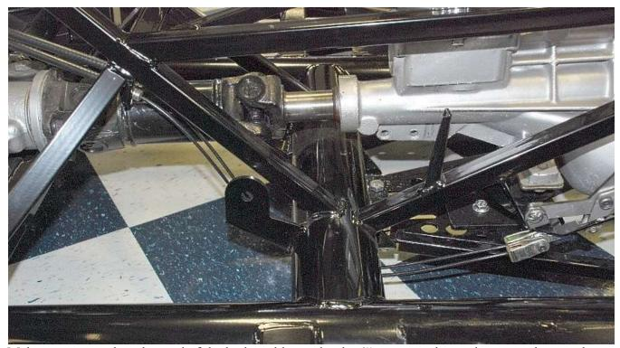
Make sure to run the other end of the brake cables under the 4" crossmember and connect them to the ebrake handle and adjust.
