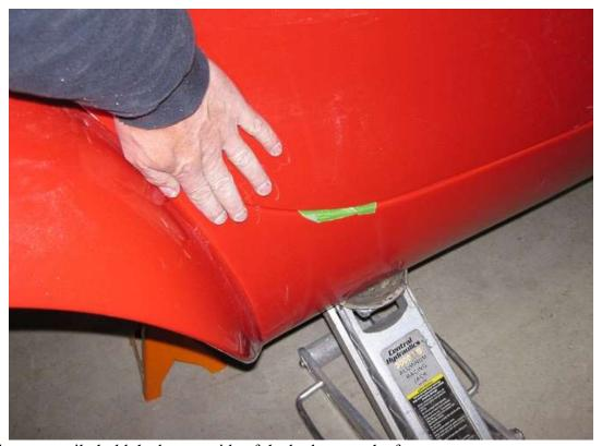
Use a jack temporarily hold the bottom side of the body up to the frame.
