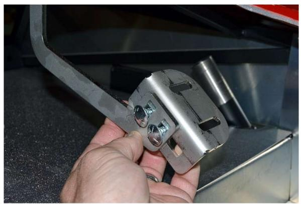
Use the carriage bolts and  $\frac{5}{16}$ " locknuts to bolt the mounting pads to the arms leaving them just snug so they can be moved without loosening the bolts.
