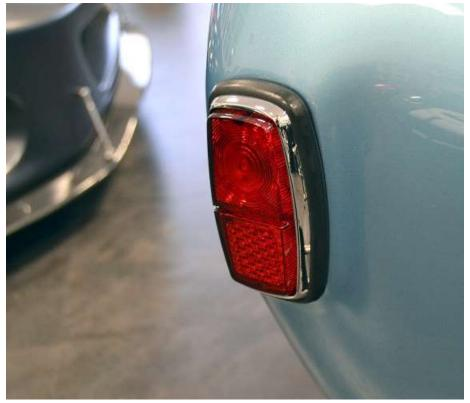
Use one of the black tail light mounting gaskets as a guide to locate the taillight on the body.
