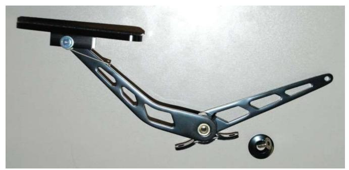
Roughly adjust the pedal as shown and reinstall the washer and screw. The pedal will get adjusted later after install.
