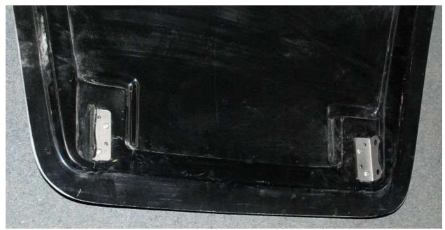
The hood hinge pivot mounts attach to the hood using rivets, the holes are predrilled in the hood liner but you may need to clean them out with a  $\frac{3}{16}$ " drill bit. This is the initial install so you only need a few rivets if you are going to remove the hinge brackets prior to body painting (recommended).
