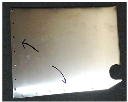
Mark the holes in the passenger footbox front panel upper and outer edges but do not drill yet.
