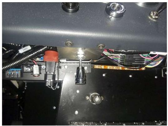
The panel with the key hole can be used to mount the headlight switch if desired. If using the panel for the switch, locate it so it can be reached by the driver.
