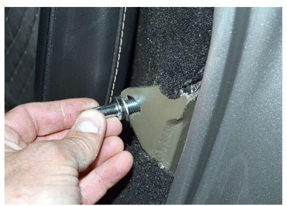
Put a  $\frac{3}{8}$ " washer on the striker then pass the striker through the mount on the frame next to the seat followed by a  $\frac{3}{8}$ " nylon locknut.
