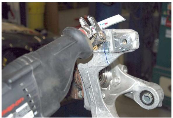
Use a saw to cut the ear off the spindle. If using a Sawzall or similar, use a wood blade; a 14tpi blade or finer will just get gummed up with the aluminum.
