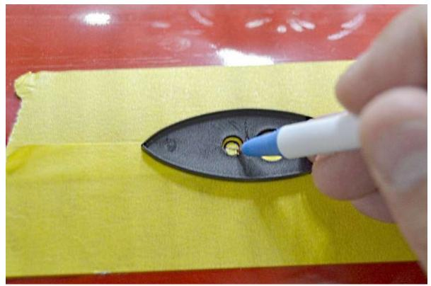
Hold the gasket in place, remove the mirror and mark the location of the mounting holes.
