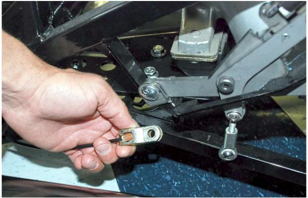
Remove the cable clevises from the rod end and attach them to the cable ends.
