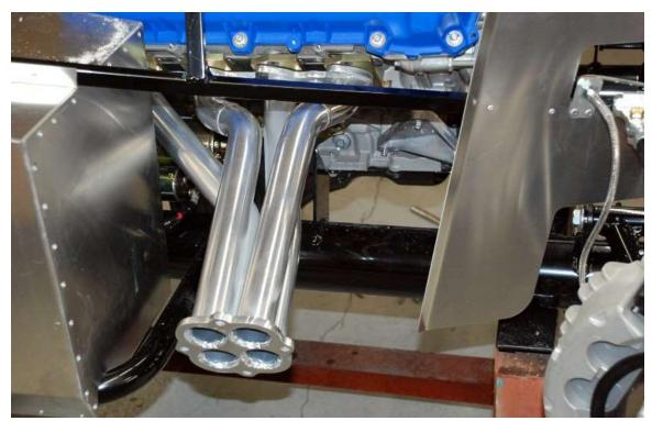
Mount up your headers to the engine. If you are using full length headers they bolt in place with the gaskets and hardware provided. Thread locker is recommended.
