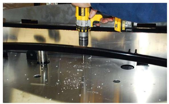
Drill the 1/4" mounting holes in the floor.
