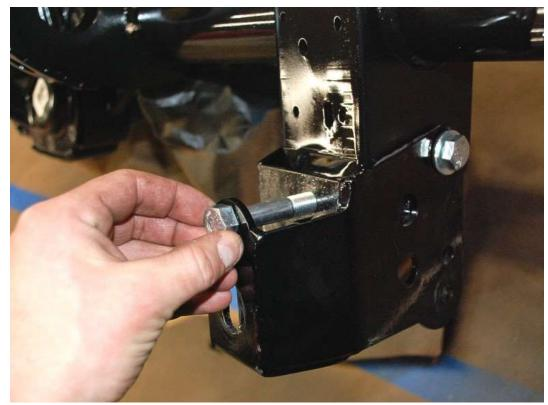
Temporarily put the lower shock bolt (½"x 3" bolt) through the traction lock bracket and stock shock hole on the axle.
