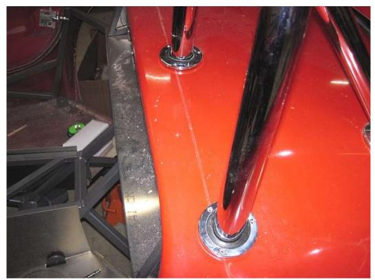
If using rollbar grommets, put the front rings and grommets onto the rollbar hoop then put the hoop through the body and on to the frame.
