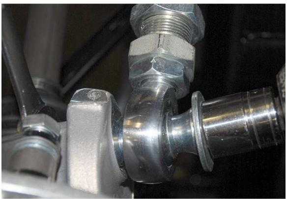
Use a <sup>15</sup>/<sub>16</sub>" wrench, <sup>15</sup>/<sub>16</sub>" socket and ratchet to tighten the locknut.
