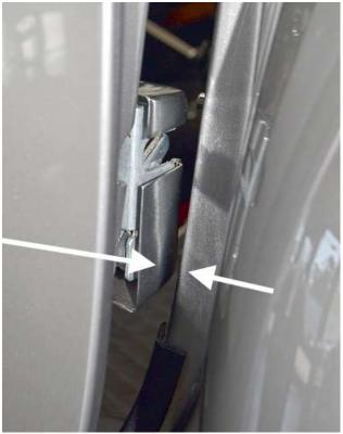
Hold the latch assembly up to the location on the door and check clearance between the latch cover and door opening while closing the door.
