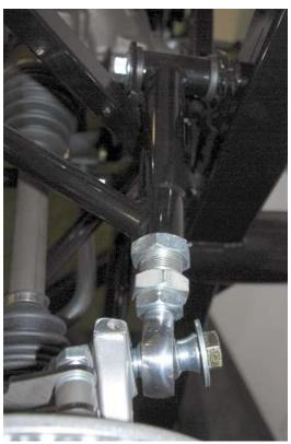
Check the angle of the upper control arm rod end, make sure that the rod end is not touching the spindle and that it is aligned with the upper control arm.
