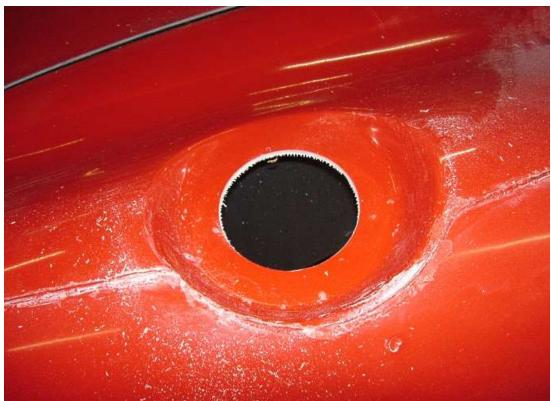
Use a 3½" hole saw for the center opening. If you do not have a hole saw this size, you can cut the center circle out of the template and use the remaining template to mark for a jig-saw instead.
