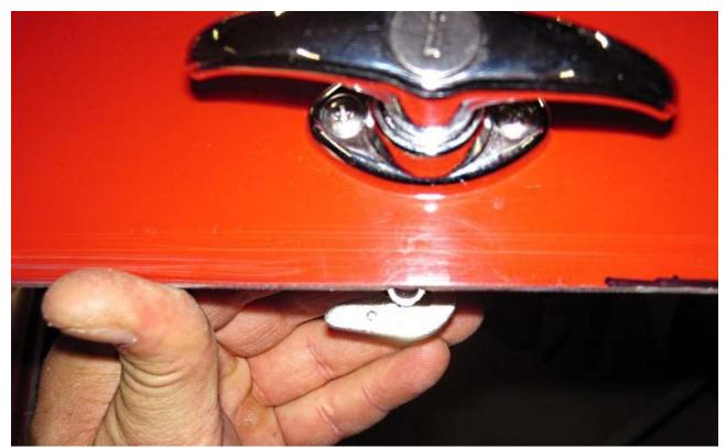
Use the latch sleeve on the latch to see the center height of the latch sleeve compared to the edge. Make sure the sleeve is 90 degrees to the latch. In the picture this is just above the edge but this is dependent on the gap around the trunk that you make.
