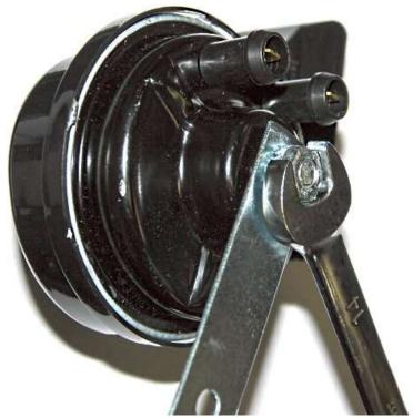
Attach one horn to the included bracket using one of the 14mm lock washers and nuts included. Note the orientation of the wire connectors when tightening the bracket so that it will be correct when installed. The flat horn outlet is pointed right.
