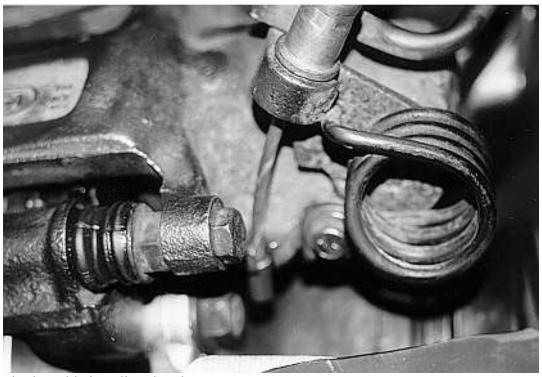
Emergency brake cable in caliper bracket.
