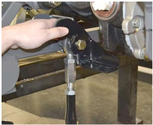
Attach the toe arms to the frame below the front lower arm mount using the 1/8" thick spacer in the back and the 1/4" spacer on the front side of the rod end. Use the 5/8" x 2.25" bolts to attach them to the frame.
