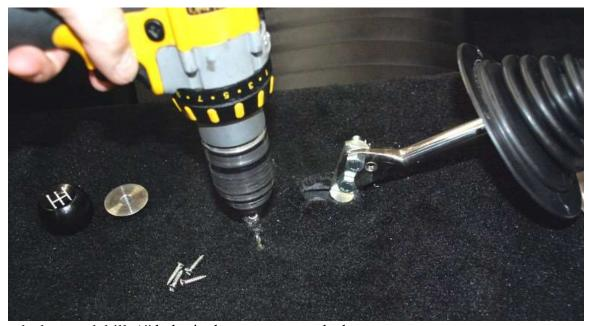
Remove the boot and drill 1/8" holes in the spots you marked.
