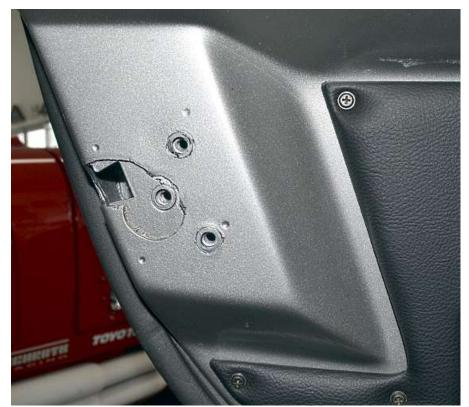
Look at the holes and area drilled. If there is 1/8" in total thickness or less including the fiberglass and steel use the **shorter** rivnuts. If the thickness is greater, use the longer rivnuts. Install the three rivnuts on the door.
