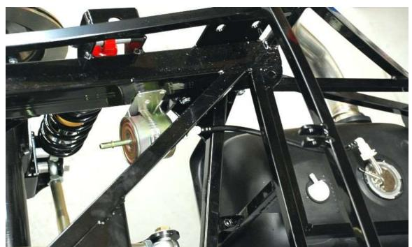
Hold the filter up to the 2"x 3" chassis tube, mark the holes, then drill and rivet the bracket on using <sup>3</sup>/<sub>16</sub>" rivets.
