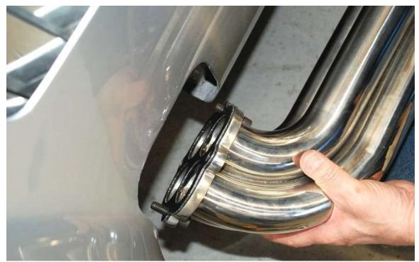
Bolt the pipe and gasket to the header or J-pipe flange with using the 3/8"x 1.25" socket head bolts and mechanical locknuts.
