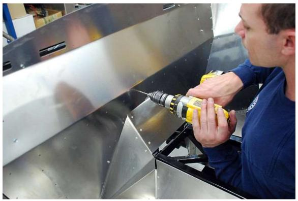
Mark and drill the rear cockpit wall. Silicone the chassis and aluminum flanges where it attaches and rivet it into place.
