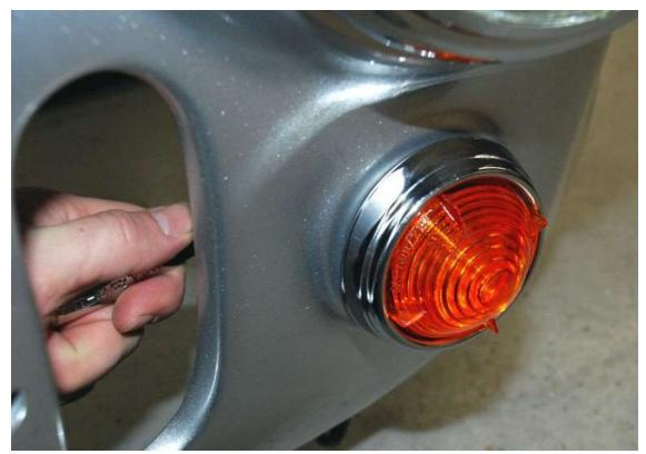
Mount the turn signals to the body being careful not to over tighten the locknuts.
