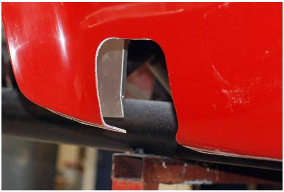
Using a jig saw cut the remaining straight sections and radius on the lower rear corner.
