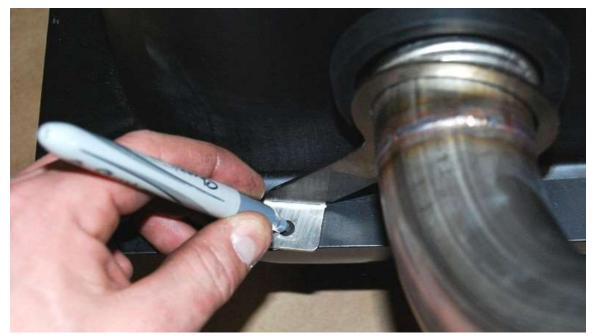
Slide the retaining bracket down the filler tube and mark its mounting location on the tank.
