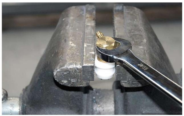
Screw the vent into the plastic bushing and tighten with a  $\frac{7}{8}$  wrench.
