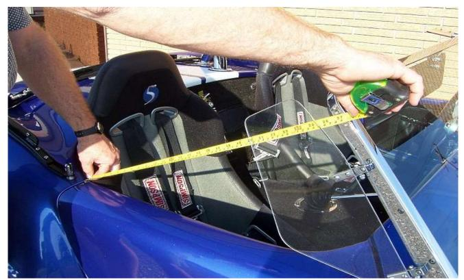
Measure from the middle of the top windshield screw to the inside corner of the rear door, this should be set at 27.00". If necessary slot the holes more so that the angle can get set and there is no side loads on the windshield frame.
