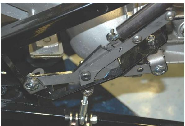
Attach the handle to the frame using the <sup>5</sup>/<sub>16</sub>" carriage bolts. Leave the locknuts loose enough so that the mount bracket can still slide on the frame mount. The front mount bracket goes under the frame bracket while the rear goes on top. The fixed gear straddles the frame mount.
