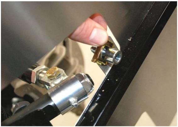
Push the brake line adapters through the brackets from the outside in and install the clips that hold them in place.
