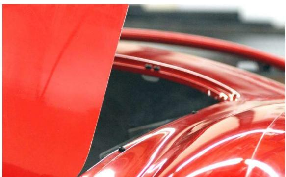
Put the small bumpers around the edge of the hood opening and try closing the hood. If it is too low try the large bumpers.
