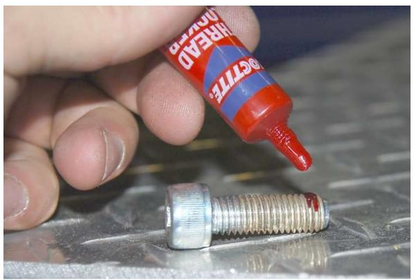
Apply Loctite to the (6) M10 x 25mm socket head screws.
