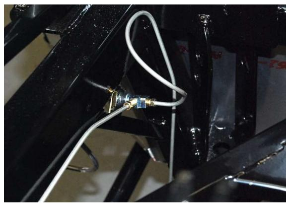
Attach the "T" adapter to the flexible brake line and route the hard brake line coming from the front to the "T".
