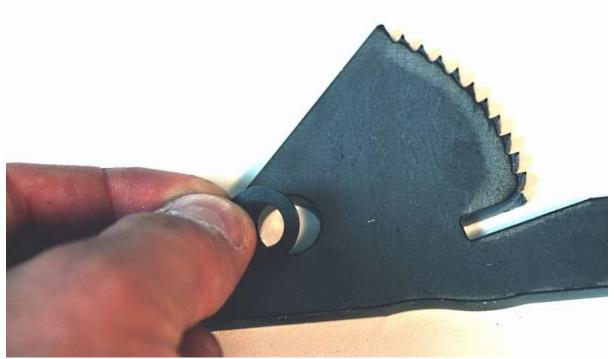
Push a nylon bushing into one side of the fixed gear.
