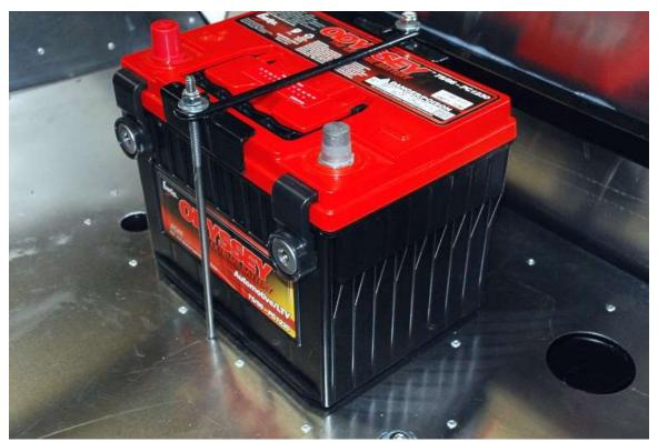
Hook the j-bolts through the floor and bolt the battery down. Hold the j-bolts with a vice grip and be careful not to over tighten and crack or distort the battery.
