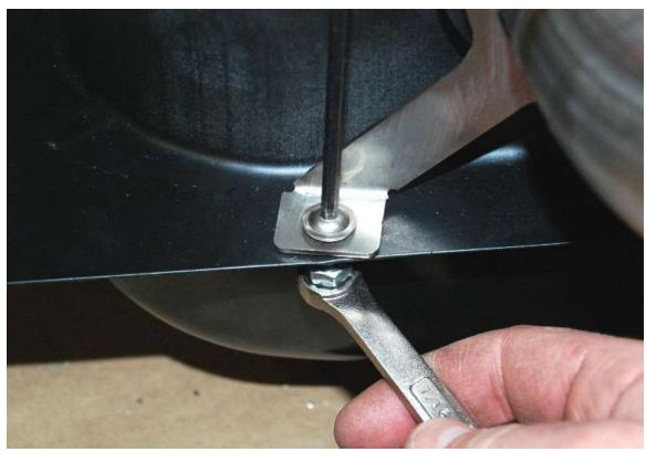
Use the 1/4" bolt and locknut to attach the retainer to the tank.
