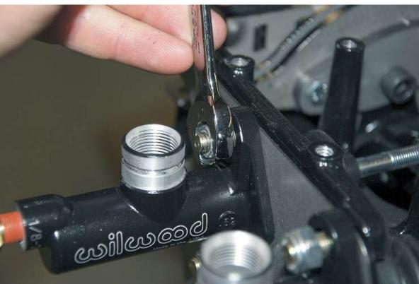
Attach and tighten the locknuts using a ½" wrench and ½" deep socket holding the master cylinder to the pedal box then repeat for the other master cylinder.
