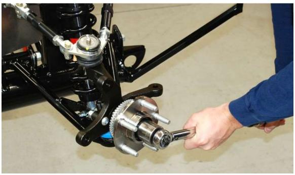
The hub is a snug fit on the spindle and may require a light tap with a soft mallet to get in place. Torque the hub nut to 305-338Nm (225-250 lb-ft).
