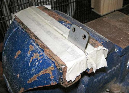
The flexible brake line mount can be on the 1" square tube but the mount may need to be bent so the T clears on the inside.
