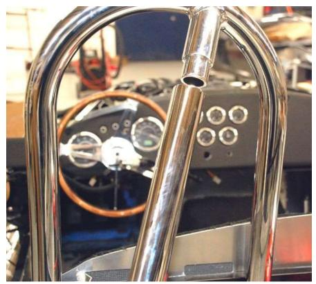
Slide the main hoop into the chassis mounts and wiggle or tap with a soft mallet until it lines up with the rear leg.
