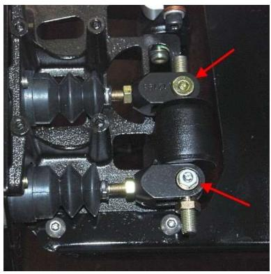
The brake pedal master cylinder pushrod mounts are different from each other. Only one has a screw and nut. This is normal.
