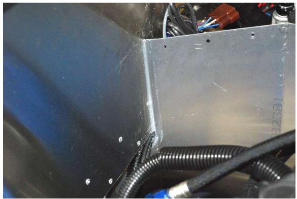
Rivet the remaining inner cockpit wall flange to the firewall.
