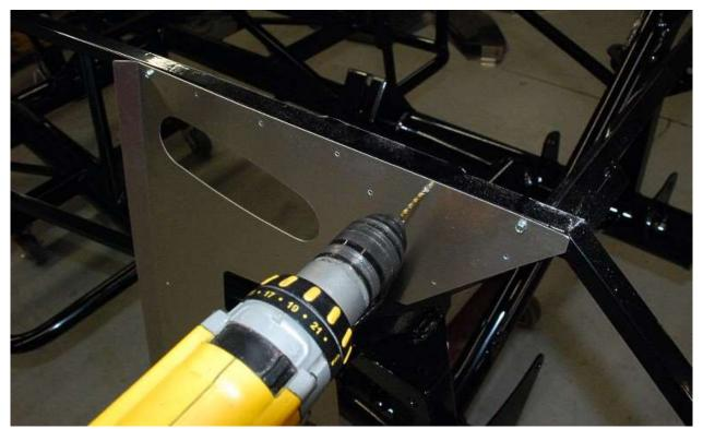
Use the original #6 screws to remount the panel then drill the 1/8" rivet holes through the panel holes into the chassis.
