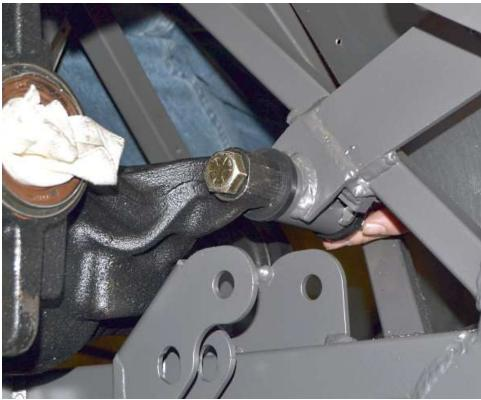
The larger/longer 15963 M16 x 130 bolts and 14515 flanged nuts are used for the front mounts.
