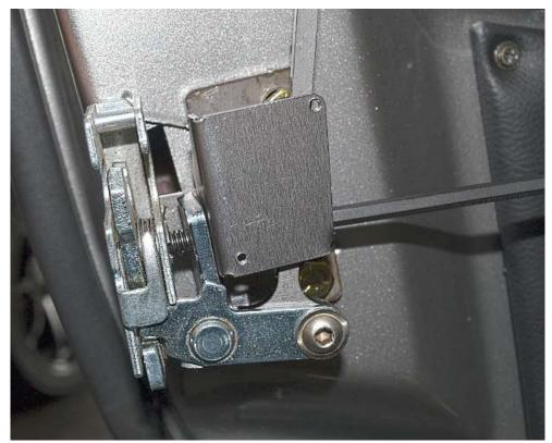
Reattach the cover mount and latch to the latch base using the socket head bolts and 3/16" hex key.
