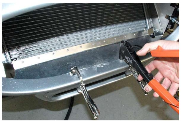
Silicone and rivet the aluminum to the nose lip using three <sup>3</sup>/<sub>16</sub>" rivets.
