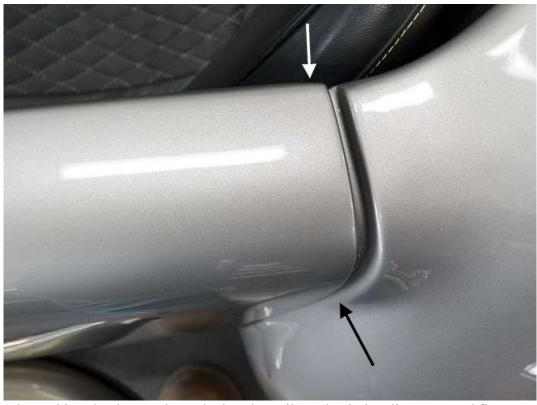
With the latch touching the door and attached to the striker, check the alignment and fitment of the door to the body.
