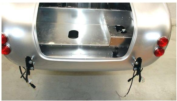
Re-mount the body in the rear with the quick jacks.
