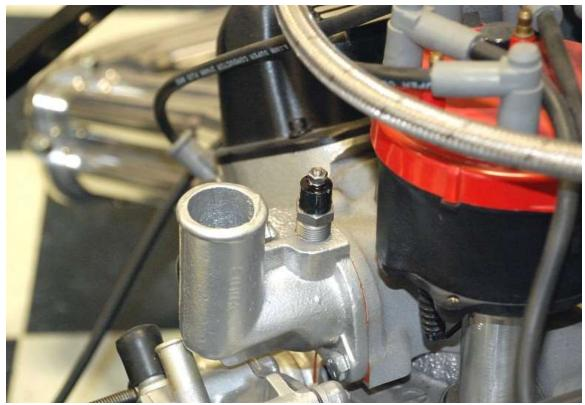
In your engine block or cylinder head, locate a coolant access point to install the thermostat switch and screw it in.
