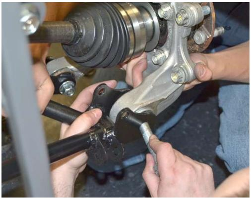
Connect the bottom of the spindle to the lower control arm using the M16 x 90mm bolts and locknuts. Right side shown.
