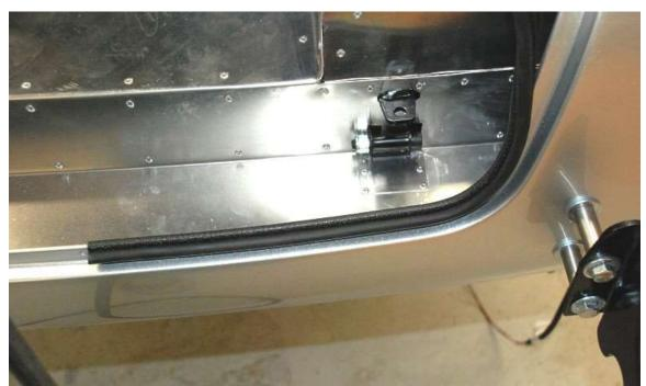
Push the side mount weatherstrip on the trunk opening starting at the bottom next to the latch pin hole and working all the way around just leaving a small gap for the head of the latch pin bolt.
