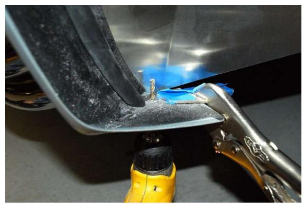
Use one of the <sup>3</sup>/<sub>16</sub>" rivets to attach to the bottom of the fender just forward of the exhaust cut-out.
