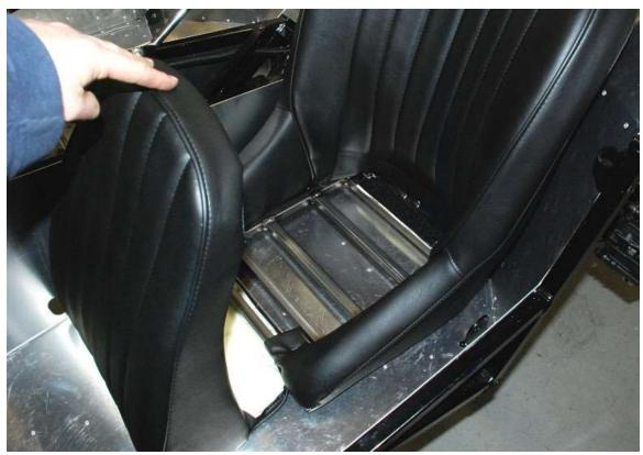
Lift up the bottom of the cushion to reveal the seat frame.
