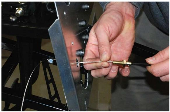
Route the cable through the hole in the firewall and slide the sheath back over the cable.
