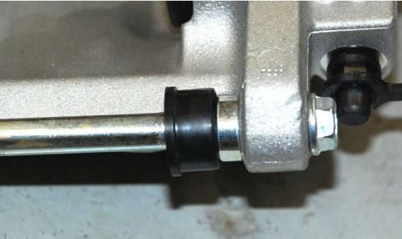
Install the slider grease boots on the slider pins.
