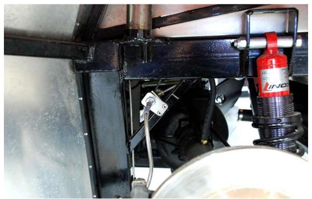
Using the FFR rear brakes, we attached the flexible brake line mount to the driver side diagonal 3/4" tube with the brake line clip.
