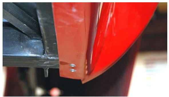
Once the body is painted and final mounted rivet the bottom lip of the body to the chassis using the long  $\frac{3}{16}$ " rivets.
