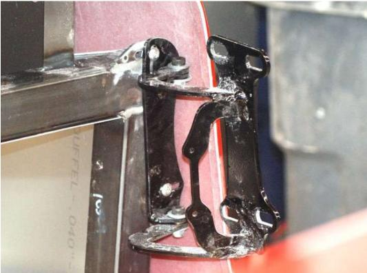
If you have removed them, remount the door hinges on the chassis. The square nuts sit alongside the tube so only one hex wrench is needed for adjustment.
