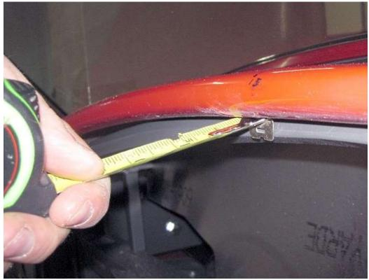
Use a tape measure to measure in from the body lip to roughly the center of the dash tube.
