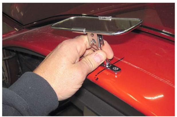
Line up the rearview mirror with the center mark and mark the holes in the body.
