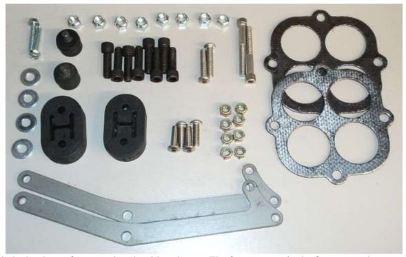
Unpack the hardware for mounting the side exhaust. The fasteners are in the fastener pack.
