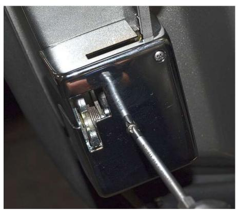
Attach the cover to the latch using a Philips heads screwdriver and the #4 x 0.188" oval head screws.
