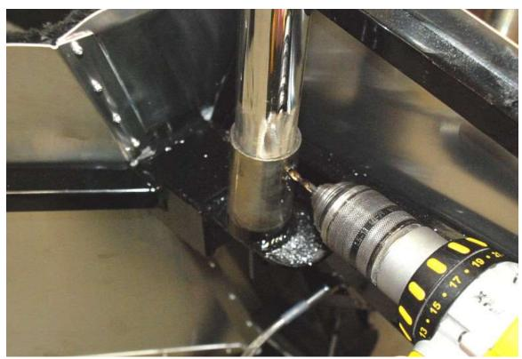
Drill a hole all the way through each of the lower mounts and rollbar main hoop.
