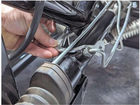
As the bracket goes forward, rotate it to go under the hydraulic line.
