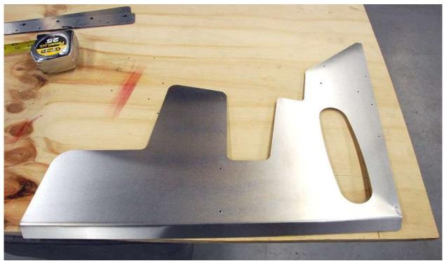
Drill the panels using a 1/8" bit then clean the marker lines and labeling off using acetone or brake cleaner.
