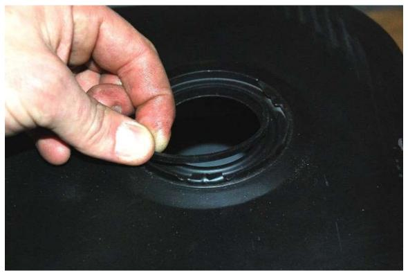
Set the rubber O-ring gaskets in place for the fuel pump pickup.
