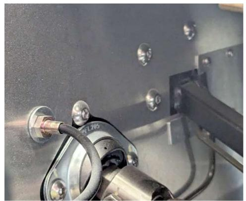
Insert (4) 3/8" x 1" Button head screws through the front of the footbox and through the pedal box mount.
