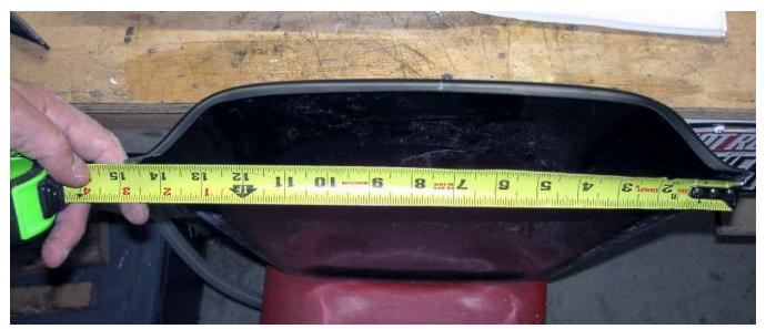
At the front of the scoop, measure across the front and find the center then mark the top of the scoop.
