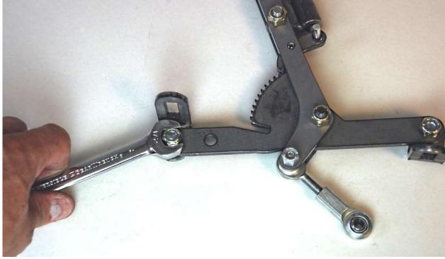
Attach the mount brackets to the fixed gear using a ½" wrench. Leave the locknut slightly loose so positioning can be done on the frame later.
