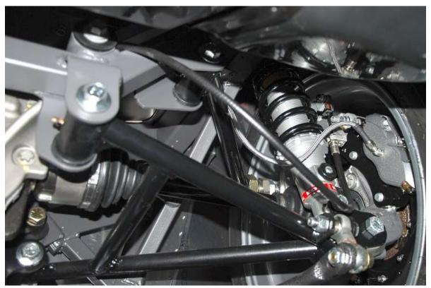
Run the right cable over the center section and right rear mount then down and over to the brake caliper.
