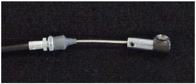
Push and twist the ball stud retainer onto the end of the cable and attach the ball stud retainer using a  $\frac{5}{64}$ " hex key.
