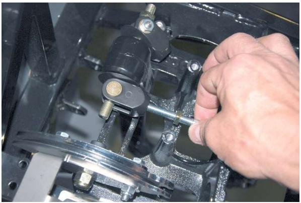
Put one of the master cylinders onto one of the brake master cylinder mounts and turn the threaded shaft into the threaded mount on the brake pedal. As a starting point, thread the shaft in until you can see it is flush on the other side of the mount.
