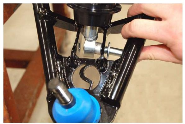
Pass the shock assembly (with the body of the shock up) through the upper A-arm and attach them to the lower control arm using the 0.43" spacers and  $(2) \frac{1}{2}$ " x 2.75" for the lower mounts
