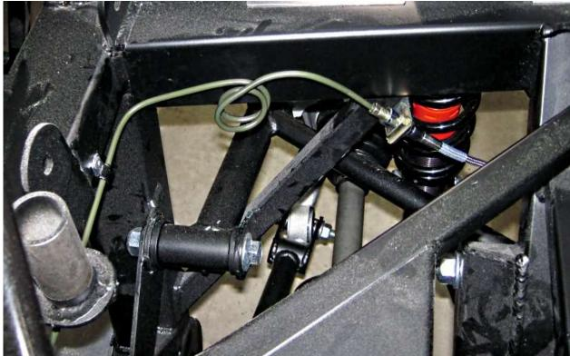
For the right side run a 60" line from the end of the left side connector then forward to the 2"x 3" tube, across and back to the 1" square tube and flexible brake line mount.
