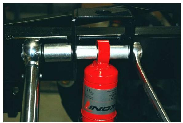
Attach the body end of the shock to the upper shock mount using the two equal length (1.09") spacers,  $12332 \frac{1}{2}"-13 \times 4"$  hex head bolt and 10834 nylon locknut.
