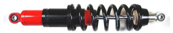
Assembled solid axle Koni coil-over shock.
