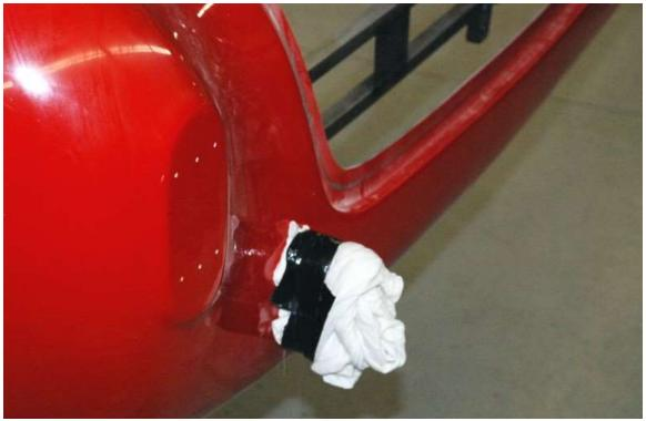
Even with the quick jacks removed, it is still a good idea to wrap the bolts with some rags and duct-tape to save yourself from painful cuts or bruises.
