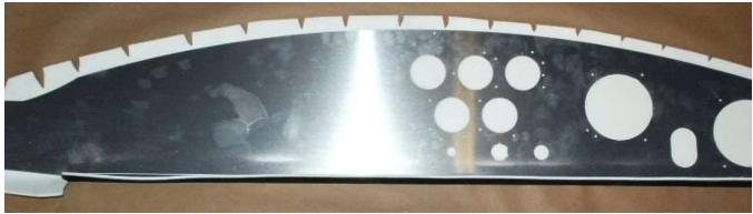
Cut the dash pad in angle shaped cuts every 2" (even closer in the corners) up to about 1/4" from the dash.
