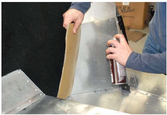
The cockpit rear corners go on next. Be very careful spraying the adhesive once some carpet is mounted. Guard the carpet with masking tape or cardboard.
