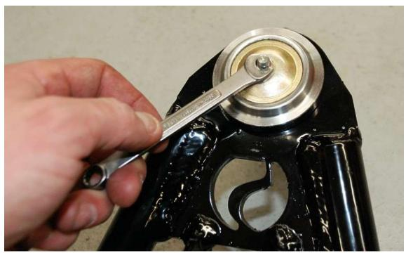
Screw the grease fittings into the arms using a 5/16" wrench.
