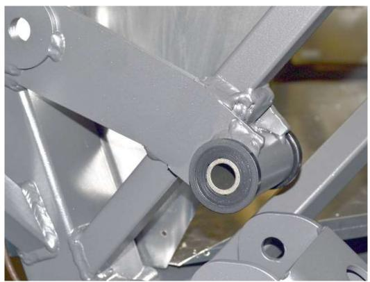
Use a plastic mallet to install the polyurethane bushings marked 2048 and the longer  $(3^{1}/_{16})$  sleeves where the front of the center section will mount.
