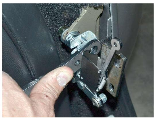
Put the rivnut tool between the latch and the latch base so that the flat end of the striker will touch the tool. This will allow the latch to get mounted 90 degrees to the striker and to get spaced correctly.
