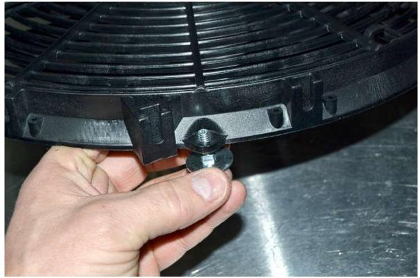
Insert an elevator bolt into the fan from the bottom.
