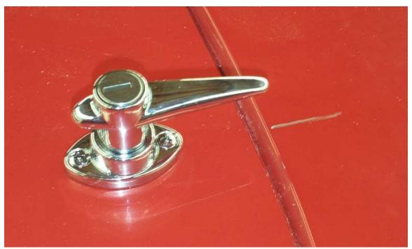
Shut the hood and mark the body where the hood handles line up.
