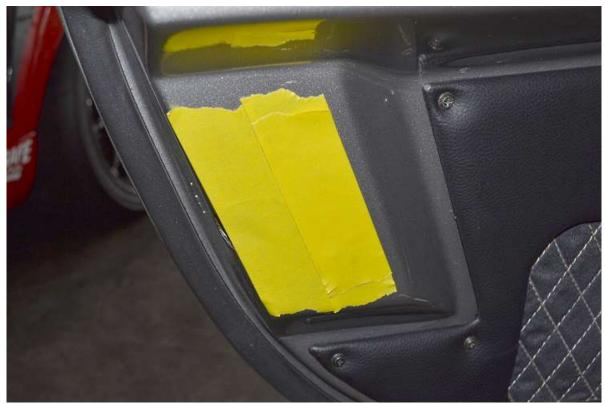
Cover the latch location on the door with masking tape.
