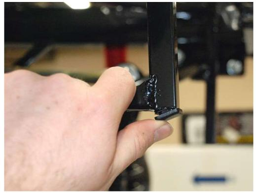
Push the two plastic end caps into the tubes hanging down in front of the gas tank area.
