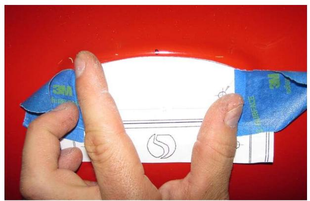
Align and tape the drill template in place.
