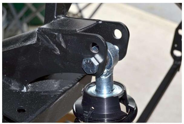
Fasten the shock to the top mount with the  $\frac{1}{2}$ "x 3.25" bolts and 0.675" spacers provided. Torque both upper and lower mounts to **40 ft-lbs**.
