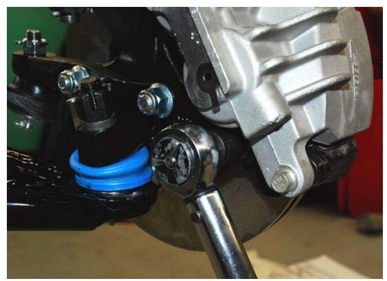
Torque the caliper mounting bolts to 130Nm (95 lb-ft).
