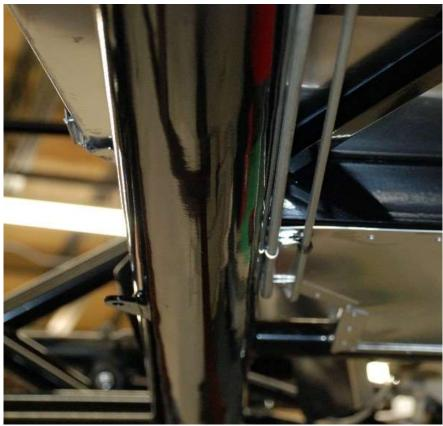
Which side you run down may depend on where you are hooking up to your fuel rail, carburetor, or pressure regulator. We usually run the fuel lines on the passenger side of the car and the brake lines on the driver side of the car.
