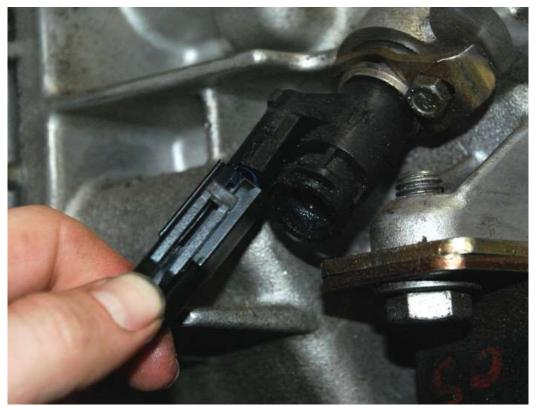
Connect the plug and plug it into the sender. If you are running fuel injection you may also need to send this signal to the computer as well depending on your system.
