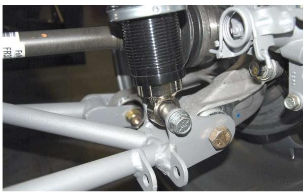
Jack the spindle up so the body end of the shocks can be mounted on the shock mount on the control arm using the longer 1.09" spacer on the back and  $^{7}/_{16}$ " spacer in front of the shock along with the  $^{1}/_{2}$ " x 3.25" bolts and locknuts.
