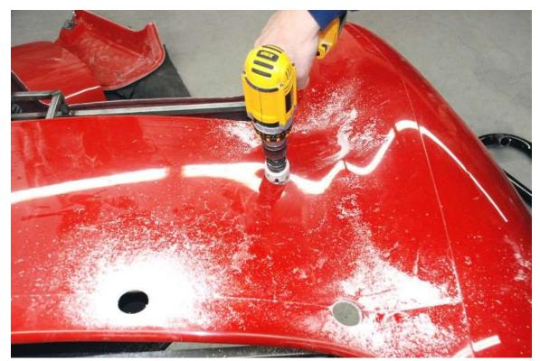
To cut the rear roll bar leg, make 2 holes overlapping so that they form the right length. Use the same 13/4" hole saw centered in the front of the traced opening and with the drill leaning at a 45° angle toward the inner front leg. Stop the drill when it has cut through half of the hole.
