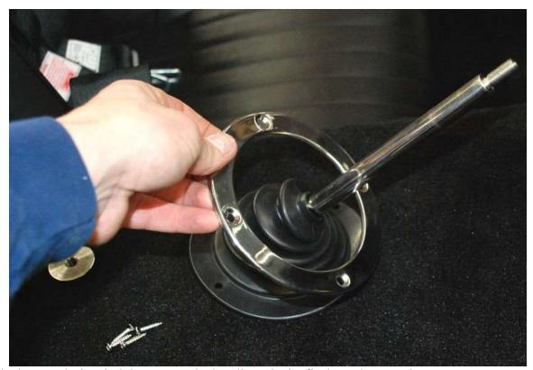
Push the boot and trim rind down over the handle so it sits flush on the tunnel.
