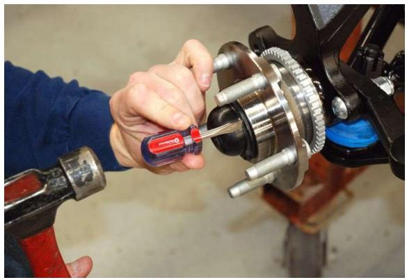
Using a large socket or a flat head screwdriver and rubber mallet, hit the dust cap onto the hub.
