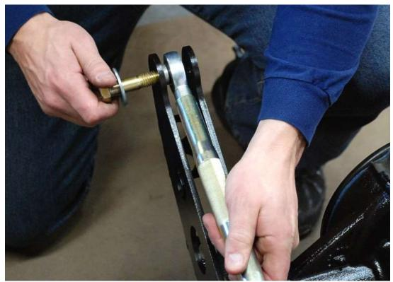
Attach the short upper link tube to the axle upper link mount using the  $\frac{1}{4}$ " spacers on either side of the rod end using a 12382  $\frac{5}{8}$ "-11 x 3" hex head bolt and 15216 mechanical lock nut.
