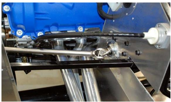
Route the clutch cable down to the bellhousing. Using zip ties or insulated clips tie the cable safely away from the headers and the moving steering components. It can be fastened to the engine using the bracket on the cable to the front lower bolt that holds the starter cable just before it leaves the block or, to the lower engine bay 3/4" tubing.
