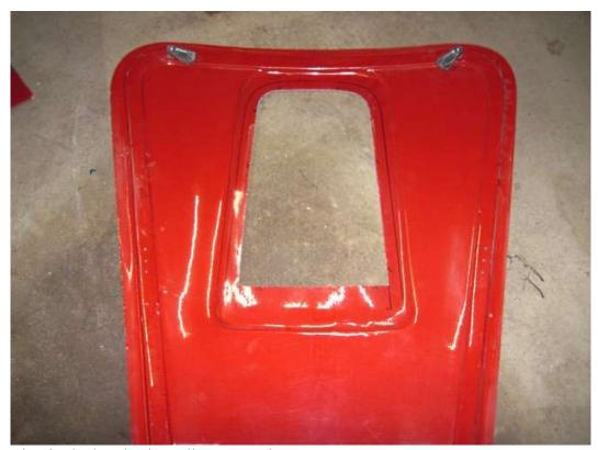
Cut the opening in the hood using a jig saw or air saw.
