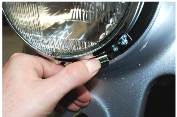
Push the spring clip onto the boss near the bottom of the bucket.
