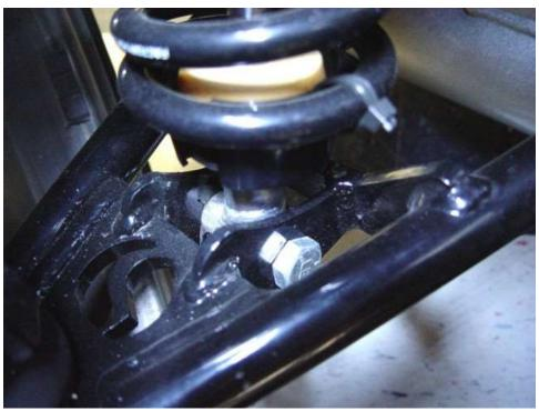
Run zip ties through the holes in the spring hat and around the spring to prevent the spring from becoming unseated.
