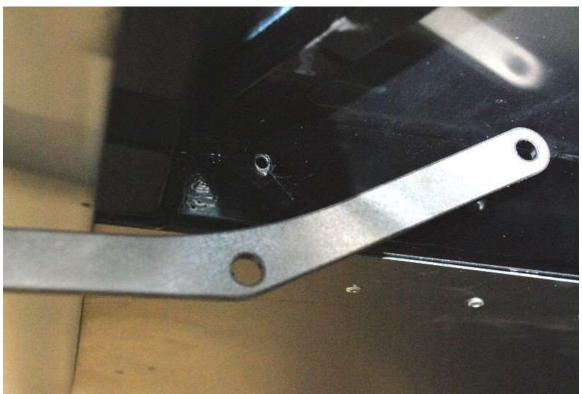
Drill a  $\frac{3}{16}$ " hole in the 2"x 2" outrigger tube directly above the middle hole in the mounting bracket. You want this hole as high as you can get it while still being able to mount the rubber exhaust hanger. About  $\frac{1}{2}$ " down from the aluminum floor.
