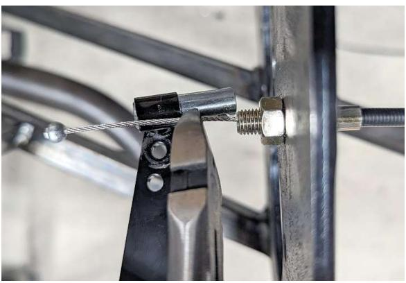
While pulling the cable tight, push the accelerator pedal up until the ball stud retainer hits the end of the throttle cable and clip off the cable ball fitting end so that the cable is long enough to go into the ball stud retainer  $\frac{3}{8}$  and get tightened with the set screw.
