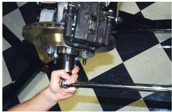
Have a friend sit in the car and step on the brakes. Torque the rear axle nuts to 175 lb-ft.
