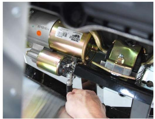
Attach the battery cable to the battery post on the starter.
