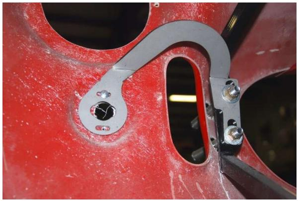
Use the shipping carriage bolt through the turn signal mounting hole until the turn signals are mounted.
