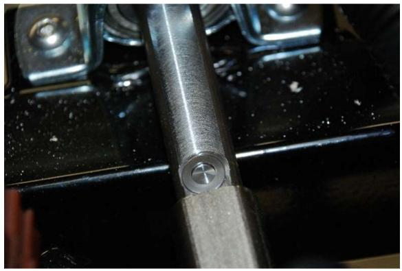
Turn the steering shaft so the recessed bosses for the spring washers are facing up and set the washers in place. Then tap the upper shaft down until the upper clip just disappears into the lower shaft.
