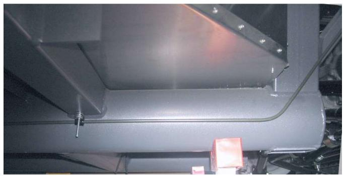
Run the brake line up the back of the 2"x 3" tube using line clips and rivets on the 2"x 2" tubes.
