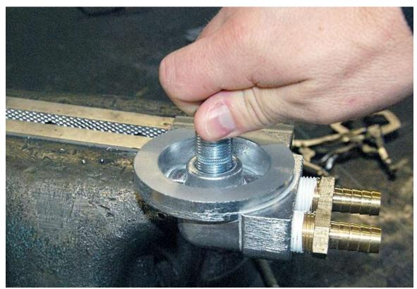
Thread the short end of the threaded nipple into the relocator.
