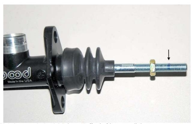
With the jam nut on the threaded shaft, cut 5/8" off each of the master cylinders.
