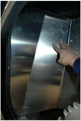
Fit the splash guards in position. If needed, trim them to fit around the outside edge, the weatherstrip will cover the trimming.
