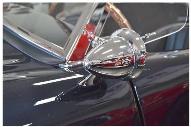
From the underside of the body, use a 5/16" socket to attach the mirror to the body.
