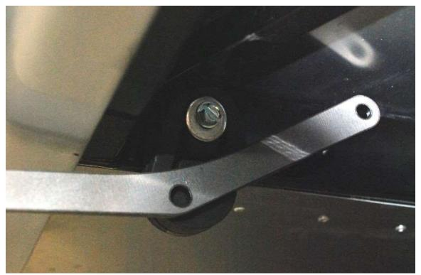
Screw the rubber hanger onto the chassis with the #14 x 1.5" tapping screw using one of the washers between the rubber and the head of the screw.
