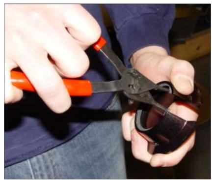
The coil-over hats have a snap ring which holds it in place. Remove this snap ring to assemble the coil over shock.
