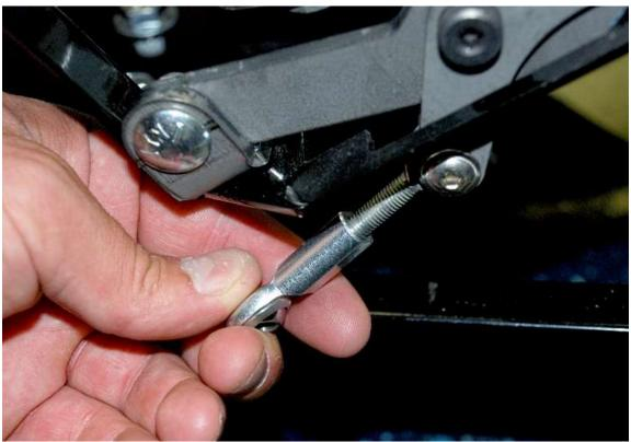
Release the brake and if necessary, remove the 1/4" clevis bolt and readjust the rod end so that the cable is tight.
