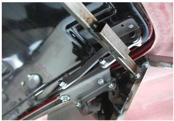
Set the hood in place and attach the two arms to the brackets from the underside of the body.
