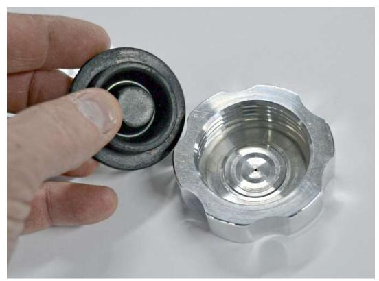
Remove the cap and put the reservoir gasket in the cap.
