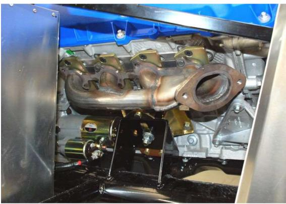
If you are using Shorty headers or stock manifolds bolt them back on. On a small block (302 or 351) the headers are switched side to side and on the 4.6 the headers are flipped upside down. In either case this puts the collector toward the front.
