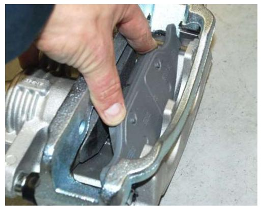
Install the brake pads in the Caliper.
