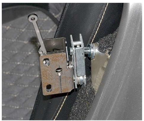
Attach the latch assembly to the striker.
