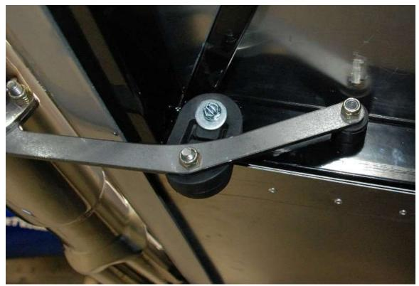
Insert the rubber standoff between the bracket and outrigger and put the nut on finger tight then run the long  $\frac{5}{16}$ " bolt through from inside the footbox into the threads in the standoff.
