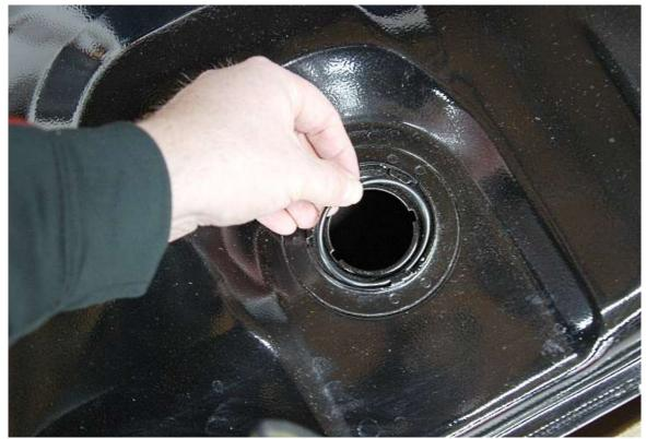
Set the rubber O-ring in place for the fuel level sending unit.
