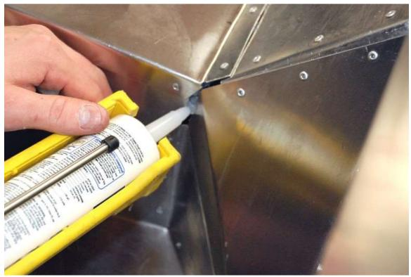
Double check the aluminum edges and corners for any areas that look like they are not sealed. Run a small bead of silicone in these corners, seams and around the slots where the seat harness mounts poke through.
