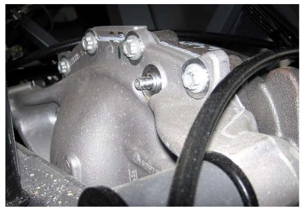
Use a hammer on the end of the barb to put the nipple in the rear cover.
