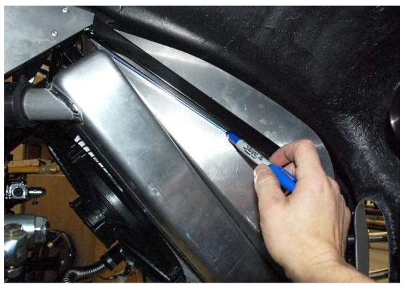
From the backside of the panel, mark the location of the 3/4" tube.
