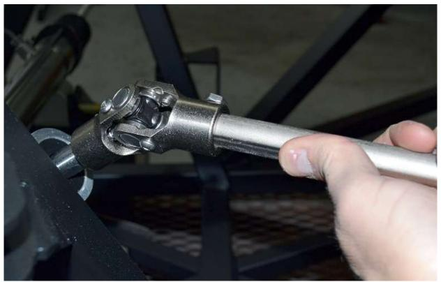
On the lower shaft make sure the shaft does not go into the lower joint and is no more than flush on the inside.
