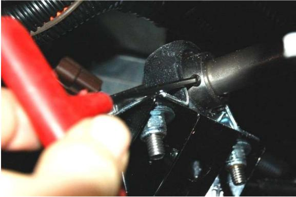
With the steering wheel in the position that is most comfortable for you tighten the set screws on the collar of the upper steering bearing.
