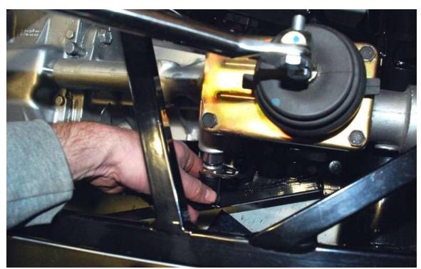
Put a little oil on the O-ring and install the sender in your transmission. Use the original bolt to hold the sending unit in place.
