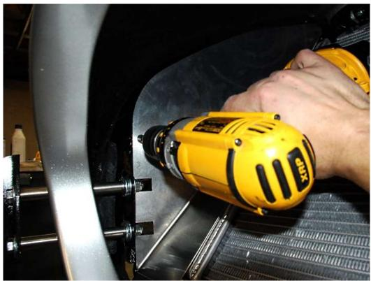
Line up the edge of the radiator fins with the edge of the side aluminum and attach the piece to the 3/4" tube using a self-tapping screw.
