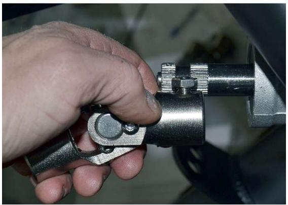
Note the location of the set screw on the splined end of the u-joint compared to the recessed unsplined area in the middle of the input shaft on the steering rack.
