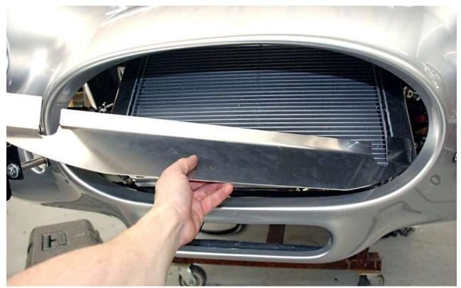
Pass the radiator floor piece through the nose.
