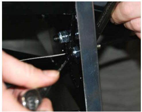
Tighten the cable sheath to the firewall with the retaining nut. A piece of tape on the end of the cable will help prevent it from backing out of the sheath.
