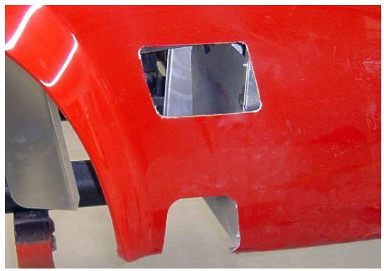
Connect the flush surfaces of the holes with a jig saw.
