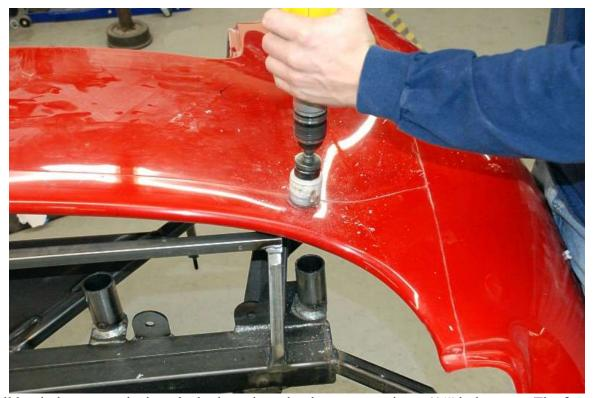
The roll bar holes are marked on the body and need to be cut out using a  $1\frac{3}{4}$ " holes saw. The front two holes are cut centering the saw in the marked circle and drilling vertically to match the angle the bar comes through the body.
