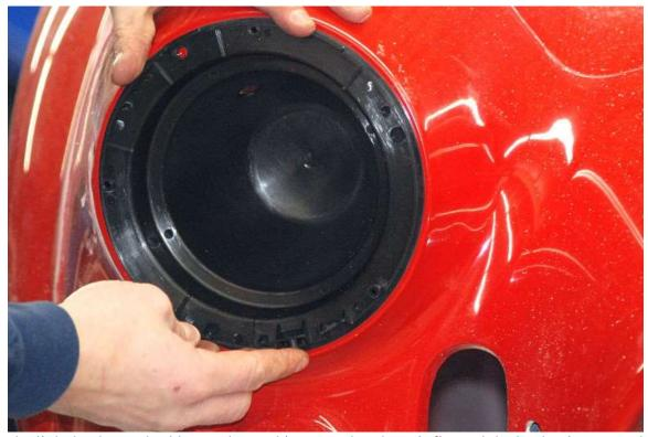
Test fit the light bucket and rubber gasket making sure that they sit flat and the bucket is centered on the fender. Mark and drill the four mounting screws for the headlight bucket using a  $\frac{1}{8}$ " drill bit.
