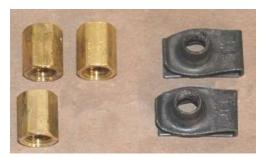
Unpack the hardware from the brake line components. The U-nuts on the right are for the E-brake handle
