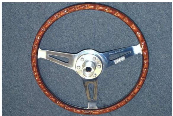
Bolt the steering wheel to the boss using the M6 x 30mm Philips head screws and locknuts. The pattern is not symmetrical so it will only line up one way.
