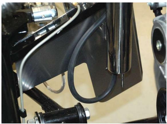
Make sure you attach the hose to the tube that runs off the bottom of the tank and not the one that extends up into the tank.
