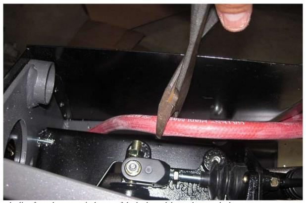
Route the line from the reservoir the top of the brake pedal area then cut the hose.
