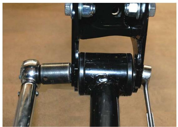
Attach the lower control arms to the brackets on the axle using the M12 x 110mm bolt provided. Torque to 101-111Nm (75-82 lb-ft).
