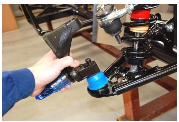
Make sure the grease boot is in place on the balljoint then mount the spindle to the lower control arm.
