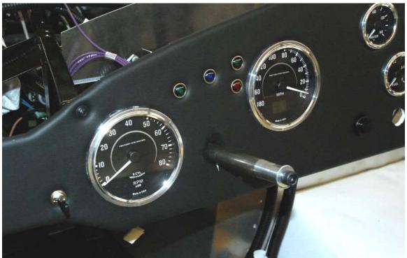
Mount the turn signal switch and high low beam switch as well as indicators in the dash. These can be mounted wherever you like, use a ½" drill bit for the holes on both the switches and indicator lights.
