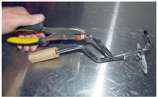
Remove and discard the rubber piece on the end of the return line, this can affect the fuel pressure at the engine.
