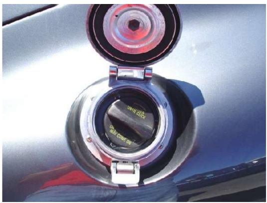
Screw the plastic gas cap into the Aston Lemans style cap.
