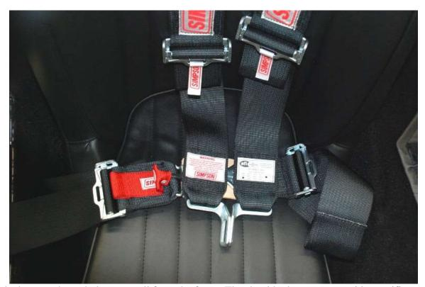
Slide the harness through the rear wall from the front. The shoulder harnesses are side specific so make sure you have the sides correct.
