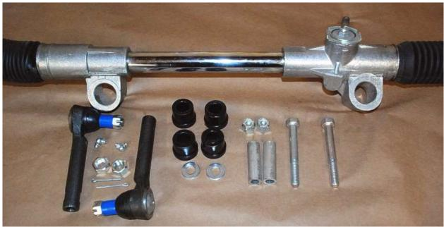
Unpack the steering rack and the mounting assembly. Manual rack shown.
