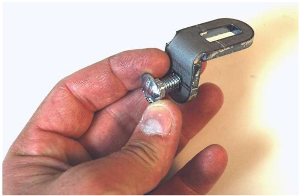
Insert a  $\frac{5}{16}$ " carriage bolt into one of the bent mount brackets so the square shoulder is in the square hole.
