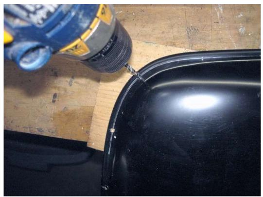
Drill <sup>3</sup>/<sub>16</sub>" holes around the edge of the scoop.
