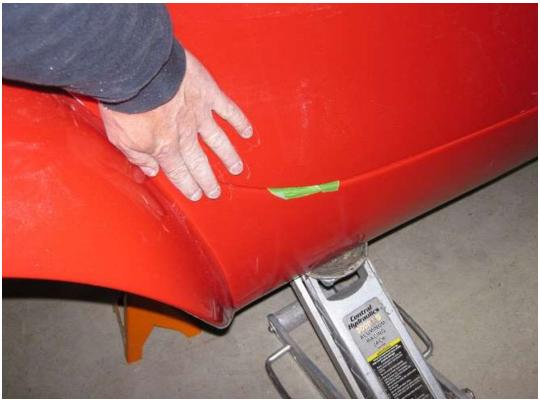
Push or pull the back of the body to line it up with the door if necessary.
