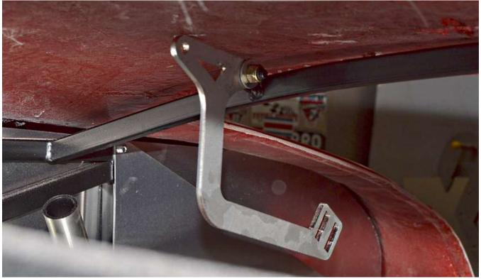
Hang the hinge arms on the chassis using the shoulder bolts.
