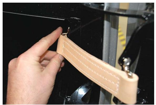
While holding the door open, pull the check strap tight and mark the location of the mount holes on the inside face of the 2"x 2" tube.
