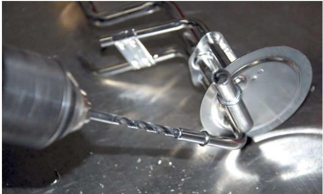
Starting with a  $\frac{1}{4}$ " drill bit drill out the end of the return line then change to a  $\frac{9}{32}$ " or  $\frac{19}{64}$ " drill bit, the pressed end is a little restrictive.
