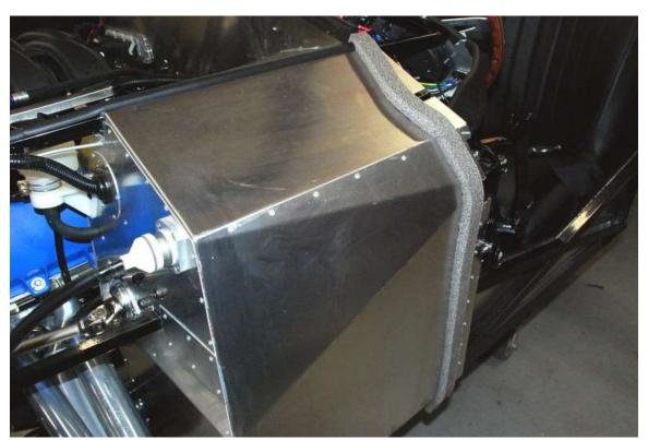
When you are ready to mount the body, unpack the expanding foam and run a small section up the outside of each footbox just forward of the door hinge.
