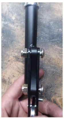
Slide the lower handle between the ratchet to handle mount plates and bolt the three pieces together using the two  $^{5}/_{16}$ "x 1" button head screws as shown above. The bolt heads should be on the right so there is more clearance against the transmission tunnel.
