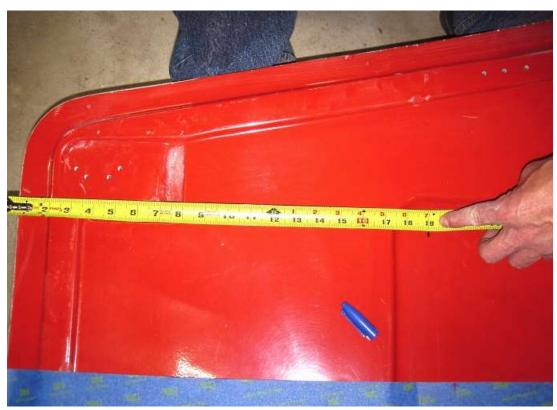
From the front edge of the hood measure back 19" and mark the underside of the hood.
