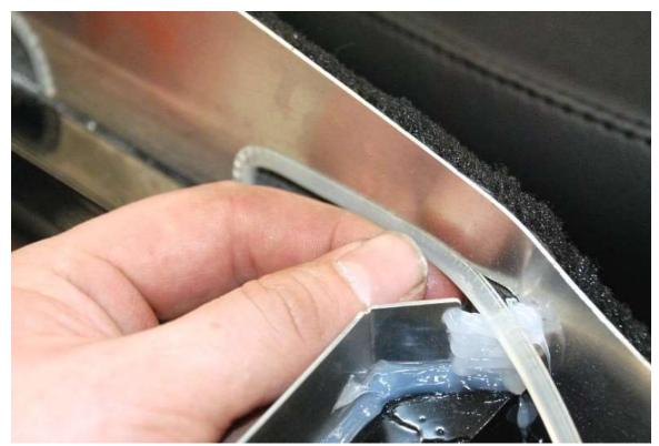
Use some of the serrated grommeting from the electrical assembly to cover the edge where the harness passes through.
