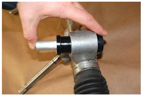
Push the bushings and sleeves (from Box 1) into the mounting bosses on the rack.
