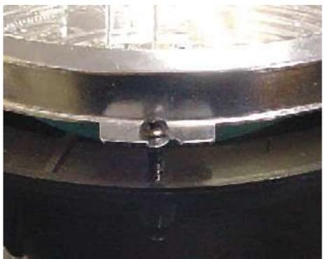
Plug the light into the connector and mount the bulb to the bucket. The slotted parts of the mounting flange go onto the adjusting screws between the screw head and flange.
