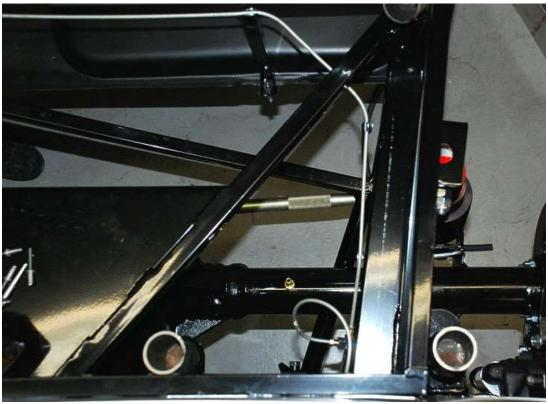
Run a 60" brake line from the "T" up the ¾" tube to the front fuel tank mount tubes and over to the passenger side ¾" tube. An alternative to running it this way would be to run it across the backside of the 2"x 3" tube.
