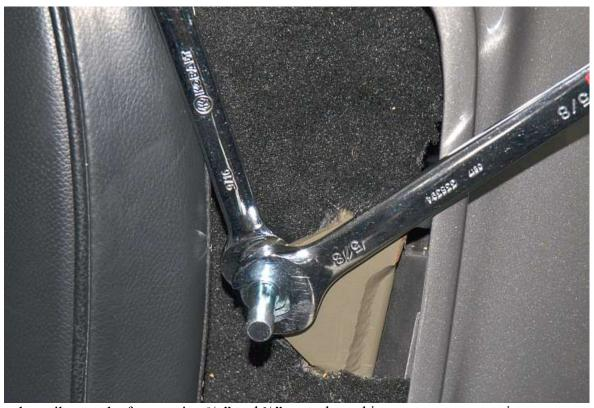
Tighten the striker on the frame using 9/16" and 5/8" wrenches taking care not to move it.
