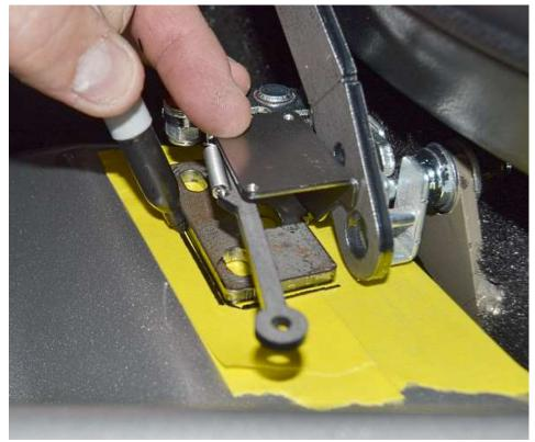
Close the door so that it contacts the latch base then, holding the latch against the rivnut tool so the latch is 90 degrees to the striker, mark around the latch base on at least 2 sides.
