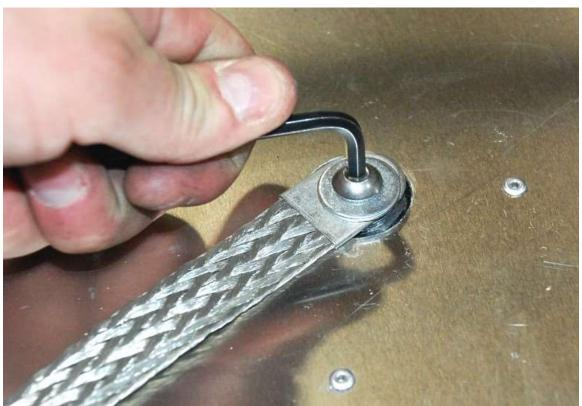
Attach the ground strap to the chassis with the supplied  $^{5}/_{16}$ " button head screw, locknut,  $^{3}/_{16}$ " hex key and  $^{1}/_{2}$ " socket.
