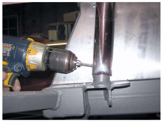
Repeat the step drilling through the rollbar for both front lower mounts. After drilling each hole, put the bolt in the hole so the rollbar stays in the correct location.
