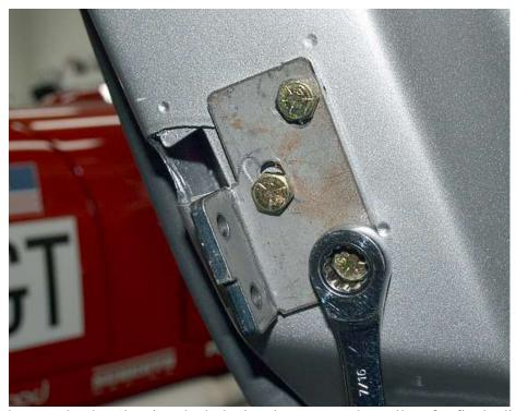
Attach the latch base to the door leaving the bolts just loose enough to allow for final adjustments using a  $\frac{7}{16}$ " wrench.
