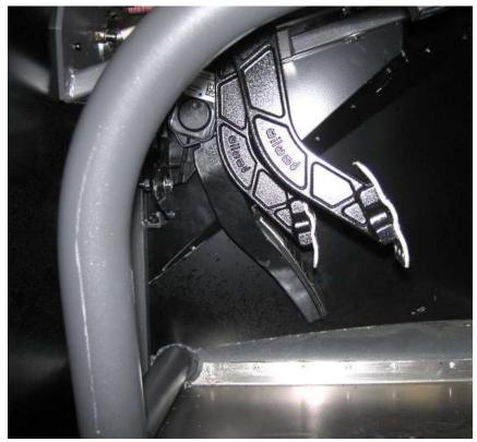
Adjust the clutch pedal stop and master cylinder threaded shafts so that the pedal height is comfortable. In general, the clutch pedal is about 2" higher than the brake pedal and the brake pedal is higher than the accelerator pedal so that when the brakes are pressed the brake pedal is even with the accelerator pedal.
