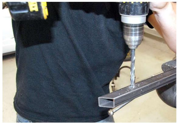
Starting with a  $\frac{3}{16}$ " drill bit then opening it up to  $\frac{25}{64}$ ", drill a hole where you want to install the rivnut. Installed in tube for demo purpose.
