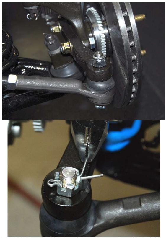
Torque the Tie Rod End nut to 25 lb-ft. If a castle nut is used, torque the nut then install the cotter pin.
