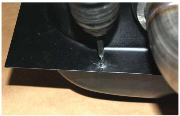
Drill a ¼" hole through the tank flange on the mark made.
