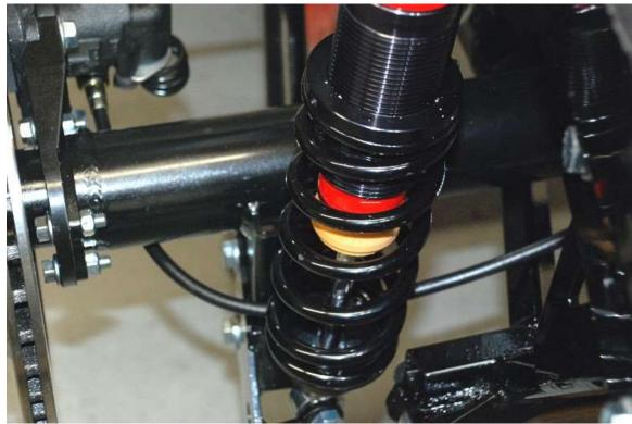
Route the cables back to the calipers and attach. Make sure your routing is out of the way of any moving parts and the cable has slack to move with the axle.
