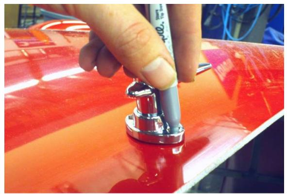
Set the handles in the holes drilled in the hood so that they are lined up squarely with the edge and mark the screw holes on the hood.
