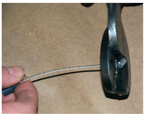
Unpack the throttle cable and cut the cylinder end off. Make sure your cutters are very sharp so as not to fray the cable.
