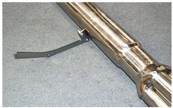
Bolt the mounting bracket to the pipe on the forward side of the bracket.
