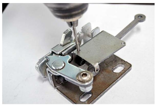
With a bit of oil or other lubricant on the tap, **slowly** run the tap through the small holes in the cover mount plate.
