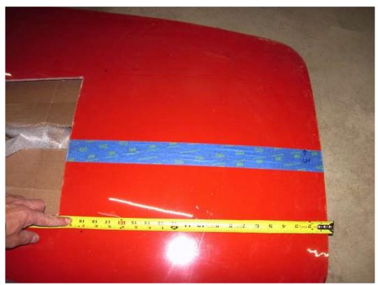
On the top side of the hood measure back from the front and mark the hood at 19".
