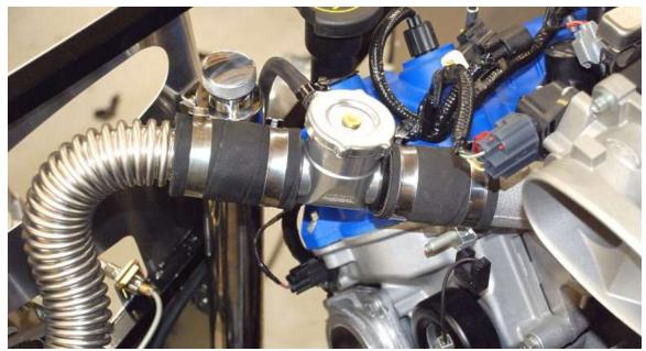
Put the radiator cap in place on the filler for now so it doesn't get lost.
