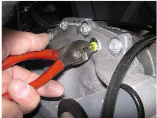
Remove the plug at the top of the rear cover.
