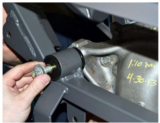
Flatten the center section out so it is horizontal then back it up so it is above the mount locations and lower it down so the bolts can be installed. The 15962 M14 x 100 bolts are used for the rear mounts.
