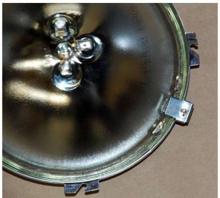
Screw the mounting flange onto the light with the 3 small tabs and small screws. The tabs are bent to fit around the bosses on the light.
