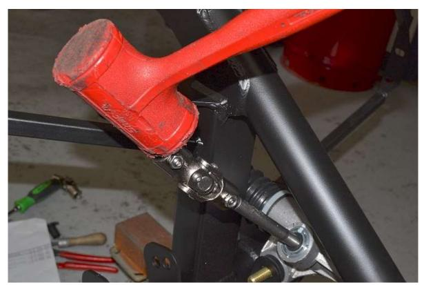
If necessary, use a plastic mallet to get the joint onto the spline, it is tight.
