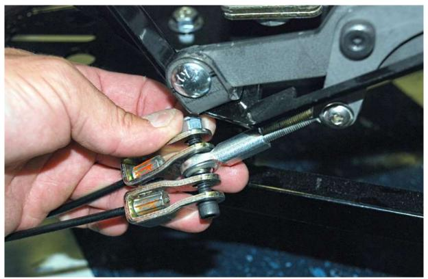
Put the locknut back on the 1/4" bolt hand tight.
