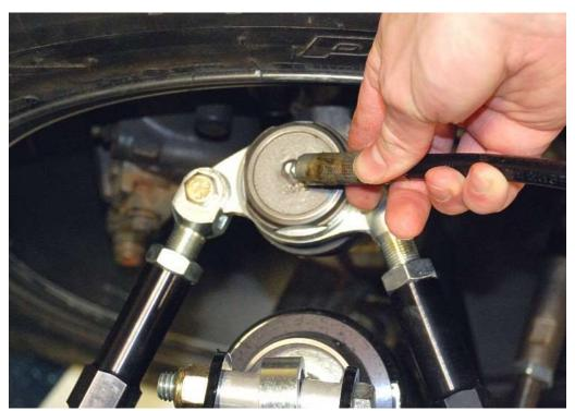
All of the suspension and steering components that have grease fitting need to be greased. With a grease gun squeeze grease into each fitting on all the control arms, including rear lowers on a slid axle, and tie rods.
