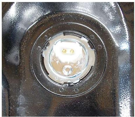
Make sure that the lock ring is held by all three locking tabs on the tank or the sender will leak.
