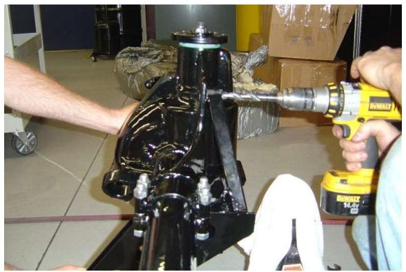
The front attachment of the upper link axle mount attaches to the hole on the flange section of the pumpkin. This hole has some variance and may need to be drilled out from the bottom side using the mount as a guide.
