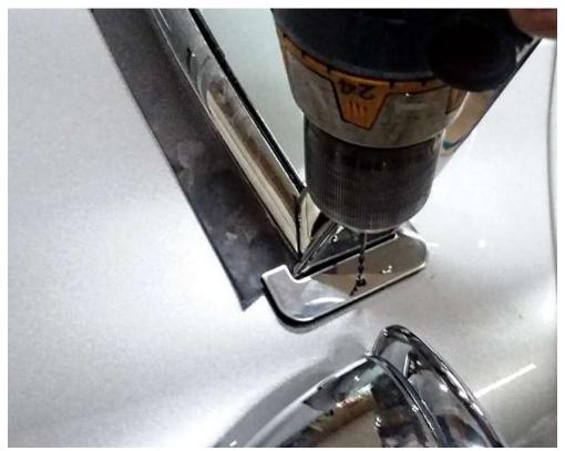
Use a <sup>3</sup>/<sub>32</sub>" drill bit through the base plate holes for the mounting screws.
