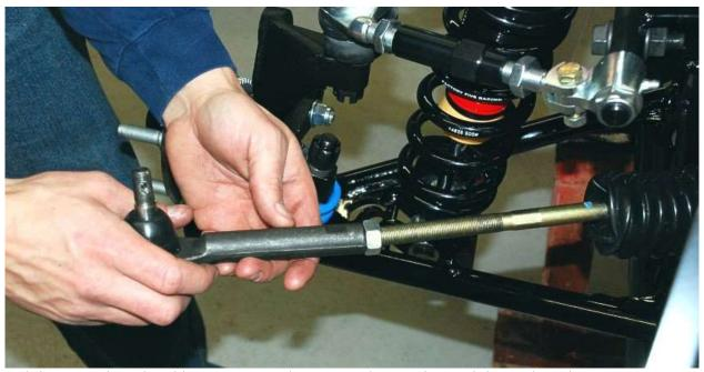
Thread the outer tie rod and jam nut 1"-2" down onto the steering rack inner tie rod.
