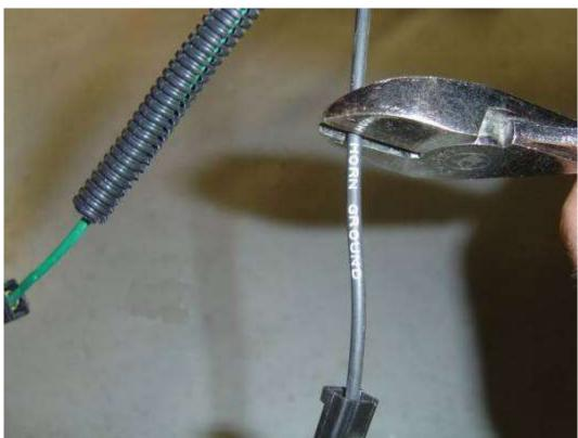
Locate the chassis harness horn wires on the front chassis harness. Cut 2" off the end of the chassis harness horn ground wire and strip the end of the chassis harness ground wire.
