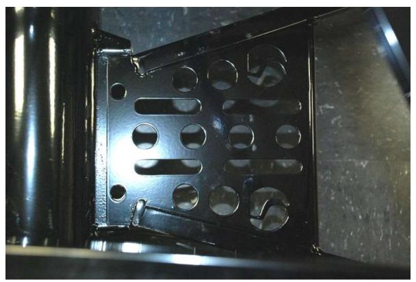
Jack the transmission up and mount the a-frame underneath it. Normally this sits above the frame tabs but can be mounted underneath if extra clearance is needed.
