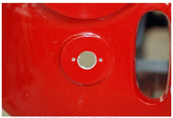
Drill the outer holes with a  $\frac{7}{32}$ " drill bit and the inner with a  $\frac{11}{4}$ " hole saw.
