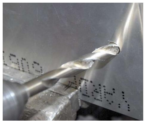
Decide the routing of your reservoir to master cylinder hose and drill a ½" hole through the aluminum for the bulkhead fitting. The fitting is slightly larger than ½" so wiggle the ½" bit around to oversize it.
