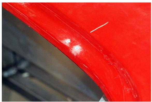
Open the hood and drill two  $_{3}/_{16}$ " holes in the hood opening recess  $_{4}$ " on either side of the centerline and  $_{4}$ " back from the edge of the opening. These are for mounting the hood catch brackets.
