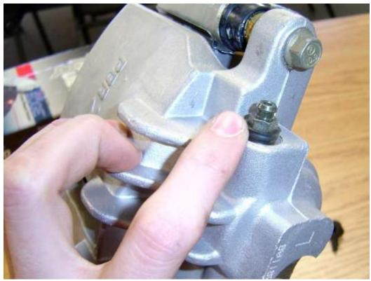
Install the caliper on the spindle; make sure that the fluid bleeder is at the top of the caliper; use the M12 x 35mm bolts packed with the spindles.
