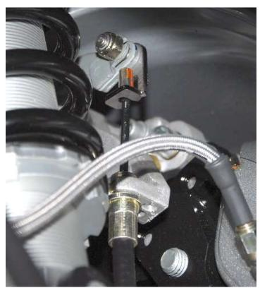
Insert the cable end into the bent bracket then bolt the bracket to the e-brake lever.
