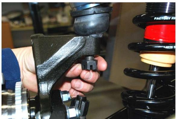
Attach the upper ball joint to the spindle and torque to 75 lb-ft and install the cotter pin.
