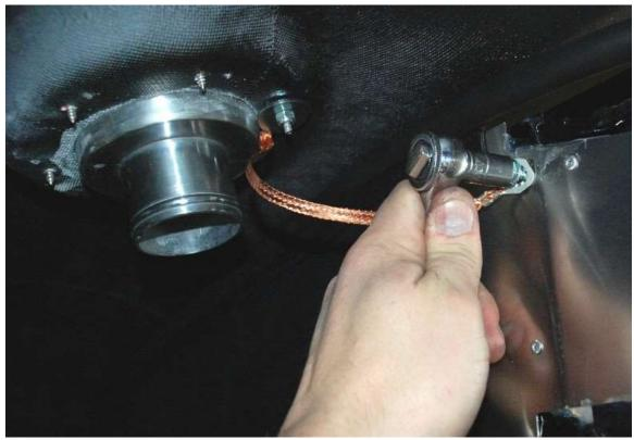
Ground the fuel filler strap to the chassis using the screw that came in the cap hardware.
