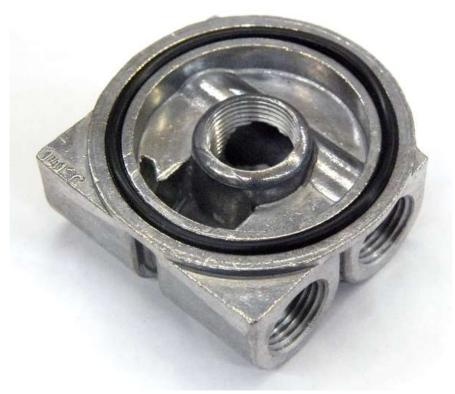
Place the O-ring in the adapter groove.
