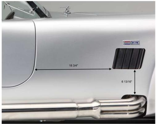
Use the template and measurements in the picture below to locate the template on the body.
