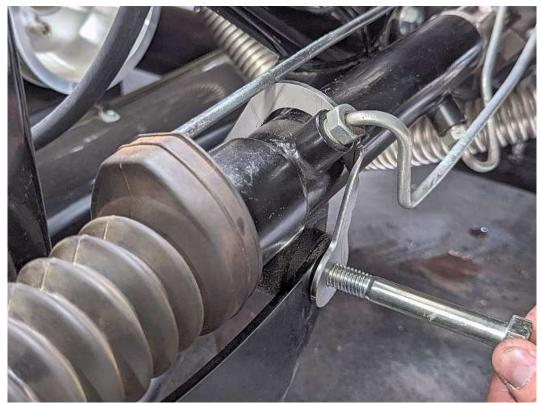
Remove the washer from the bolt then insert it through the bracket and frame.
