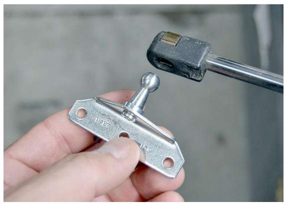
Attach the rod end of the gas strut to the ball stud bracket.
