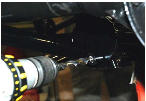
For the front mount, use a ½" drill bit and drill through the sleeve on the mount. Make sure before drilling that the hole is away from the side of the 2"x 3" tube so that a nut can be attached on the back of the bolt from the bottom of the tube.
