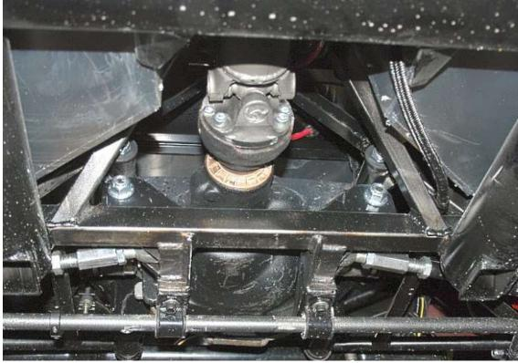
Insert the driveshaft into the transmission, check which bolt length is needed, the  $M10 \times 25 mm$  socket head or the  $M10 \times 20 mm$  socket head depending on the flange thickness. Make sure the bolt goes all the way into the adapter but does not bottom out before tightening.
