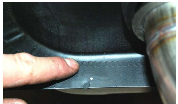
Move the retainer out of the way and make sure your mark is outside the weld that holds the two tank halves together.
