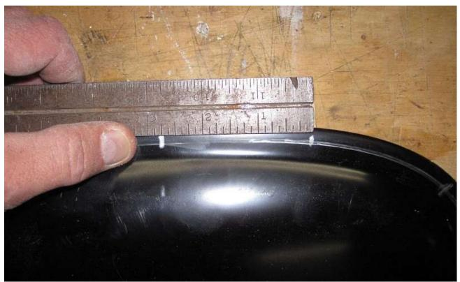
Where the scoops starts to curve measure from the last straight rivet location 2.50" back and mark the line then another 2.50".
