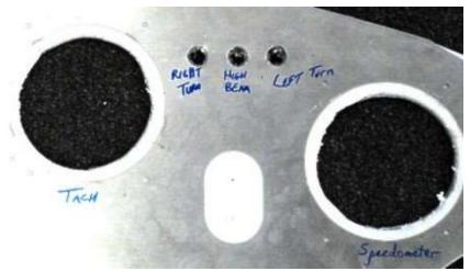
If you would like to install the three lights that are included in the kit, one possible layout is similar to the original Roadsters, positioned directly over the steering column in a straight line. Use a ½" drill bit for the holes.
