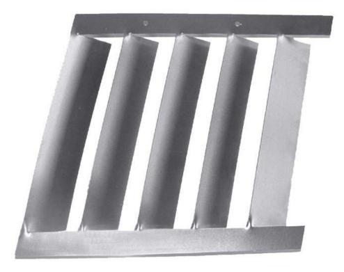
Holding the top and bottom flanges, bend the fins in so they are roughly at a  $45^{\circ}$  angle.
