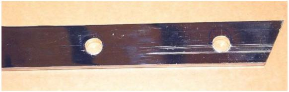
At the marks made on the sidebar, measure and mark the center of the sidebar to give the correct angle adjustment on the windshield. Drill the holes with a ½" bit.
