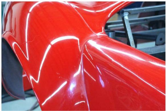
Adjust the door with the hinge until the panel surfaces are lined up with the body. Start at the top of the door and match the curved surfaces.
