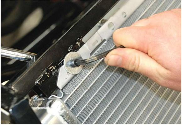
Mount the radiator top to the flange using the #14 x  $\frac{1}{2}$ " tapping screws. The bottom stays zip tied for now.
