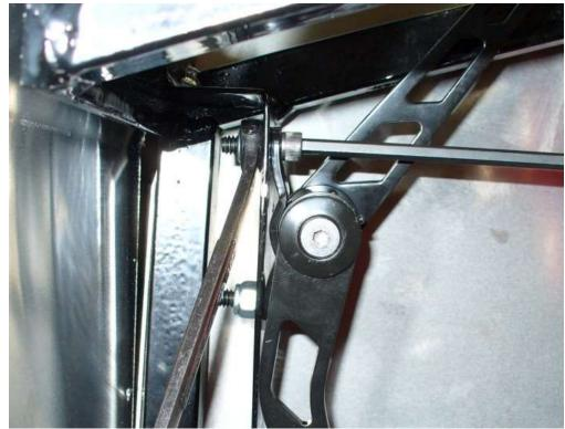
Bolt the pedal to the mount plate using the 1/4"x 3/4" screws and locknuts.
