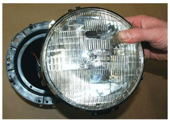
Line up the headlight with the bucket to get the proper orientation. The bottom of the bucket is the only screw boss that comes in from the side and the writing on the headlight should be right side up.
