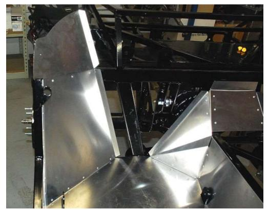
The outer cockpit corners get marked on the bottom flange and where they meet the chassis. Drill silicone and rivet these in place.
