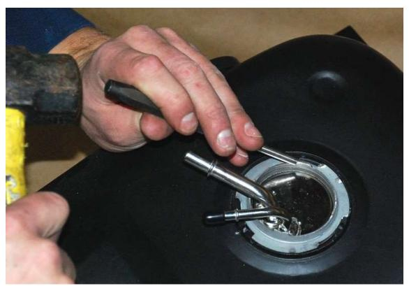
With the pickup all the way down, slide the mounting collar and tap tightly into place with a punch and hammer.
