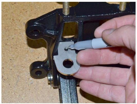
Place the switch mount between the clutch pedal mount tabs on the side closest to the clutch pedal pivot holes and drill a  $^{3}/_{16}$ " hole through the switch mount hole and the pedal box.
