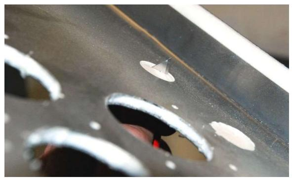
Using a razor knife, cut the gauge holes and switch holes out of the dash pad, cut the holes in from the aluminum about 1/8". DO NOT cut out the steering shaft hole.
