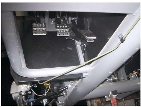
From the front of the footbox angle into the 4" main tube under where the footbox floor would be.
