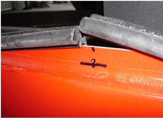
With the pin location compared to the trunk edge known and the trunk edge marked on the body along with the lowest mount point of the pin cover marked, the locations should match up. The latch cover may need to be trimmed slightly to go onto the radius of the body.
