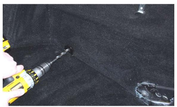
Drill through the inner lap belt mount into the tunnel with a ½ in. bit.
