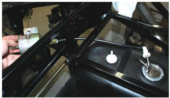
Attach the short nylon fuel line to the filter and the tank to show where your mounting location must be. The elbow end can attach to either end as shown here; we have attached it to the tank.
