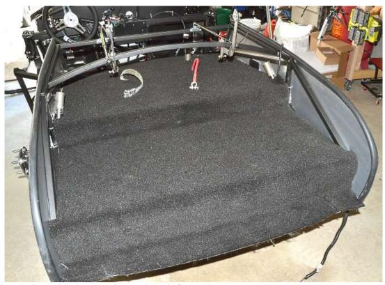
Line up the notches with the 3/4" tubes and work forward.
