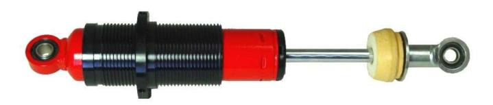
Slide the coil sleeve over the body of the damper beginning at the end which has the rubber bump stop. The unthreaded end of the sleeve goes first so that it will sit on the snap ring on the shock body.
