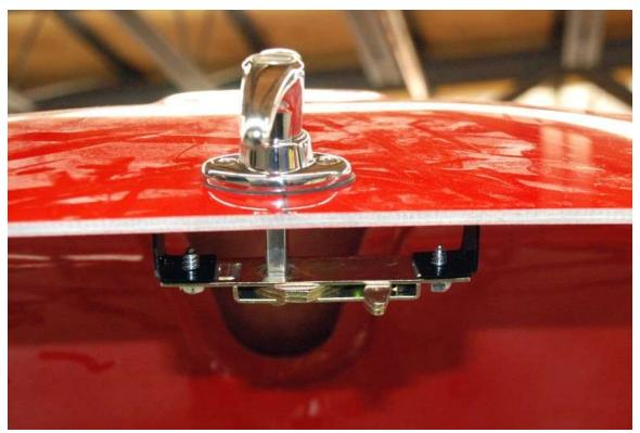
Bolt the handle to the trunk running the bolts through the trunk and the latch mount.
