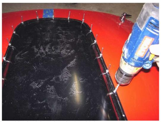
Drill out the remaining rivet holes putting a rivet in each hole as you go.
