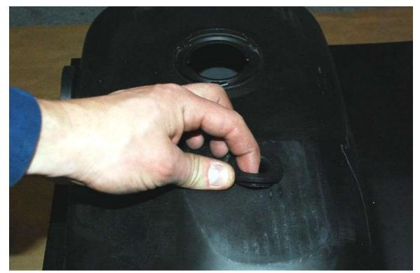
Insert the small rubber vent gasket in the small hole on the top of the tank.
