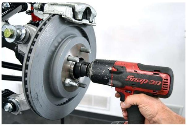
Use a 36mm deep socket and impact wrench to tighten the CV axle nut until it touches the bearing.
