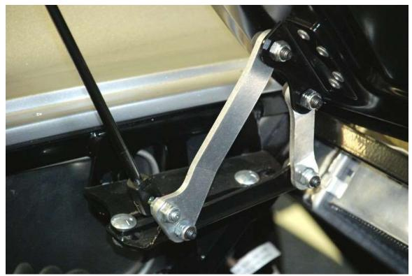
If not already done, install the threaded ball studs in the hole on the long hinge arms with the ball pointed toward the outside of the car using a  $\frac{5}{16}$ " locknut. Then snap the gas piston shaft onto the ball.
