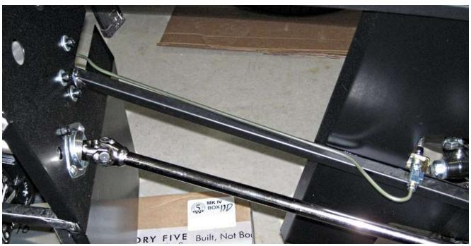
Run a 60" brake line from the front master cylinder out the front of the pedalbox along the 3/4" tube to the front left brake line mount.
