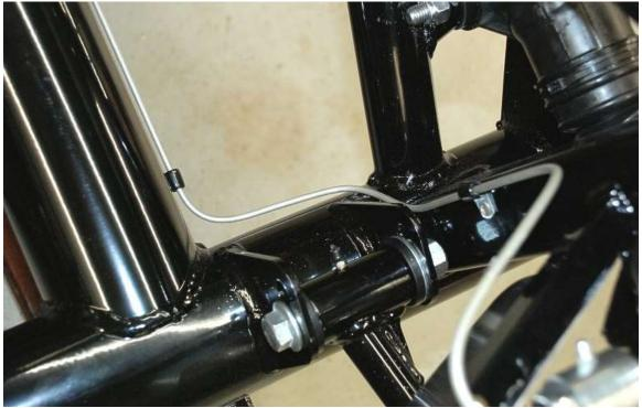
When you are happy with the routing use the small insulated line clips and 3/16" rivets to hold it in place.
