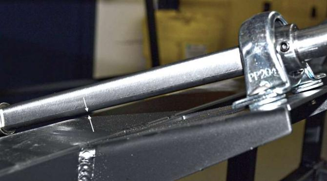
If necessary or to raise the height of the steering wheel, put washers under the upper pillow block bearing mount so that the upper shaft does not hit the frame or the wheel is at the height desired.
