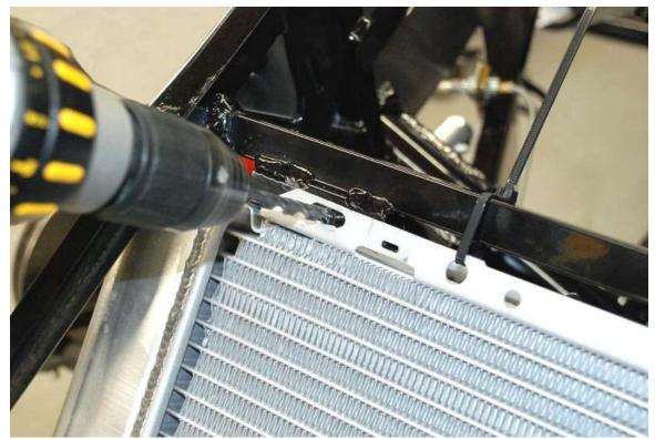
Drill  $\frac{3}{16}$ " holes through the first side of the tube only in order to mount the radiator top flange to the two small mounting tubes on the chassis.
