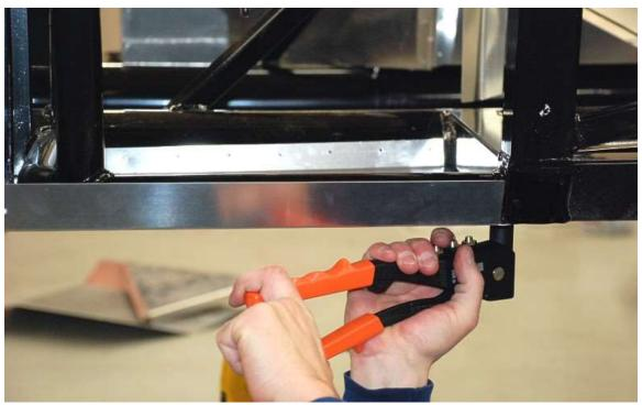
Drill silicone and install the driver's footbox floor. The outer flange does not get drilled yet.
