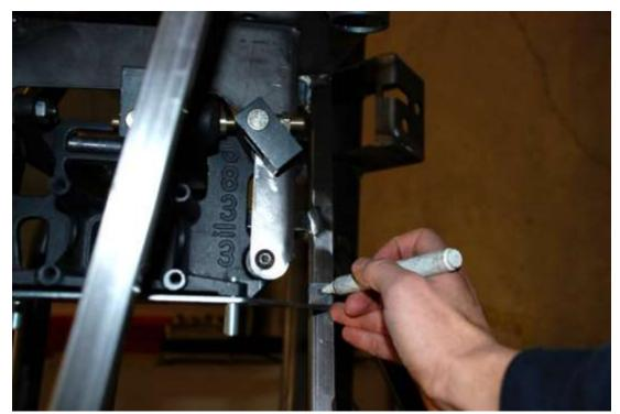
Tighten two of the front 3/8" screws then use a marker to mark the locations of the rear mount holes on the 3/4" tubes.
