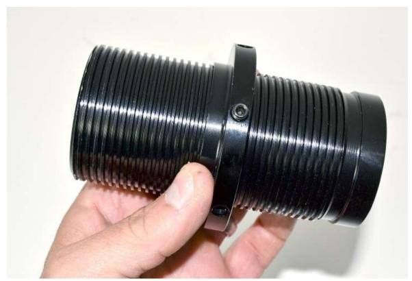
Screw the spring seat down on the sleeve so it is closer to the unthreaded end.
