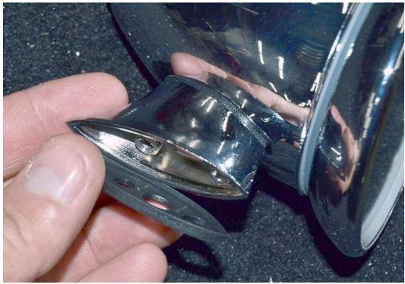
Put the gasket on the bottom of the mirror so the holes line up with the threaded hole locations.
