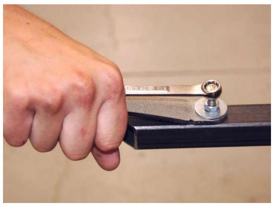
Insert the rivnut in the hole holding onto both the tool handle and the wrench.
