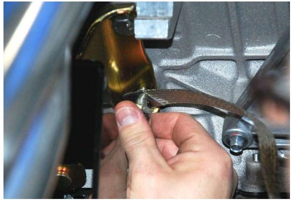
Bolt the ground strap to the hole on the frame engine mount.
