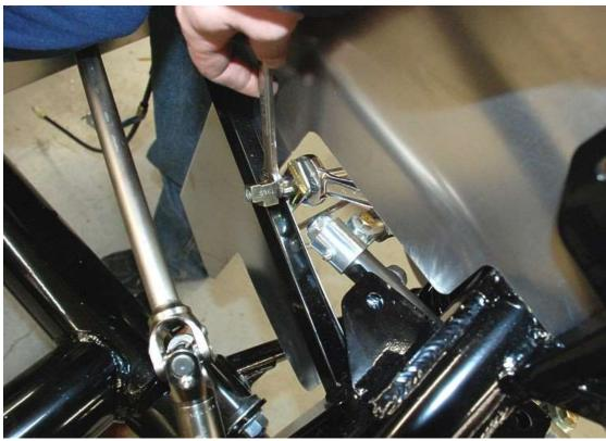
Screw the brake line T fitting into the end of the left side brake adapter and tighten with ½" and ¾" wrenches.
