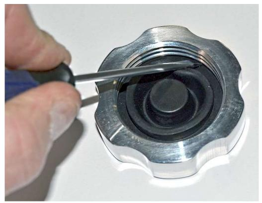
Use a small screwdriver to get the edge down under the threads.
