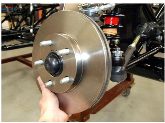
Clean the rotor with brake cleaner and push it onto the hub.
