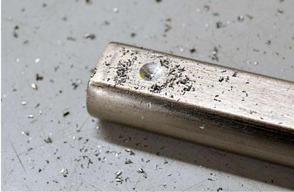
Use a  $\frac{3}{16}$ " drill bit followed by a  $\frac{5}{16}$ " drill bit at the point marked to create a slight recess for the set screw.
