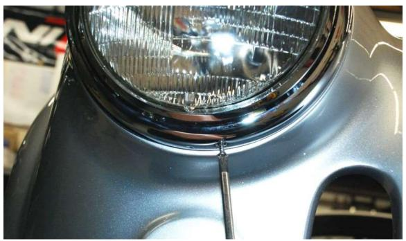
Mount the trim ring hooking it over the bucket on the top and screwing it into the bottom using the countersunk screw.
