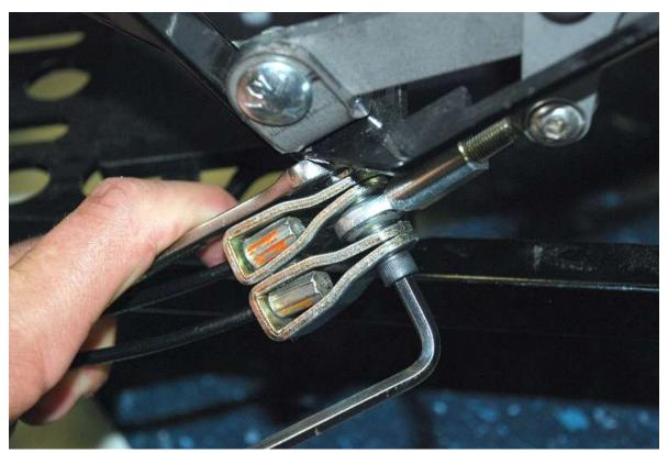
Reinstall the clevises and 1/4" bolt then tighten the bolt so that the clevis ends are closed, this will prevent the cable ends from coming out.
