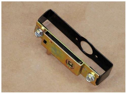
Screw the trunk latch to the holder with the short #14 screws lining the small square hole with the hole for the handle.
