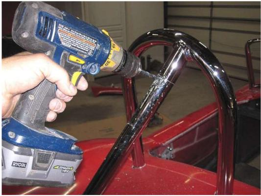
Step drill the top of the rear leg first using an 1/8" bit followed by a 3/16" then a 5/16" bit.
