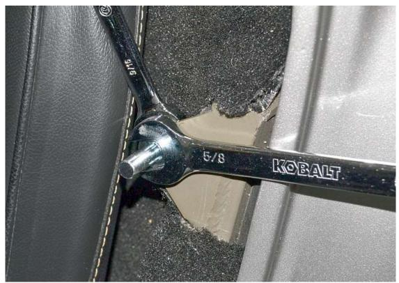
Snug up the locknut so that the striker can just move in the slot but stay in place using  $\frac{9}{16}$ " and  $\frac{5}{8}$ " wrenches.
