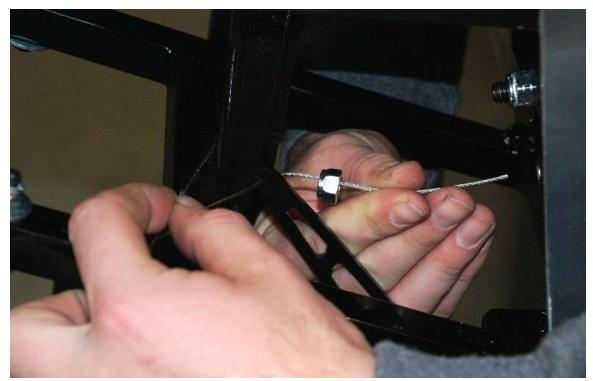
Thread the inner cable through the cable retaining lock nut from the accelerator cable components assembly.
