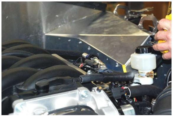
Silicone and install the footbox inside top panel. Leave the top flange un-riveted for now; use some clamps or tape to hold it in place.
