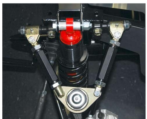
Mount the upper control arms to the chassis with the grease fittings pointed up using the  $\frac{1}{2}$ "x 1.75" flange head bolts and locknuts. Use the mount holes that are vertical on the side of the 2"x 3" tube, not the top horizontal ones.
