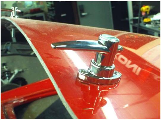
Drill the holes with a 7/64" bit then screw the handles down using the screws from the set.
