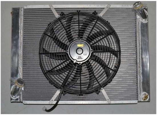
Place the fan on the radiator and rotate the mounts so that the smaller holes line up with the radiator flange.
