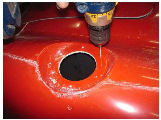
Remove the cap and finish drilling the 1/8" holes.
