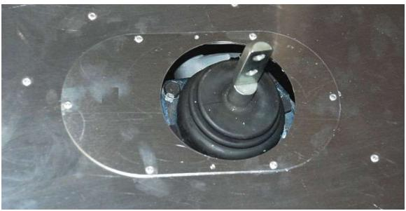
Silicone and install the shifter hole cover. Make sure it does not interfere with the movement of the shift lever.
