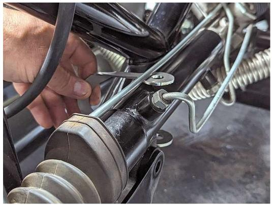
From the back side of the rack, slide the bracket under the bellows cross tube and to the left side of the hydraulic line connection.
