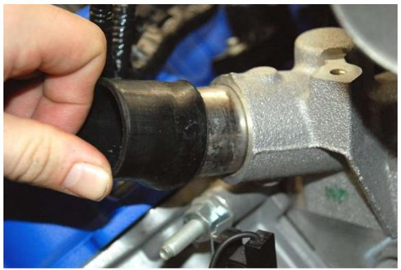
Use the smaller sections of tube inside the adapters to fit them to smaller fittings on the radiator and intake.
