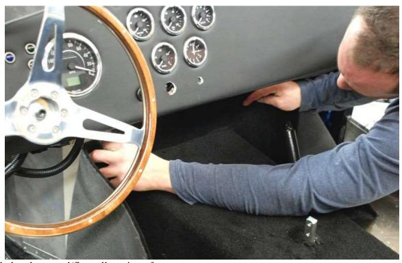
Fit and glue the tunnel/firewall section of carpet.
