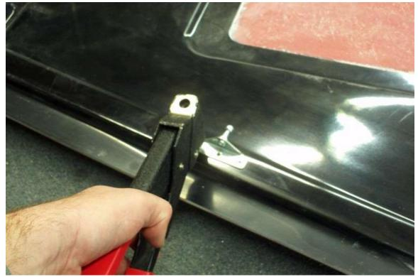
Install the ball pivots for the hood struts on the hood using  $\frac{3}{16}$ " rivets. The ball points toward the inside of the car.
