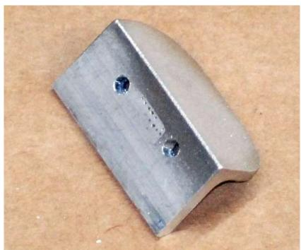
Drill the two holes just marked with a  $\frac{7}{64}$ " bit and file the edged of the bracket round with a file or grinder for a nice finish.
