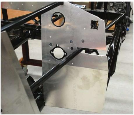
Mark, drill, and rivet in place the left side footbox front panel, do not silicone or rivet the right lower section that attaches to the 3/4" vertical tube in order to allow the inside wall to slip underneath.
