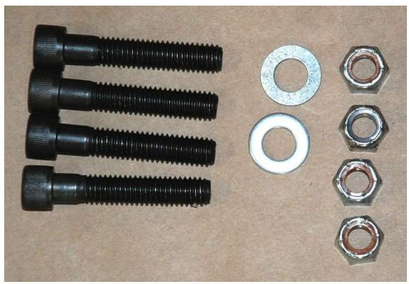
Unpack the fuel strap fasteners; <sup>3</sup>/<sub>8</sub>"x 2" socket head screws and locknuts.
