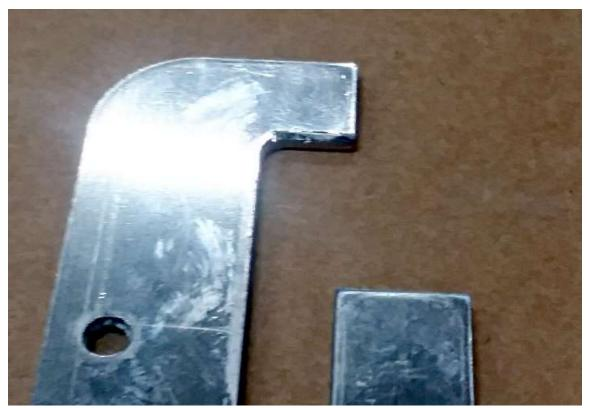
Make sure the base plate sits flat on the gasket, if it hits the side bar on the ends, file and angle on the end of the base plate.
