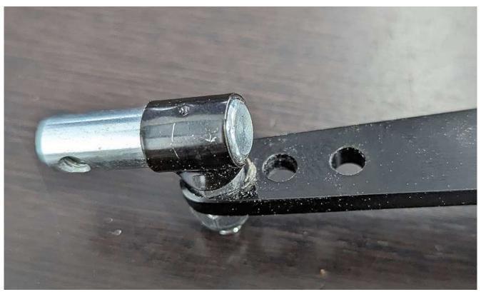
Attach the ball stud to the top hole in the pedal using a 5/16" wrench and 3/8" socket.
