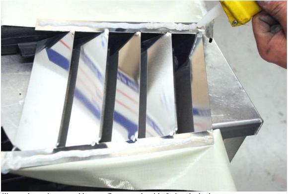
Apply silicone down the top and bottom flange on the side facing the body.
