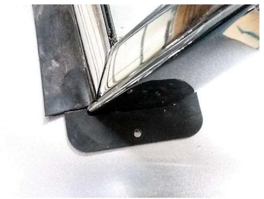
Put the rubber base plate gasket around the side bar and make sure the rubber does not go up onto the windshield bottom wipe. Trim the base plate gasket if necessary.
