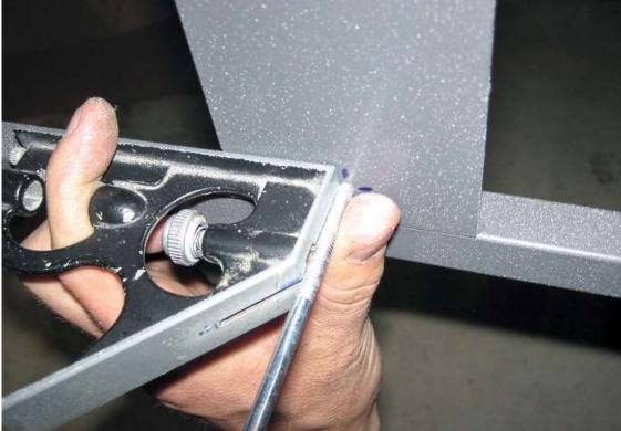
Put the pin screw through the body and up to the frame. Use a level and a square to locate the end of the screw.
