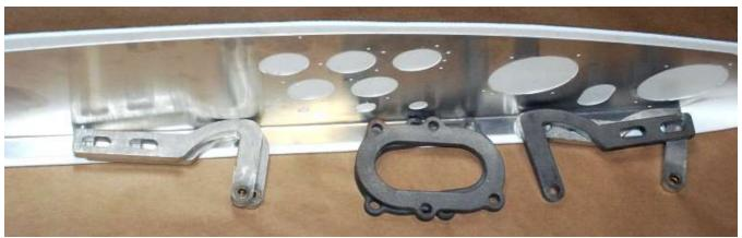
After giving the front adhesive time to set spray the bottom flange and pad and adhesive them together. This is a fairly tight corner so hold the dash in position with pressure on the mating surface with some full paint cans or something else heavy.
