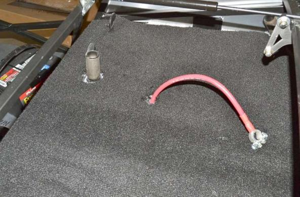
Pull the battery cables through the holes.
