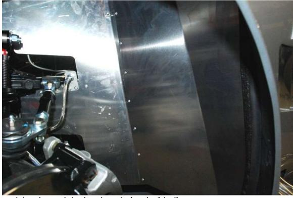
Silicone and rivet the panels in place down the length of the flange.
