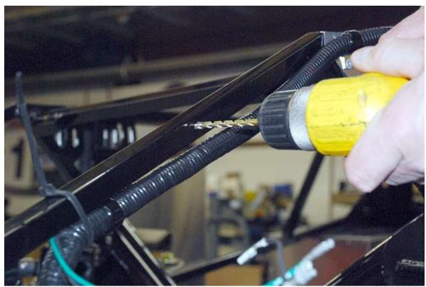
Locate the horns on the upper radiator down tube and drill a <sup>3</sup>/<sub>16</sub>" mounting hole.
