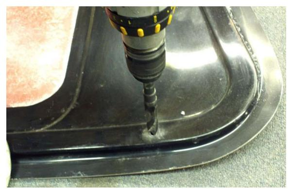
Drill through the hood and the liner starting with smaller bits working up to a \( \frac{5}{8} \) hole. The larger bits sometimes work better by running the drill in reverse so they do not tear the fiberglass.
