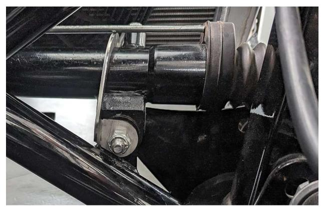
Tighten the locknut on the bolt.
