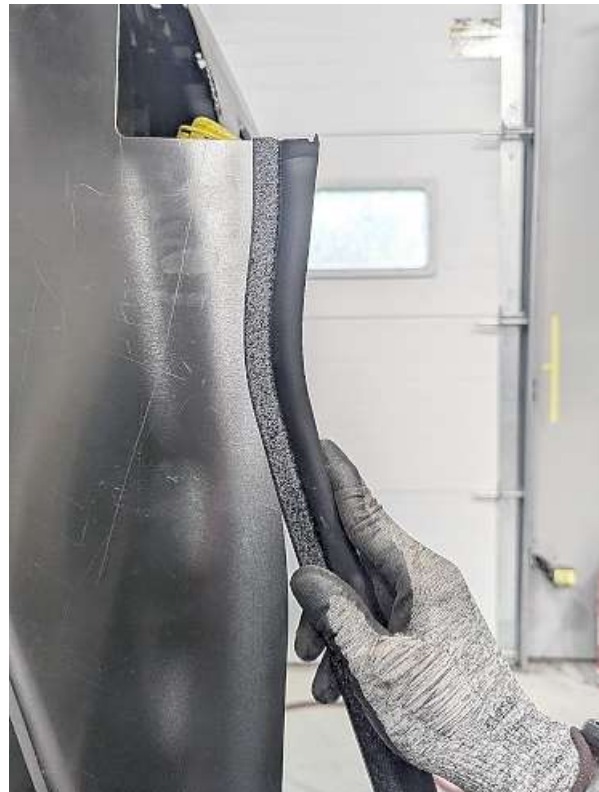
Push bulb seal onto the splash panel edges that will be against the inside of the body panels. Driver's side shown.
