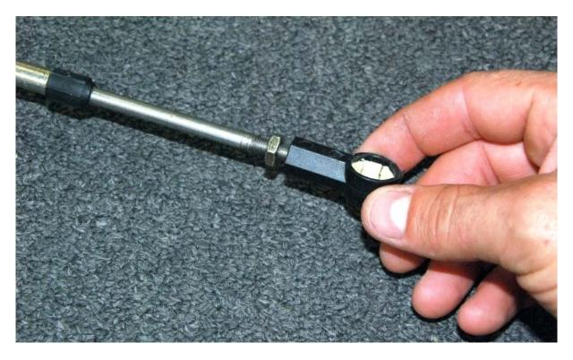
Attach the ball stud retainer to the end of the other control cable so that there are  $\frac{5}{16}$  of threads showing.
