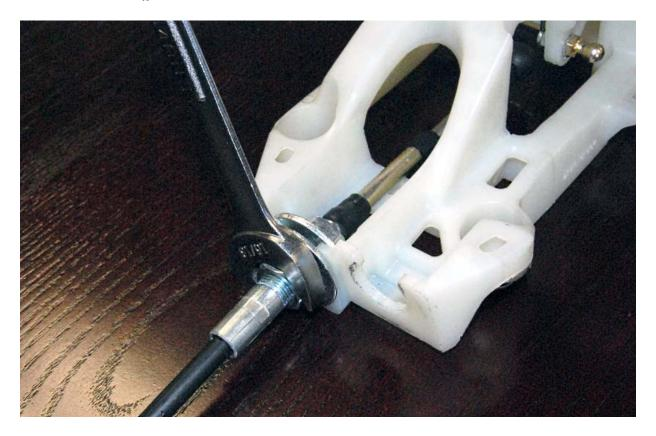
Attach the ball stud retainer on the other control cable to the ball stud mounted on the side of the shifter.
