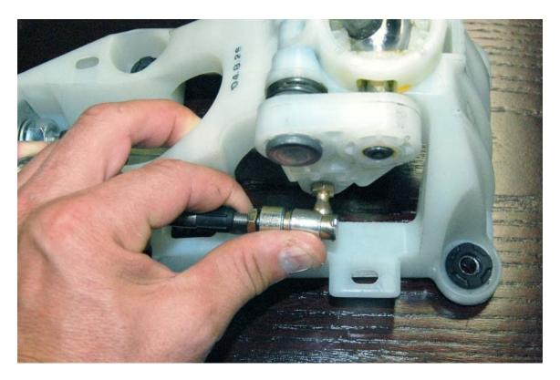
Making sure that the nut on the end of the control cable sheath is flush with the end of the threads, tighten the outside nut with a  $^{15}/_{16}$ " wrench.
