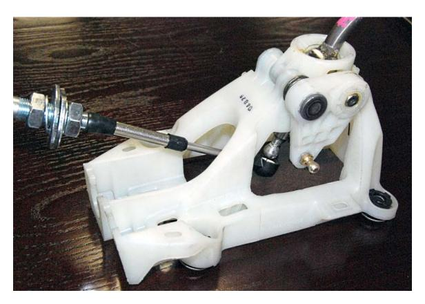
Attach the ball stud retainer to the ball on the end of the shifter handle.
