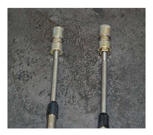
Mark the cable that goes into the center of the of the shifter at both ends for easy identification later.
