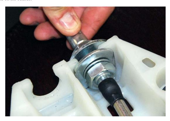
Making sure that the nut on the end of the control cable sheath is flush with the end of the threads, tighten the outside nut with a  $^{15}/_{16}$ " wrench.
