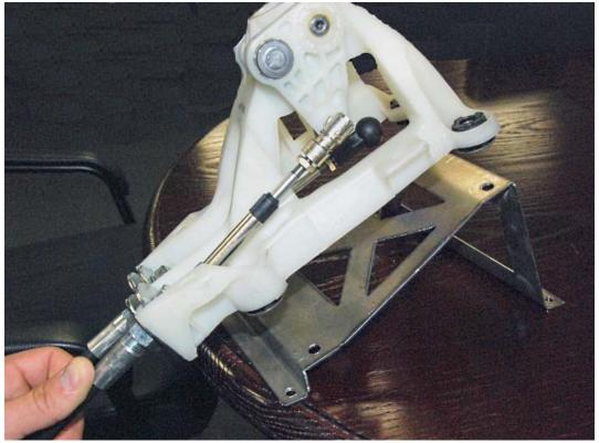
Attach the ball stud retainers from the transaxle onto the control cables.
