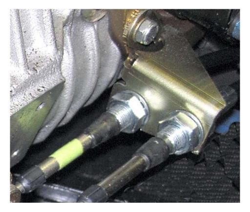
Attach the other control to the transaxle mount using a 15/16" wrench.
