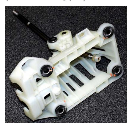
Use a saw to cut off the mounting post on the side of the shifter.
