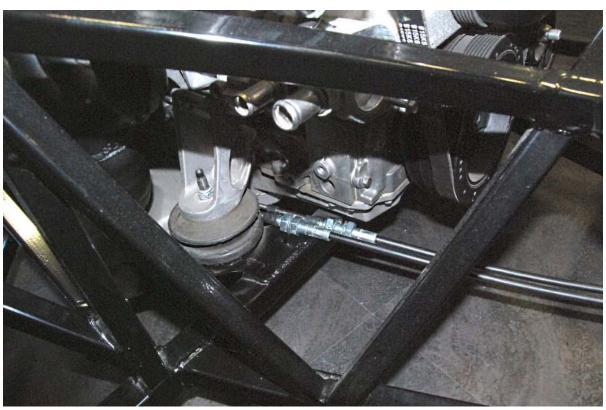
Insert the shifter assembly into the center tunnel and clamp the assembly to the frame as far back as the control cables will allow.
