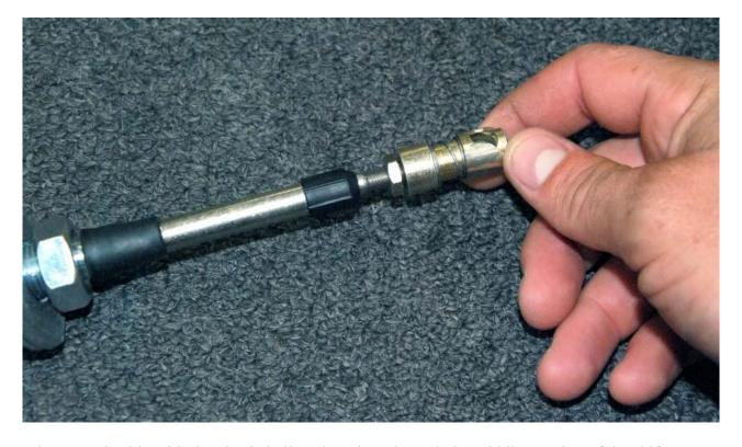
Pass the control cable with the plastic ball stud retainer through the middle opening of the shifter.
