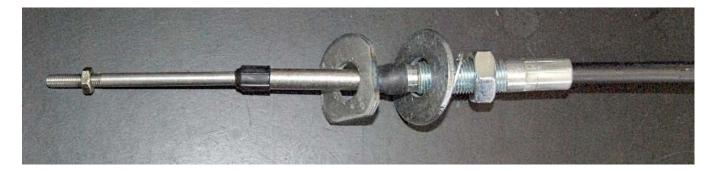
Slide the lock washer and nut onto the end of the cable. Leave the nut so that it is flush with the end of the threads.
