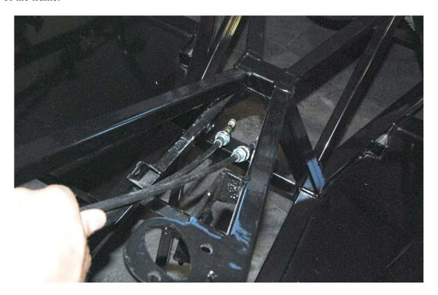
Pass the cables to the right side of the engine to the inside of the engine mount, under the CV axle to the back of the transaxle.
