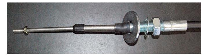
Slide one of the cut washers onto each of the cables.
