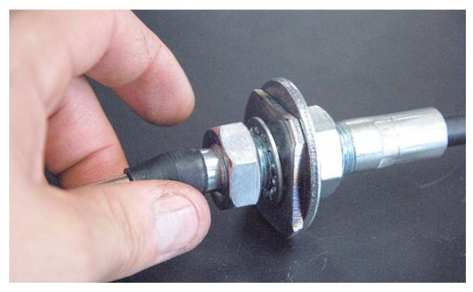
Attach the ball stud retainer to the end of one of the control cables so that there are  $\frac{3}{16}$ " of thread showing.
