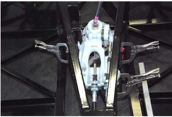
Use a marker to mark the shifter mount holes on the frame. Move the shifter forward for easy access to the mount hole locations.
