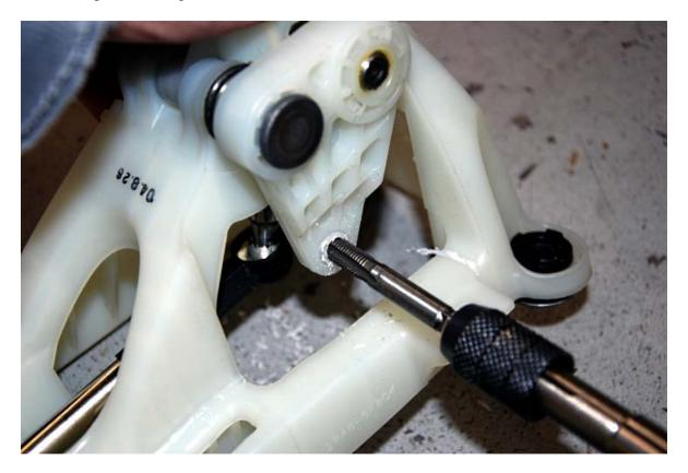
Attach the ball stud to the shifter using a  $\frac{3}{8}$ " socket.
