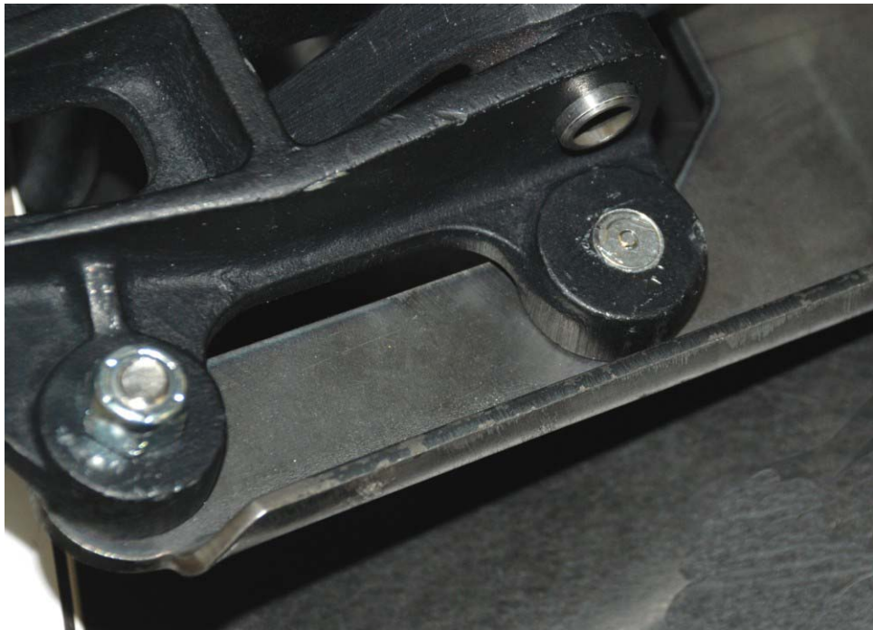
16. Attach the Clutch pedal stop mount to the bottom of the pedalbox using two 1/4" socket head screws, spacers and locknuts.
