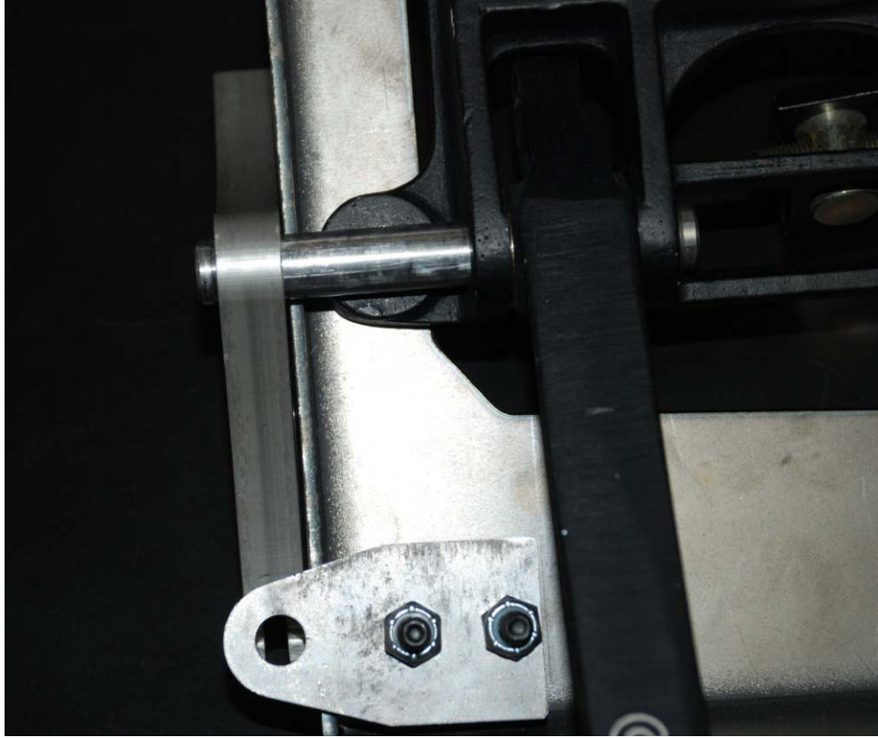
18. Put the remaining thin washer and snap ring on the pivot sleeve.
