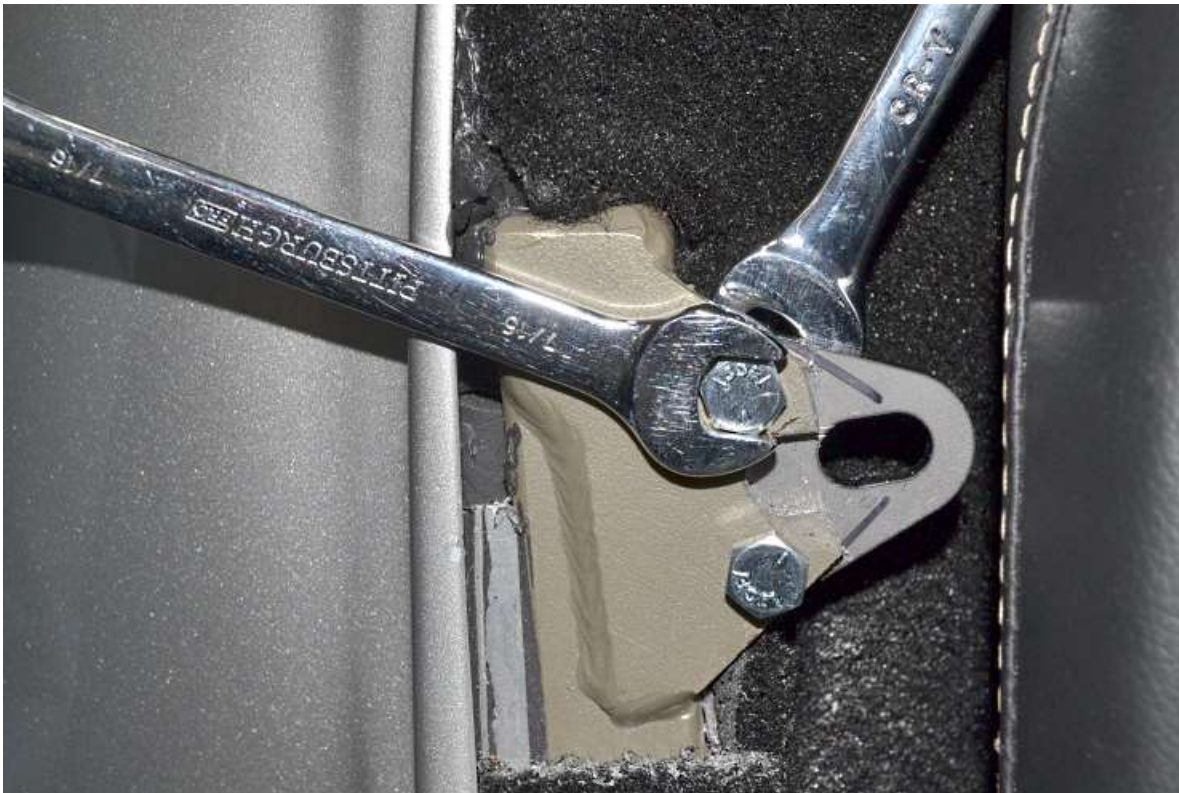
Attach the adapter to the back side of the frame tab using the \frac{1}{4} "x \frac{3}{4} " bolts and locknuts.
