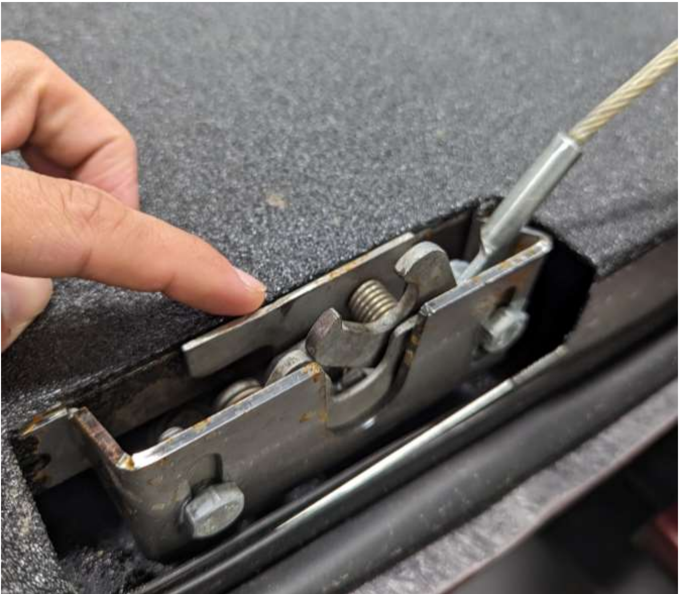
The OEM latches need trimmed to avoid sticking up past the inside surface of the tailgate.
