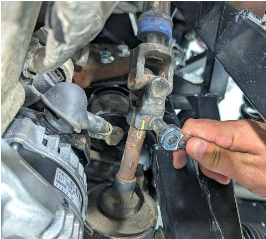
Tighten the lower steering shaft bolt to 22 lbft (30Nm) .
