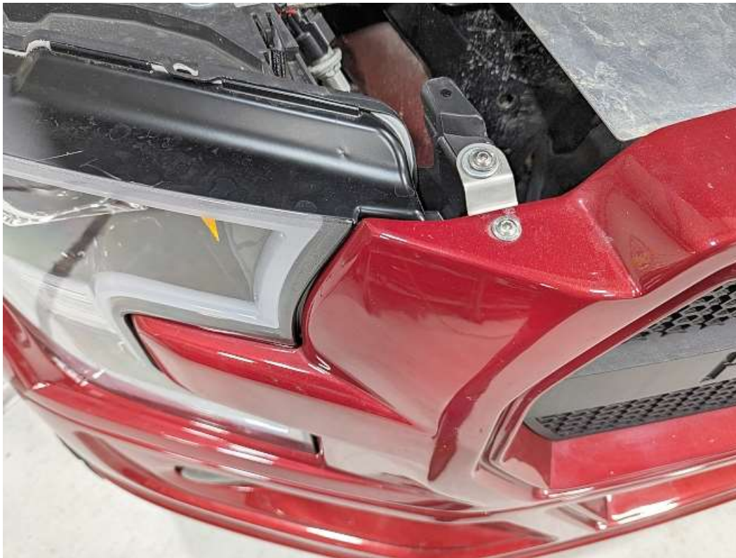
Attach the nose to the headlights at the top inside of the headlight using the 1/4" flanged button head bolts.
