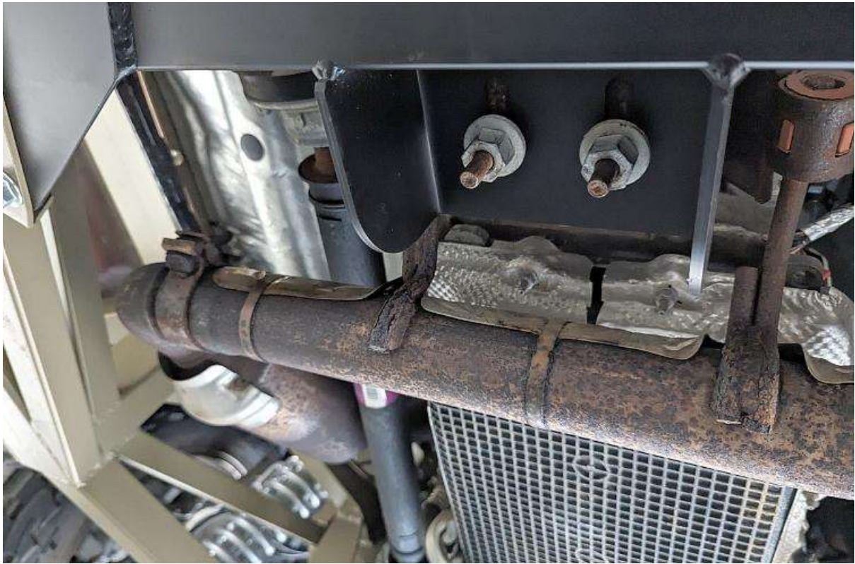
Attach the transmission mount to the frame using the OEM nuts.
