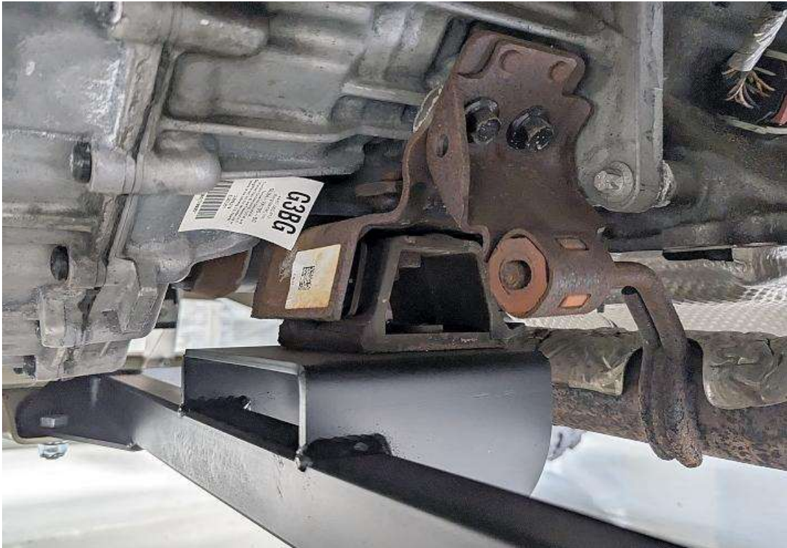
Set the transmission mount on the frame mount.
