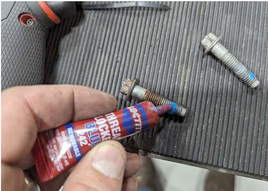
Put blue lock-tite on the OEM steering shaft bolts.
